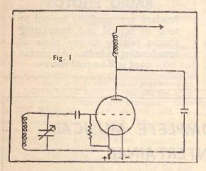
This radio frequency portion may be usefully employed by passing it, before grounding, through a coil which is inductively coupled to the grid tuning coil. Provided the connections are made in the proper direction, the effect will be to induce currents in the grid coil which add to the signal current and consequently the
