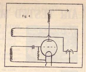
(c) Insufficient by-pass capacity between anode and ground (L. T. negative) is a common source of trouble which can be cured by condenser of .00005 to .0001 microfarad. Of course a differential reaction condenser obviates the necessity for a separate by-pass.
