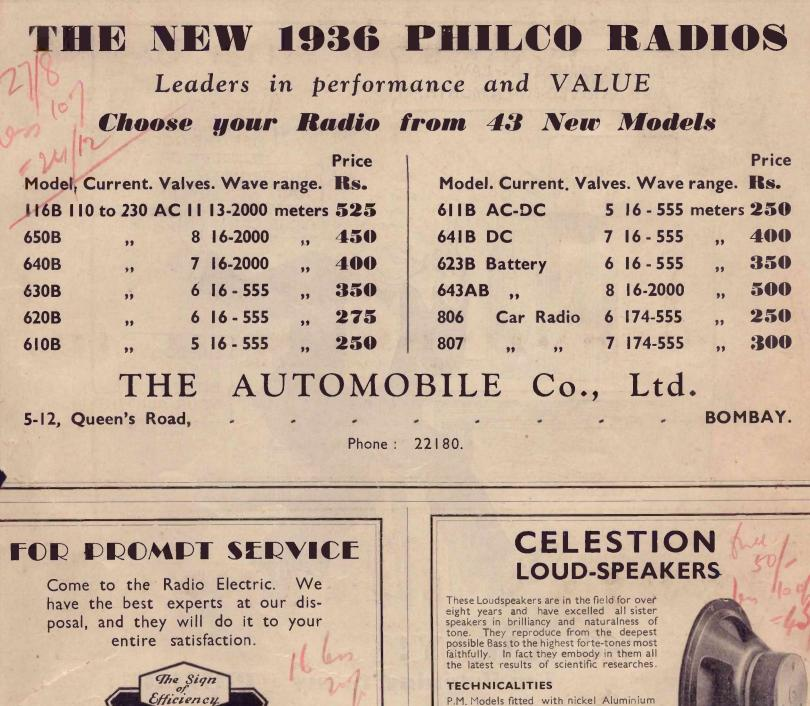
P.M. Models fitted with nickel Aluminium steel magnet of high efficiency and energised types with hum neutralising coils. Standard types fitted with comprehensive universal transformers having screw terminals and wander plugs to provide 10 high impedance ratios for ordinary output, 5 for push-pull output and 5 low impedance ratios up to 20 ohms.
