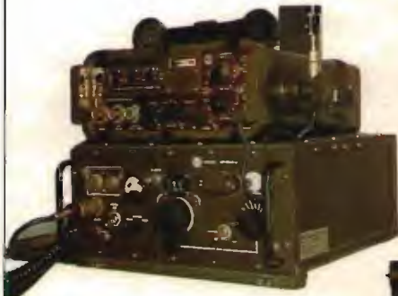
SOUTHCOM SC 130 - Ricetrasmittitore SSB. 2-12 MHz, 20 Watt out, con lineare SC 200A, 200 W. out.
