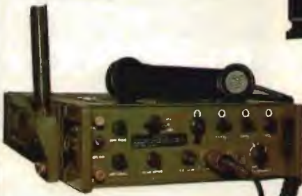
HUGHES - Aircraft ricetrasmittitore PRC - 74C - 2-18 MHz SSB 20 W. out.
