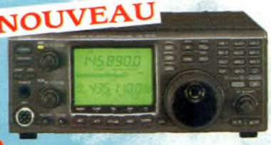
IC-910H VHF/UHF tous modes 100 W (VHF) et 75 W (UHF) Option 1200 MHz (10 W)
