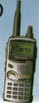
TH-D7E Portatif FM VHF-UHF Modem Packet 1200/9600 bds APRS
