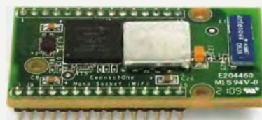
Obr. 3. WiFi modul Nano SocketWiFi™ s integrovanou anténou
