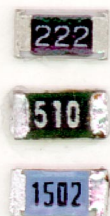
Obr. 3. Rezistory SMD shora: 2,2 k \Omega ( 22 \times 10^2 ), 51 \Omega ( 51 \times 10^0 ) a 15 k \Omega ( 150 \times 10^2 )
