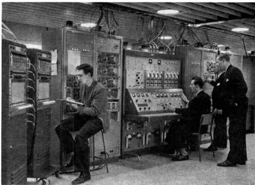
Early next year Britain's Minitrack Station at Winkfield, Berkshire, will be used to track two satellites, one American and the other Canadian. At left are: the phase recorders, phase measuring gear, control console and standard frequency/timing rack. The telemetry receiving rack is on the extreme right.
