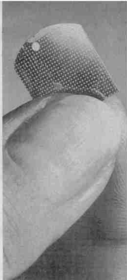
A glass seal, 1/10,000 inch thick, protects several hundred tiny diodes on this section of a silicon wafer. A new reliability seal technique, developed by scientists in IBM's Components Division, uses a special glass powder fired at temperatures exceeding 1500°F to produce a pinhole-free, chemically resistant surface.
