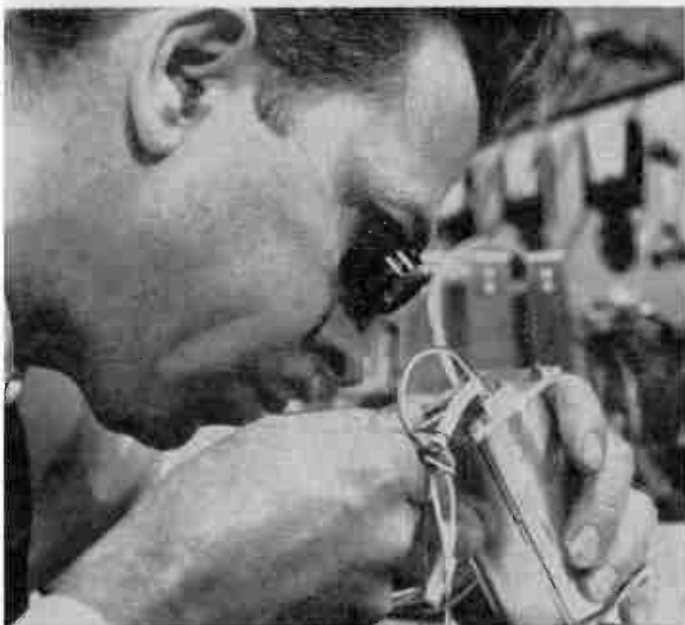
An engineer makes careful adjustments on gas bearing memory drum developed for space vehicles by Librascope Division of General Precision, Inc. This unit is utilized in the L-70 flight guidance computer. The memory drum spins on a thin film of helium gas replacing metal bearing suspension system of earlier computers.
