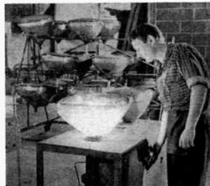
A new screen is applied to the old television picture tubes and the entire inner surface of the container is aluminized in a special process by Industrionics' technicians.
