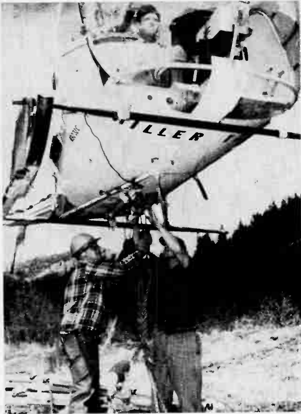
Figure 2. Hovering over staging area, Hiller 12E gets its 900 lb. cargo attached. Copter hook is released electrically by pilot.
