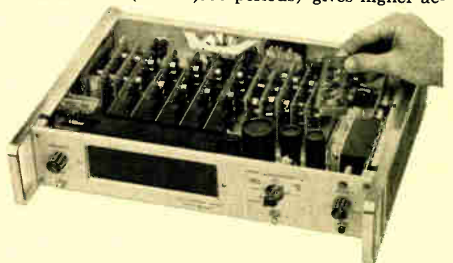
Note clean, compact, easy-to-service physical arrangement of new Ⓢ solid-state counters.
