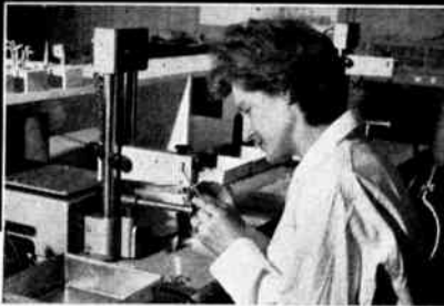
Contact welding with precision tool electrodes.
