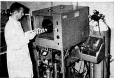
High vacuum oven for degassing and backfilling with inert gas.
