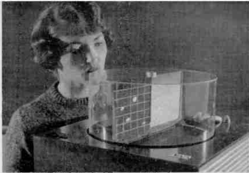
A three-dimensional display of lights for air traffic control, missile tracking, etc. was recently exhibited by International Telephone and Telegraph Corporation. The lights are visible from all sides and appear to hover or move through the display presenting a clear visual three-dimensional picture to the observer.
