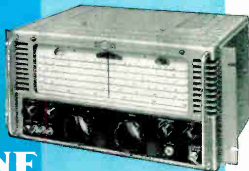
Model "730/4" General Purpose HF receiver. Developed to meet a Government specification and capable of an excellent performance. Range 480 kc/s to 30 Mc/s. (Special versions available giving crystal control and low frequency coverage.)
