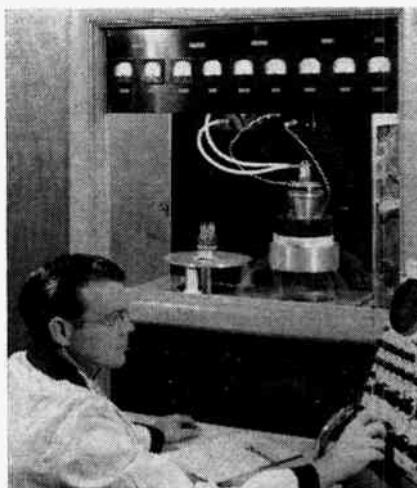
Technician adjusts oscilloscope at Canadian Marconi's new laboratory for pre-testing special purpose tubes. In the background is the pressure controlled test room in which tubes are tested under simulated operating conditions.
