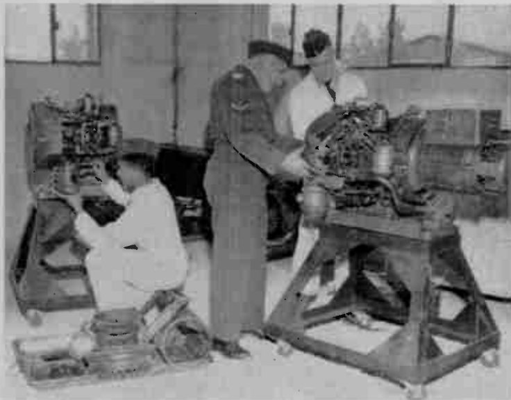
Dismantling and rebuilding auxiliary power units is the job of the maintenance workshop. Seen here working on two units are (left to right) Leading Aircraftman Joe Elliott, Corporal Colin Carnegie and Leading Aircraftman Ron Shettler.
