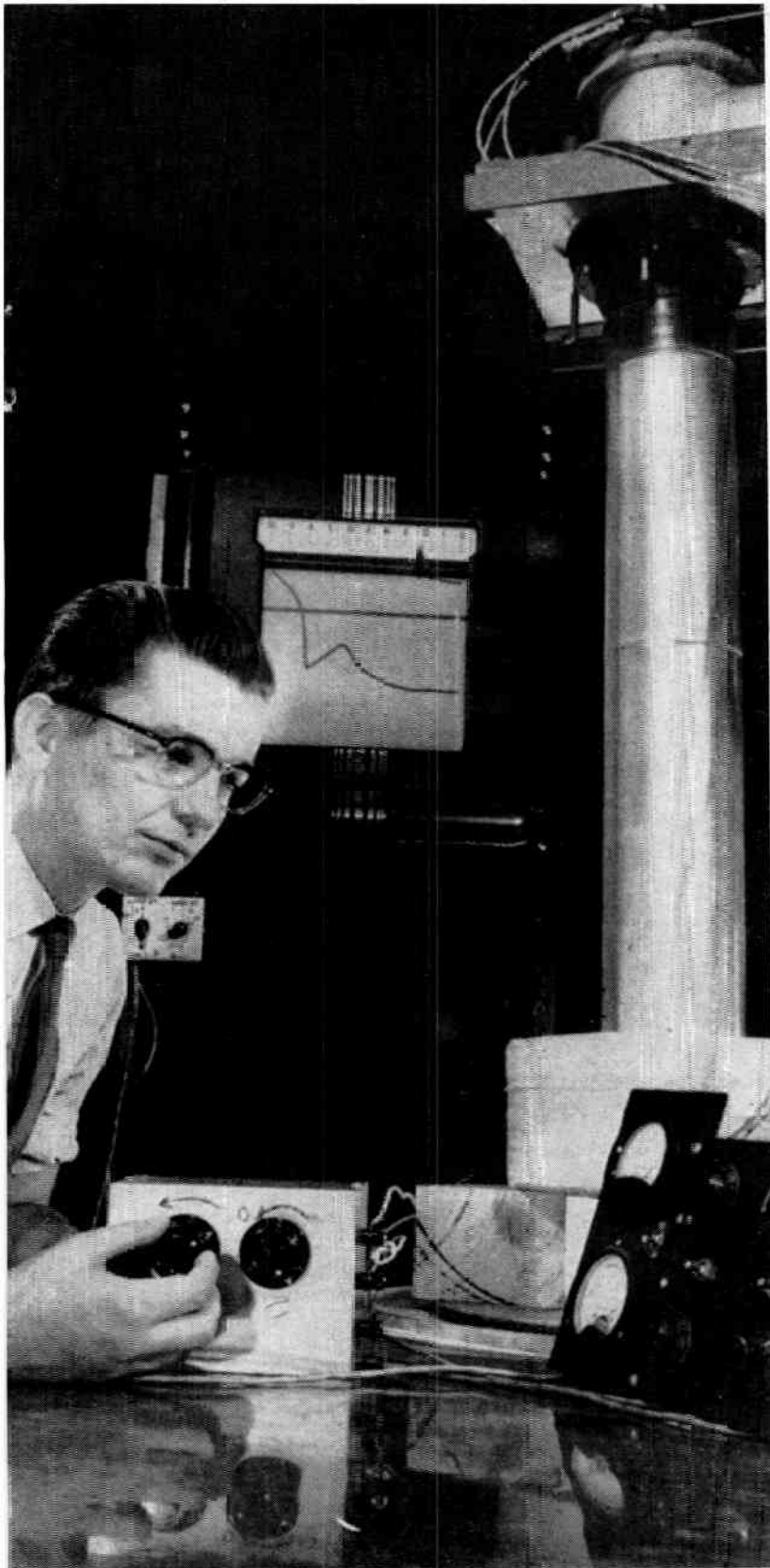
In the picture at left a scientist at General Electric Research Laboratory in Schenectady, N.Y., adjusts the voltage applied to a thin-film experimental device. In the background is the recording instrument on which a current-voltage curve has been traced. The dip in the curve marks the region in which negative resistance is observable.
