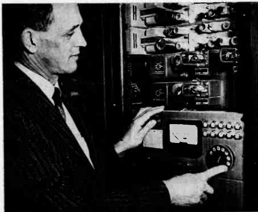
CHAB-TV Chief Engineer Merv Pickford has his finger on the dial that operates the RCA Victor remote-control equipment. The unique set-up supervises all functions of the transmitter, located 15 miles from the studio in Moose Jaw, without the use of wire lines.
