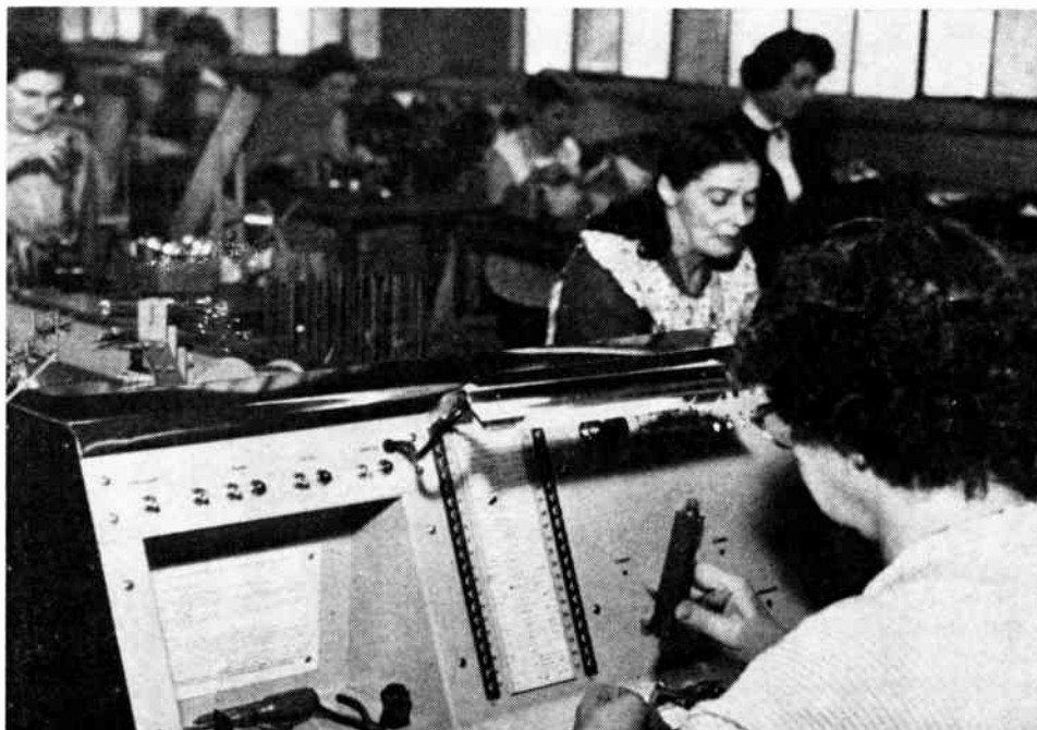
A view of the telephone instrument assembly line at TMC's London works. The instrument under test is seen "jacked-in" to the desk front of the automatic tester in the foreground.
