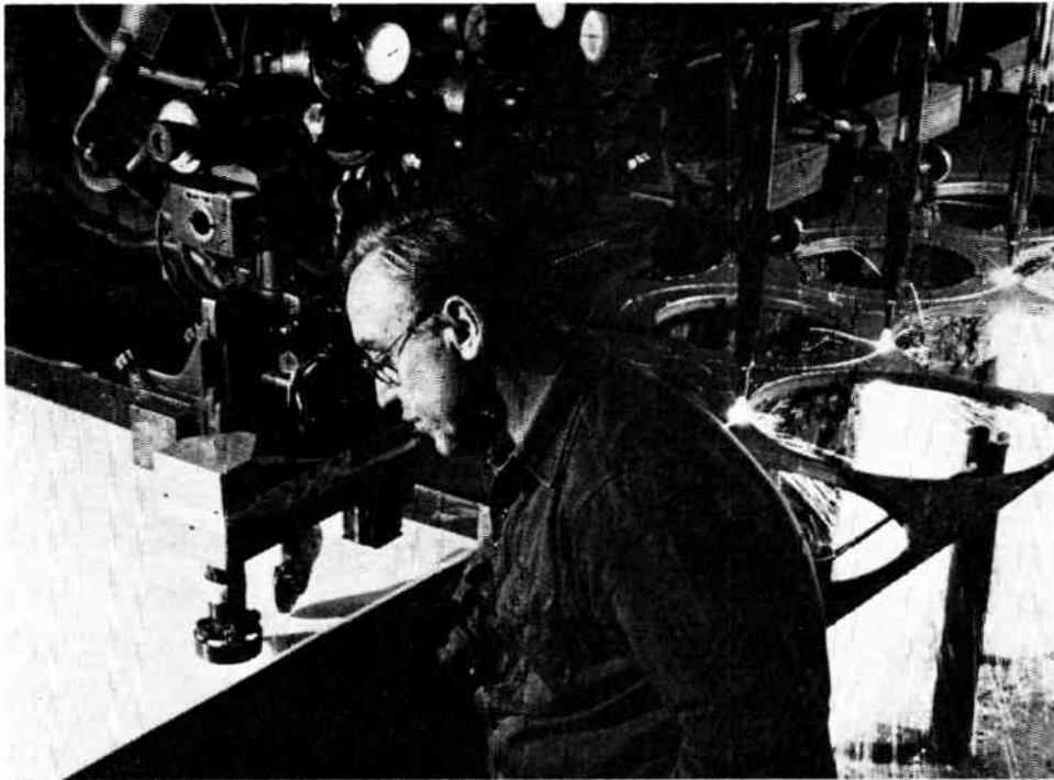
The "Linatrol" shown in operation automatically following the pencilled outline of a drawing while the torches to the right burn a true duplicate pattern of the master drawing.
