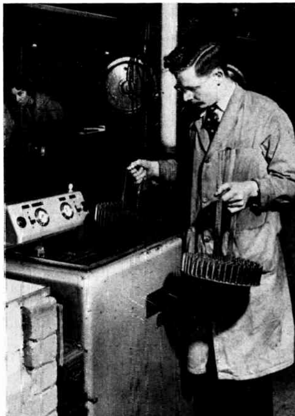
Caps for fountain pens being loaded into the Kerry-Mullard ultrasonic cleaning plant at the Newhaven, Sussex factory of the Parker Pen Co
