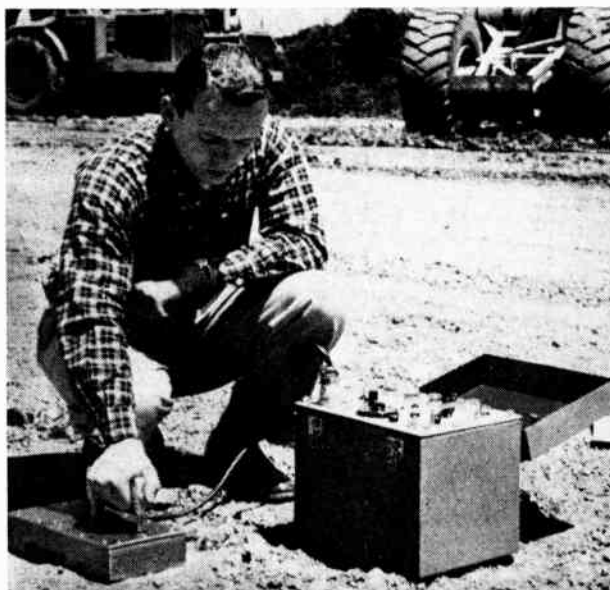
A complete d/M-gauge system for surface moisture or density determinations consists of a surface moisture probe or surface density probe (pictured above) and the portable scaler. Here the operator has placed the surface density probe on a relatively smooth part of the road surface and lowered the handle to the "use" position.
