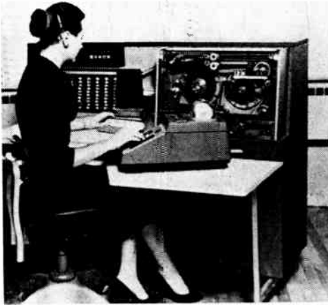
Here intermixed paper and card checks are received by operator at inscriber unit for inserting identification and amount on checks in magnetic ink.
