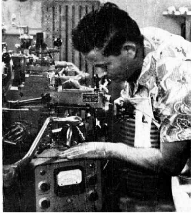
(Right) Vibration meter on tool post of turret lathe shows cutting-edge life shortened by excessive vibration.
