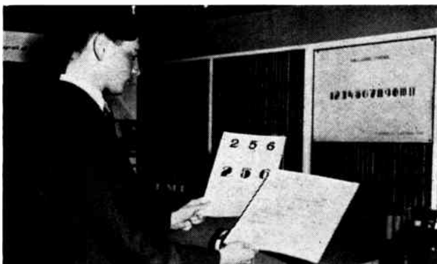
Figure 2. Operator shows a special typeface used by the reading device and examples of how cheques can be overprinted.
