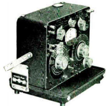
... panel tilts to any convenient angle
