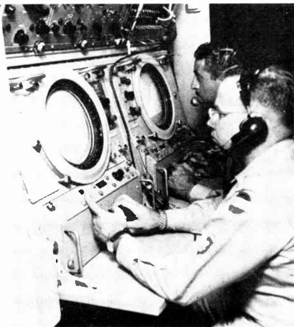
These two scopes receive target information from radome-encased antenna of Frescanar. Scope on left displays target range and bearing, that on right, altitude. Data is instantaneously transmitted to missile anti-aircraft batteries which automatically track down targets.
