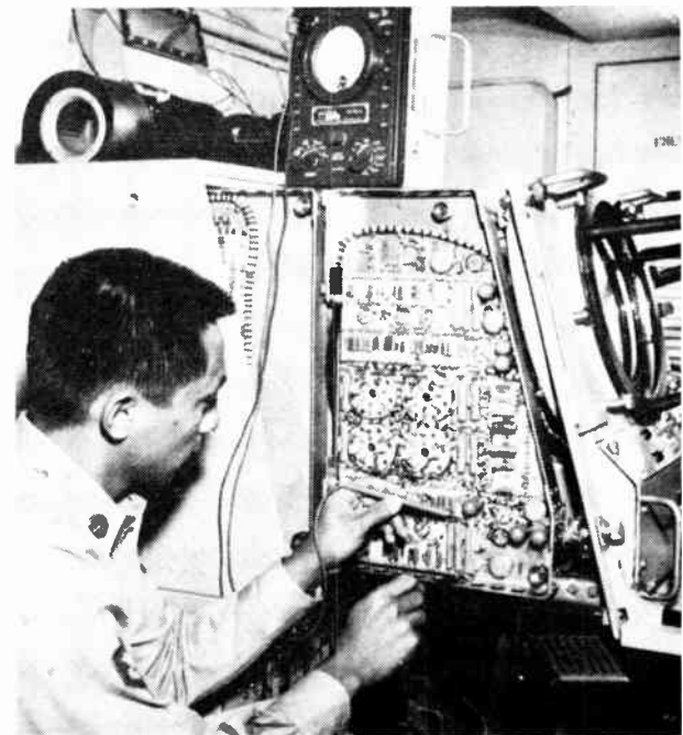
Entire console section of new three-dimensional radar slides out on rollers for easy maintenance. Here specialist uses voltmeter to check resistors in electronic circuit. Interior of radar trailer contains dozens of "cards" with printed electrical circuits that can be replaced instantly.
