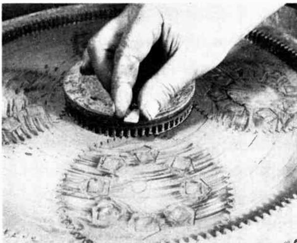
Figure 2. Lapping brings quartz crystals down to final thickness, sometimes no more than 0.002 in. All traces of oil and compound must be removed if crystal is to function dependably.
