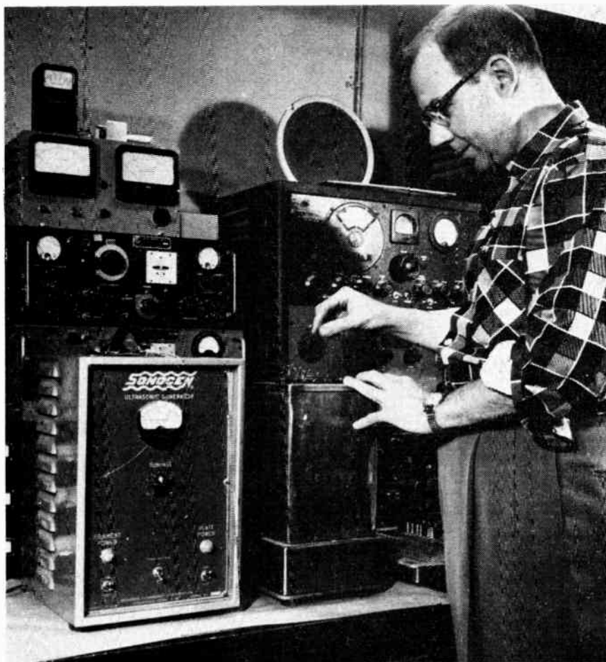
Figure 1. Ultrasonic generator (left in photograph) produces high frequency (38 kc) vibrations which are sent to transducer in bottom of stainless steel cleaning tank. Cavitation produced in liquid removes all vestiges of oil, dirt, dust, contaminant which would interfere with operation of crystal.
