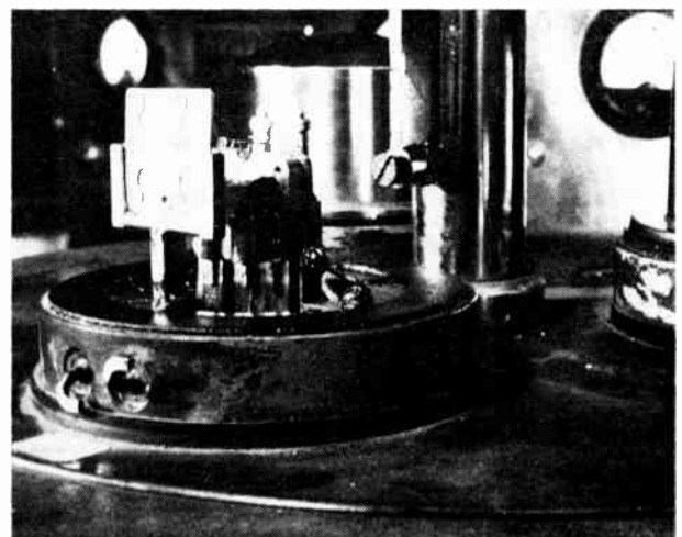
Figure 7. After cleaning, silver contacts are vacuum-plated onto crystals. Holder can handle four at one time.
