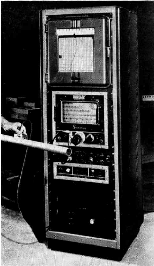
Figure 1. General view of the self-contained ultra-sonic gage for automated production.
