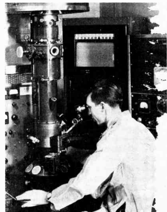
● An electron microscope, modified for analysis by X-ray emission spectroscopy of areas a few microns in diameter in steel specimens, is shown being focused by a scientist.
