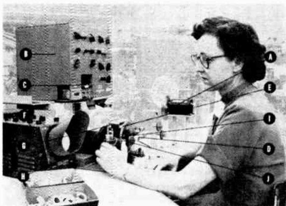
● Fig. 3: A complete toroidal winding installation. The principal components of the equipment are: (a) turn counter and loading pulleys; (b) inductance measuring panel; (c) standard coil; (d) tension arm; (e) shuttle; (f) oscilloscope; (g) winding machine; (h) core holder; (i) tension pin; and (j) core.
