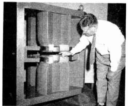
Indiana's C. A. Maynard inspects air gap of giant Alnico V magnet assembly
