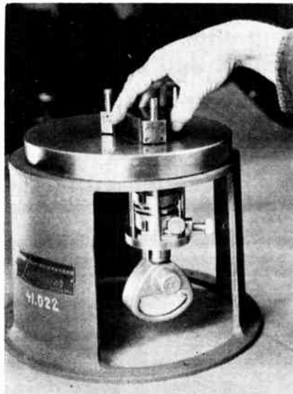
● Fig. 2. Final setting of diamond point to microinch accuracy.
