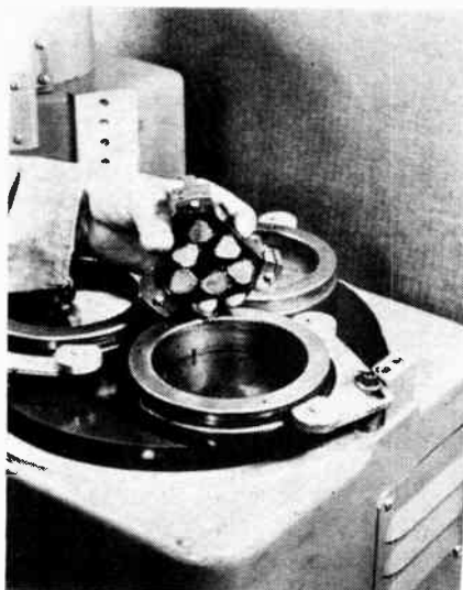
● Fig. 4. Diamond fixture with germanium wafers attached being placed on Model 12 Lapmaster for final side lapping operation to a thickness of .003" \pm .0005".
