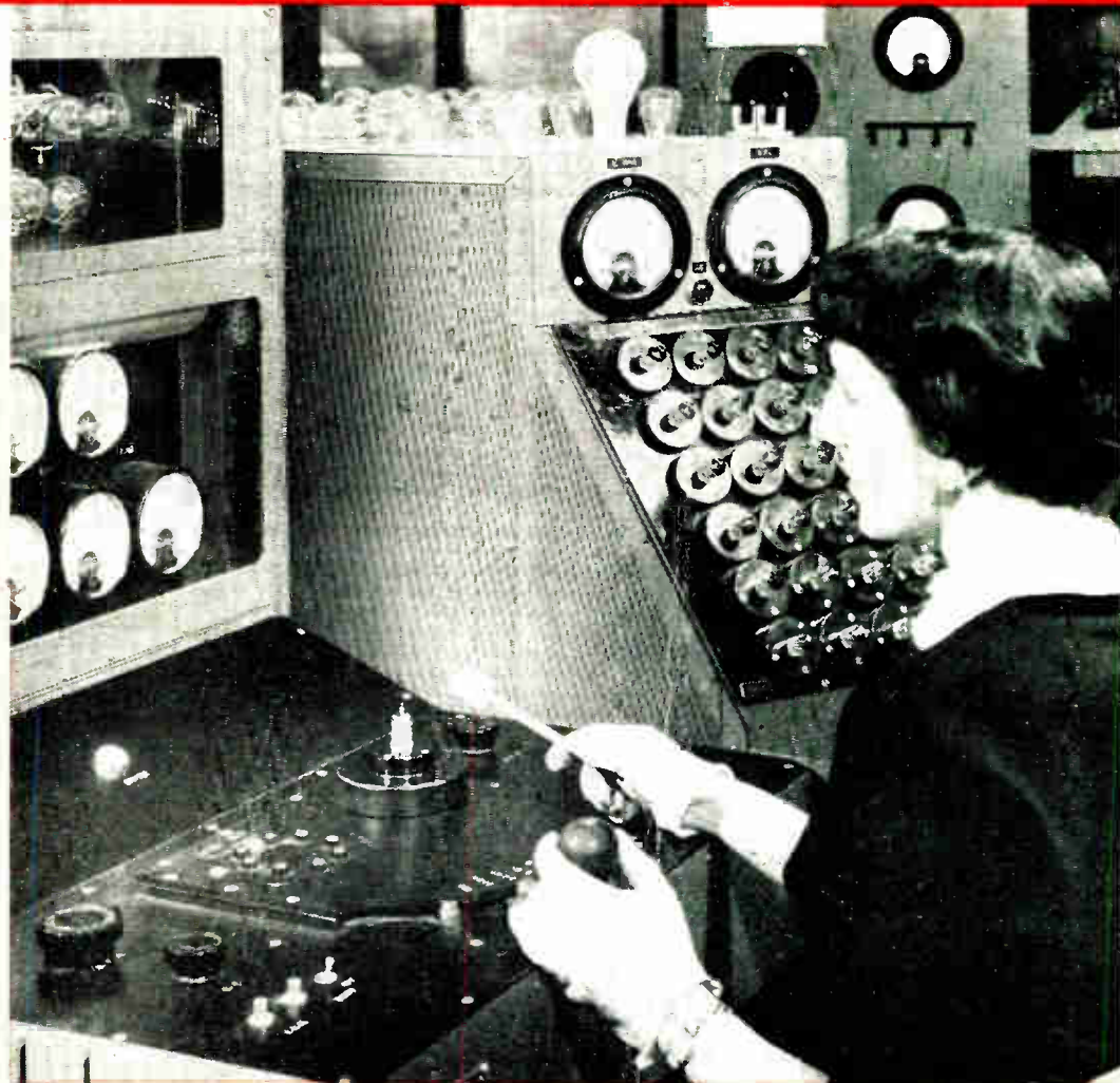
The mass production of miniature vacuum tubes used in television and radio receivers is now in full swing in Canadian plants. The above photo shows a characteristic testing unit where the tiny tubes receive a thorough inspection before being given their final check out.
