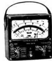
625-NA The First V-O-M With 10,000 Ohms/Volt AC
