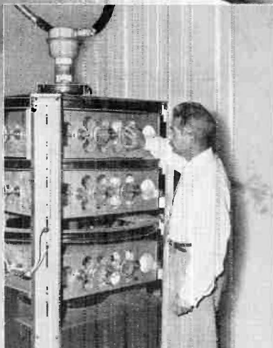
Eimac X590D amplifier klystron with circuit components permit ease of transmitter design by equipment manufacturers
