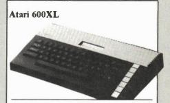
Operating BASIC System: Processor(s): 6502C RAM: 16K Printer I/O: Serial
