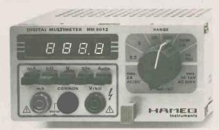
This digital multimeter measures voltage, current, and resistance with **increased accuracy and resolution** (4½ digits, 10 $\mu$ V), featuring professional **autorange** convenience. Measurements are taken periodically at 0.4s intervals. **True RMS** capability provides more accurate AC measurements on distorted, noisy, random, or other nonsinusoidal waveforms. 100ms integration time effectively eliminate adverse influence from line power disturbances.
