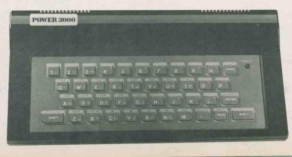
Yes, I did mention a speaker. As there is no true tactile feedback to the rubber keys, each keypress elicits a small 'bip' from the speaker to assure you that the struck key registered. After you pick up your typing speed, however, the audio feedback starts to sound like a bad rendition of *Popcorn*. Typing a quick 'NOBEEP' will silence the cacophony.
