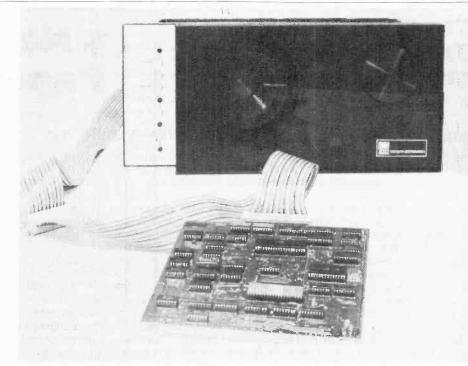
gaps and file marks. The tape decks are available in the three usual sizes with 7, 8½ or 10" reels. They operate on 115 or 230 VAC or, optionally, on 28 VDC. For more information contact: Mr. Bob Morgan, Sonotek Limited, 2410-5 Dunwin Drive, Mississauga, Ontario, L5L 1J9. Telephone 416-828-6810.
