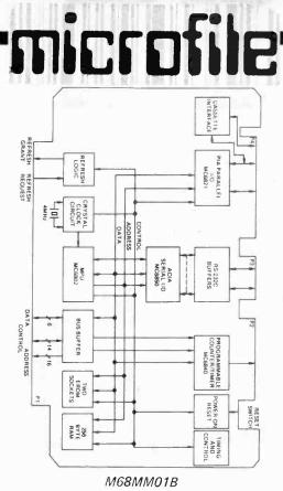
provisions for off-board dynamic memory refresh, an asynchronous communications interface adapter
