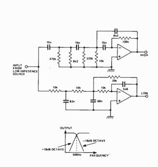
The circuit shown is for a two speaker system having a crossover frequency of 500 Hz. The filter structures are third order Butterworth multiple feedback, low pass and high pass. (Third order implies that roll off slopes of  $\pm 18$  dB/octave are obtained.)
