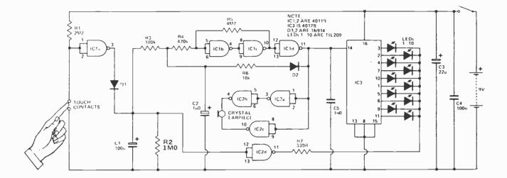
Fig. 1. Circuit diagram of the Wheel of Fortune.
