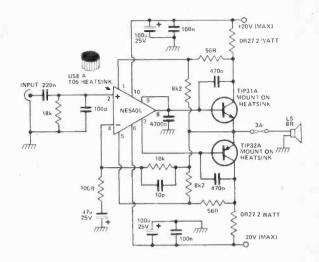
An audio power amplifier can be constructed from a power driver op amp plus a pair of transistors. The power driver is a NE540 made by Signetics. It generates quite a bit of internal heat and so a TO5 heat sink is required. Note that this design uses five stabilising capacitors.
