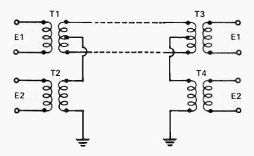
Fig. 2. Basic Simplex circuit, sometimes called "Phantom". Originally used in opera broadcasts.
