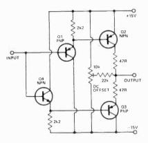
When you want to buffer a test generator to the outside world it is often very difficult to get an amplifier with sufficient bandwidth and power handling to do the job. The circuit is a very simple unity gain buffer. It has a fairly high input impedance, a 50 ohm output impedance, a wide bandwidth and high slew rate.
