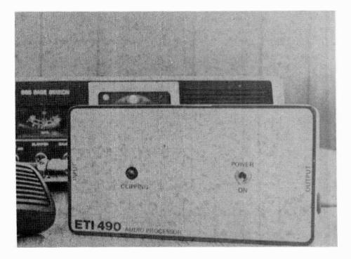
drastic change in its output. To overcome this a variable gain amplifier can be used which senses the average speech level and adjusts its gain accordingly for a constant output voltage. The compressor operates with a fast attack (gain reduction) and a slow decay (gain increase), to quickly respond to the voice while remaining at this level to prevent amplification of background noise during speech pauses.
