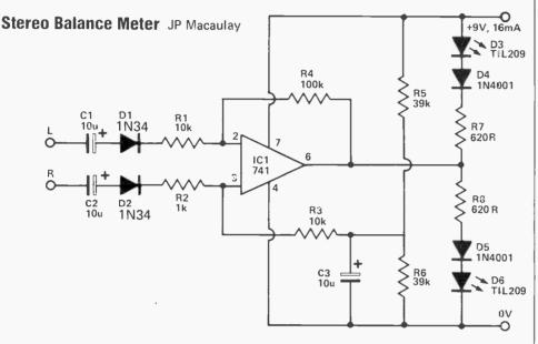
One of the more irritating aspects of owning a stereo system is the need to keep both channels in balance. What often sounds right when adjusting the controls turns out wrong when resuming one's normal listening position.
