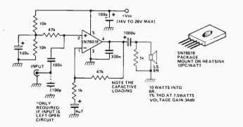
This is a very simple and inexpensive monolithic power amplifier made by Texas Instruments. It comes in a package that looks like a plastic power transistor with five legs.
