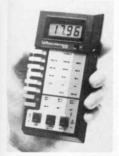
The meter offers 20 ranges of DC or AC voltage and current and resistance measurements, including both high and low resistance excitation capability. Ranges, functions, and excitation level are selected using pushbutton switches, allowing one-handed operation. Measurements including appropriate polarity sign and decimal points and a warning indicator for low battery voltage are displayed on a 31/2 digit, 0.5" high, liquid crystal display.
