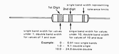
Fig. 9. This code varies the widths of the first two bands to indicate the position of the decimal point in the value. The code is read from left to right, as is conventional.
