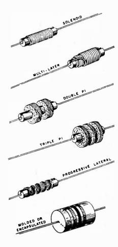
Fig. 1. General range of constructor styles of RF chokes. The particular style employed depends on the required or allowable component. Size, the inductance, the application and the required characteristics. the result that it has a very weak stray field, reducing 'crosstalk', or coupling, between the choke and adjacent components. In fact, two chokes can be mounted so that they touch each other over the full length of the bobbin – and crosstalk attenuation is guoted as 60 dB.
