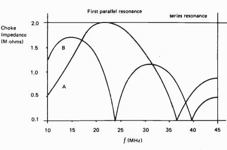
Fig. 4. Typical behavior of two RF chokes (A = around 10  $\mu$ H, B = around 40  $\mu$ H) over a range of frequencies.
