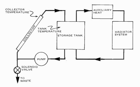
Fig. 2. Space Heating. A radiator system is shown here. This is essentially similar to the water heating system shown in Fig. 1.. However, it is not necessary to keep the two liquids apart. Thus, as long as your collector liquid is compatible with your rads, the tank can simply be a common storage tank for both circuits. The control system is similar to that of Fig. 1. as are the commonly used turn-on and turn-off differential figures.
