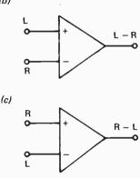
Fig. 4. Extracting Difference Signal. (a) Differential Amp. (b) and (c) Block diagram of differential amps.
