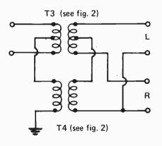
Fig. 5. Recovery of L and R signals in Simplexed sum and difference system.
