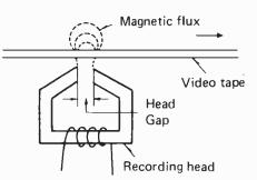
Fig. 1 — The record/playback head is simply an electromagnet. The small slit is called the head-gap and is the portion of the head that actually contacts the tape.
