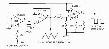
repeated. The ramp rate is determined by the size of the current IABC is linearly proportional to the oscillation frequency. At very low currents the triangle waveform may become very asymmetrical. This is due to current mirror mismatches inside IC1 and this device may have to be specially selected for continuous symmetry.
