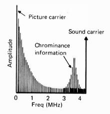
Fig. 15 — The line-by-line phase inversion of the chroma signal causes frequency interleaving which allows the comb filter to be used to separate the chroma information.
