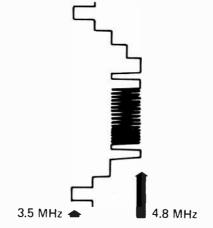
Fig. 12 - An FM carrier allows the entire video spectrum to be recorded with less than 1 octave of bandwidth.
