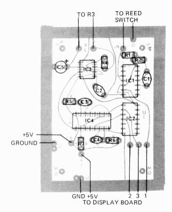
Component placement diagram for main and display boards.
