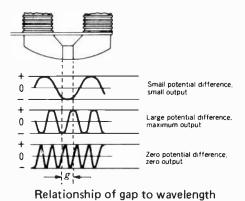
Fig. 3 - Cancellation reduces the output of the head if the wavelength of the signal on the tape is shorter than twice the gap width.
