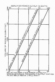
Fig. 1. Graph relating room size to required amplifier power.
