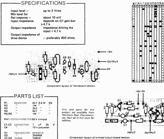
Nine volt battery and clip Veroboard or pc board ETI 071. Veroboard, and perhaps the name of a local supplier may be obtained from: Electronic Packaging Systems, P.O.Box 481, KINGSTON Ontario, K7L 4W5
