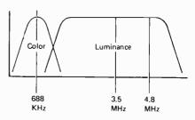
Fig. 13 — The frequency of the chroma information is converted to a lower frequency by hetrodyning.
