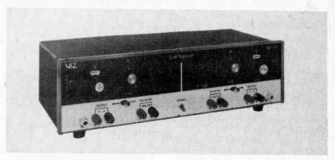
The unit has current-limiting overload and short-circuit protection; each output has its own LED to indicate an overload, and its own reset button.
