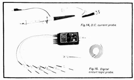
in Fig. 15. Power for the gate is obtained from the circuit under test
