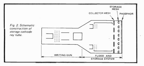
It is called a variable persistence storage tube and is a development of early 1950's storage tubes in which the waveform could only be held at a constant intensity (without the feature of gradual fade out). In fact variable persistence is a feature of tube operating circuitry not the tube itself.
