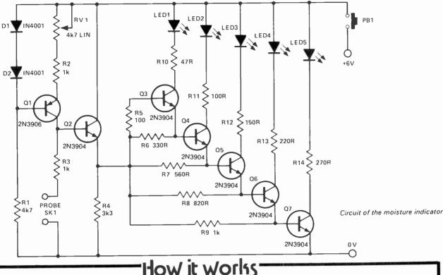
Fig.1 is the basic diagram of the system. A constant current (preset to suit local soil conditions) through the probe tips, and the moist soil, produces a volt drop that is proportional to the resistance of the soil. This voltage then turns on an LED, which typically requires some 2 V at 15 mA for adequate brightness. A soil
