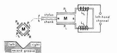
Figure 1. The workings of a moving magnet cartridge, which in this case is a Philips 412. The bar magnet is marked 'M', and PL and PR are the pole pieces for each channel.
