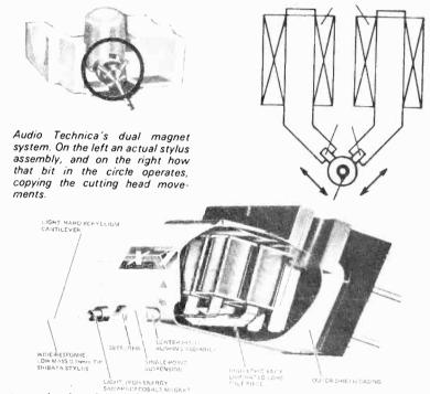
A cutaway drawing of the JVC XI cartridge. This device has an extended h.f. response to allow it to produce CD4 records, a task for which it has become the standard machine!
