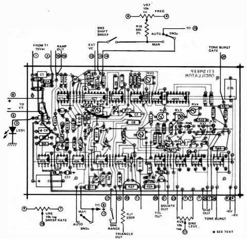
Fig. 8 Overlay and interconnection pattern.
