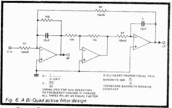
Figure 6 shows a Bi-Quad active filter. It looks very similar to the state variable filter, but the small changes make it behave quite differently. It only has a bandpass and a low pass output. The resonant frequency is given by
