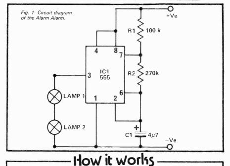
The 555 IC is used as an astable (i.e. not stable) multivibrator. As soon as it is connected to the supply it starts to oscillate (slowly in this case) and the output voltage at pin 3 changes regularly and suddenly from high to low and low to high as the capacitor is charged and discharged.
