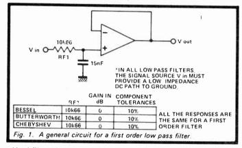
Key' filters have been used as the basic building blocks. If operation at a frequency other than 1kHz is required, then the resistor/s Rf should be scaled accordingly, (the Rd resistors are not altered). For example, if operation is required at 250Hz, then the Rf in the chart must be multiplied by 1000
