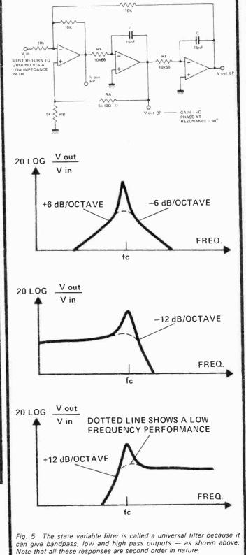
The Q is determined by the ratio of two resistors, RA and RB, where RA/RB = (3Q-1). The resonant frequency fc =
