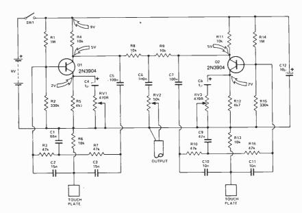
Fig. 1. Circuit diagram for the bongo circuit. Note that the voltages given around the circuit are all with respect to ground, and are intended as an aid to fault finding.
