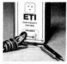
NOT your hackneyed multivib with a break in the supply rail but a properly designed unit which will tell you if there's continuity and very little else — no voltages to turn on transistors etc.
