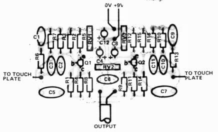
Above: The component overlay for the design. The board is symmetrical which may or may not make it easier to get working as there is a good chance one half will work first time! No case details are shown as the board will probably be built into something else. Below: The foil pattern, shown full size.
