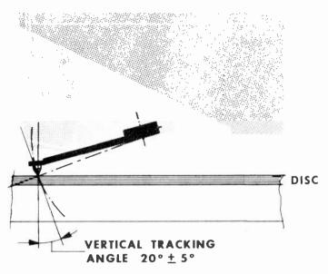
Fig. 3 Vertical tracking angle
