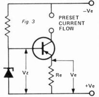
the collector current too) is thus defined as Ie = VeRe and by selection of Re the value of Ie (or Ic) is determined. As long as there is about one volt between emitter and collector the collector current remains constant at this chosen value - or at least until a resistor or load of too large a value is connected and so robs the collector of its working voltage.
