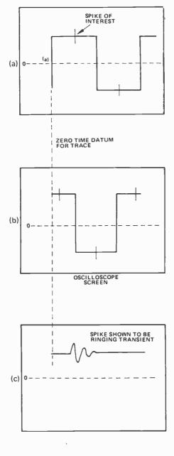
Fig. 8. Use of introduced delay in triggering to enable an event away from trigger transient to be investigated.
