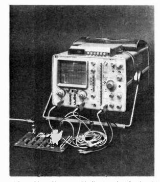
The H.P. 1715A oscilloscope with direct readout for time interval measurements.
