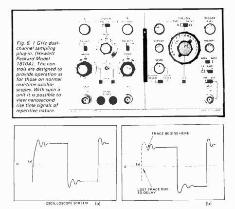
Fig. 7.Inherent trigger delay, if not compensated for, will lose the leading\_edge of a waveform.
