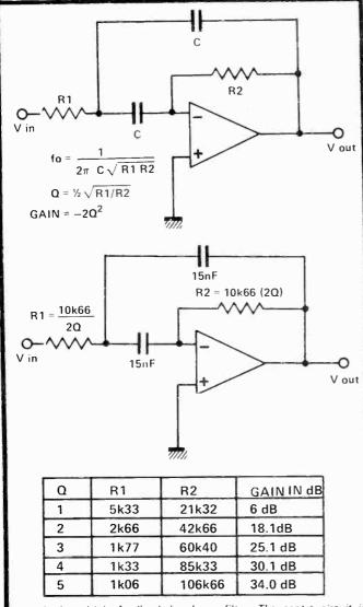
Fig. 4. A multiple feedback bandpass filter. The centre circuit is normalised for 1kHz. The table is the design table for this circuit. To change the centre frequency change  $R_1$  and  $R_2$  by an equal factor
