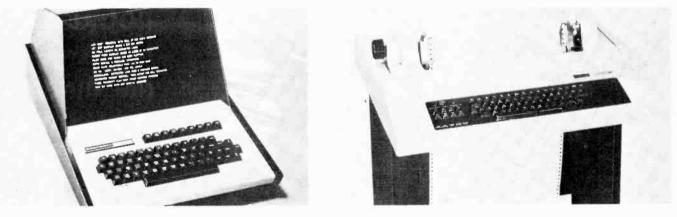
button program loading or storing. The H11 is a 16-bit computer using the Digital Equipment Corporation (DEC) LSI-11 with 4k memory, a built-in backplane and regulated switching power supply. System compatible peripherals include a CRT terminal, paper-tape reader/ punch, serial and parallel interfaces, a "hard-copy" printing terminal and a cassette player/ recorder. Input/output interfaces, additional memory and supple-
