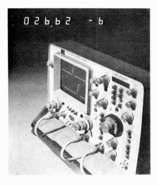
The H.P. 1743A oscilloscope with built in averaging counter
