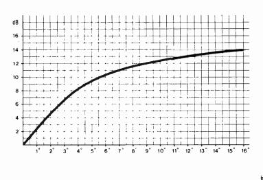
Fig. 1 Channel separation deteriorates if the cartridge is not perpendicular to the record.
