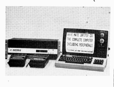
*Fig. 5. The Jupiter II is a 6800-based computer built using wire-wrap cards. Again, a VDU is the prime method of communication with the computer.*
