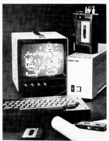
Fig. 3. The Poly-88 is a 'front-panelless' computer and uses a built-in VDU to control its operation.
