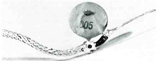
Photo 23 — Proper method of by-passing the end of a shielded lead using a disk ceramic condenser. A 0.001 ufd. to 0.005 ufd should be used for 1600 volts or less; 500 uuf. at higher voltages. The leads are wrapped around the inner and outer conductors and soldered so that the lead length is negligible.
