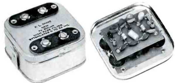
Photo 29 — Inside and outside views of new Drake Type TV-300-HP filter. This filter is the new type that cuts off at 52 Mc. and therefore gives protection to TV receivers from adjacent channel TVI from 50 to 51 Mc. amateur stations. It also, of course, works on all other lower frequency amateur bands as well as commercial stations.
