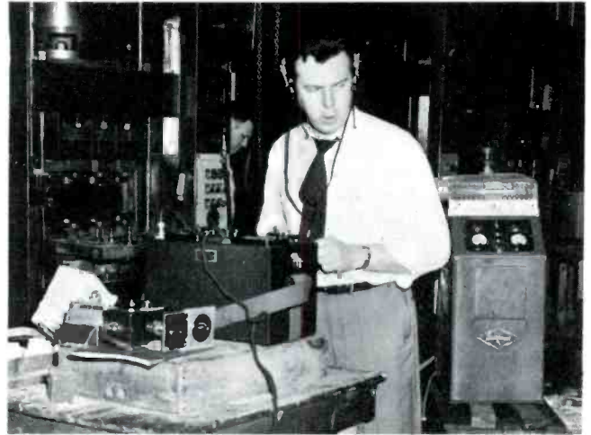
Photo 19 — Measurements being made at close range. The TVI producing plastic pellet preheater, behind the engineer's left elbow, operated in the 30 to 35 Mc. range and caused TVI with its harmonics.
