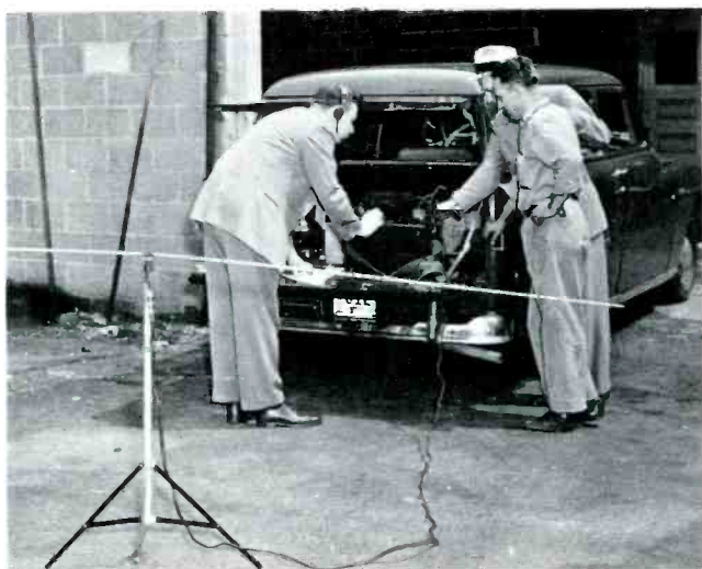
Photo 17 — Engineers measuring the signal strength of TVI from a battery of induction heaters just outside of a plastic molding plant.
