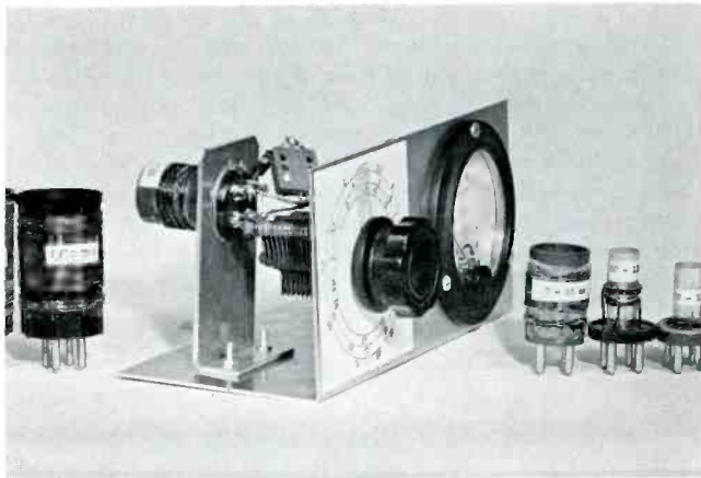
Photo 18 — This shows the construction of a simple wavemeter with its calibrated plug-in coils.
