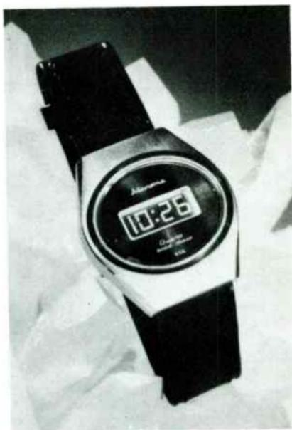
Fig. 8-6. A CMOS wristwatch.
