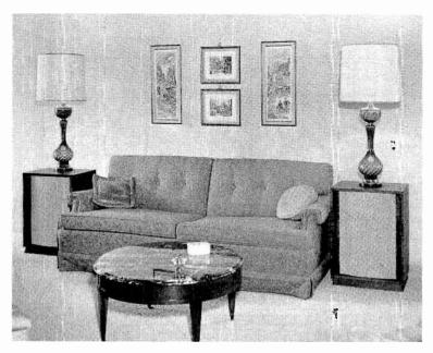
Fig. 4-15. Bass-reflex enclosures made smaller than optimum to meet room decor requirements.
