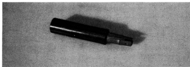
Fig. 6-5. Noise suppressor resistor for a distributor.
