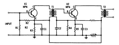
Fig. 3-12. Transformer-coupled transistor amplifier.
