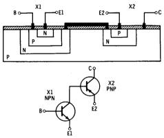
Fig. 7-21. Integrated circuit and schematic of complementary transistors.
