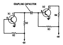
Fig. 3-11. Capacitive-coupled transistor amplifier.
