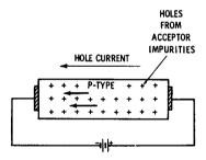
Fig. 1-7. Direction of hole flow.
