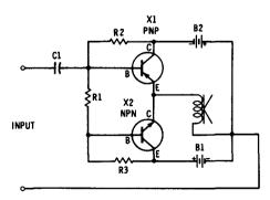
Fig. 3-23. Transformerless output stage.
