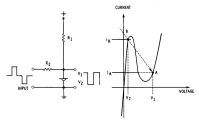
Fig. 6-8. Tunnel-diode circuit and characteristic curve.
