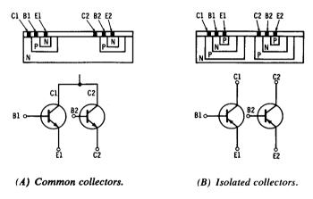
Fig. 7-12. Two transistors on one substrate.
