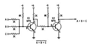
(B) Schematic diagram of a gate and inverter.
