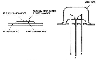
Fig. 3-3. Mesa transistor construction.
