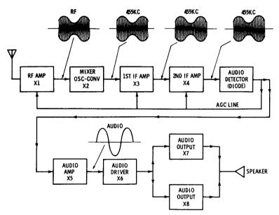
Fig. 3-24. Block diagram of a broadcast receiver.
