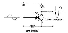
Fig. 3-7. PNP transistor amplifier.
