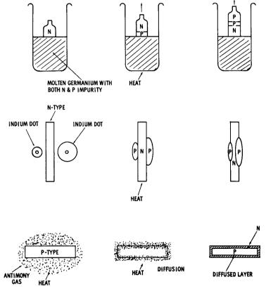
Fig. 3-1. Transistor manufacturing methods.
