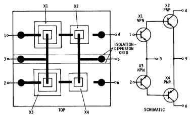
Fig. 7-22. Integrated differential amplifier and schematic diagram.
