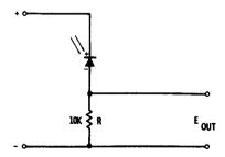
Fig. 2-14. Circuit for indicating light intensity.
