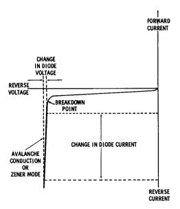
Fig. 2-6. Breakdown diode characteristic.
