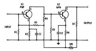
Fig. 3-13. Direct-coupled transistor amplifier.
