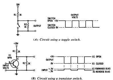
Fig. 5-1. Switching circuits.
