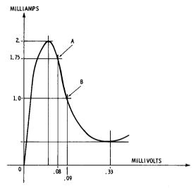
Fig. 4-7. Tunnel-diode curve.
