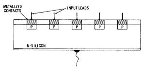
Fig. 7-9. Integrated circuit containing five diodes.
