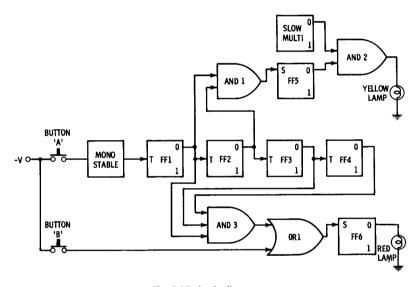
Fig. 5-17. Logic diagram.
