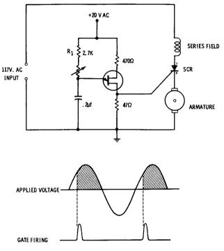
Fig. 6-6. Speed control for motor.
