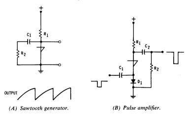
Fig. 6-5. 4-layer-diode circuits.
