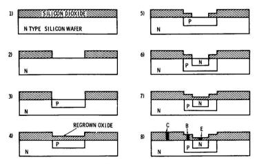
Fig. 7-7. Planar-passivated process.
