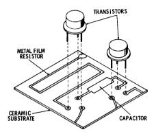
Fig. 7-5. Hybrid thin-film circuits.
