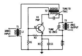
Fig. 3-20. Transistor converter stage.
