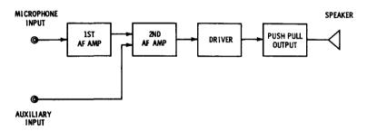
Fig. 3-26. Block diagram of an audio amplifier.
