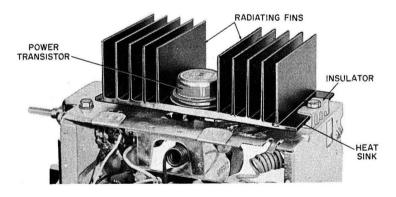
Fig. 3-29. Finned heat sink.
