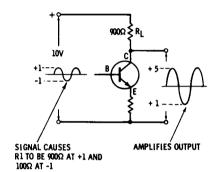
(C) Transistor substituted for the variable resistor.
