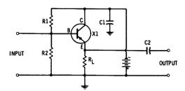
Fig. 3-15. Common-collector amplifier.
