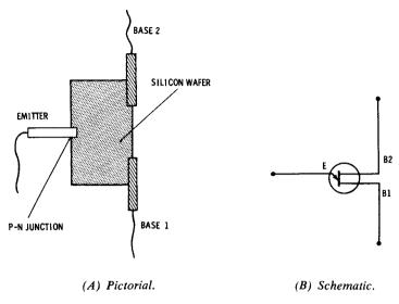
Fig. 6-1. Unijunction transistor.
