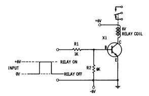
Fig. 5-3. Transistor used to operate a relay.
