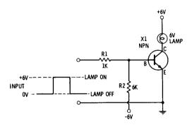
Fig. 5-2. Transistor lamp driver.
