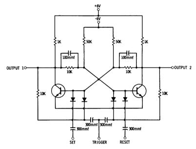
Fig. 5-12. Set-reset trigger flip-flop.
