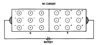
Fig. 1-11. Zero current flow with voltage applied.
