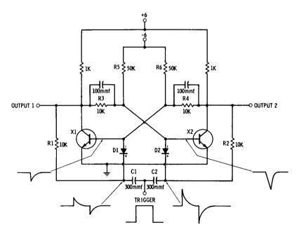
Fig. 5-11. Triggered flip-flop.
