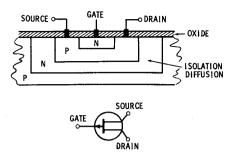
Fig. 7-20. Integrated field-effect transistor.
