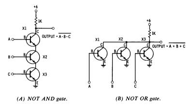
Fig. 5-7. Typical transistor gate circuits.
