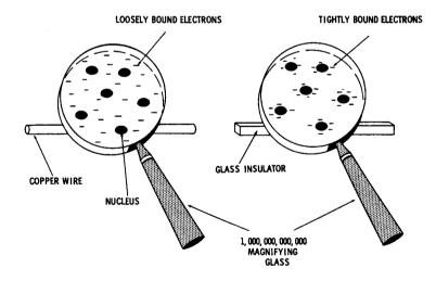
Fig. 1-1. A magnified conductor and insulator.
