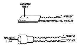
Fig. 4-10. Physical configurations for commercial types of Hall-effect devices.
