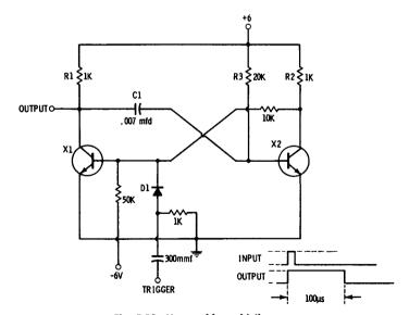
Fig. 5-13. Monostable multivibrator.
