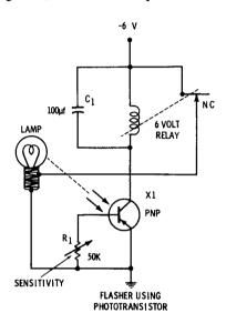
Fig. 6-7. Flasher using phototransistor.
