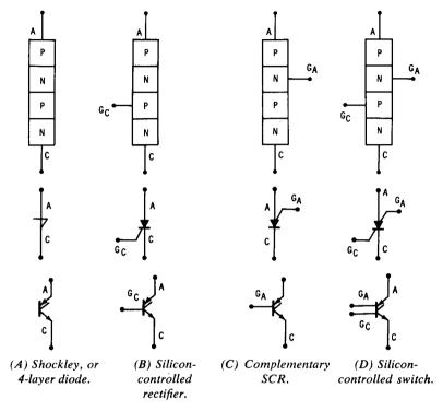
Fig. 6-4. Types of 4-layer devices.
