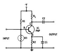
Fig. 3-10. Stabilized transistor amplifier.
