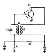
Fig. 3-17. Tuned-base oscillator.
