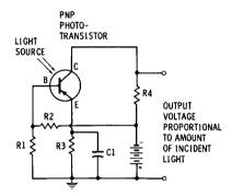
Fig. 4-13. Light level indicator using a phototransistor.
