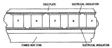
Fig. 2-16. Multiple thermocouples.
