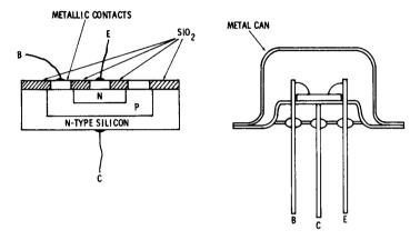
Fig. 3-5. Planar-passivated transistor.
