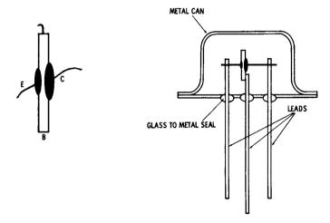
Fig. 3-2. Alloy transistor construction.
