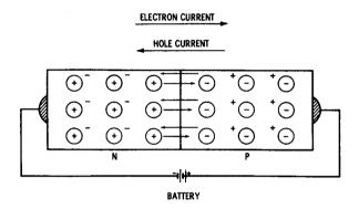
Fig. 1-10. Electron-hole flow produced by applied voltage.
