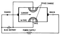
Fig. 4-1. N-type field-effect transistor.
