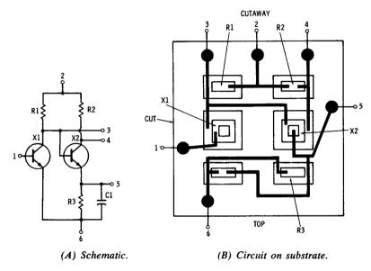
Fig. 7-18. Typical integrated circuit.
