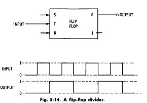
transition for every eighth pulse. Using four flip-flops in this fashion, one feeding the other, it is possible to count from 1 to 15. After the fifteenth count, all the flip-flops go back to the zero state and the count will start all over again. Each additional flip-flop enables the counter to count twice as high. One flip-flop can count to 2; two can count to 4; three can count to 8; four can count to 16; five can count to 32, etc.
