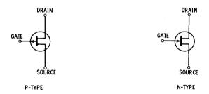
Fig. 4-2. Schematic of N- and P-type field-effect transistors.
