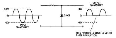
Fig. 1-15. AC voltage applied to a diode.
