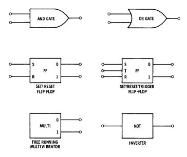
Fig. 5-16. Block diagram of logic elements.
