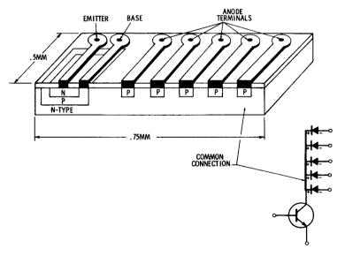
Fig. 7-10. Transistor-diode gate.
