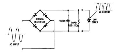
Fig. 2-8. Regulated power supply.
