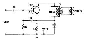
Fig. 3-21. Single-ended output stage.
