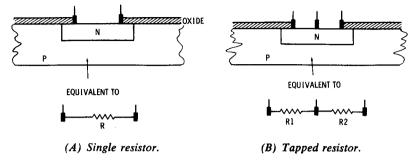
Fig. 7-15. Integrated resistors.
