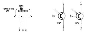
Fig. 4-12. Phototransistor.
