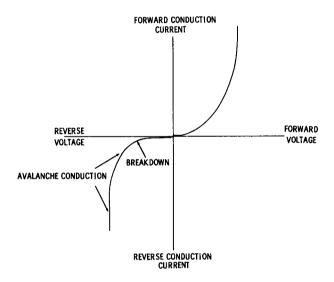
Fig. 1-12. Characteristic curve for a semiconductor diode.
