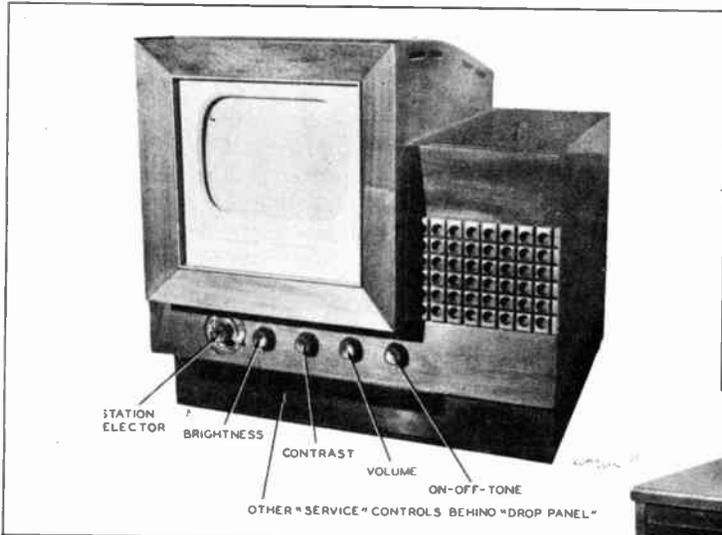
Receiver example employing five front panel controls. (Photo from a sample receiver courtesy the Philco Corporation.)
