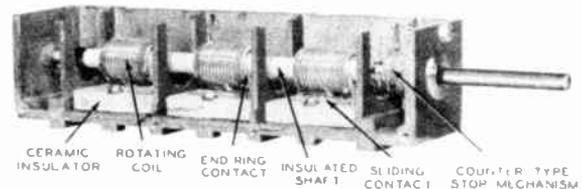
B TOP VIEW OF "INDUCTUNER" (SHIELD REMOVED)
