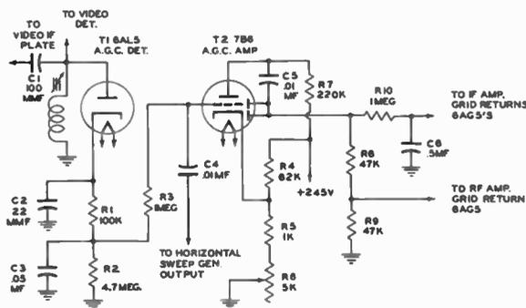
Fig. 244. An Amplified A. G. C. Circuit.
