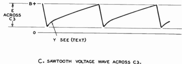
Fig. 63. Voltage Waveforms in Blocking Oscillator
