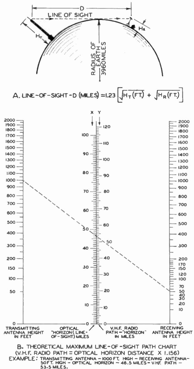
Fig. 147. V. H. F. Path Length as a Function of Height of Transmitting and Receiving Antennas
