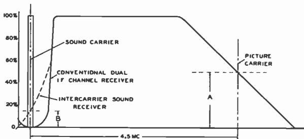
Fig. 247. IF Response Characteristics of Conventional Dual Channel and Intercarrier Sound Systems.
