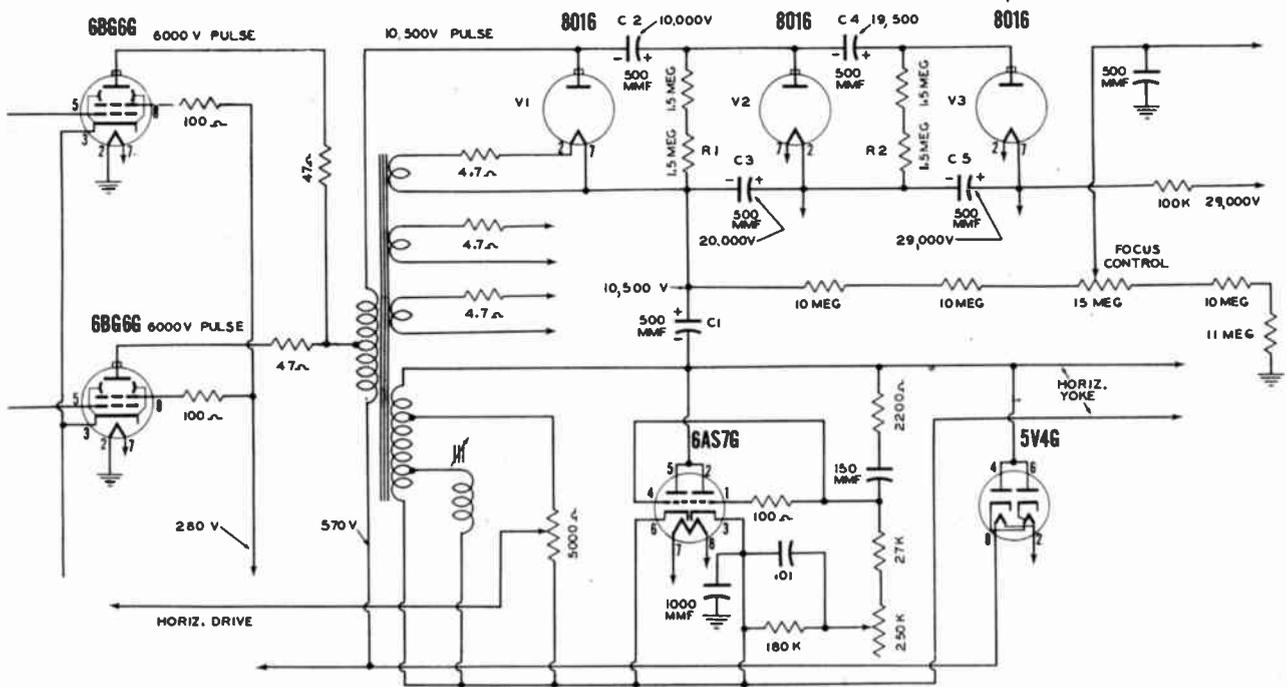
Fig. 38. Horizontal Flyback High-Voltage Tripler
