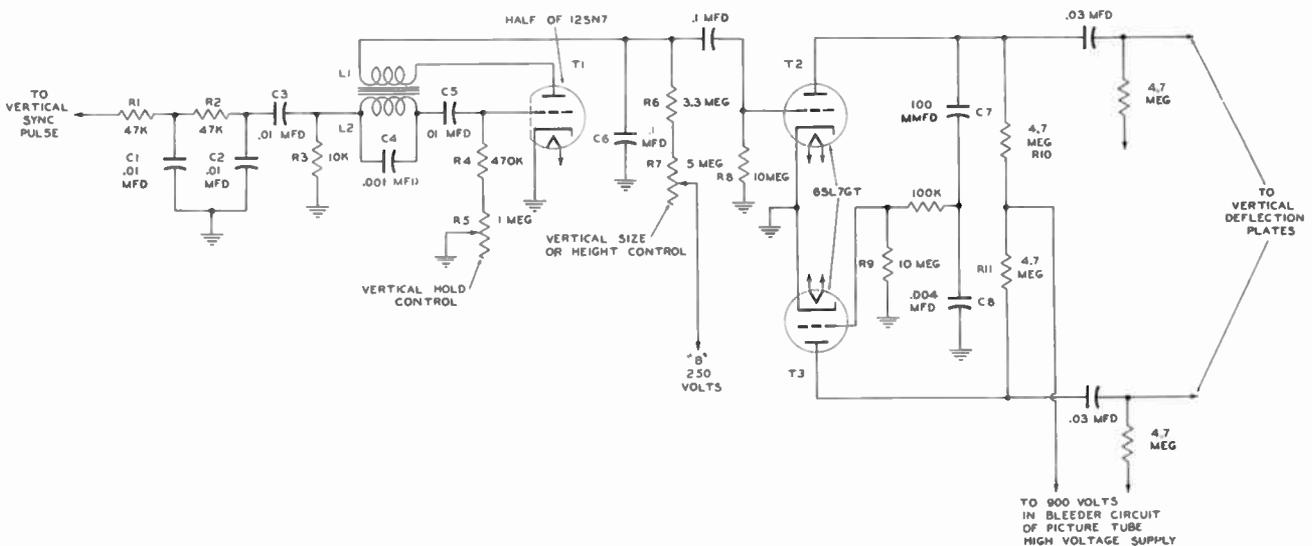
Fig. 79. Blocking Oscillator - Vertical Electrostatic Deflection Circuit
