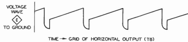
Fig. 85. Electromagnetic Deflection Systems - Example 2. Horizontal Circuit.
