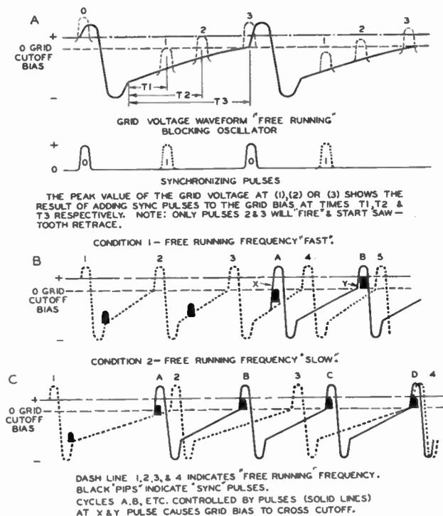
Fig. 68. Pulse Control of the Blocking Oscillator
