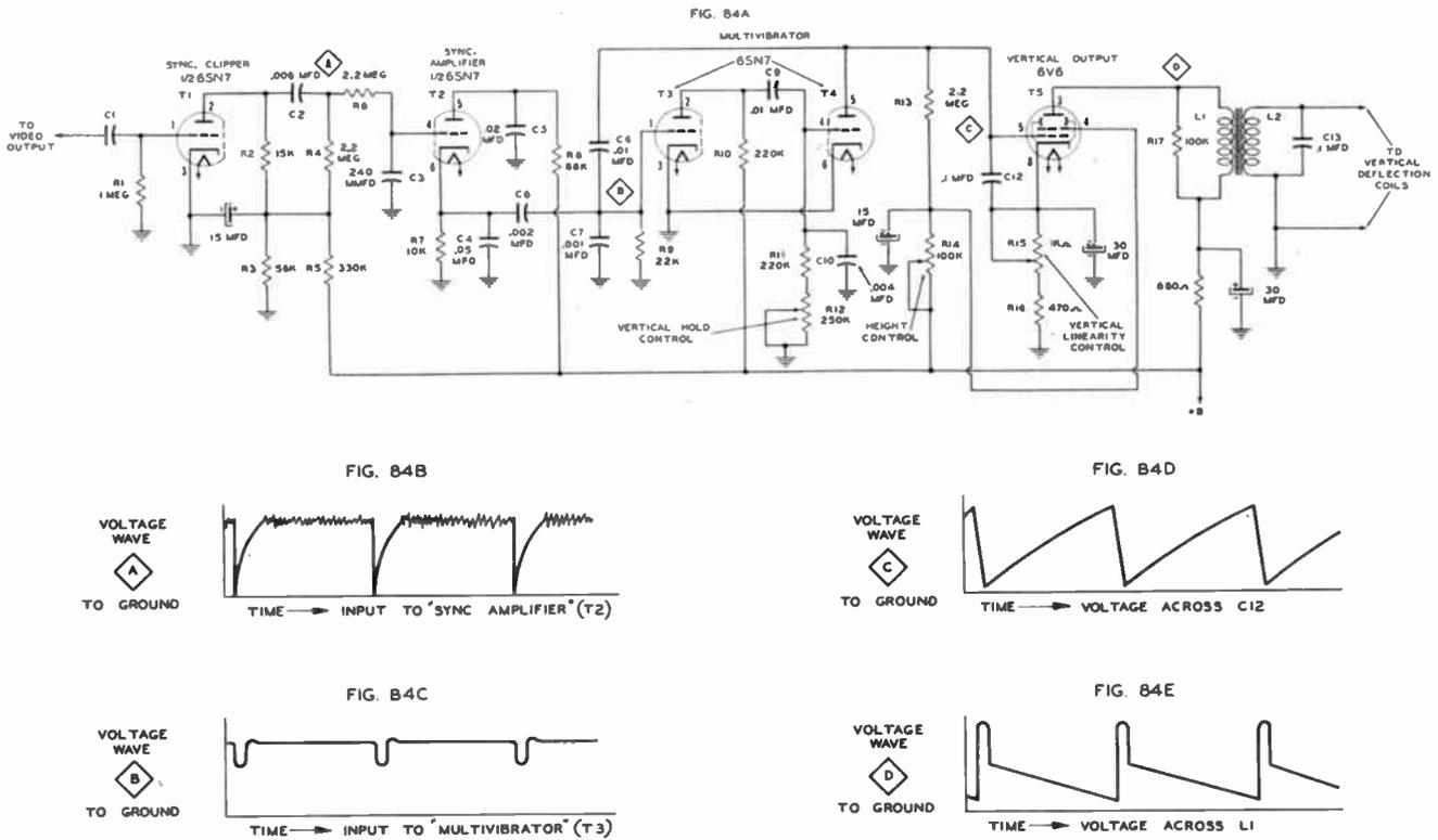
Fig. 84. Electromagnetic Deflection Systems - Example 2. Vertical Circuit
