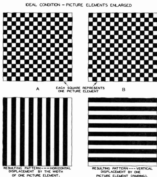
Fig. 67. Picture Element Displacement which might Result from Scanning Oscillator Instability
