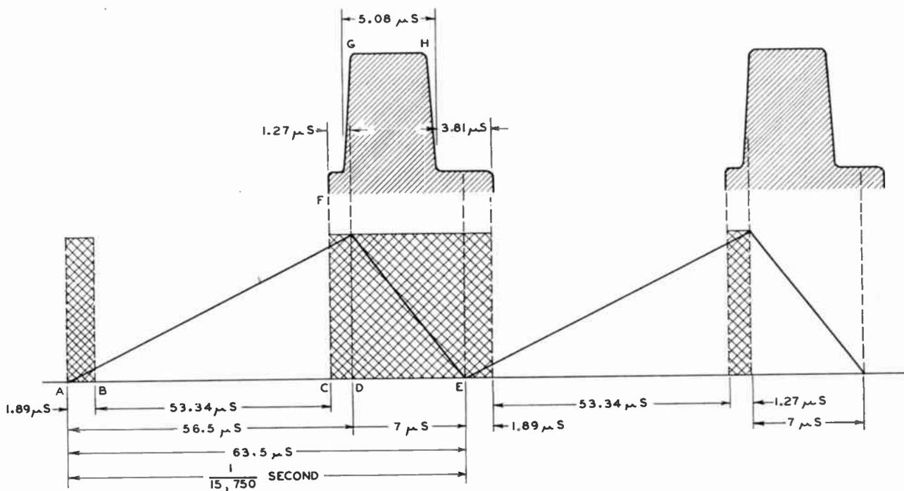
Fig. 65. Horizontal Scanning Wave
