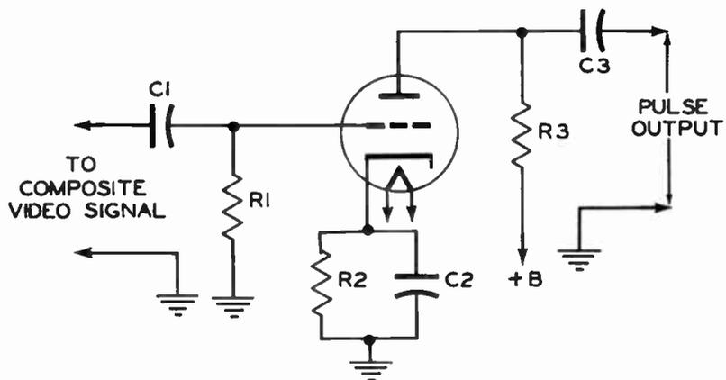
Fig. 95. Triode Sync Separation Circuits
