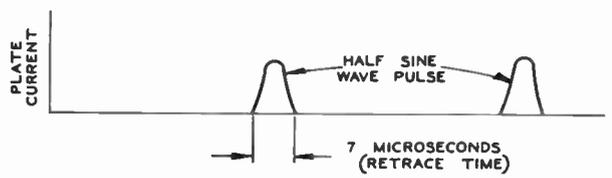
Fig. 80. Blocking Oscillator - Horizontal Electrostatic Deflection Circuit
