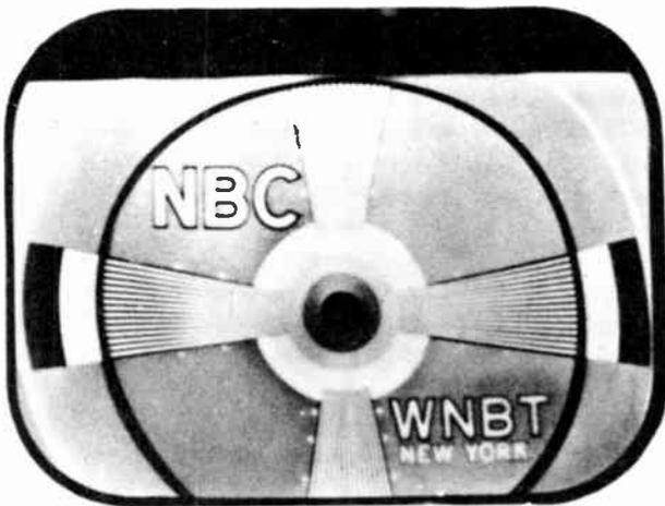
Fig. 129. Vertical Centering Control Misadjusted
