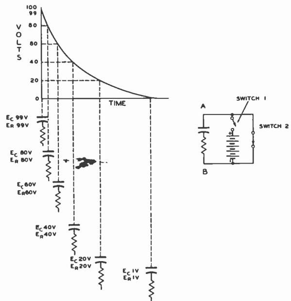
Fig. 44. Resistor-Capacitor Discharging Curve
