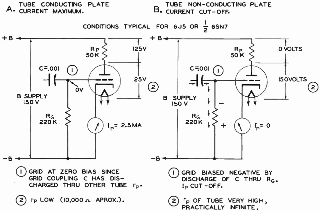
Fig. 56. Tube Operating Conditions in Multivibrator Oscillators
