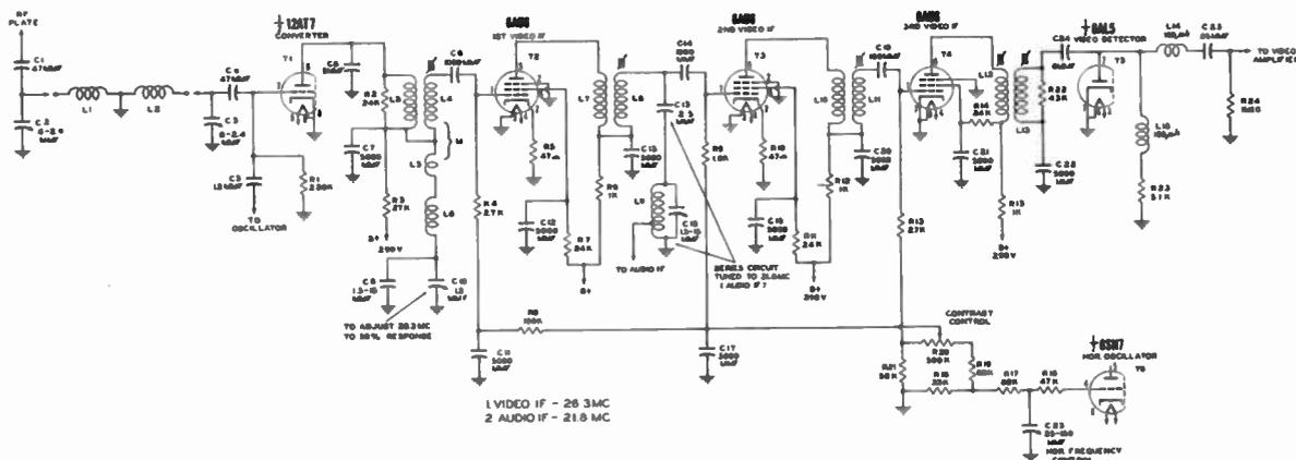
Fig. 191. Video I-F Amplifier Employing Over-Coupled Transformers.
