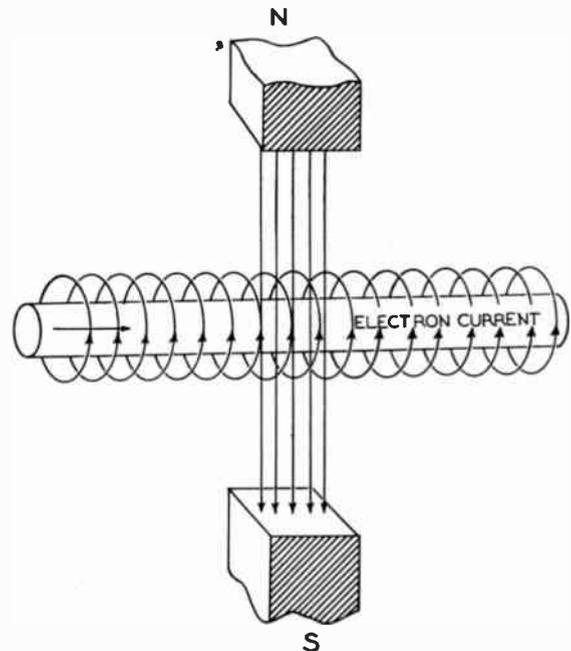
Fig. 15. Conductor at Right Angles to Magnetic Field
