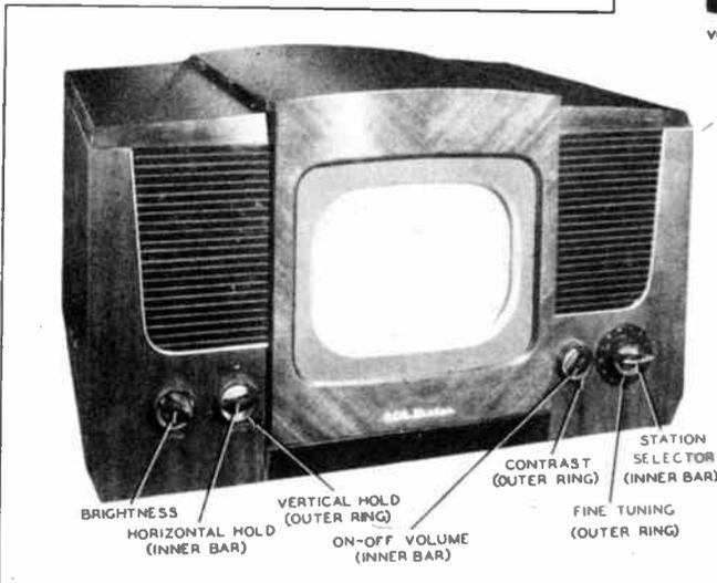
Receiver example employing seven front panel controls. (Photo from a sample receiver courtesy R. C. A.)
