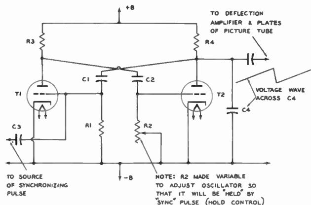
Fig. 59. Sawtooth Scanning Wave from Asymmetrical Multivibrator
