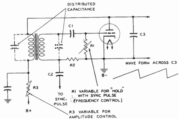
Fig. 62. Blocking Oscillator as a Sawtooth Generator
