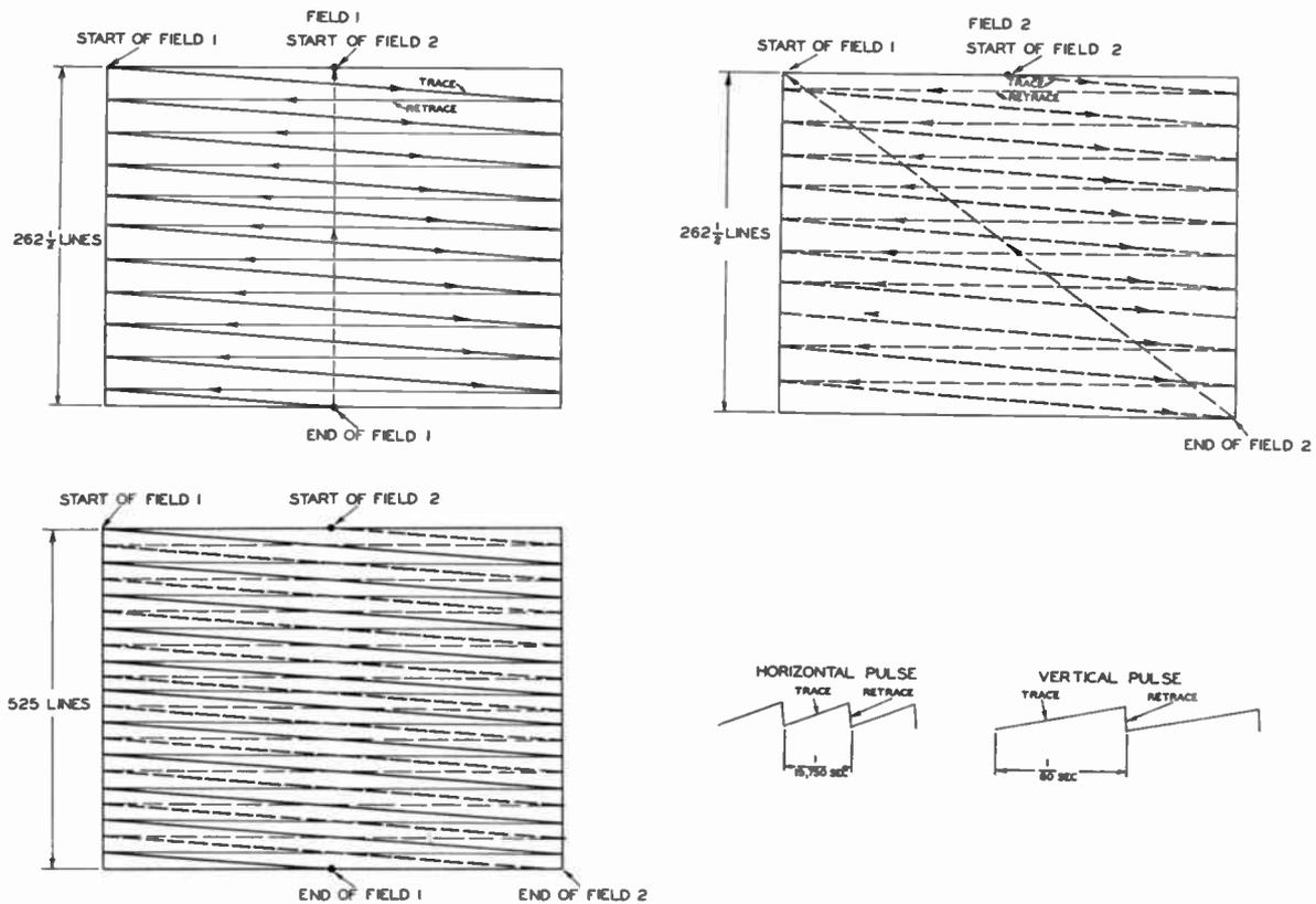
Fig. 28. Interlaced Scanning
