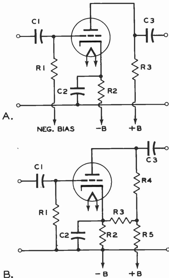
Fig. 91. Cut-off by Combination Bias
