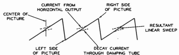
Fig. 75. Current Waveforms In Horizontal Reaction Scanning
