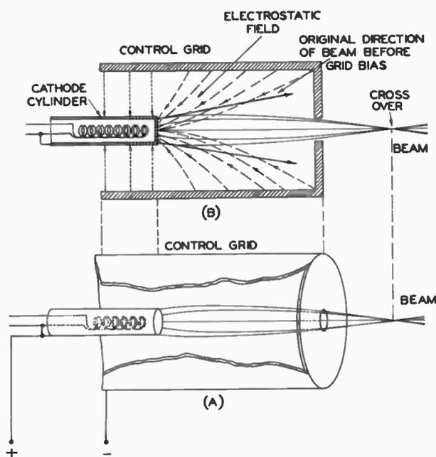
Fig. 4. Action of Cathode and Control Grid Assembly.
