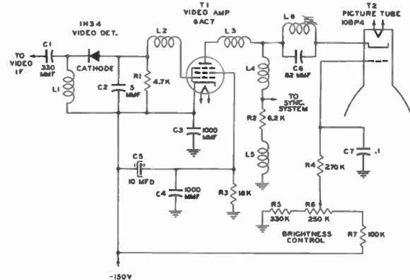
Fig. 237. DC Restoration by Direct Coupling from the Video Detector to the Picture Tube.
