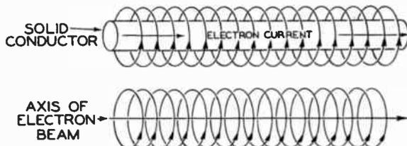
Fig. 13. Similarity of Solid Conductor and Electron Beam
