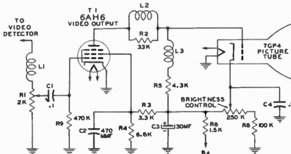
Fig. 234. DC Restoration by Grid Circuit Rectification in the Video Output Stage.
