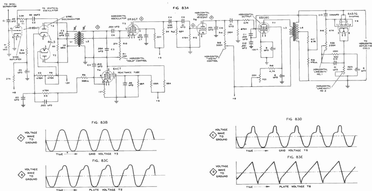
Fig. 83. Electromagnetic Deflection Systems - Example 1. Horizontal Circuit
