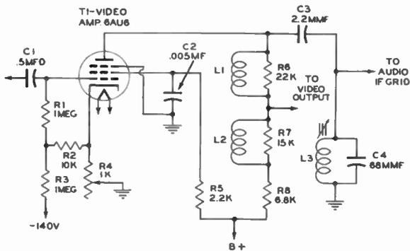
Fig. 249. Audio IF Take-off Employing a Shunt-Tuned Trap.
