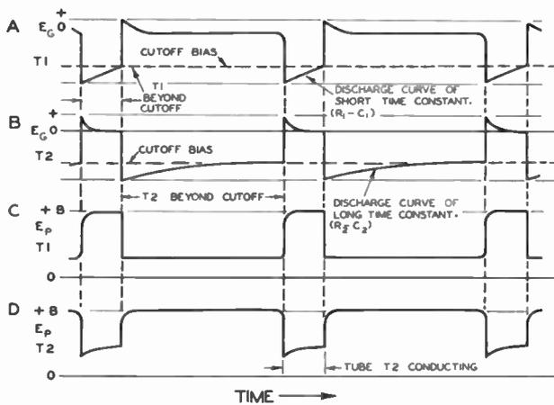
Fig. 58. Waveforms of an Asymmetrical or Unbalanced Multivibrator
