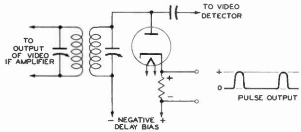
A. POSITIVE PICTURE POLARITY - POSITIVE PULSES.
