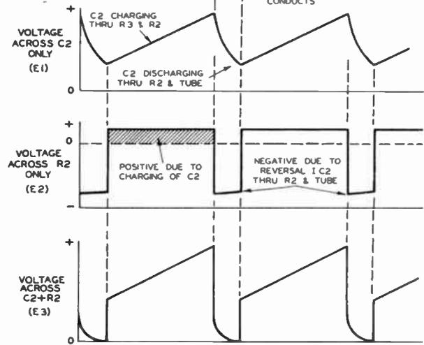
Fig. 72. Representative Peaking Circuit
