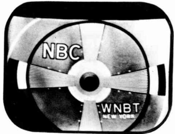
Fig. 117. Focus Coil and Ion Trap Misaligned
