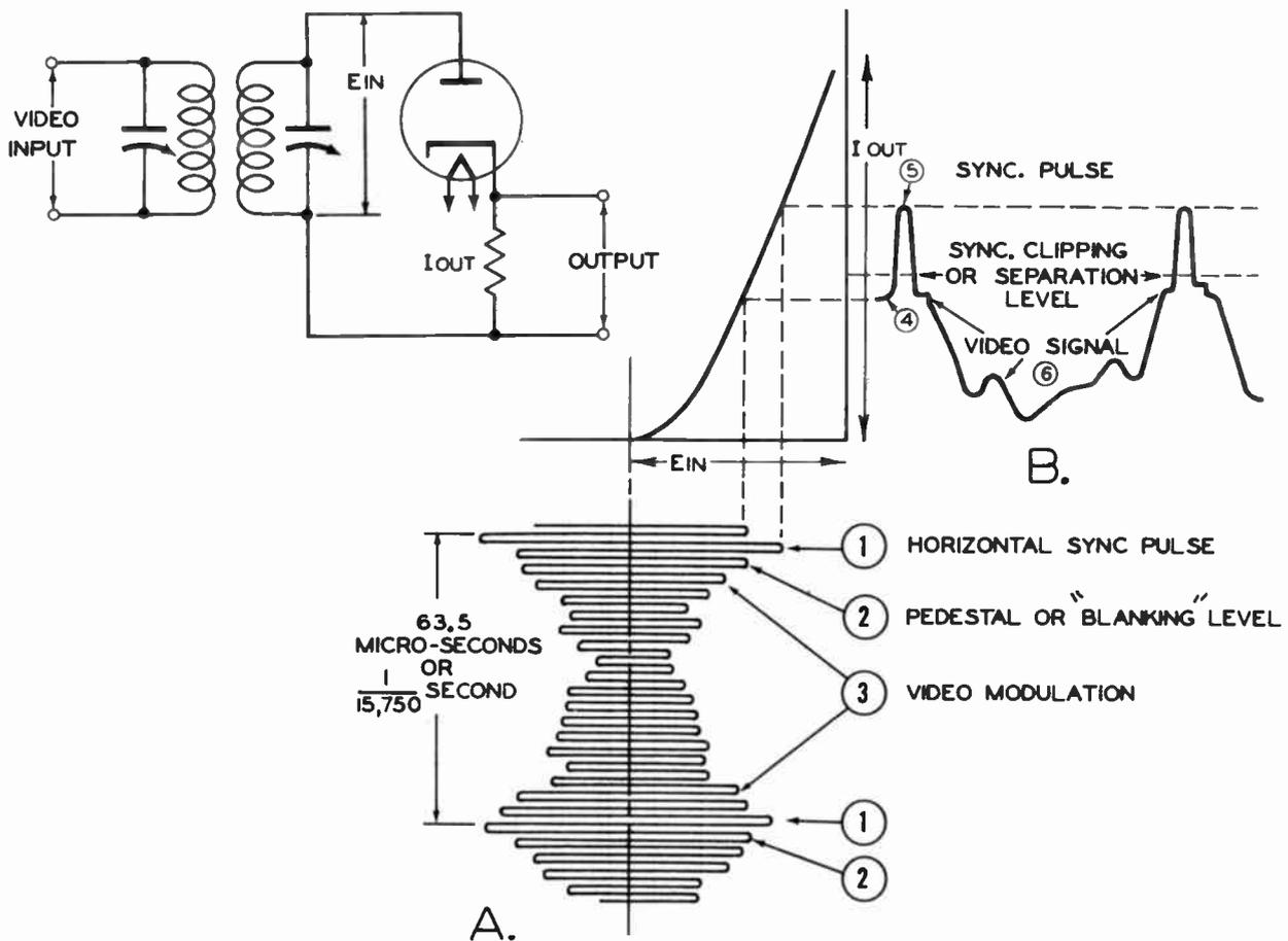
Fig. 93. Demodulation (Detection) of the Video (Picture) Carrier
