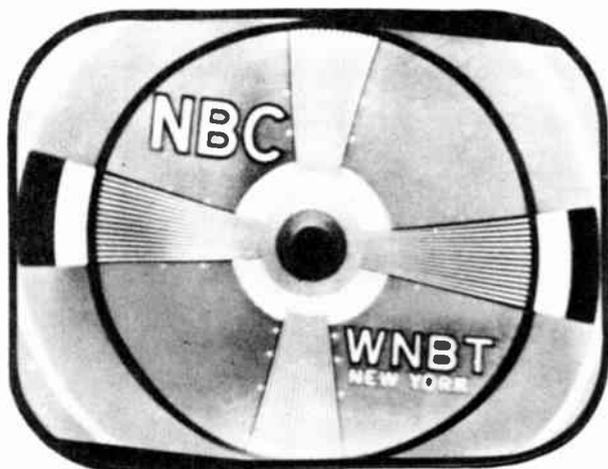
Fig. 118. Deflection Yoke not Properly Adjusted. (Rotated)
