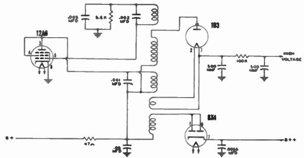
Fig. 32. RF Oscillator-Rectifier High Voltage Supply System
