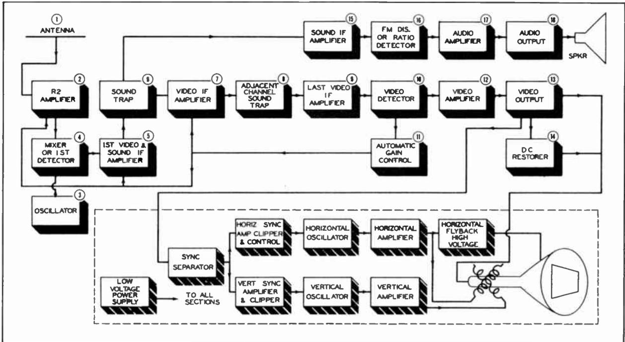
Fig. 144. Block Diagram of Complete Television Receiver. (Electromagnetic Deflection Type)
