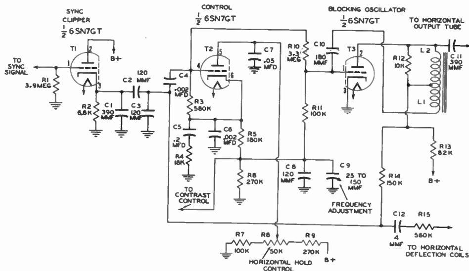
Fig. 90. Automatic Pulse Width Control of Blocking Oscillator
