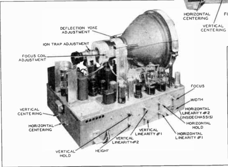
An example of service controls available on top, back and side of chassis. (Photo from sample courtesy the Motorola Co.)
