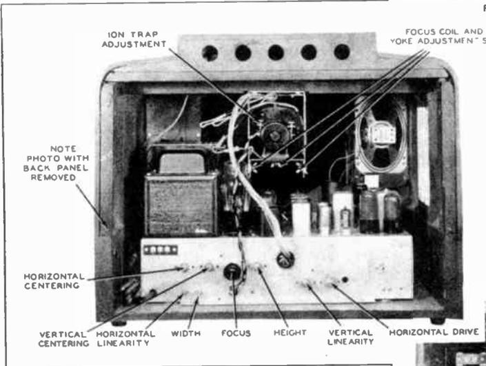
An example of service controls available at back of chassis. Back panel removable for servicing picture tube. (Photo from sample receiver courtesy Emerson Radio and Phonograph Corp.)
