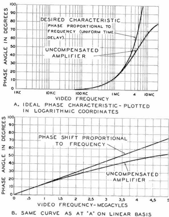
Fig. 228. Phase Shift Requirements of a Video Amplifier for Perfect Reproduction.
