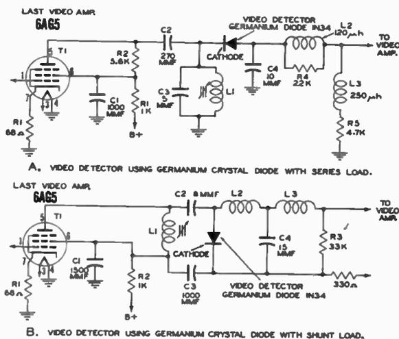
Fig. 209. The Germanium Crystal as a Video Detector.
