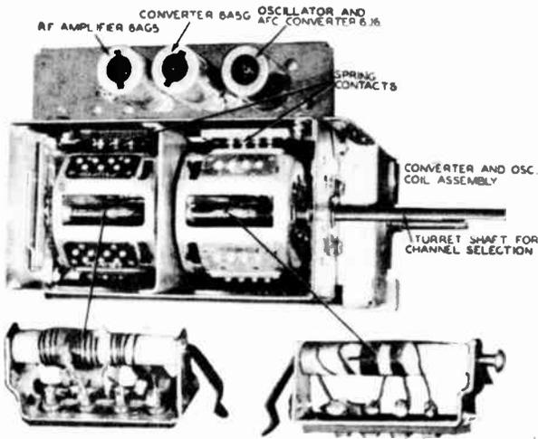
Fig. 178. A Turret Type of Input Tuning System. Photo from Sample Receiver Courtesy Philco Corp.
