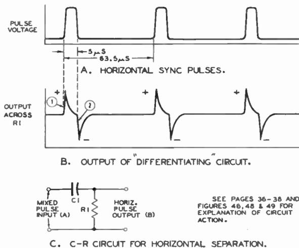
Fig. 98. Horizontal pulse separation or "Differentiation"
