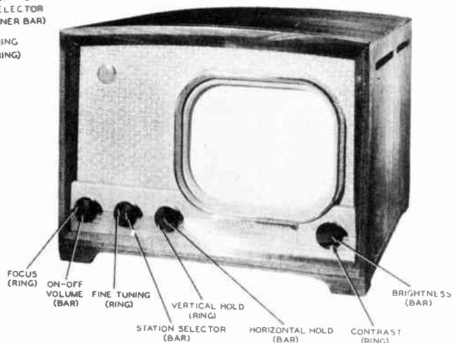
Fig. 115. Typical Examples of Operating or Front Panel Controls
