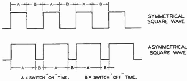
Fig. 47. Square Waveforms
