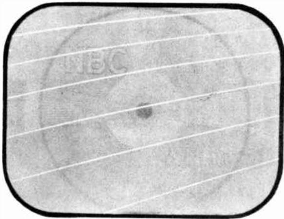
Fig. 120. Brightness Control Misadjusted. (Brightness too High)
