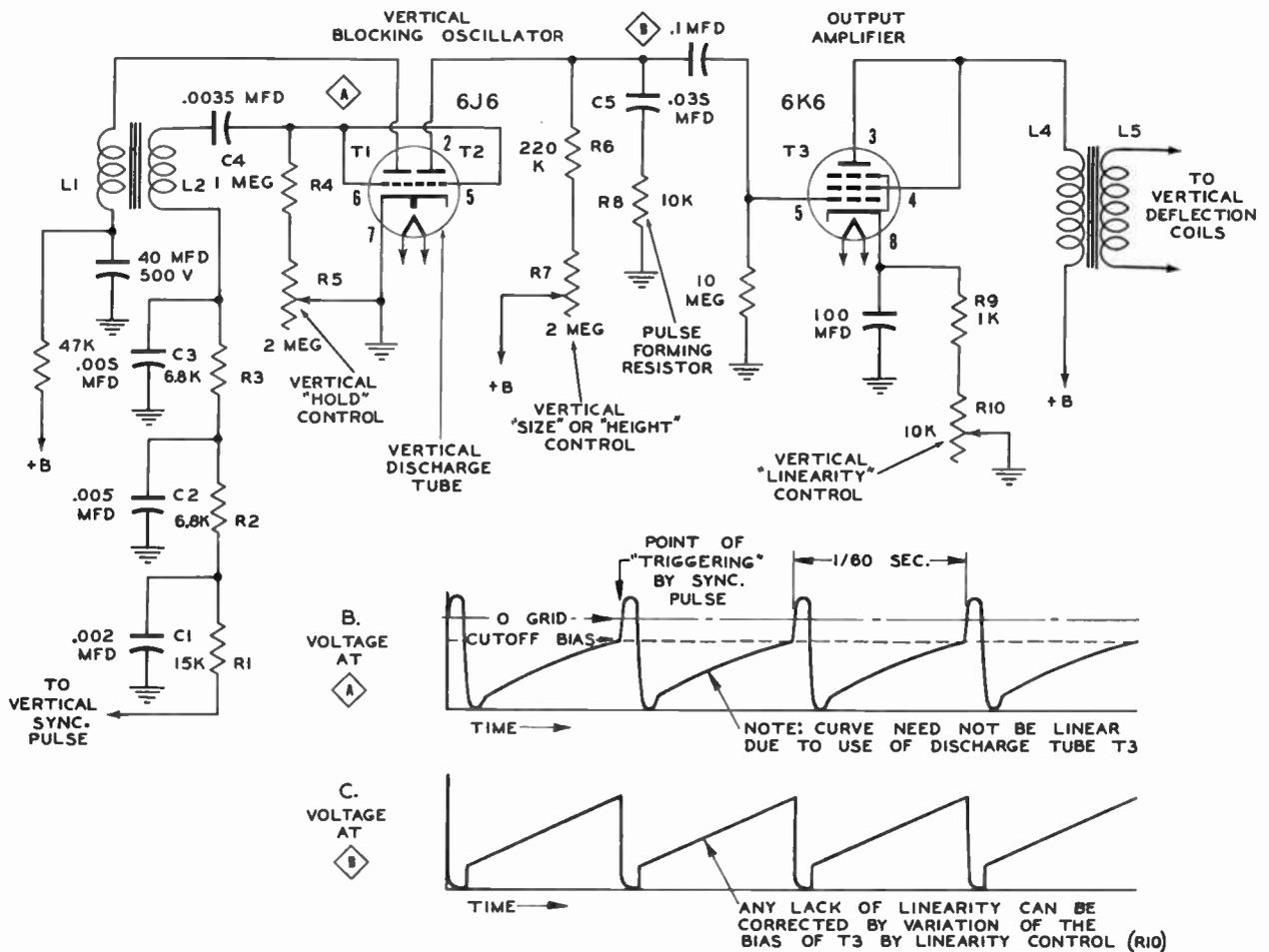
Fig. 82. Electromagnetic Deflection Systems - Example 1. Vertical Circuit
