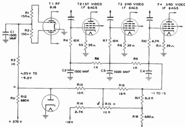
Fig. 240. Use of a Diode Gate to Provide Improved Contrast Control Action.
