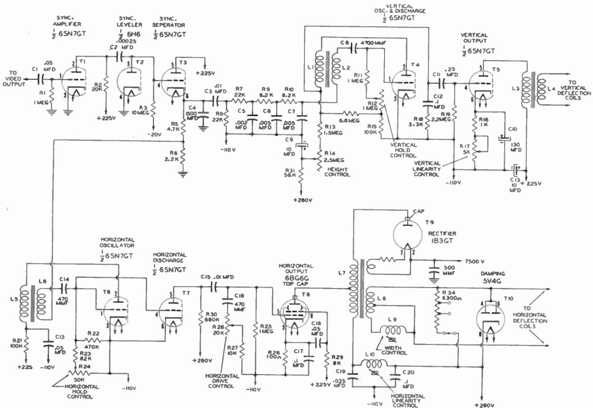
Fig. 86. Typical Electromagnetic Deflection System - Example 3
