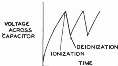
Fig. 52. Neon Tube Relaxation Oscillator
