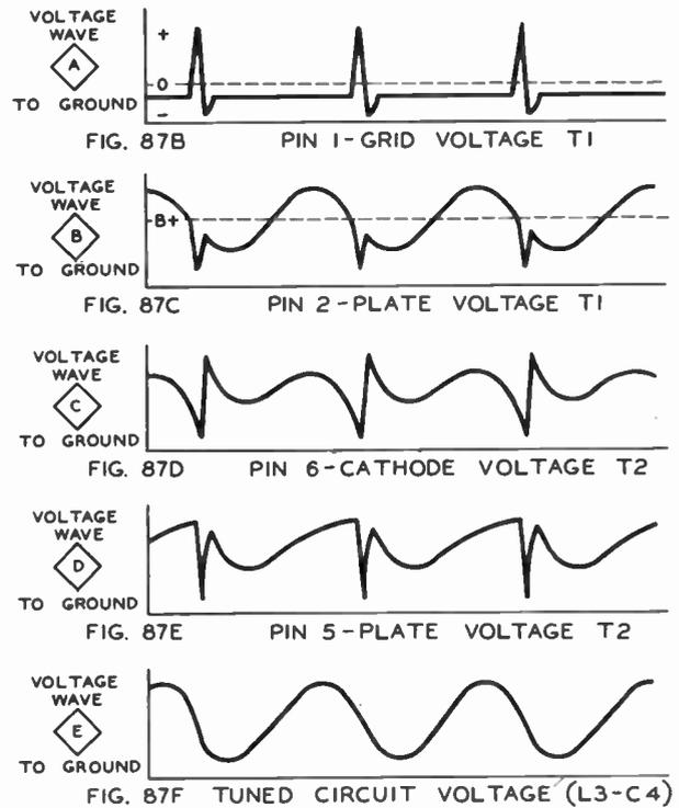
Fig. 87. A Variation of the Blocking Oscillator
