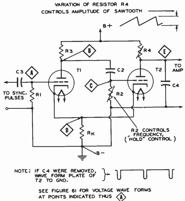
Fig. 60. Cathode-Coupled Multivibrator as Sawtooth Wave Generator
