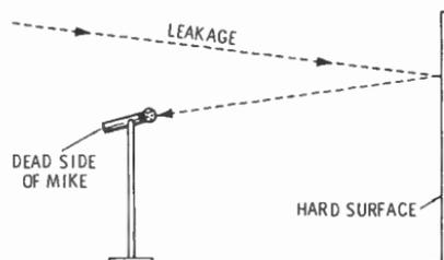
Fig. 9-3. A hard surface on the live side of a mike can put the undesired off-axis signals on-axis, by reflecting them.
