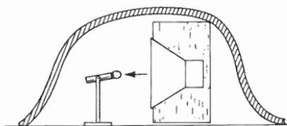
Fig. 9-1. Isolating an instrument amplifier by covering it with a sound-absorbing blanket.
