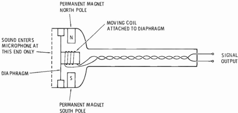
Fig. 3-1. The components of a dynamic microphone.
