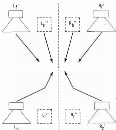
Fig. 13-5. Side effect images  $L_b''$ ,  $R_b''$ ,  $L_r''$ , and  $R_r''$  are offset in the direction of their main images.
