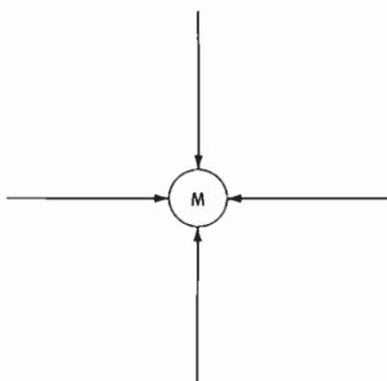
Fig. 3-2. A pressure-operated mike is sensitive to sound waves originating from any direction.
