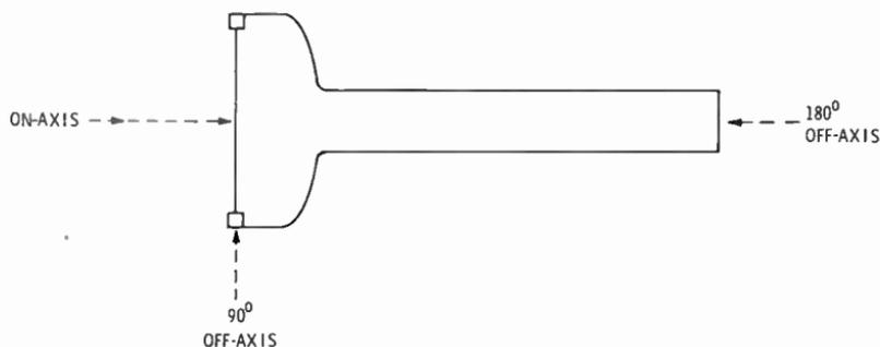
**Fig. 3-5. A microphone axis is the line perpendicular to the diaphragm on the side exposed to the sound waves.**
