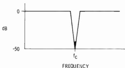
Fig. 5-22. Frequency response of a notch filter.
