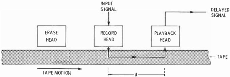
Fig. 5-57. Delaying a signal with a tape recorder.
