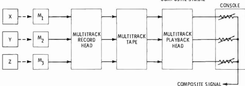
Fig. 1-6. Instrumental balance by recording instruments on separate tracks of multitrack tape.
