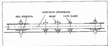
FIGURE 1. SIMPLIFIED TAPE PATH CENTERLINE
