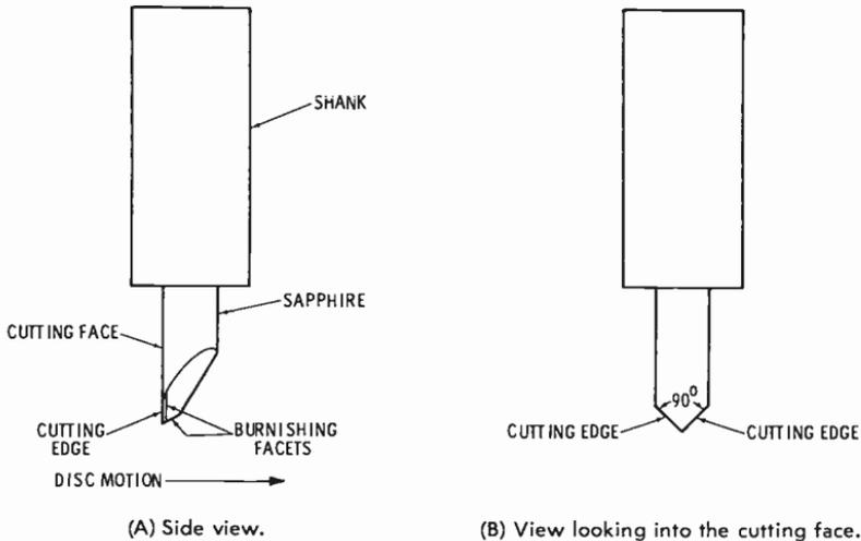
Fig. 12-11. A recording stylus.
