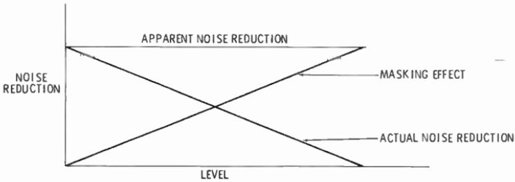
Fig. 7-9. The masking effect and the actual noise reduction combine to keep the apparent noise level constant.
