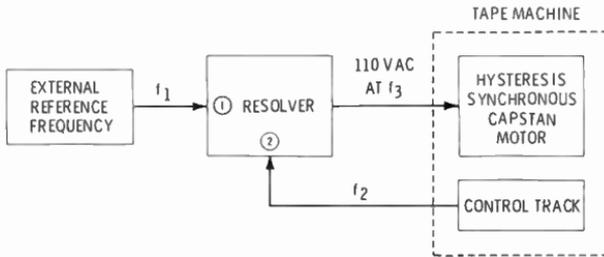
Fig. 10-3. Controlling tape speed with a resolver and a 60-Hz synchronous capstan motor.
