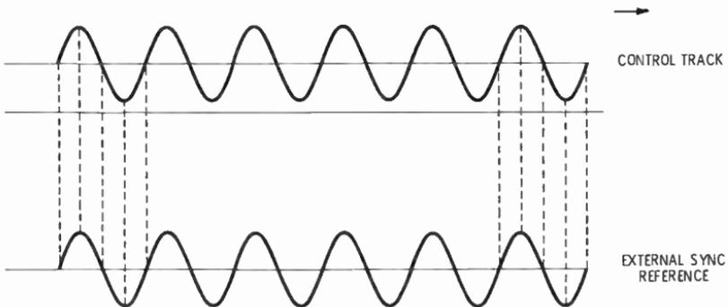
Fig. 10-2. Phase-locked operation. The resolver brings the control track signal precisely into phase with the external sync reference, and then maintains this relationship.
