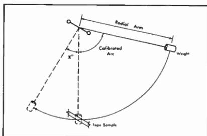
FIGURE 7. SHOCK TENSILE TEST APPARATUS DIAGRAM
