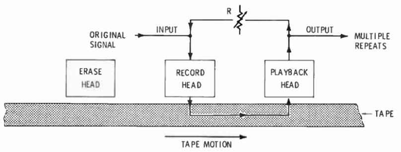
Fig. 5-58. Producing multiple repeats of a signal with a single playback head tape recorder.
