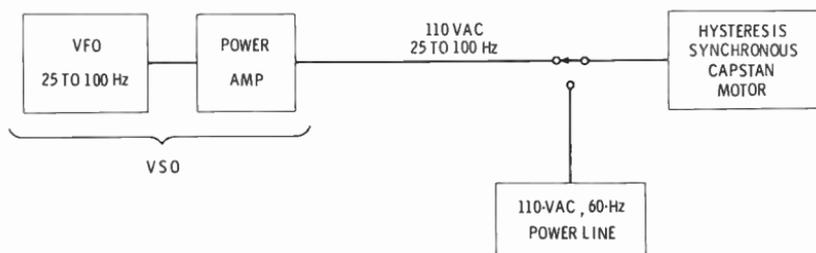
Fig. 5-64. Varying the speed of a hysteresis synchronous motor.
