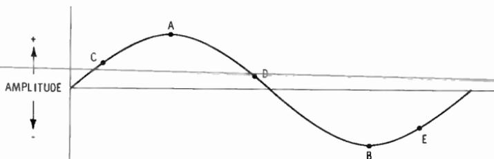
Fig. 2-16. The different values of waveform amplitude.
