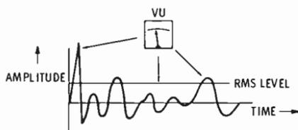
Fig. 5-25. A VU meter reads the rms level and ignores the peaks that do not contribute to loudness.
