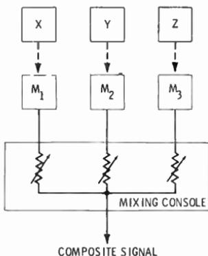
Fig. 1-5. Controlling instrumental balance by using separate mikes and a mixing console.
