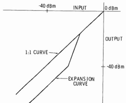
Fig. 7-6. The Dolby expansion curve.
