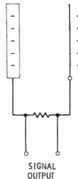
Fig. 3-15. Diagram of an electret condenser microphone. Its circuit is equivalent to that of Fig. 3-13.
