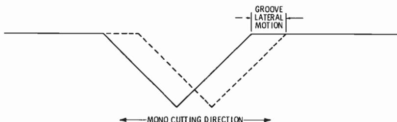
Fig. 12-22. A mono groove producing lateral motion.
