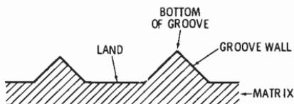
down, and the matrix is attached to a metal or wood-backed plate to make it easier to handle. Since the groove walls containing the signal are now raised above the surface of the disc, they are very vulnerable and care must be taken to prevent damage to them.
