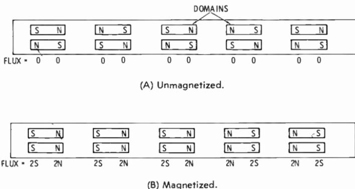
Fig. 4-6. Fields of domains on unmagnetized and magnetized tape.
