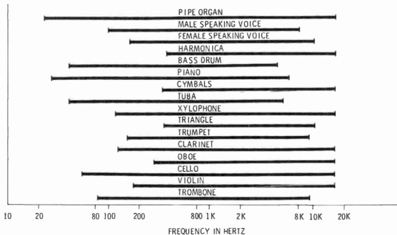
Fig. 5-23. Frequency ranges of instruments.
