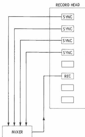
adjacent recording and reproducing heads would cause high-frequency oscillations (Fig. 9-9). This procedure, called *bouncing tracks* or *ping-ponging*, can also be used to mix entire performances onto one or more tracks either to make the final mixdown easier or to open up their original tape tracks for additional overdubs.
