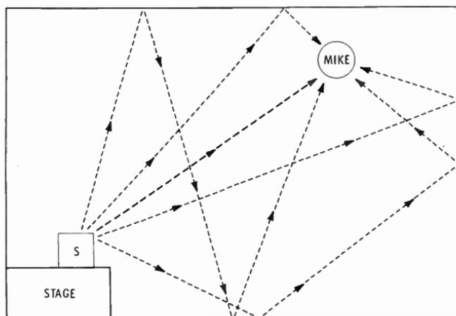
Fig. 1-9. Distant microphones pick up both direct and reflected sound.
