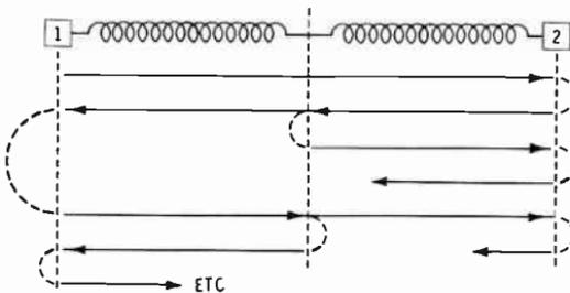
Fig. 5-50. The signal path in a spring reverb unit. A reflection occurs at each boundary: spring to spring and spring to rod.
