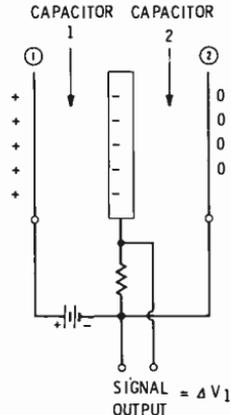
Fig. 3-17. A cardioid condenser microphone.
