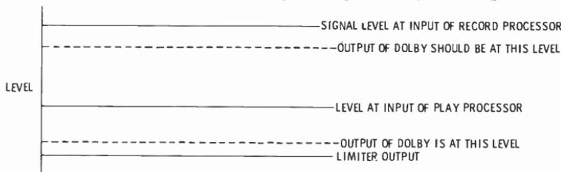
Fig. 7-14. The tape output is fed to the Dolby playback processor at too low a level.
