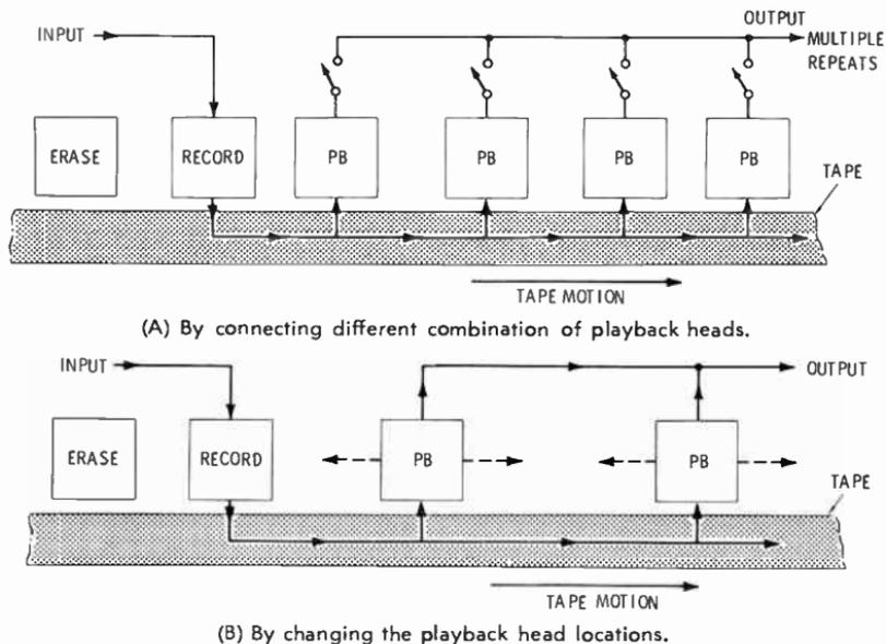
Fig. 5-59. Producing multiple repeats and variable delays with a tape recorder.
