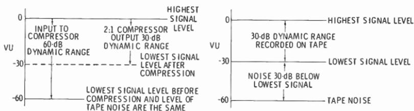
(A) A 60-dB dynamic range compressed to 30 dB before recording.
