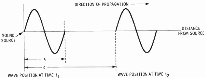
Fig. 2-2. Demonstrating velocity of a wave.
