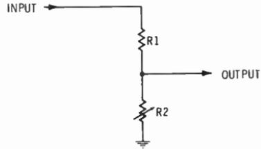
other a cadmium selenide cell) which are part of a volume control circuit. The value of the attenuator changes with the illumination received by the phototcells, and thus turns the volume of the signal up or down. The Kepex and the 1176LN use a *field-effect transistor (FET)* as a *voltage-variable resistor*. The FET changes resistance in proportion to a voltage (obtained from the input signal) applied to it, and this resistance change is used to control the signal in the same
