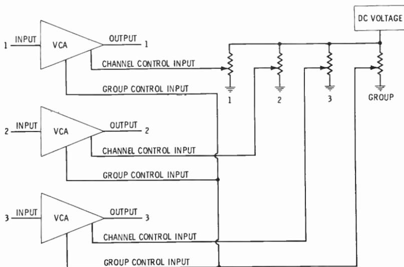
(D) Retaining separation using VCAs with several control inputs.
