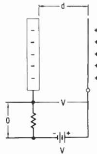
Fig. 3-13. The power supply charges the capacitor through a high-value resistor.
