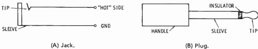
Fig. 6-6. Unbalanced jack and plug.
