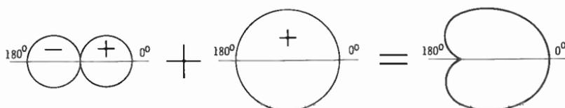
Fig. 3-19. A bidirectional pattern added to an omnidirectional pattern produces a cardioid pattern.
