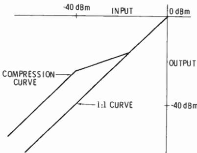
Fig. 7-5. The Dolby compression curve.
