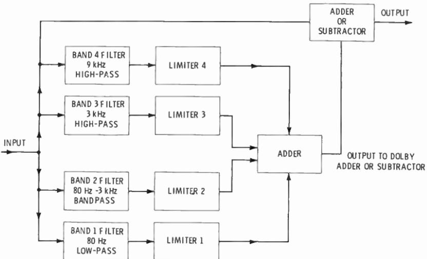
Fig. 7-8. Block diagram of the filter/limiter networks.
