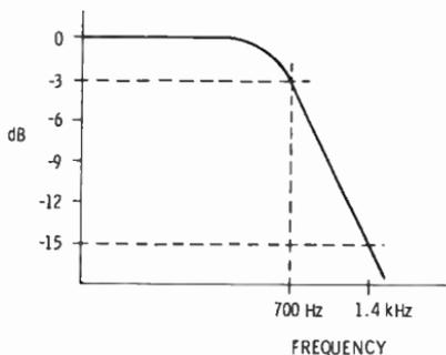
Fig. 5-20. A 700-Hz, low-pass filter with a slope of 12 dB per octave.
