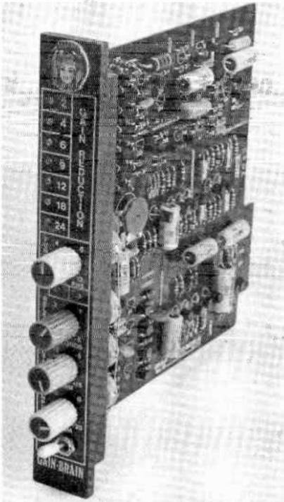
Fig. 5-32. The Gain Brain limiter uses light emitting diodes to indicate gain reduction.
