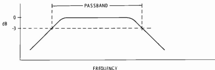
Fig. 5-21. A bandpass filter created by combining high- and low-pass filters with different cutoff frequencies.
