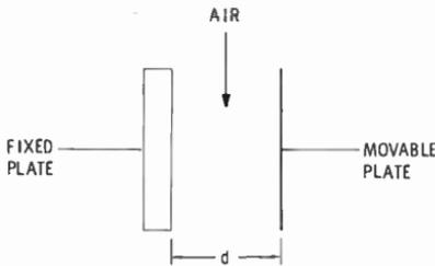
Fig. 3-12. In a condenser microphone capsule the sound pressure varies distance  $d$  between plates.
