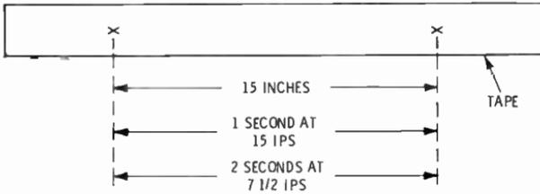
Fig. 4-1. Magnetic tape recording equates lengths of tape to periods of time.
