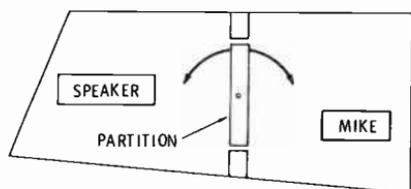
Fig. 5-56. An acoustic echo chamber. Decay time is a function of the partition position.
