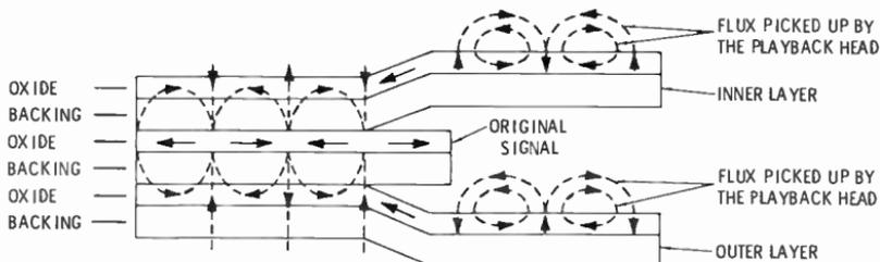
Fig. 4-25. The difference between print-through to the inner and outer layers of tape.
