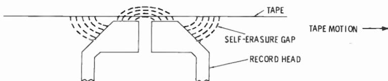
Fig. 4-12. High frequencies are partially erased by the flux induced in the self-erase gap by high frequencies and by the bias current.
