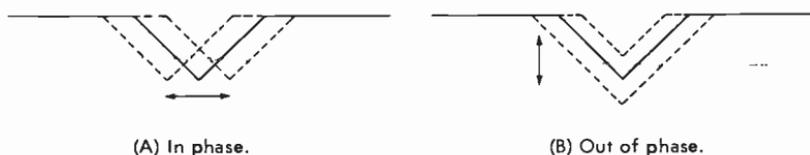
Fig. 12-3. Groove motion in stereo recording. The solid line is the groove with no modulation.
