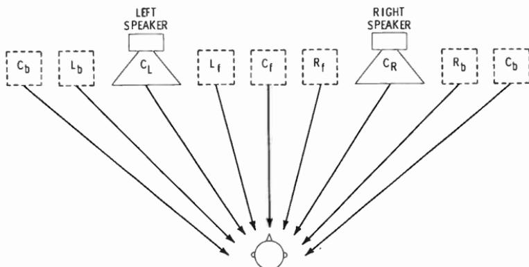
Fig. 13-12. The stereo stage created by a QS-encoded disc played in stereo.
