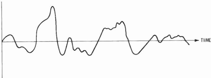
**Fig. 2-4. A complex waveform.**
