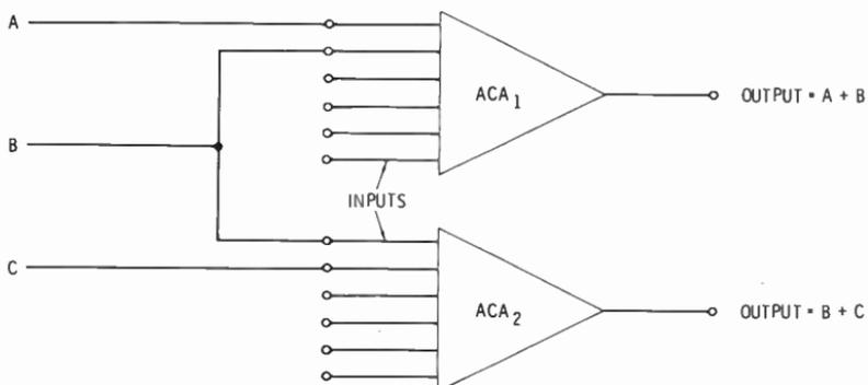
Fig. 6-12. Isolation between inputs of an ACA.
