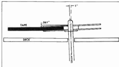
FIGURE 2. IMPROPER PEDESTAL POSITION
