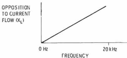
Fig. 5-8. Inductive reactance ( $X_l$ ) is proportional to frequency.
