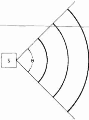
Fig. 1-7. Waves leave the sound source (S) in an arc with angle  $\theta$ .
