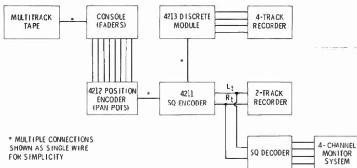
Fig. 13-9. SQ position encoding at the multitrack stage.
