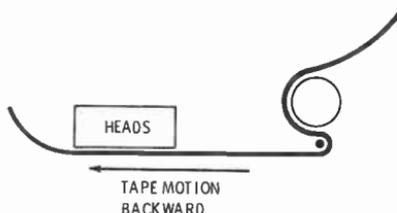
Fig. 5-66. Tape path to play a tape backward.
