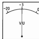
(B) The input signal exceeds the threshold causing 3 dB of gain reduction. The meter indicates that the gain is 3 dB lower than normal.
