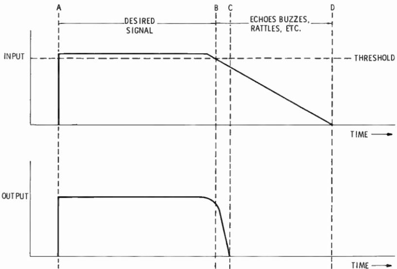
(B) Using the Kepex to remove echoes, buzzes, and rattles from a signal.
