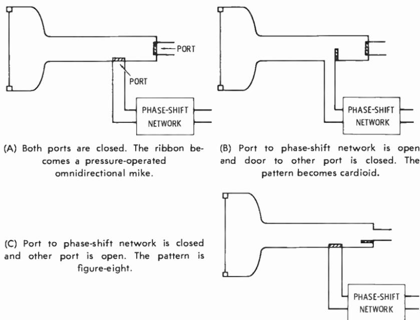
**Fig. 3-11. A method of producing variable pickup patterns from a ribbon microphone using ports and an acoustical phase-shift network.**
