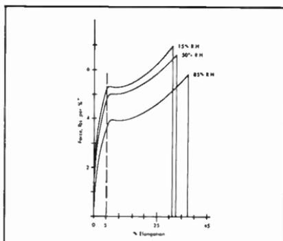
FIGURE 6. ACETATE TENSILE PROPERTIES AT DIFFERENT RELATIVE HUMIDITIES
