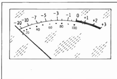
Fig. 5-26. A VU meter. The upper scale is calibrated in volume units for use in recording. The lower scale is percentage modulation for use in broadcasting.
