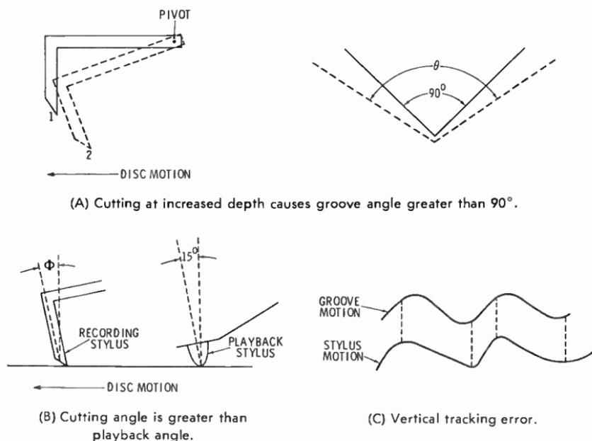
Fig. 12-14. Tracing angles for cutting and playback styli.
