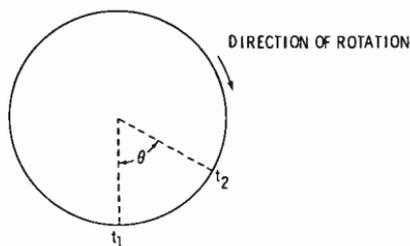
Fig. 12-1. A period of time is represented by a disc rotation of angle  $\theta$ .
