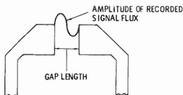
**Fig. 4-10.** The recorded wavelength is equal to the gap length, so the head produces no output.
