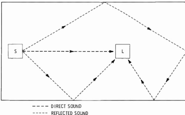
Fig. 1-8. In an enclosed space, some sound reflects off the surrounding surfaces before reaching the listener (L).
