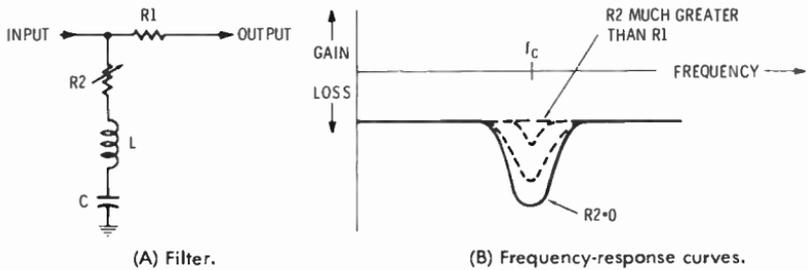
Fig. 5-17. A dip cut filter and frequency-response curves.
