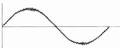
Fig. 7-2. Modulation noise on a sine wave.
