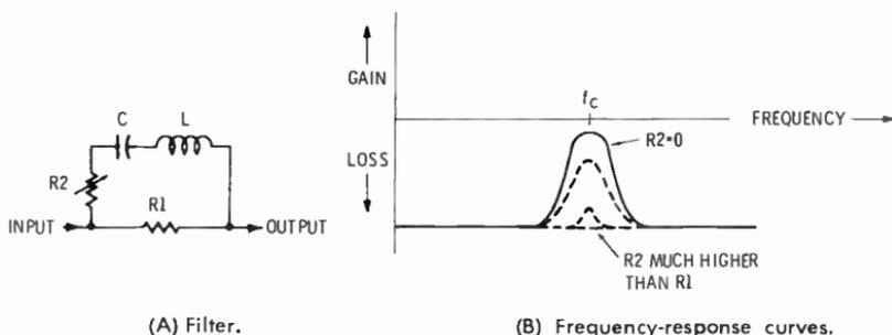
Fig. 5-16. A peak boost filter and frequency-response curves.
