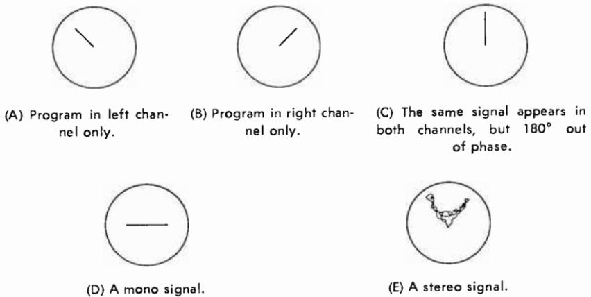
Fig. 12-24. Phase oscilloscope displays.
