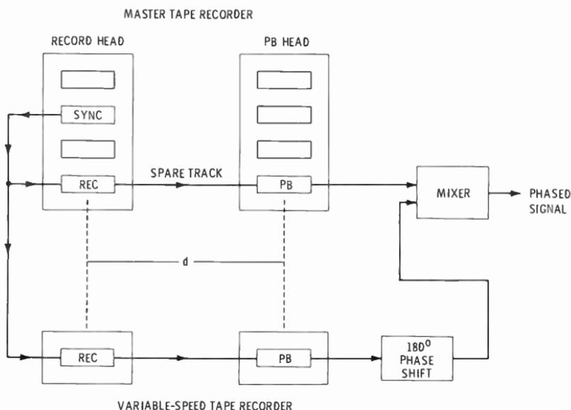
Fig. 5-70. The signal path to create the phasing effect using a master tape machine with a spare track and one extra recorder.
