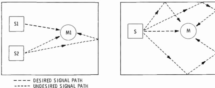
(A) The direct and reflected sound of  $S_2$  is picked up by the mike intended for  $S_1$  only. (B) Microphone  $M$  picks up the reflected sound as well as the direct sound from  $S$ .
