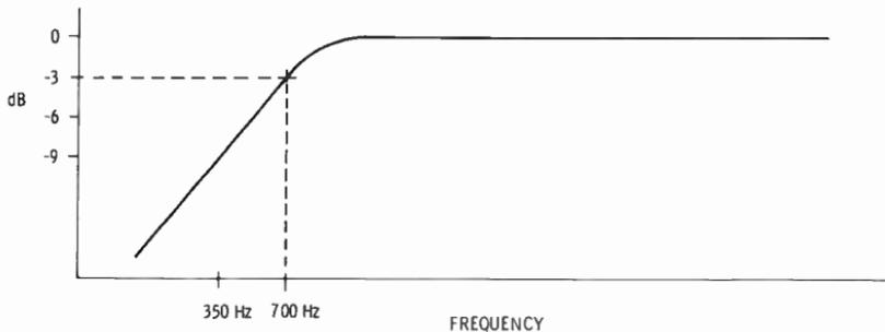
Fig. 5-19. A 700-Hz, high-pass filter with a slope of 6 dB per octave.
