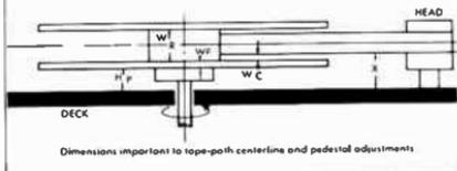
FIGURE 4. PEDESTAL HEIGHT & TAPE PATH DIMENSIONS (CONT.)
