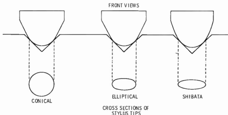
Fig. 12-18. Groove contact for the conical, elliptical, and Shibata styli.
