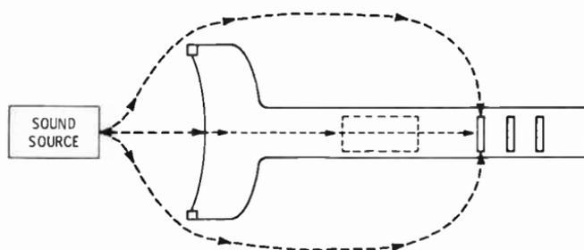
(B) Signal through port is shifted to be in phase with front signal.
