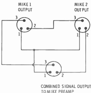
Fig. 3-28. Connecting two microphones in series. Pin 1 is ground, pin 2 is the high signal output, and pin 3 is the low signal output.
