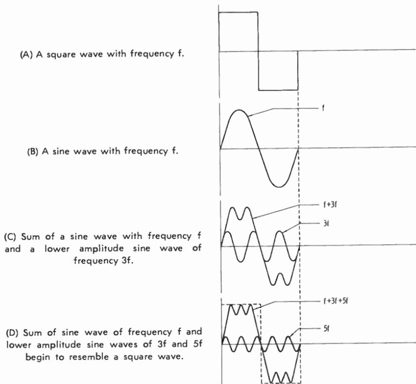
Fig. 2-8. Obtaining a square wave by adding odd harmonics.
