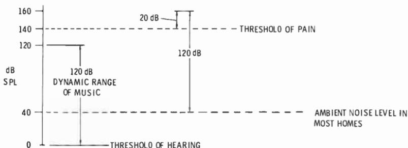
Fig. 5-28. The ambient noise level of most homes would obscure the lower 40 dB of a 120-dB dynamic range program. If the volume of the program is raised so that the softest portion is above the ambient noise, the loudest portion would be 20 dB above the threshold of pain.
