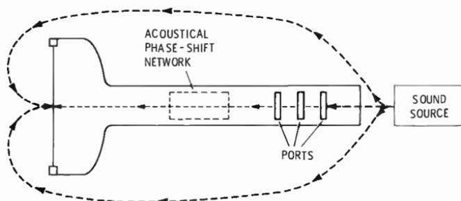
(A) Signals arrive at front and rear of the diaphragm.
