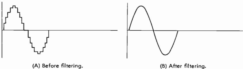
Fig. 7-23. Sine-wave output of a digital playback processor.
