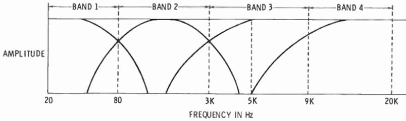
Fig. 7-7. The four filter bands of the A-type Dolby system.
