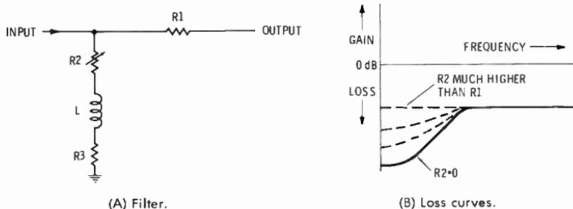
Fig. 5-12. A low-frequency shelf cut filter and loss curves.
