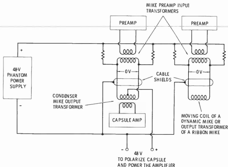
Fig. 3-20. The phantom powering system permits simultaneous operation of phantom-powered condenser microphones and dynamic or ribbon microphones.
