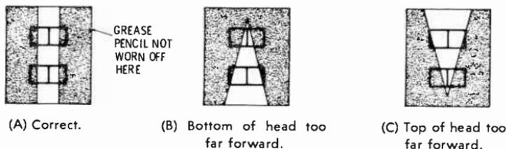
Fig. 4-26. Grease pencil wear patterns for checking zenith adjustment.
