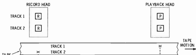
Fig. 4-17. If an overdub is attempted without the use of sel sync, the signal on track two will lag the original signal by a time equal to the distance ( $d$ ), divided by the tape speed.
