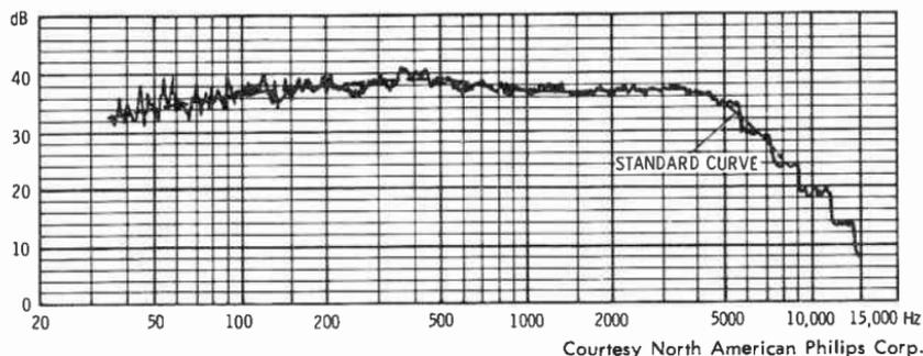
Fig. 5-54. BX20E frequency response measured with  $\frac{1}{3}$ -octave noise.
