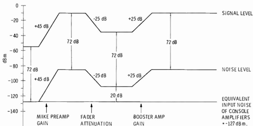
Fig. 3-23. Good console operating procedures do not degrade the signal-to-noise ratio.
