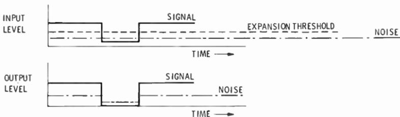
Fig. 5-34. When signal is above expansion threshold, gain is unity and both signal and noise appear at the output. When signal is below threshold, the gain decreases and reduces the level signal and the noise levels in the output.
