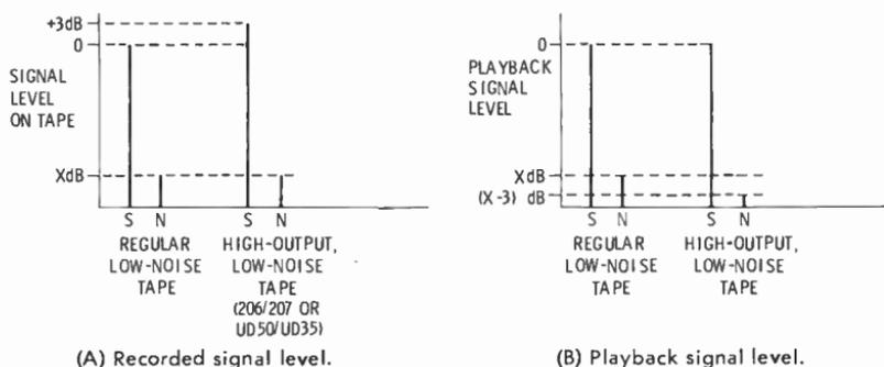
Fig. 4-21. Comparison of high-output, low-noise tape with regular low-noise tape.
