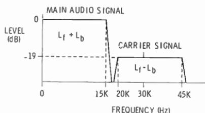
Fig. 13-13. The signals recorded on the inner groove wall of a CD-4 disc.
