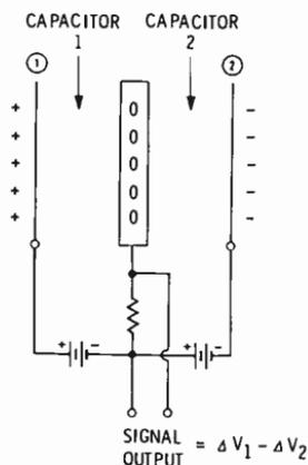
Fig. 3-18. A figure-eight condenser microphone. Operation is the same as in Fig. 3-16 except that capacitors 1 and 2 produce voltages across the resistor that are 180° out of phase with each other.
