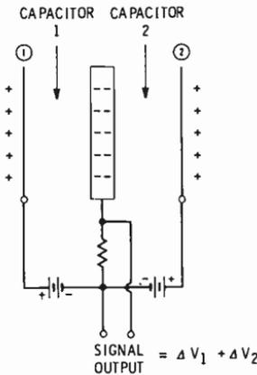
Fig. 3-16. An omnidirectional condenser microphone diagram.
