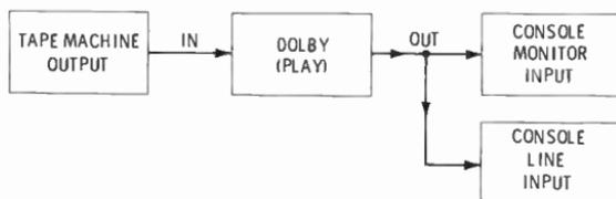
Fig. 7-12. Connecting the Dolby system for playback processing.
