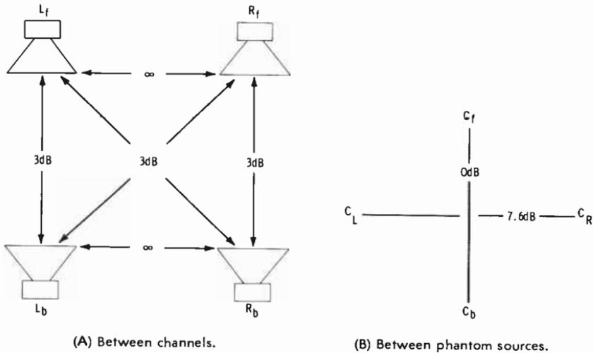
Fig. 13-4. Separation in the SQ system (with no logic or blending).
