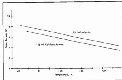
FIGURE 5. TEMPERATURE EFFECTS ON 5% ELONGATION POINT
