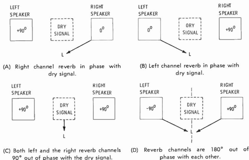
**Fig. 5-46.** The random phase relationship of the signals at the EMT plate outputs make the reverb appear to come from all directions.
