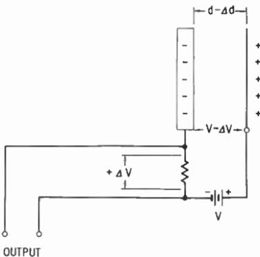
Fig. 3-14. If a sound wave decreases the plate spacing by  $\Delta d$ , the capacitance increases by  $\Delta C$  and the voltage across the plates falls by  $\Delta V$ .
