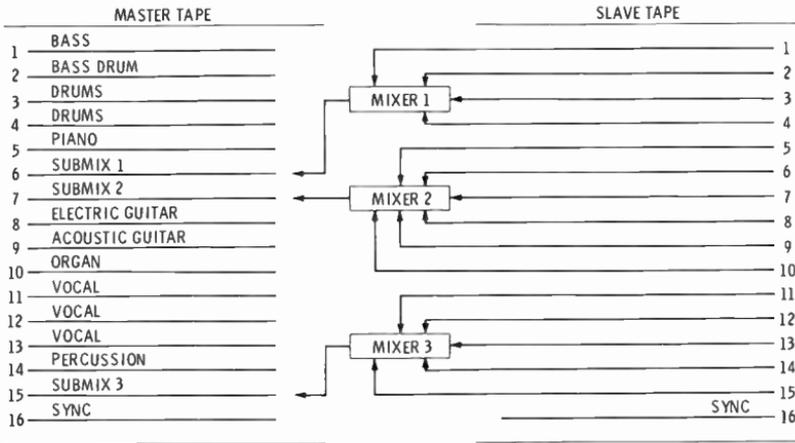
Fig. 10-6. Reducing the mixdown capacity requirements for interlocked tapes.
