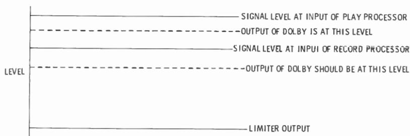
Fig. 7-13. The tape output is fed to the Dolby playback processor at too high a level.
