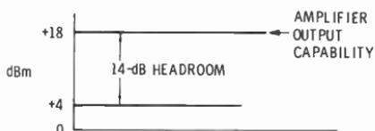
Fig. 5-27. If the console is to have 14 dB of headroom above 0 VU (+4 dBm), the amplifiers must be capable of output levels of at least +18 dBm.
