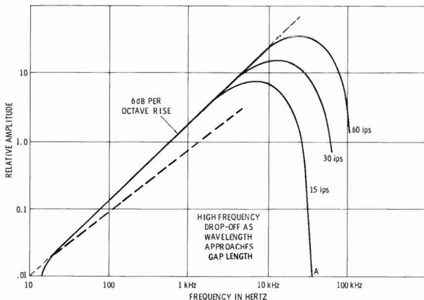
**Fig. 4-9.** The output of a playback head rises with frequency until the wavelength of the recorded signal approaches the gap length.
