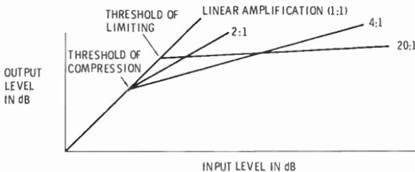
Fig. 5-33. The output of a compressor is linear below the threshold point and follows the slope of the selected compression or limiting curve above the appropriate threshold.
