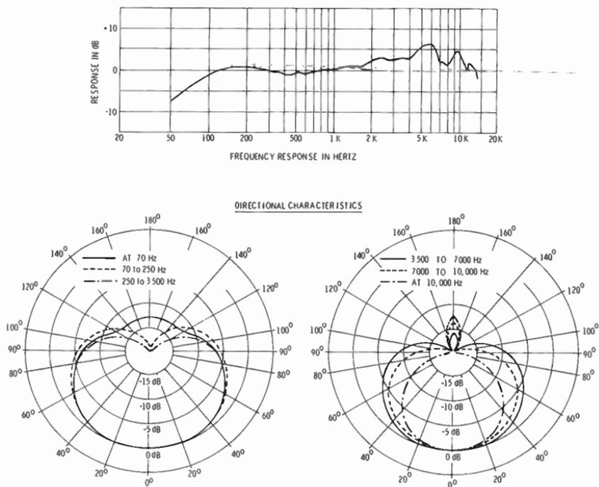
Fig. 3-34. The Shure SM57 dynamic cardioid microphone.
