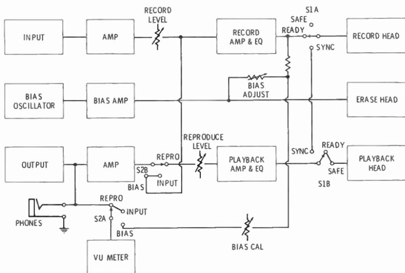
Fig. 4-16. A simplified block diagram of a single channel of AG440 electronics.
