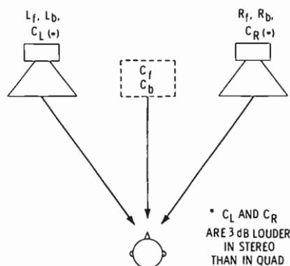
Fig. 13-14. The stereo stage created by a CD-4 encoded disc played in stereo.
