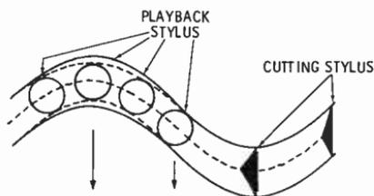
(A) Top view of a laterally modulated groove.
