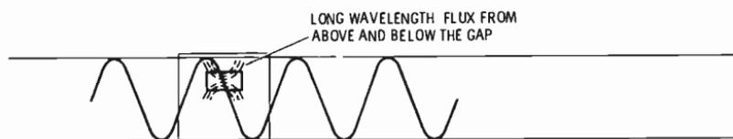
Fig. 4-23. A half-track mono head reproducing a tape recorded full track.
