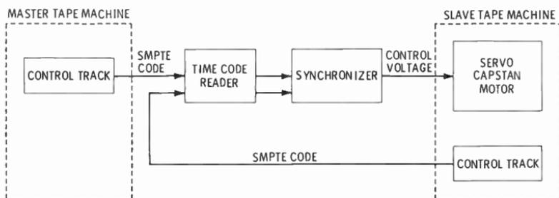
Fig. 10-10. Synchronizing two tape machines using the SMPTE code.
