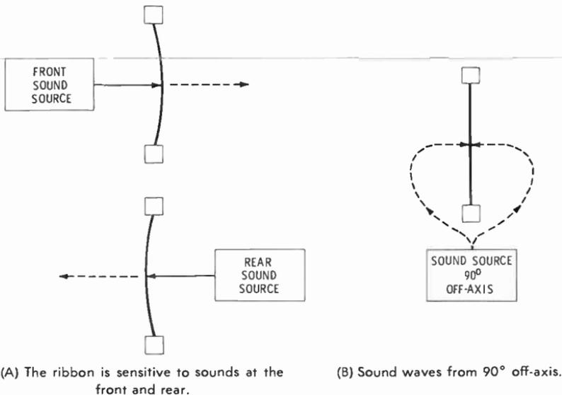
**Fig. 3-9. Sound sources on-axis and 90° off-axis at a ribbon mike.**
