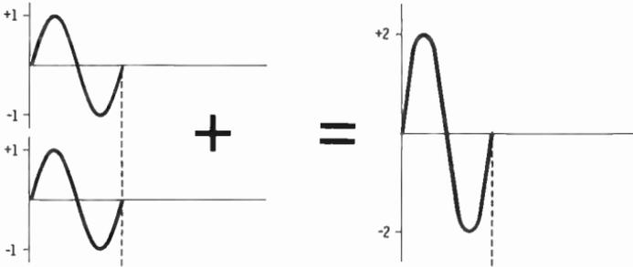
(A) The amplitudes of in-phase waves add when they are mixed.
