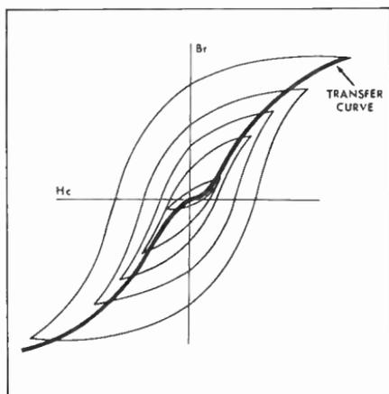
FIGURE 2. TRANSFER CURVE DERIVED FROM A FAMILY OF HYSTERESIS LOOPS
