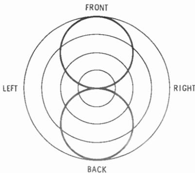
**Fig. 3-10. The normal pickup pattern of a ribbon microphone.**
