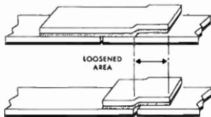
FIGURE 4. ENLARGED VIEW OF LOOSENED SPlice
