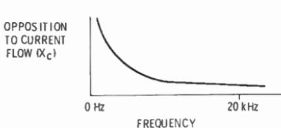
Fig. 5-7. Capacitive reactance ( $X_c$ ) is inversely proportional to frequency.
