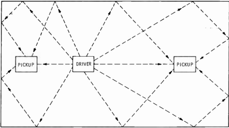
Fig. 5-44. The waves induced in the plate by the driver are reflected at the edges and converted into electrical signals by the pickups.
