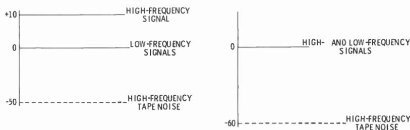
(A) High frequencies are boosted by 10 dB. (B) High-frequency signal level reduced to original level by the post-EQ.
