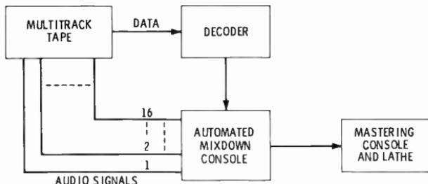
Fig. 11-12. Mastering a disc directly from a multitrack tape.
