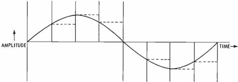
Fig. 7-21. The audio-signal amplitude is measured at each vertical line, and each measurement is converted into a binary word.
