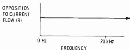
Fig. 5-6. The frequency response of a resistor is flat.
