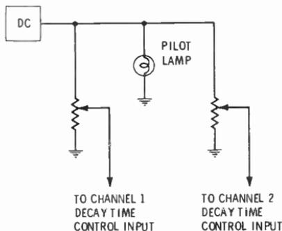
Fig. 5-55. The remote decay time-control circuit for the BX20E.
