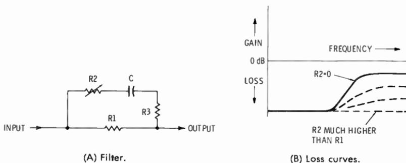
Fig. 5-10. A high-frequency shelf boost filter and loss curves.
