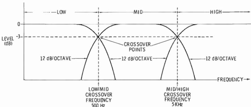
Fig. 8-4. Frequency response of a three-way crossover network with crossover frequencies of 500 Hz and 5 kHz.
