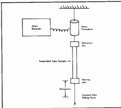
FIGURE 2. TENSILE STRENGTH TESTING APPARATUS DIAGRAM
