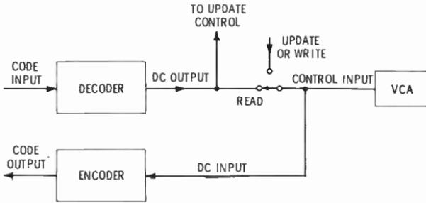
Fig. 11-10. The data for a function in the read mode is decoded and then re-encoded when recorded onto the other data track.
