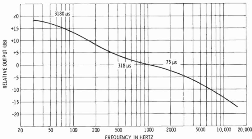
Fig. 12-20. The RIAA disc playback equalization curve.
