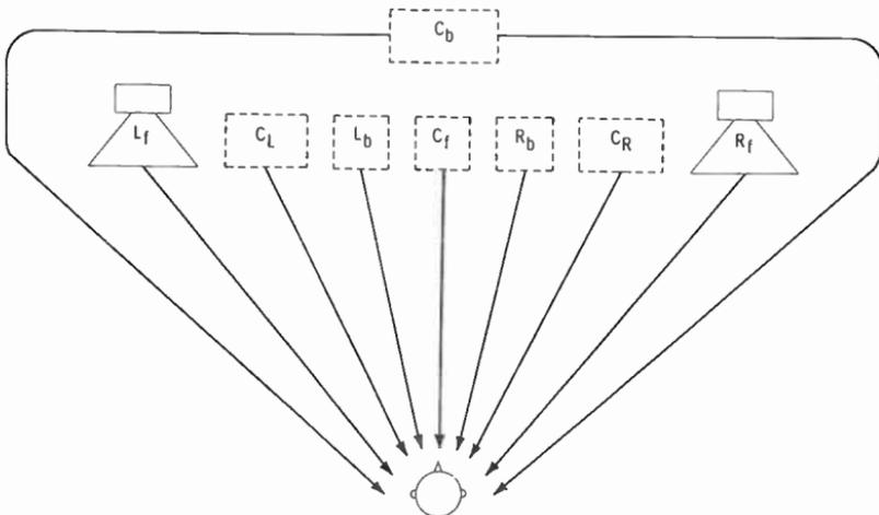
Fig. 13-7. The stereo stage created by an SQ-encoded disc played in stereo.
