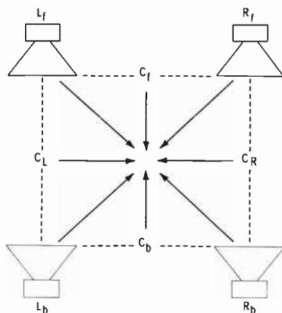
Fig. 13-2. The four sound sources in a quad system and the four principal phantom source images.
