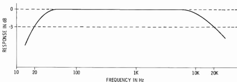
Fig. 4-13. A frequency-response curve with a 20-Hz lower cutoff frequency and a 20-kHz upper cutoff frequency.
