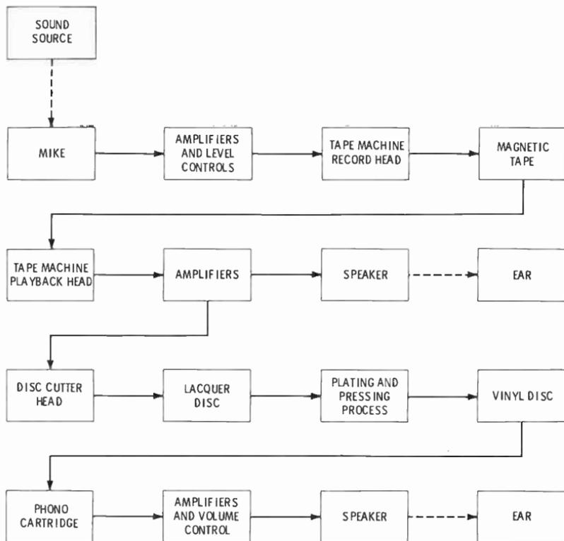
Fig. 1-3. The recording chain.
