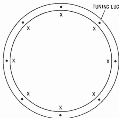
Fig. 9-5. Tuning a drum head. The pitch should be the same at each point around the rim (marked by Xs).
