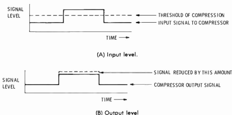
Fig. 5-29. The compressor reduces the level of the portion of the signal that exceeds the threshold.
