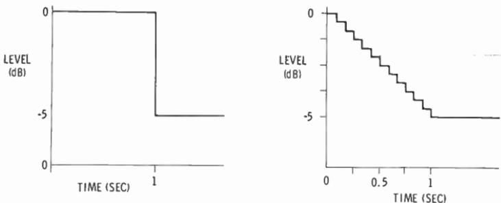
(A) Updating occurs once each second. The fade is encoded as a step change of 5 dB.
