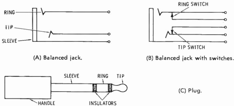
Fig. 6-5. Types of balanced jacks, and plug used with them.
