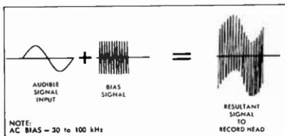
FIGURE 1. PRODUCTION OF RESULTANT SIGNAL
