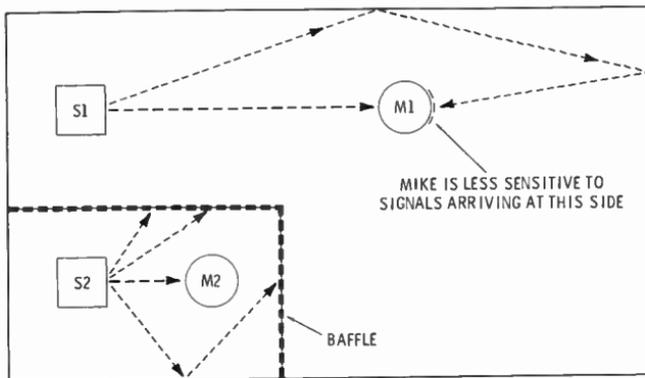
Fig. 1-11. Close miking using sound-absorbing baffles and unidirectional mikes.
