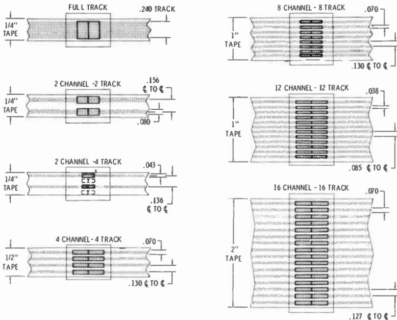
Fig. 4-19. Some track configurations available for magnetic tape recording.
