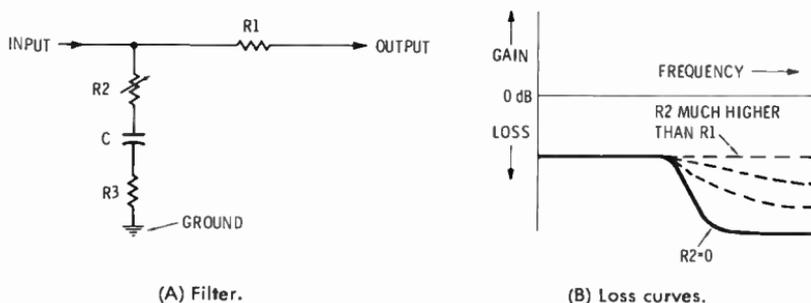
Fig. 5-11. A high-frequency shelf cut filter and loss curves.
