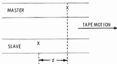
Fig. 10-5. Sync tones are regular and continuous waves. Thus the resolver can lock any two cycles together.
