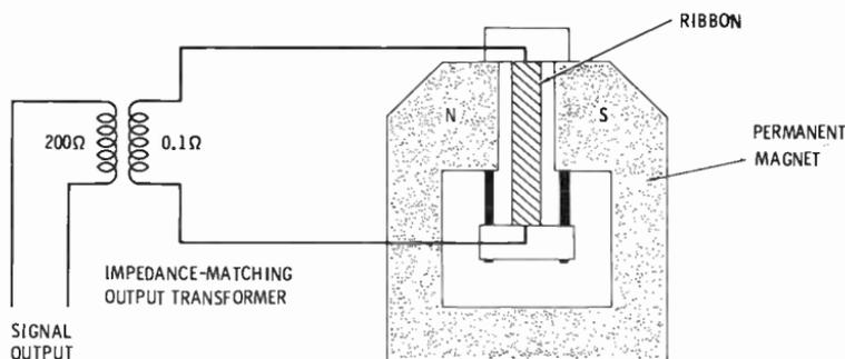
**Fig. 3-8. The basic components of a ribbon microphone.**
