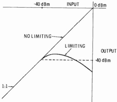
Fig. 7-4. Output of the limiter used in the Dolby system rises slightly above -40 dBm.
