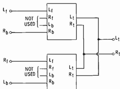
Fig. 13-8. Connecting two SQ encoders to permit encoding along the  $L_t/R_b$  and  $R_t/L_b$  diagonals.
