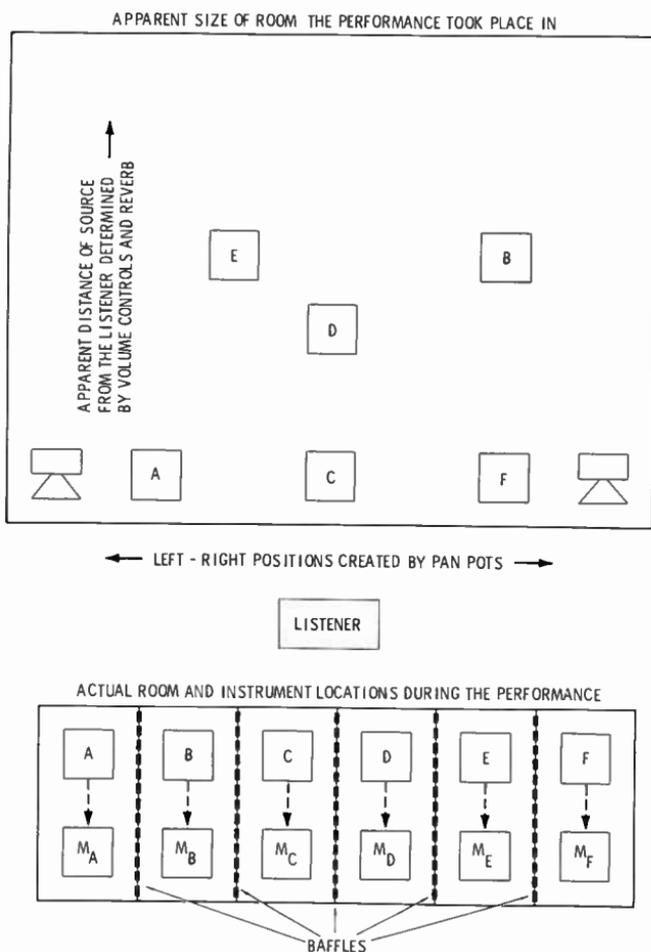
Fig. 1-12. Close-miked instruments A through F can be made to appear as if they originate from various locations in an imaginary stage behind and between the stereo speakers.
