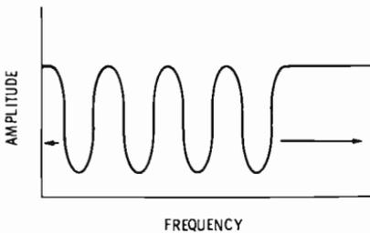
Fig. 5-68. The phasing effect creates a comb filter with variable dip frequencies.
