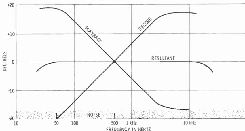
Fig. 4-11. The basic EQ used for magnetic recording.
