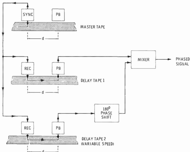
Fig. 5-69. The signal path to create the phasing effect using a master tape machine and two extra recorders.
