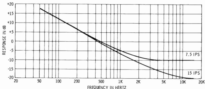
(D) Typical post-equalization curves for 1/4-inch recorders using CCIR characteristics at 7.5 and 15 ips.
