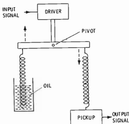
Fig. 5-51. A simplified diagram of a spring reverb unit using oil to damp the vibrations.
