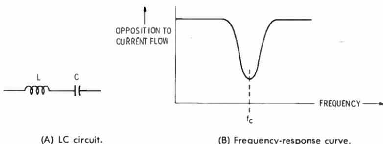
Fig. 5-15. A series LC circuit and frequency-response curve.
