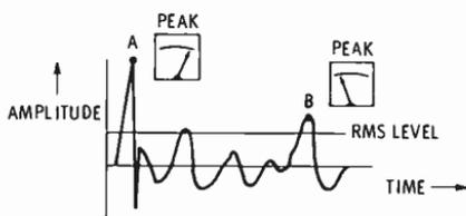
Fig. 5-24. A peak meter reads higher at point A than at point B, even though the loudness is the same.
