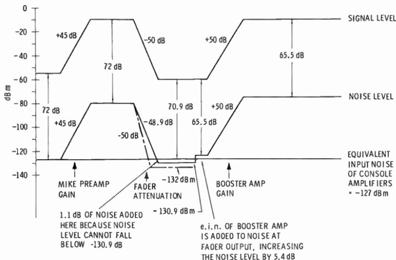
Fig. 3-24. Attenuating the input signal within  $20$  dB of the amount of the mike preamp gain lowers the signal-to-noise ratio.
