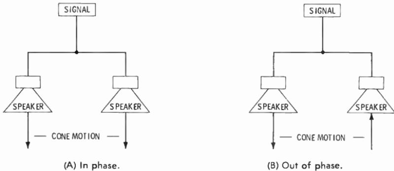
Fig. 8-5. Relative cone motion, speakers in phase and out of phase.
