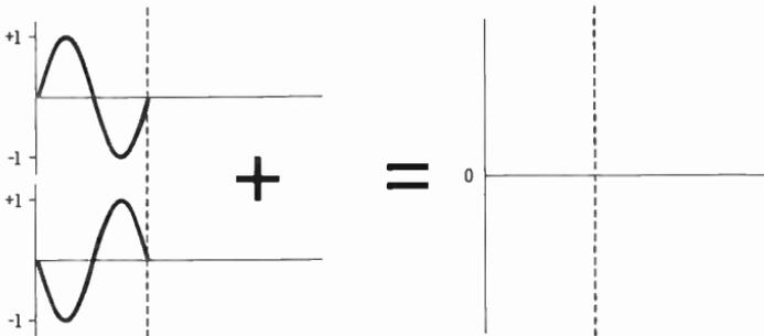
(B) Waves of equal amplitude cancel completely when mixed  $180^\circ$  out of phase.
