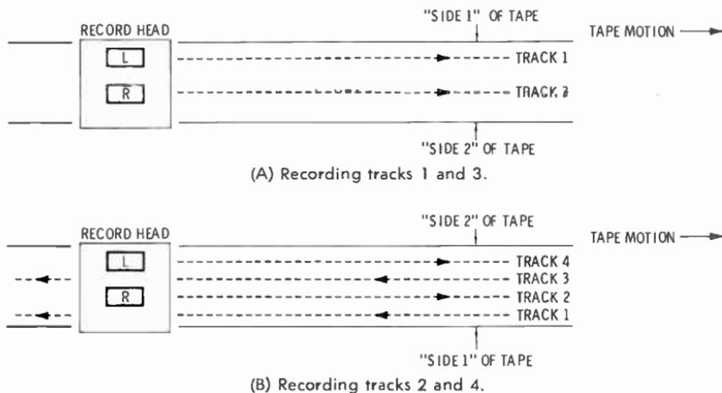
Fig. 4-20. The quarter-track stereo configuration.
