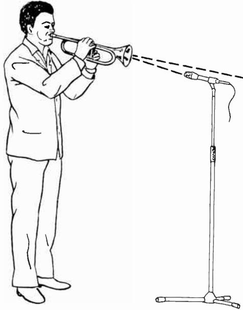
Fig. 8-4. Typical mike positioning for single trumpet.
