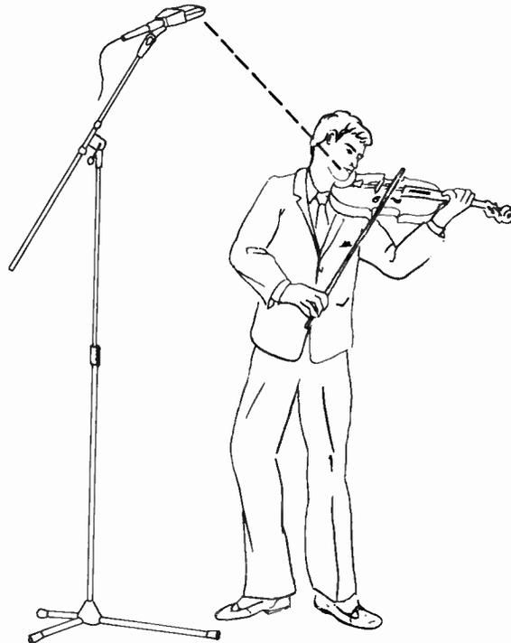
**Fig. 8-23.** Typical pickup placement of violin.
