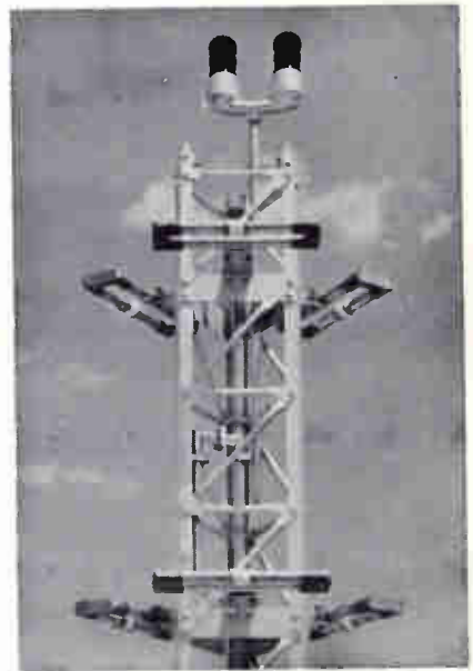
Fig. 2-16. Low-Power Antenna with Power Gain of Two. Courtesy of Prodelin, Inc.
