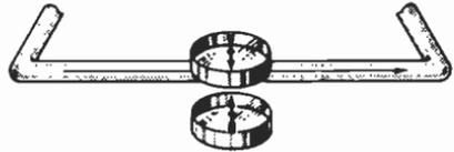
**Fig. 9-3.** One way to determine the direction of the lines of force.
