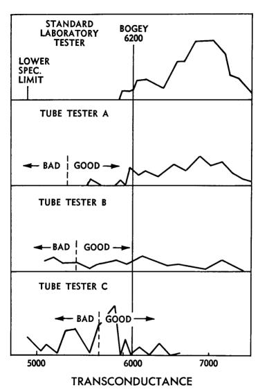
Fig. 8-1. Comparison of results obtained when a number of tubes were tested in three commercial tube testers and in a standard laboratory tester.
