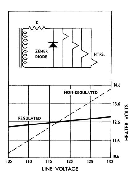
Fig. 10-1. Zener-diode regulator and chart, showing the improvement of the voltage stability.
