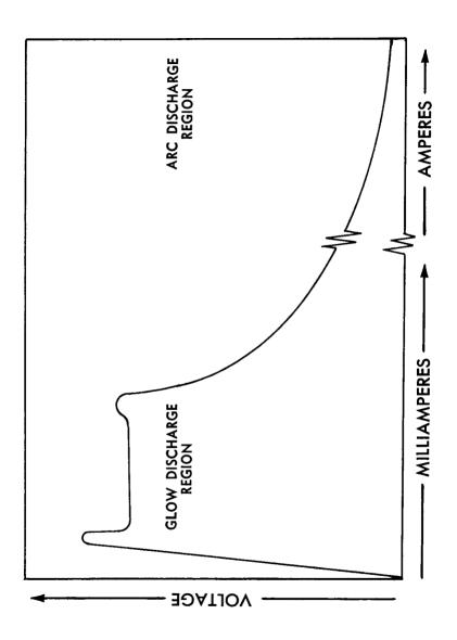
Fig. 9-3. A curve showing the glow-discharge and arc-discharge regions of voltage-regulator tubes.
