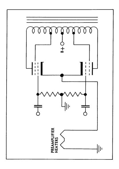
Fig. 3-3. Using amplifier cathode current for heaters. The heater voltage drop provides the necessary bias for the output stage.
