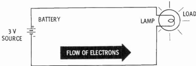
This process continues until the charges on the two terminals are equal. This does not mean the terminals have to be so completely neutralized that no electrical charge exists on either terminal. Under this condition, the battery is discharged (run down).
