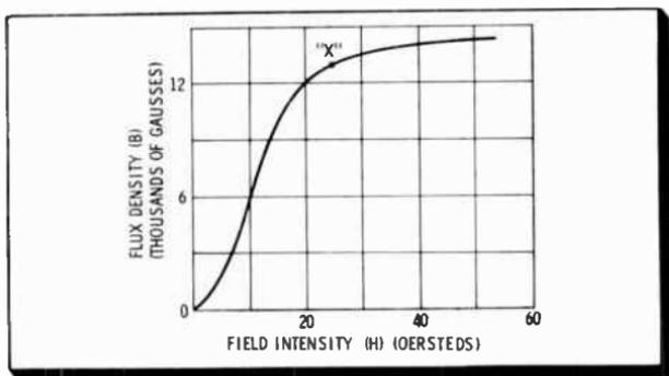
The flux density increases rapidly with only a slight increase in the magnetizing force when the core material is at a point of low field intensity (only a few thousand magnetic lines of force). At a point of high field intensity, a large change in the magnetizing force is required to cause a small change in flux density. Point X indicates the point of saturation.
