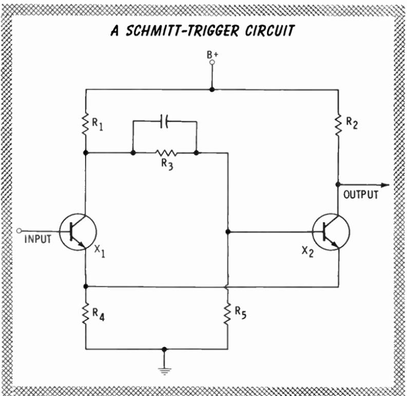
With no input, transistor  $X_1$  is cut off, and its collector voltage equals the battery voltage. This voltage is coupled to the base of  $X_2$  through  $R_3$ . Transistor  $X_2$  is therefore saturated. Due to the emitter current of  $X_2$ , the top of resistor  $R_4$  is positive.
