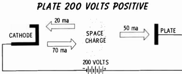
If the plate voltage is increased to 200 volts, the plate current becomes 50 ma, and the current returned is 20 ma.
