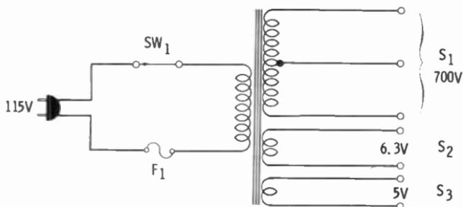
The diagram above shows a power transformer similar to those used in some radio receivers. It has three secondary windings— $S_1$ ,  $S_2$ , and  $S_3$ . Disregard the center tap on  $S_1$ .
