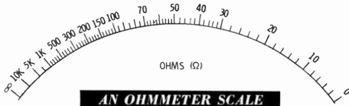
**Meter Scale**—The meter scale reads from zero to infinity, as indicated by the symbol  $\infty$ . Because it is so great, infinity has no numerical value. The “K” on the scale stands for 1,000; therefore, 5K equals 5,000 ohms.
