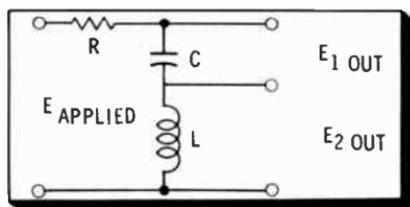
If the voltage across either L or C is used for the output, the voltage will be much greater for signals having the resonant frequency than for signals above or below this frequency. Such a circuit is called a **bandpass filter**.
