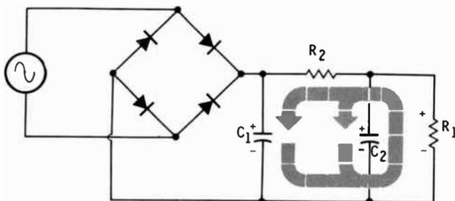
By adding another capacitor in parallel with the load resistor and another current-limiting resistor in series with the discharge path, the filter network can reduce more of the ripple.
