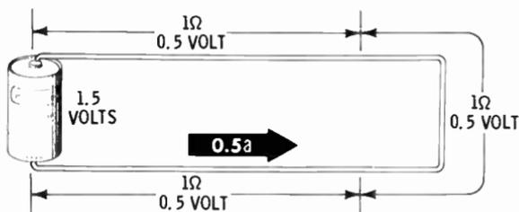
All of the source voltage is distributed proportionally across the resistance in a circuit. The voltage drop between any two points in a circuit can be determined by the ratio of the individual resistance to the total resistance of the circuit. The diagram, for example, shows a 3-yard length of wire connected to the terminals of a 1.5-volt cell. The resistance of the wire is one ohm per yard, or a total of
