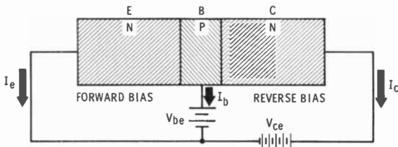
reverse bias between collector and base is provided by  $V_{ce}$  in series with but opposing  $V_{be}$ , and  $V_{ce}$  is large compared to  $V_{be}$ . Thus,  $V_{ce}$  replaces  $V_{cb}$  in series with  $V_{be}$ . This is called a grounded-emitter circuit.
