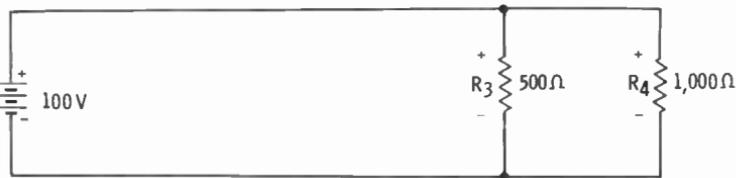
Using the same reasoning ( $I = E/R$ ), it will be found that the current through  $R_3$  in the above circuit is 0.2 amp. The current through  $R_4$  is 0.1 amp. The total current is 0.3 amp.
