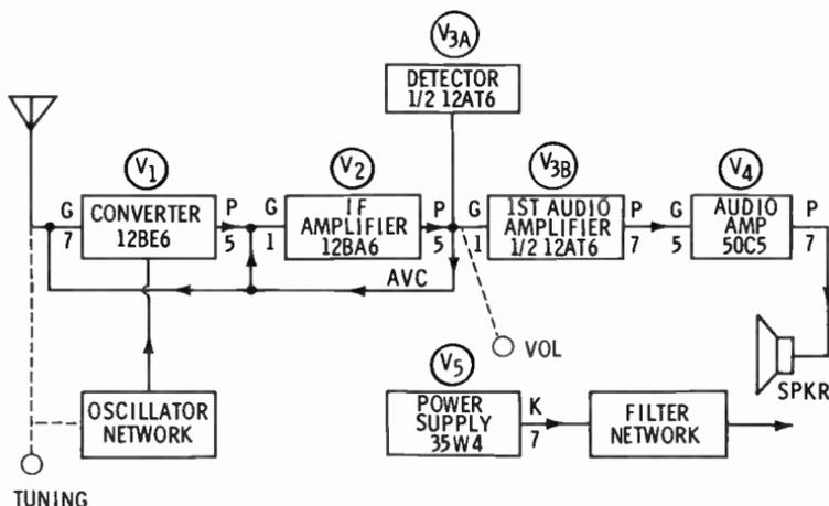
With waveforms shown between stages and input and output tests points identified, a servicing block diagram can be used for isolating a faulty circuit. In the above diagram, V<sub>1</sub>, V<sub>2</sub> and V<sub>3A</sub> are included in the RF function, and V<sub>3B</sub> and V<sub>4</sub> in the audio function. V<sub>5</sub> is the power-supply tube.
