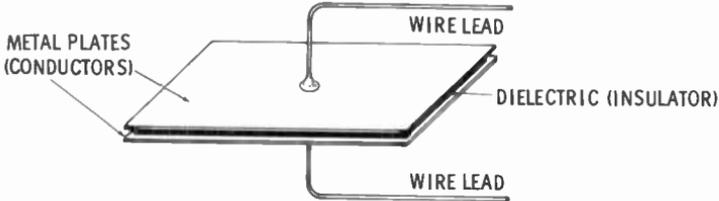
This basic principle is elaborated upon to produce the shapes shown on the opposite page. For example, the plates of the variable capacitor are curved and exposed. Since air is an insulator, it forms the dielectric.
