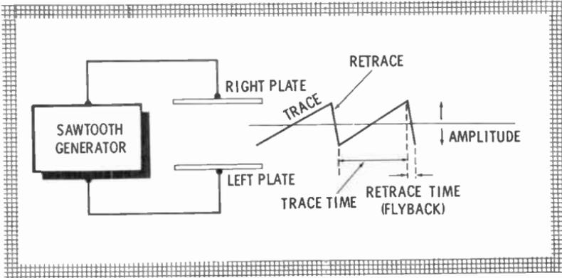
At the reference line, the potential on both plates is equal. Below the line the waveform makes the left plate more positive, and above the line the right plate is made more positive than the other. The waveform amplitude causes a uniform movement of the beam across the screen. The retrace line (trailing edge of the waveform) brings the beam quickly back to the starting point.
