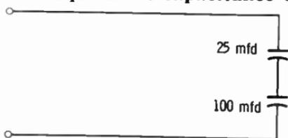
**Q6. What is the equivalent capacitance of this circuit?**
