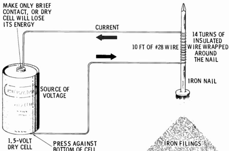
Current flowing through a wire develops a magnetic field. This field is called an **electromagnetic force** because it is the result of the flow of electric current. If, as shown in the illustration, the magnetic field passes through certain kinds of metal, such as soft iron, the metal will become **magnetized** and take on the properties of a magnet.
