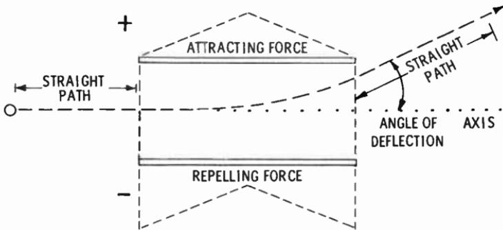
**Length of Field**—A long field has more time to exert its deflecting forces on an electron beam than a shorter field. Therefore, it bends the beam to a greater deflection angle. This fact assumes that all other factors are equal.
