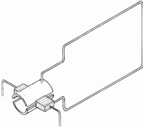
coils. Also, if the commutator of a DC generator is not adjusted to reverse the armature coil connections at the moment when the induced emf is zero, the output of the generator will not be DC. Instead, it will be AC as shown in the figure below.
