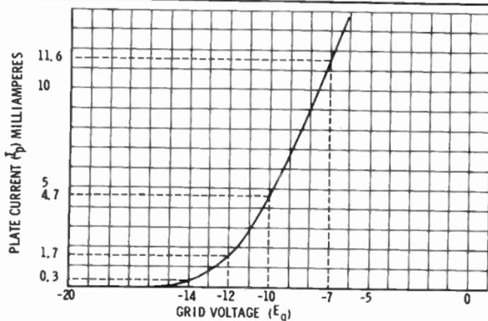
Q10. Determine  $R_p$  for each of the points on the graph.
