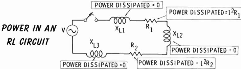
Go through all the steps necessary to find the power dissipated in the following circuit. (See Q24 through Q27.)
