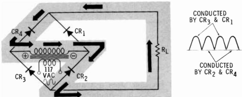
The figure above shows the current direction for the negative half cycle.
