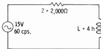
A30.  $X_L = 1,507 \text{ ohms}$      $I = \frac{E}{Z} = \frac{15}{3,000} = 5 \text{ ma (approx.)}$
