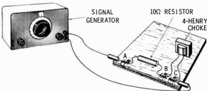
Voltages can be measured between points A and C, A and B, and B and C. Pick about 12 equally spaced frequencies. Using each as an input, measure and record both the input and output voltages.
