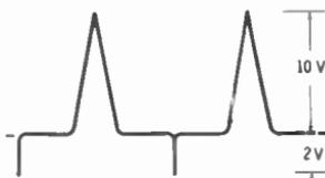
Your answer might be merely voltage. This would be a good answer, since you did not specify the amount of voltage. A multimeter or a VTVM is designed and has its scales calibrated to measure sinusoidal (sine-wave) AC voltages. It cannot accurately measure a nonsinusoidal voltage. Since the meter pointer is not able to follow the rapid rise and fall of such a voltage, the meter reading, if any, will be only a slight indication.
