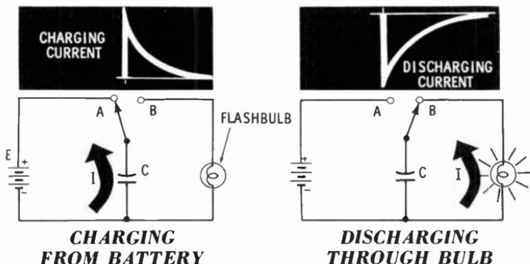
Capacitor  $C$  is charged up to the battery voltage by throwing the switch to position A. The rate of charge depends on the resistance in the battery circuit (wire resistance and internal resistance of the battery). When a flash is desired, the switch is moved over to position B. The capacitor, which
