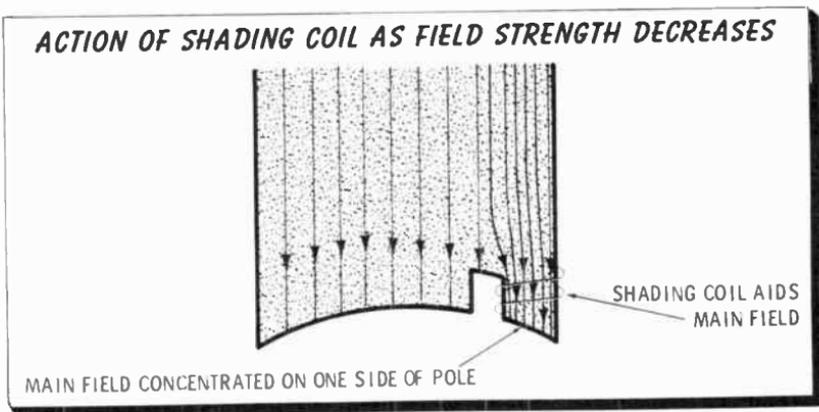
The effect of the shading coil is to produce a small sweeping motion of the main field from one side of the pole piece to the other as the field pulsates. This slight rotating motion is enough to start the motor.
