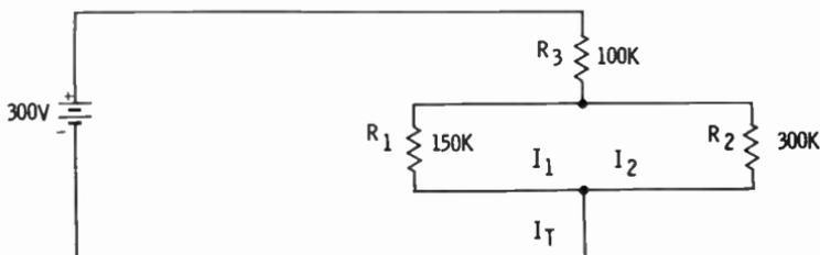
To find the effective load for the 300V source,  $R_T$  must be calculated. One approach for finding  $R_T$  is to first find the total resistance for the parallel branch ( $R_1$  and  $R_2$ ); then the sum of the total parallel resistance plus  $R_3$  should be found. After the total resistance has been determined, the total current can be calculated.
