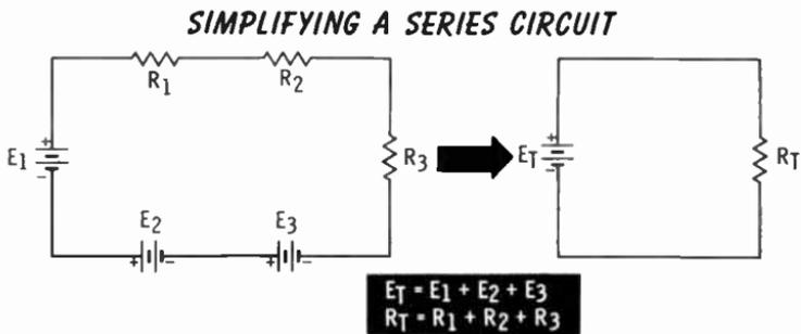
**Q4. How must you treat the following series circuit to find the total source voltage?**
