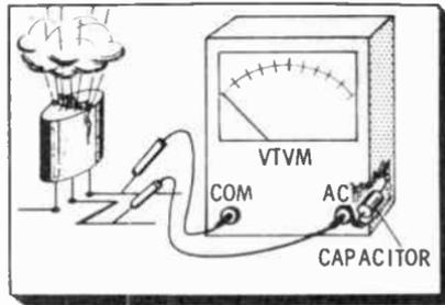
During the circuit-checking tests it is best to remove the transistor if it is the plug-in type. Removal is not absolutely necessary if you exercise necessary care.
