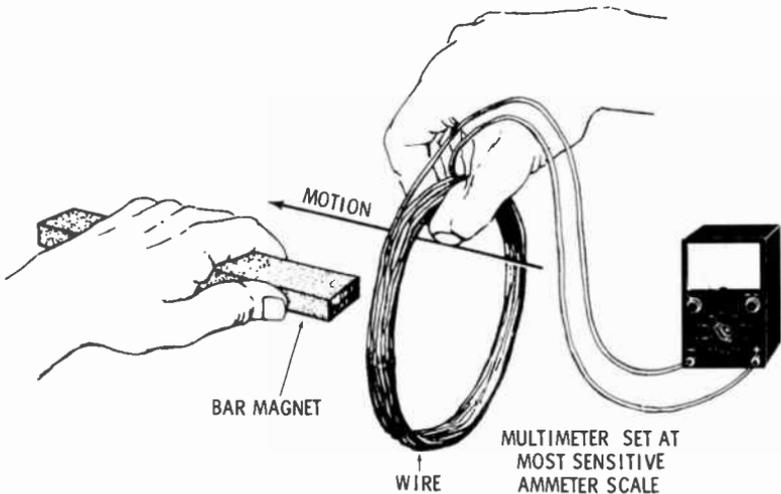
If an electric conductor is moved through a magnetic field in such a way that it cuts the lines of force, a voltage is generated, or induced, in the conductor. The induced voltage is greatest when the conductor moves at right angles to the magnetic field, and is zero when the conductor moves parallel to the lines of force.
