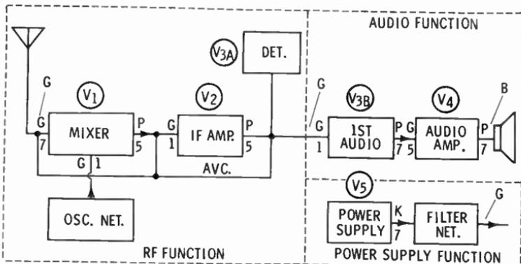
Good test indications are made at the input of  $V_1$ , the input of  $V_{3B}$ , and the output of the filter network in the power supply. A bad test is identified at the speaker input.
