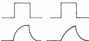
When dealing with filters and pulse circuits, circuits containing L and R in series are often described by their **time constant**. This is a measure of how quickly the current in the circuit reaches its final peak value. The time constant equals  $L/R$  and is expressed in seconds. If a circuit has an  $L/R$  time constant of one-half second, the current will reach 63% of its maximum (peak) value in one-half second when a voltage is applied to the circuit.
