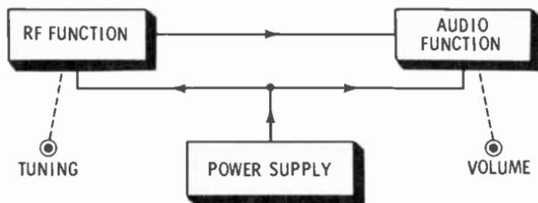
Try another problem. During Step 1, no stations are heard, regardless of where the tuning control is set. The dial lamp is on. Rotation of the volume control causes an increased crackling, rushing noise in the speaker. In which function(s) would you expect to find the trouble?
