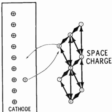
Finally, a point is reached where, when a sufficient quantity of electrons has been emitted, the cloud has enough negative charge to force newly emitted electrons back to the cathode. From then on, for every electron emitted by the cathode, one will be returned to the cathode. This condition of equilibrium is called **emission saturation**. The cloud of electrons around the cathode is called the **space charge**.
