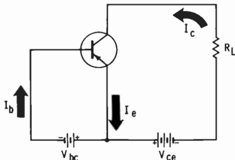
As you know,  $\alpha$  is the ratio of collector-current change to emitter-current change and is equal to  $\frac{\Delta I_c}{\Delta I_e}$ . It is also called the **common-base, forward-current transfer ratio**. If the transistor were connected in a common-base circuit,  $\alpha$  would represent its current gain (with the collector voltage held at a constant value).
