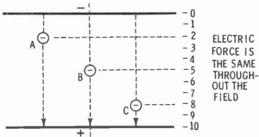
In the figure above, three electrons are located in an electrostatic field. All three are attracted by the positive plate and repelled by the negative plate. The distance between the plates is marked off in 10 equal units; electron A is 2 units away from the negative plate, electron B is 5 units away, and electron C is 8 units removed.
