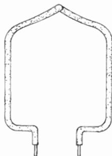
Sometimes the distance between the two sides of an armature coil is not equal to the distance between the adjacent magnetic poles. When this distance is less than the pole pitch, the coil is called a **fractional-pitch winding**.
