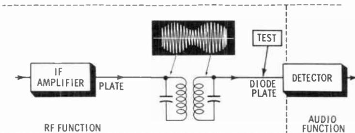
From the schematic diagram of the receiver, locate the pin number of the upper diode plate of the detector. Connect the oscilloscope to the proper socket terminal and rotate the tuning control. If no audio-modulated signal is noted at several station settings, the RF function is not operating properly.
