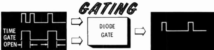
In gate-circuit action, several signals must be present at the same time for an output to be obtained. In the figure you see one signal which opens the gate at regular intervals. However, the only time there is an output is when two signals are present at the same time.
