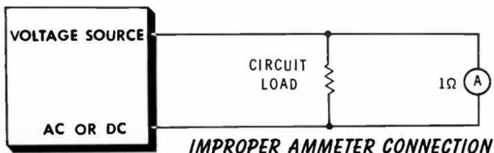
You are right, it would be damaged. But do you know why? The full voltage of the source is applied across the 1-ohm resistance of the meter. Even if the source were only a 1.5-volt dry cell, more than an ampere of current would flow through the meter. Some meters are designed to handle that amount of current, but a multimeter is not.
