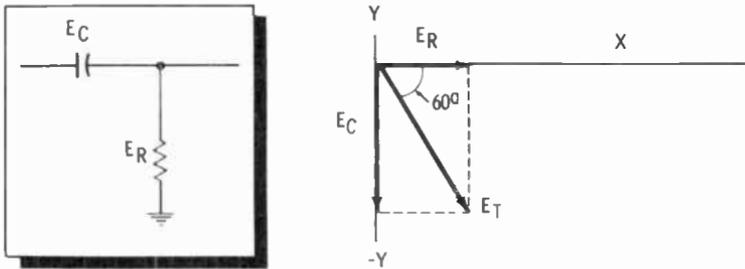
The values of  $C$  and  $R$  are selected so that the current in the circuit leads the applied voltage ( $E_T$ ) by an angle of  $60^\circ$ . The voltage ( $E_R$ ) across the resistor also leads the applied voltage by  $60^\circ$ ;  $E_R$  is the output voltage of the RC combination. Three RC combinations produce a phase shift of  $180^\circ$ .
