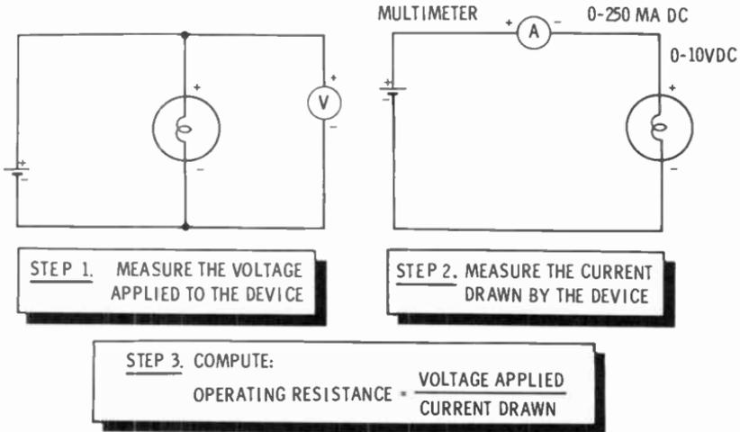
This method of measuring resistance is called the **voltmeter-ammeter method**. Using this method you will find that the dry cell measures very close to 1.5 volts and the current very near 200 milliamps (0.2 amp). In this case, the resistance will be 7.5 ohms. The arithmetic statement says that if you divide volts by amperes the answer will be the value of the heated resistance in ohms.
