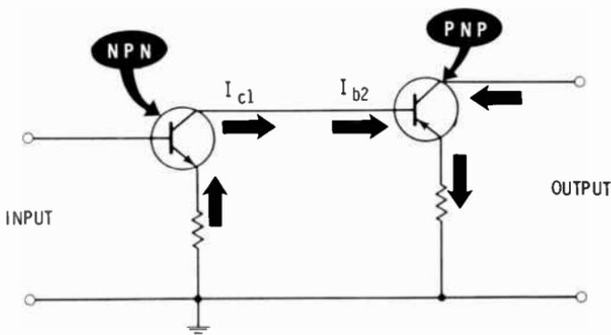
In the NPN transistor of the first stage, the collector current flows out of the transistor. In the base circuit of the second-stage PNP transistor, the base current flows into the transistor. If the NPN collector is coupled directly to the PNP base, the current between them flows in the same direction. (For simplicity the power supplies are not shown on the diagram.)
