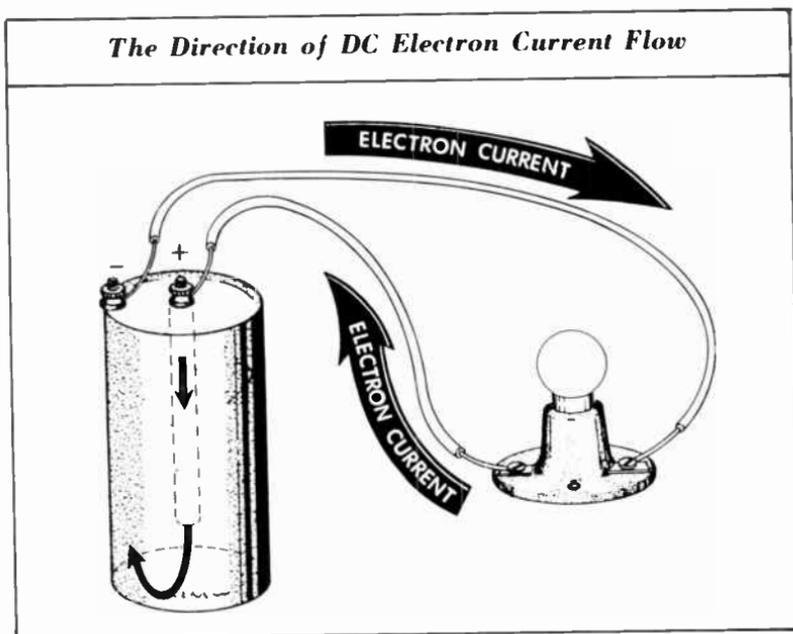
Q36. The connecting posts on the cell in the illustration are marked (+) and (-). The (+) post is the \_\_\_\_\_ terminal.
