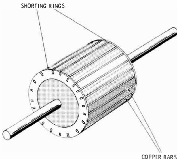
the rotor instead of a wire winding. The winding resembles a squirrel cage, from which it derives its name. The squirrel-cage motor has the advantages of requiring practically no maintenance and of costing much less than a wound-rotor motor.
