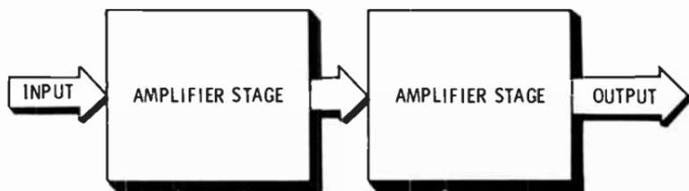
In a multistage amplifier chain, voltage amplifiers are generally used for all but the output stage. In this way only very small currents are handled. The signal is gradually developed to a higher voltage but with very little power. Only in the last stage is the signal converted into the necessary power output.
