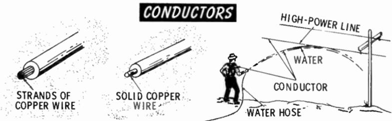
Some materials are better conductors of electricity than others. The availability of more free electrons in silver and copper, for example, makes them better conductors than iron or steel.
