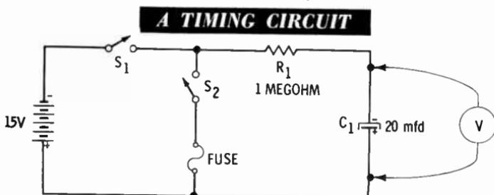
The resistor limits the amount of current flow which charges  $C_1$ . The values of  $R_1$  and  $C_1$  determine the charge time.
