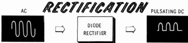
In the figure above, an AC signal is shown entering a diode rectifier and leaving as pulsating DC. This first step in changing AC to DC is called **rectification**. It is the basis for all electronic power supplies.
