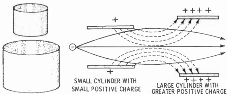
approaches the larger, more positively charged cylinder, the velocity of the electron will increase.
