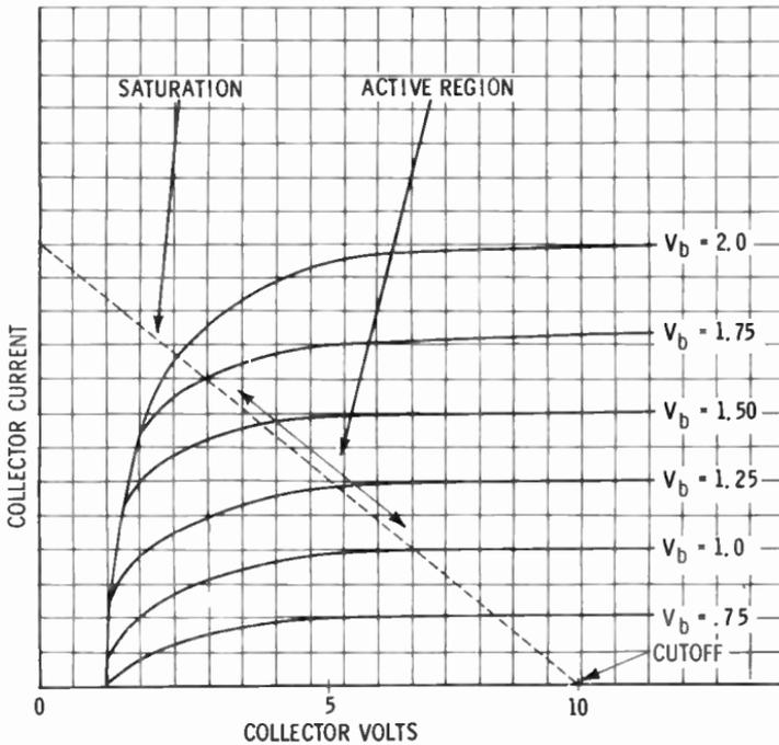
uration regions are called the **quiescent** and **stable** states, respectively. When the emitter-base and collector-base junctions are reverse-biased, the transistor is in the quiescent state. When both junctions are forward-biased, the transistor is in the saturated state.
