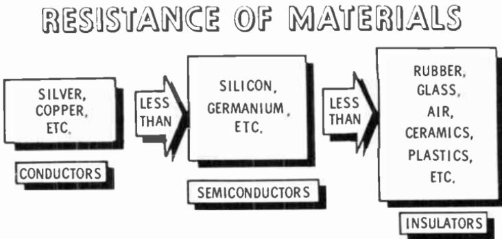
Most metals contain atoms that release electrons very easily. These materials, therefore, offer the least resistance to current flow. Insulators have the greatest resistance because their atoms resist the release of electrons. The in-between materials are neither good conductors nor insulators. Among these are certain materials, the **semiconductors**, from which **transistors** are manufactured.
