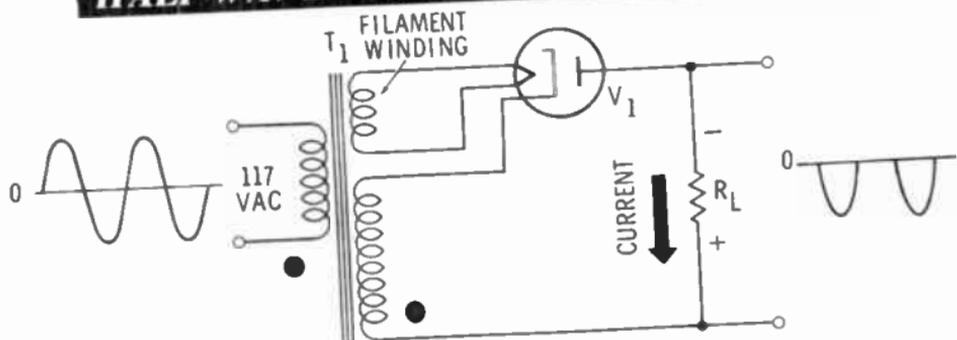
In its operation, this circuit is very similar to the semiconductor half-wave rectifier. On the positive half cycles, a positive voltage is applied to the cathode of the diode, and the diode will not conduct. On the negative half cycles a negative voltage is applied to the cathode, and the diode does conduct. Current flows down through  $R_L$ , producing an output of the polarity shown. Thus, only negative half cycles appear at the output.
