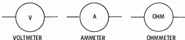
You should recognize these meters as the three types built into a multimeter. They are also available as separate meters.
