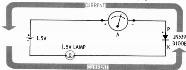
With the connections made as shown, current will flow and the lamp will light. The ammeter will record very close to 200 milliamps. Now reverse the connections of the diode. Will the lamp light? No. And, as indicated in the next drawing, the meter pointer will remain on zero. The plate-to-
