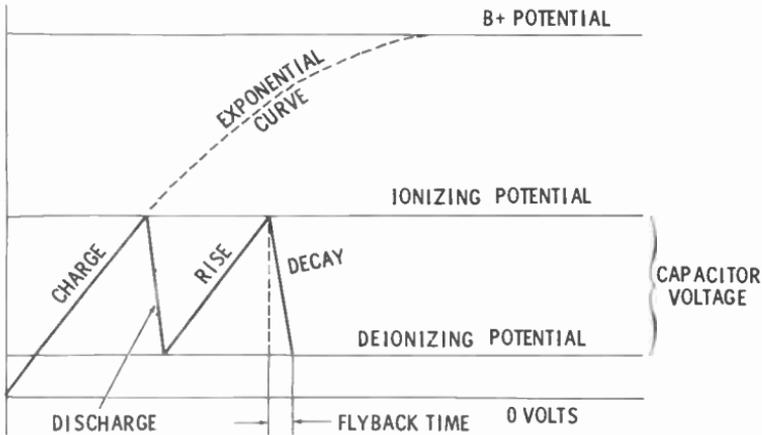
across the capacitor, the capacitor discharges rapidly. When the capacitor voltage falls to the **deionizing potential** of the tube, the thyatron stops conducting and acts as an open switch. Then the cycle repeats. The charge of the capacitor corresponds to the rise of the sawtooth, and the discharge corresponds to its decay.
