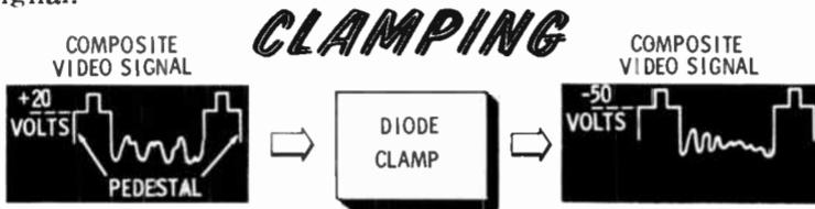
Another use for a diode is to maintain a special voltage level for a signal—this is called **clamping**, or **DC restoration**. The figure above shows a composite video signal whose pedestal is riding at positive 20 volts. The diode clamp causes this pedestal to ride at negative 50 volts.
