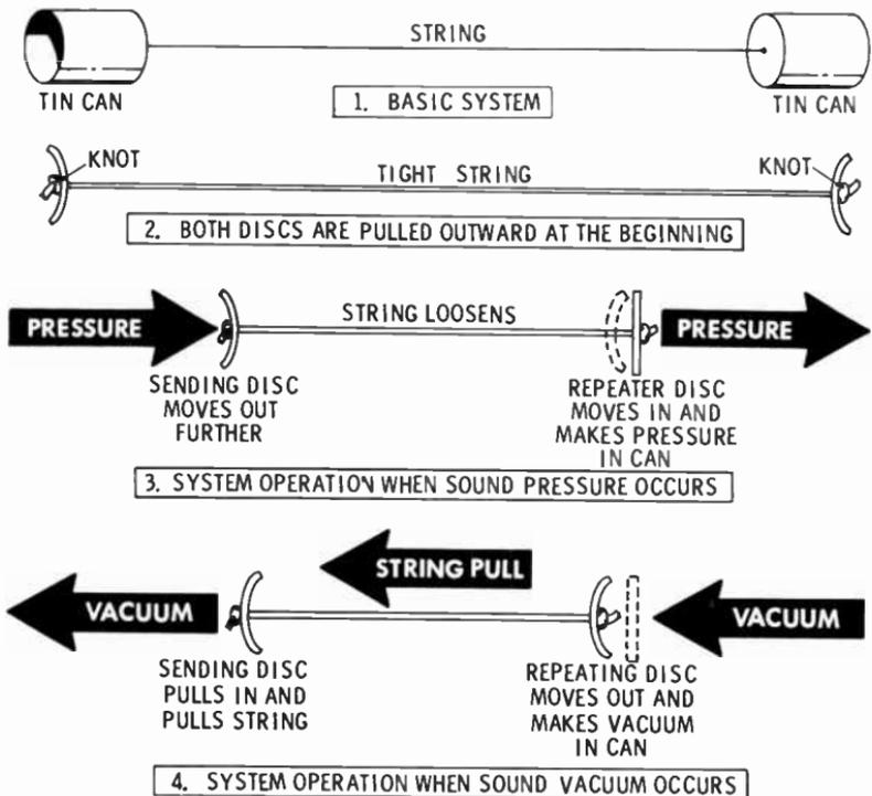
Note that the key part of the mechanical telephone system is the flexible metal disc at the bottom of each can. Speaking into the can causes sound waves to strike the disc and make it vibrate.
