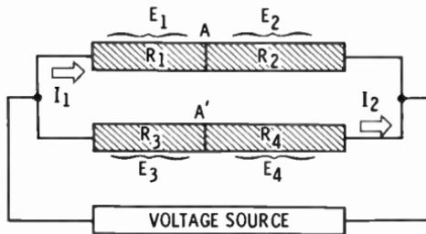
The voltage across a parallel network is the same for either leg. You can state that  $E_1 = E_3$  and  $E_2 = E_4$  in the figure above if A and A' are at the same potential. These voltage relationships can be stated in terms of equal ratios:
