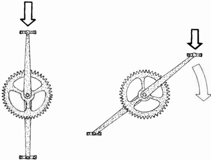
It is necessary then to find some means of giving the single-phase AC motor a means of starting the rotor into motion. Once the rotor is spinning at a reasonable rpm, its inertia will carry it through the dead-center position so that it will be kept rotating by the stationary field. An auxiliary starting system is required. The starting methods make up the primary differences between induction-motor types.
