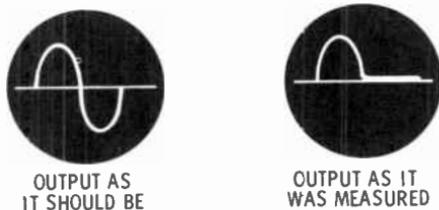
Comparing the output waveform actually measured against that of the proper waveform often provides clues as to the location and/or cause of the trouble. The above illustration, for example, shows the good and bad outputs of an amplifier. From your knowledge of how an amplifier circuit works, the trouble seems to be in the grid or cathode sections. Thus, examine that portion of the circuit.
