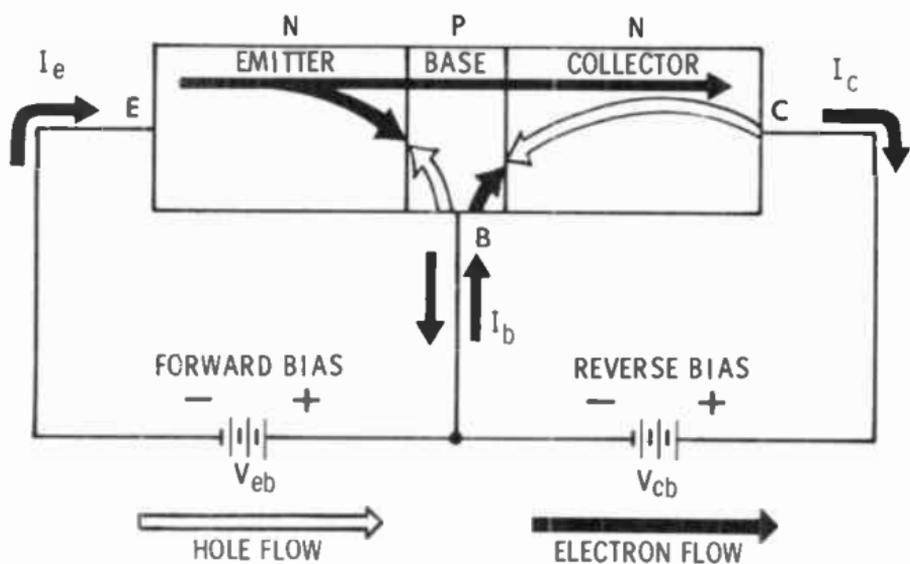
of  $V_{cb}$  and  $V_{eb}$ . The major portion of  $I_c$  is due to the electron flow from emitter to collector. Notice that current flow in the base is due to both electron and hole flow. Thus there are current flows indicated in both directions.  $I_b$  is the difference between these two currents.
