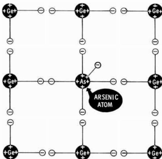
electrons in its outer ring. Therefore it can combine with four electrons from an adjacent germanium atom. When
