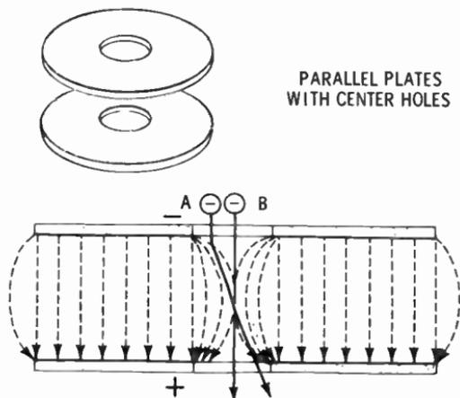
Since its path is parallel to the force lines, electron B will pass straight through the axis (center line) of the holes. Electron A starts in the same direction as electron B. When electron A enters the field, it turns in the direction of the force lines. Just before it leaves the field, it is turned even further and in the direction of the curvature of the force lines.
