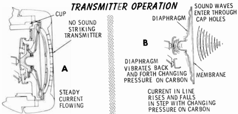
When the handset is lifted from its cradle, a steady current from the phone system starts to flow through the carbon granules. Sound striking the diaphragm places a varying pressure on the carbon. When the granules are packed tightly, current in the circuit increases. When the diaphragm releases its pressure, the granules become loose and less current flows.
