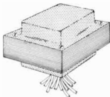
these windings (3 and 4) provides 150 volts AC, and the other (9, 10, and 11) provides 200 volts AC with a center tap. The use of this center tap will be explained later.
