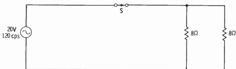
The formula for the equivalent resistance of two **equal** resistors in parallel is:
