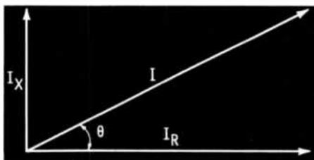
The overall current is the vector sum of the reactive current and the resistive current. This overall current leads or lags the applied voltage by an angle  $\theta$ .
