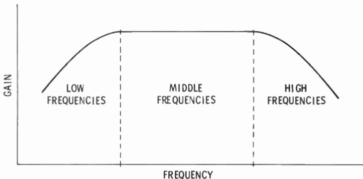
**Q28. What factors affect the gain of an RC-coupled amplifier at different frequencies?**
