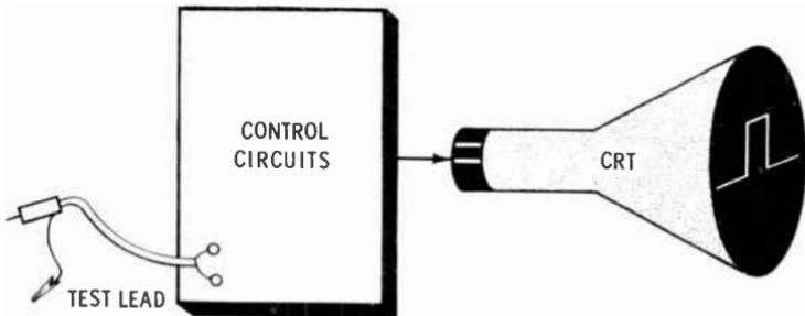
A typical oscilloscope will be described in terms of how the cathode-ray tube and the control circuits function. The test leads are only slightly different from those with which you are already familiar. Since the control circuits are designed to operate the CRT, the cathode-ray tube will be studied first.
