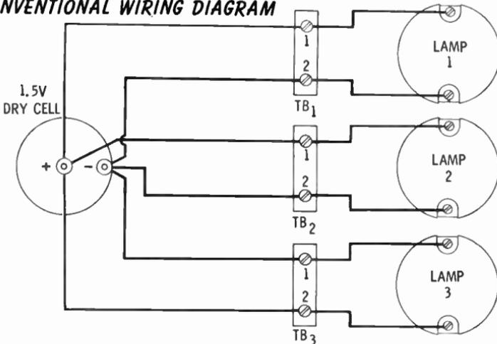
**The Highway Wiring Diagram**—Even with three lamps, the diagram is cluttered, and the lines are difficult to follow. A **highway wiring diagram** (it looks like a highway with secondary roads leading from it) removes the clutter. The same three lamps are redrawn below. Each wire entering the “highway” has its destination marked.
