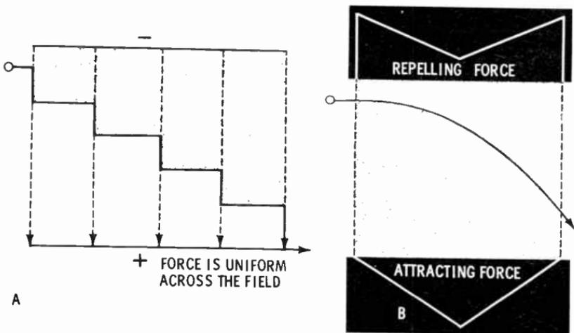
line? If this were true, an electron traveling between the plates with sufficient velocity to pass through the field would cover the distance in a stair-step pattern, as in A above. It is known that the path of an electron through a force field is curved, as in figure B. Force does not exist in distinct beams; it is continuous and uniform across the field. However, it is easier to talk about the field in terms of imaginary lines.
