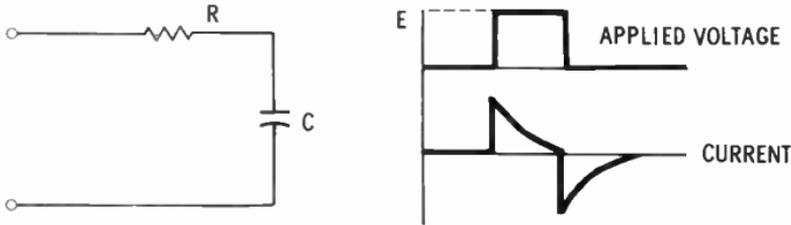
change of voltage and will gradually **charge** to source voltage  $E$ . The rate of charge (the initial current that will flow) is limited by resistance  $R$ . In fact, the initial current will be  $I = E/R$  and will gradually decrease to zero as the voltage **builds up** across the capacitor.
