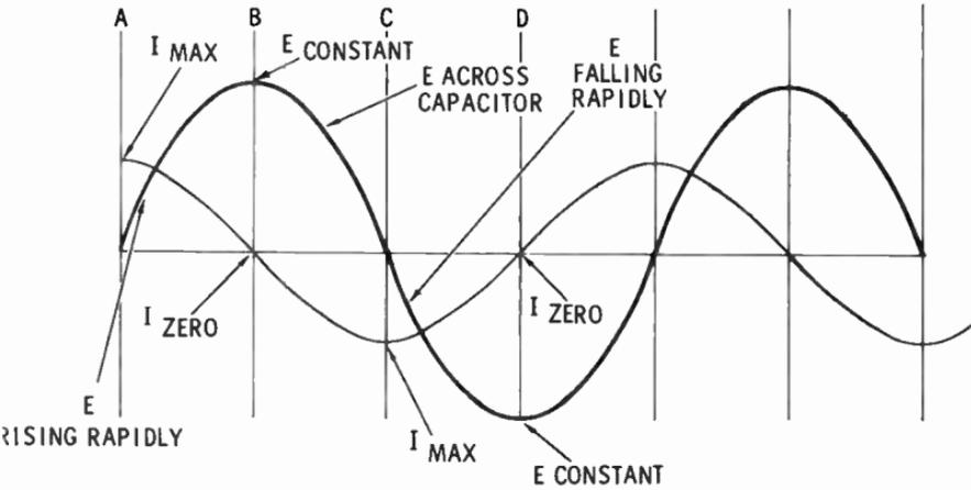
Current and voltage vectors in a capacitive circuit are  $90^\circ$  out of phase. In this case the current vector is **ahead** of the voltage vector by  $90^\circ$ .
