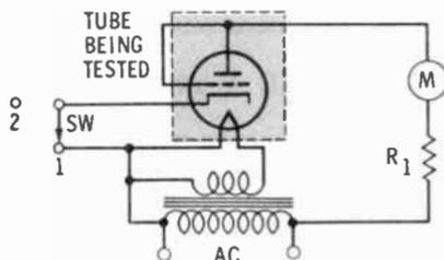
and heater, the meter pointer will drop to zero. If there is leakage, the meter pointer will drop, but not to zero.
