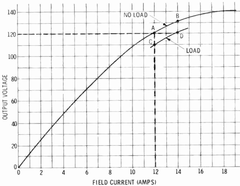
You can see that whenever a load is applied to an alternator, an increased field current should be applied in order to make up for the drop in output voltage. During the course of one day the load varies considerably. Such field-current changes must therefore be made automatically. A device for regulating the output voltage of a generator is called a **voltage regulator**.
