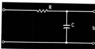
In the above circuit, the length of time it will take for the capacitor voltage to rise to some given value can be calculated. If some device, which will be triggered only when this given value of voltage is reached, is connected across the output terminals  $b$ , the device, such as a gas diode, will be triggered after a predictable time delay from the time the input voltage ( $E$ ) is applied.
