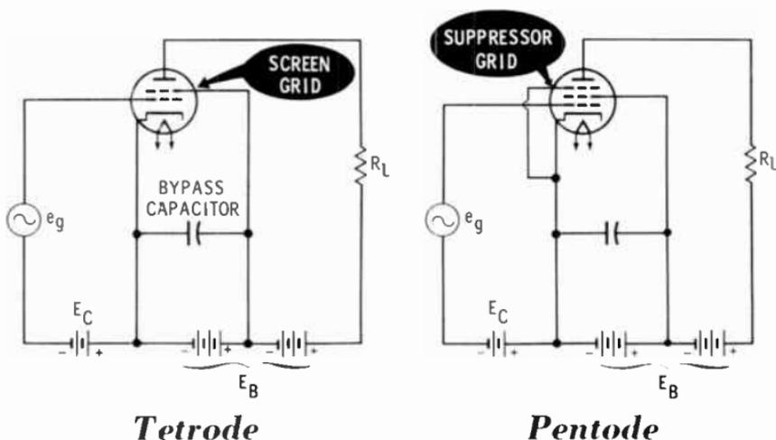
The suppressor grid prevents this current from flowing. It is electrically connected to the cathode, making it negative with respect to the plate, and thus repels any electrons that try to travel from the plate to the screen grid. The suppressor grid is actually a fairly coarse screen so that it does not interfere with the main current flow between cathode and plate.
