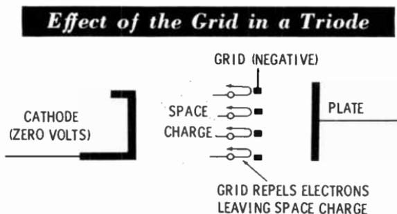
The direction of this field is determined by the polarity of the voltage applied to the grid. For reasons which will become evident later, the grid is operated with a small negative voltage (relative to the cathode) applied to it. The effect of this voltage is to repel electrons which would otherwise leave the space charge and flow to the plate.
