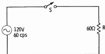
In any AC circuit the voltage shown at the generator is the rms voltage. The frequency shown is in cps (cycles per second), and the resistance is in ohms.
