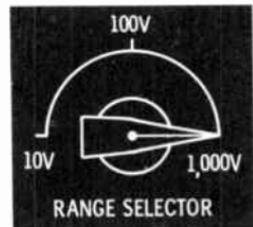
selector is set on 100V, the scale readings are multiplied by 10 to obtain the measured value. If 10 volts were the measured value, the pointer would show a full-scale reading if the meter were on the 10V range. On the 100V range the pointer would come to rest over the 1 mark—10 times 1 equals 10 volts.
