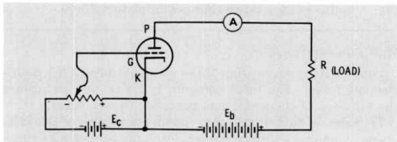
Battery  $E_b$  is connected in such a way that the plate is positive with respect to the cathode. In an actual circuit the positive voltage for the plate is normally obtained from a power supply. Battery  $E_c$  places a negative voltage on the grid with respect to the cathode. A resistor takes the place of this battery in an actual circuit.
