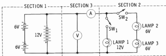
As you recall, an ammeter is always connected in the circuit path. Therefore, the ammeter in the above illustration is placed in series with the source and the load. A voltmeter is always placed across (in parallel with) the load or source.
