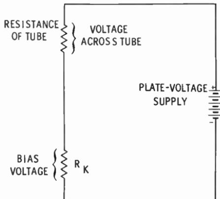
resistor and the DC plate resistance of the tube. The plate voltage as seen by the tube is only that part of the supply voltage appearing across the plate resistance. Therefore, the plate-voltage supply must provide the bias voltage in addition to the plate voltage.
