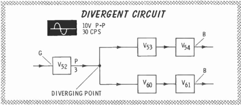
The illustration shows that the input to the divergent circuit ( $V_{52}$ ) is good and that the output should be a 30-cps sine wave at 10 volts peak-to-peak. If the B indicates no output at either point, the first test should be made at the output (pin 3) of  $V_{52}$ . If there is no output at this point, enclose  $V_{52}$  with a G and a B, and Step 4 is concluded.
