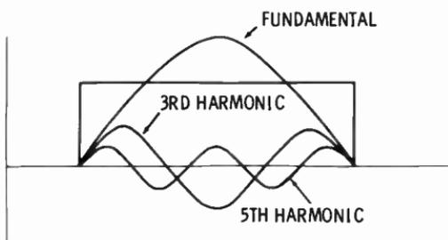
The lowest frequency contained in a train of rectangular pulses is called the fundamental frequency. This frequency has a period equal to that of the square wave. All the other
