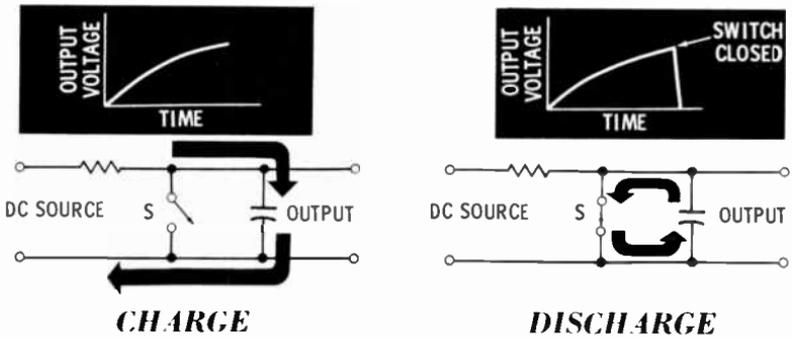
Most sawtooth generators use RC circuits. You have learned that a capacitor takes a certain amount of time to charge through a resistor. This time is determined by the RC time constant of the particular combination. If a capacitor is charged until the voltage across it reaches a given
