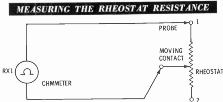
If the rheostat contact is at terminal 1 and the meter has been properly zeroed, the resistance reading should be zero ohms. Leaving the probes connected, the meter will show the gradual increase of resistance as the contact is moved toward terminal 2. At terminal 2 the total resistance of the rheostat will be read on the meter scale.
