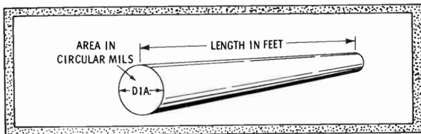
A **circular mil** is used as a unit instead of square inches to measure cross-sectional area of a wire. Circular mils can be determined by squaring the diameter (in mils) of a wire. A mil is 0.001 of an inch.
