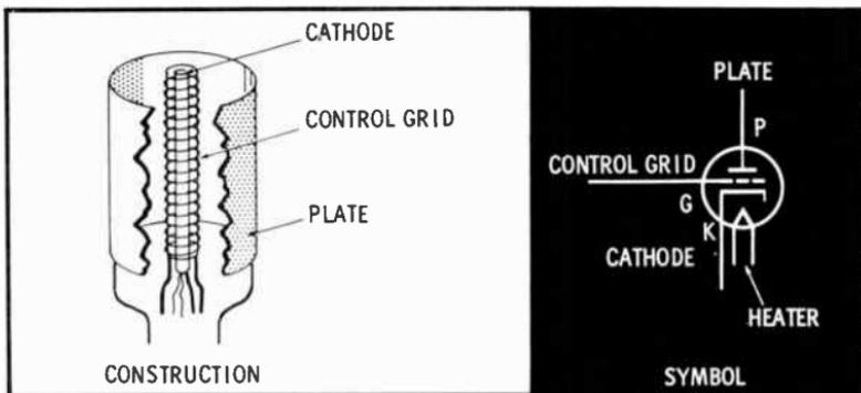
**Operation**—Plate current in a diode is determined by cathode temperature and plate voltage. In a triode, the voltage of the grid with respect to the cathode also controls the amount of plate current.
