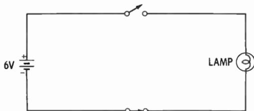
**A20.** Current will **not** flow in this circuit. The open switch breaks the path through which current would flow.
