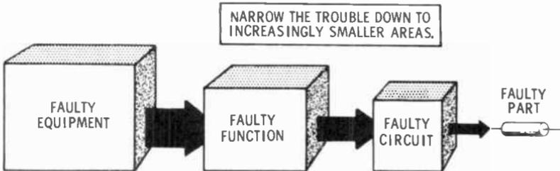
Five steps are listed below as the most reliable method of learning and applying this procedure. They can be applied to any equipment, regardless of size. The steps in the proper order are:
