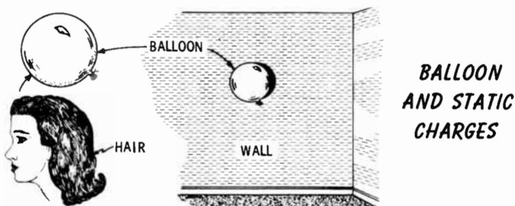
Now place the balloon near a wall. The balloon clings to the wall because of the negative static charge it accumulated.
