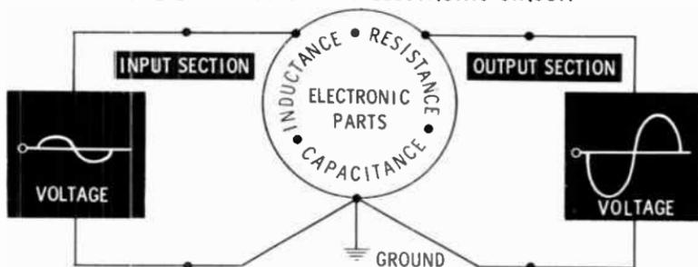
You might think that the symbol for a vacuum tube or transistor does not look like an inductance, capacitance, or resistance. You are correct. However, the way a vacuum tube or a transistor operates can be explained by how it reacts in terms of resistance, inductance, or capacitance when current is passing through it or when voltage is applied to it.
