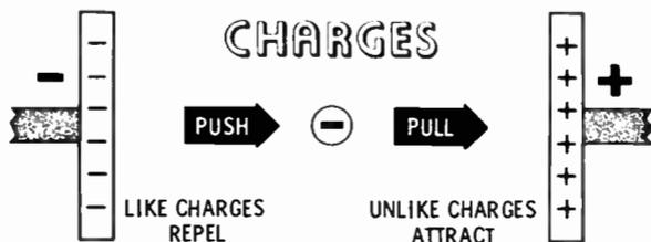
A negatively charged body placed near a positively charged body produces a force of attraction between them. One body tries to contact the other in an attempt to neutralize, or balance, the charges. You can try a simple experiment to demonstrate this principle. Inflate a rubber balloon and rub it on your hair. (Make certain your hair is dry and clean.)
