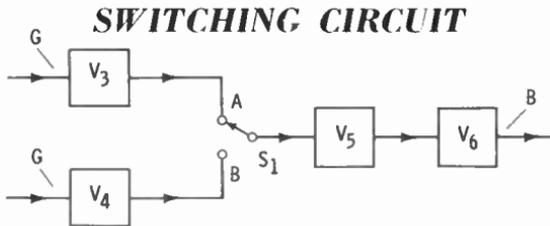
With switch  $S_1$  in position A, Step-3 tests reveal good inputs to  $V_3$  and  $V_4$  but a bad output from  $V_6$ . The first test to make in Step 4 is a reading at the output of  $V_6$  with  $S_1$  in position B. If the reading is what it should be,  $V_5$  and  $V_6$  are good and the B can be moved to the output of  $V_3$ .
