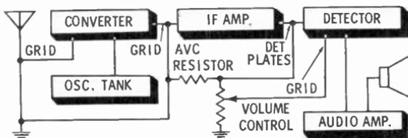
Q25. Among the many carrier frequencies that appear on the antenna, how does a superhet select a single frequency?
