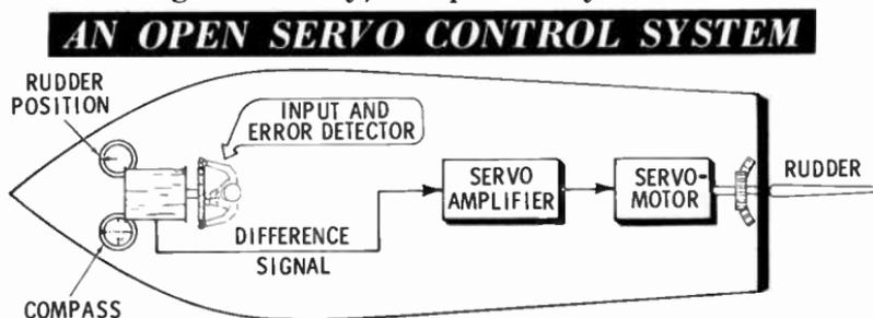
In this case, the man at the wheel is the input and error detector. He moves the wheel to maintain the ship on a specified course. He does this by watching the direction on a compass. When wind or ocean currents move the ship off
