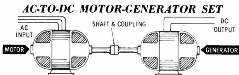
It is customary to use three-phase motors of either the induction or synchronous type. The induction motor has the advantage of being lower priced and more rugged in construction than the synchronous motor. The induction motor can be wound for voltages as high as 13,500 volts, thus eliminating the need for step-down transformers in many cases.
