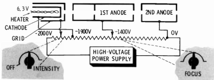
required, the other electron-gun elements are operated at negative potentials. The control grid normally operates near 2,000V negative, 90 to 100V more negative than the cathode. The first anode (focusing) can be maintained between -1,200 and -1,600V. These voltages are typical but vary among instruments.
