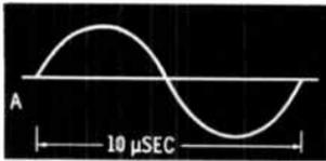
$$\text{FREQUENCY} \left\{ \begin{aligned} &= \frac{1 \text{ SECOND}}{10 \text{ MILLI SECONDS/CYCLE}} \\ &= \frac{1000 \text{ MILLI SECONDS}}{10 \text{ MILLI SECONDS/ CYCLE}} \\ &= 100 \text{ CYCLES PER SECOND} \end{aligned} \right.$$
