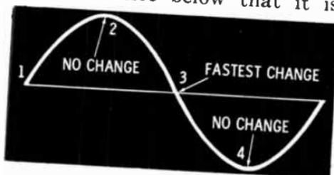
changing faster at the points where the sine wave crosses the zero line. It is not changing at all at the instant of each positive and negative peak.
