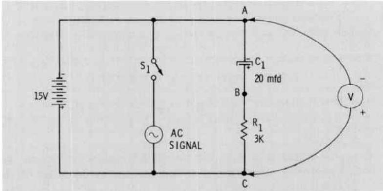
To develop a voltage across  $R_1$ , current must flow through it. At the instant the circuit is connected, current flows from the lower plate of the capacitor through  $R_1$  and the battery to the upper plate. In  $5 RC$  times, the capacitor is fully charged and current stops flowing.
