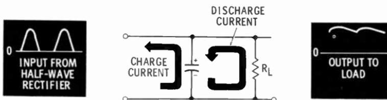
In practice, there is always a load resistance connected across the capacitor. Between peaks, the capacitor discharges through the load resistance, and the voltage gradually decreases. The amount the voltage decreases before the capacitor is charged again by a peak in the pulsating DC is called **ripple voltage**.
