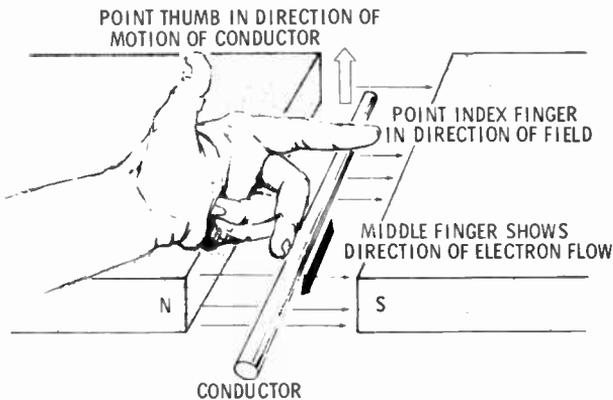
The left-hand rule for generators is shown above. This is an easy way of remembering the relationship between the direction of the magnetic field, the direction of motion of the conductor, and the direction of the induced current.
