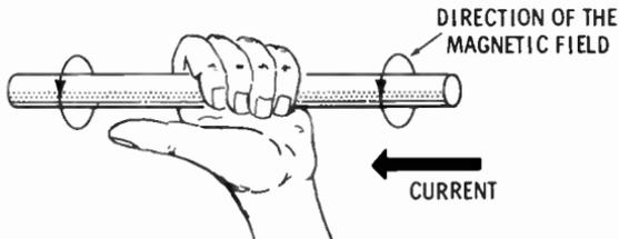
Do not attempt such an experiment on a bare wire. Instead, place your left hand in a position away from the wire with your thumb pointing in the direction of current flow. Your curled fingers will indicate the direction of the magnetic field. It isn't necessary to grasp the conductor.
