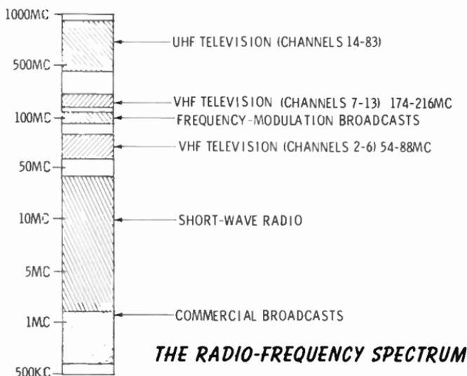
Commercial transmitters (radio and television, for example) are assigned a transmitting frequency in the appropriate part of the radio-frequency spectrum. Transmitters broadcasting in the home radio band, 535 kc to 1,605 kc (kilocycles), are required by law to be on their assigned frequency within plus or minus 20 cycles per second.
