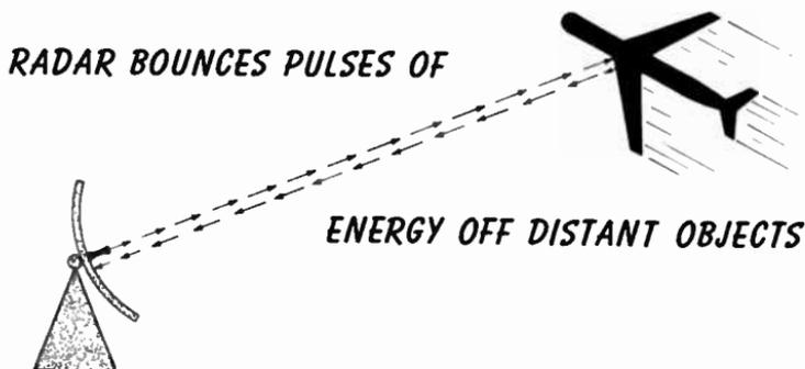
A radar set sends a pulse of energy into space. This pulse travels at the speed of light. The pulse hits an object (an airplane, for instance) and is reflected back to the set. By measuring the time it takes for this signal to travel to the object and return, the distance between the set and the object can be calculated.
