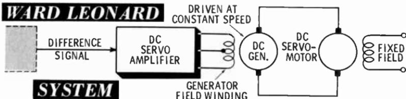
The field winding of the DC generator is in the output circuit of a vacuum-tube amplifier. The output of the generator is controlled by the strength of its magnetic field. The value of current through the field will be determined by the size of the amplified difference signal. A large difference signal will cause the servomotor to attain high speed; a smaller signal a lower speed.
