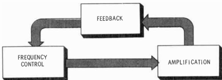
**Amplification**—An amplifier with plate current flowing will normally amplify any spurious signals appearing at the grid. A spurious signal is any unwanted signal generated either in the equipment itself or externally.
