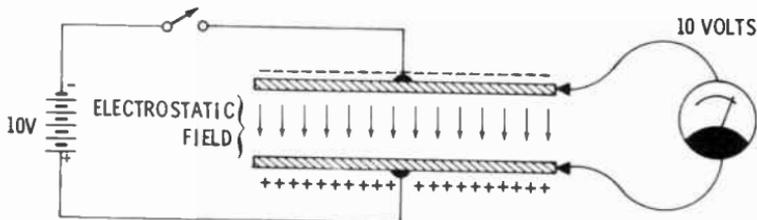
The voltage across the capacitor is still 10 volts, just as it was before the switch was opened. The excess electrons remain where they are because there is no path for them to return to the positive plate (assuming the voltmeter has no internal resistance through which electrons can travel).
