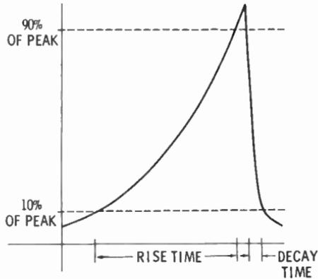
Like AC sine waves, pulses have an rms value. Unfortunately, there is no simple formula to find the rms value of a pulse. The rms value of a pulse is its working value.
