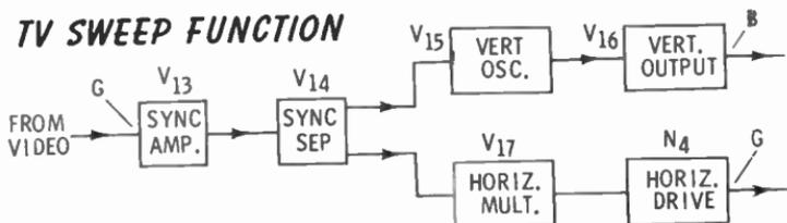
The vertical and horizontal channels generate waveforms of the proper frequency, shape, and amplitude to cause the electron beam in the CRT to sweep the required horizontal lines on the screen. Oscillations continue whether sync pulses are received or not. This is the reason for the raster appearing on the screen when a station is not tuned in.
