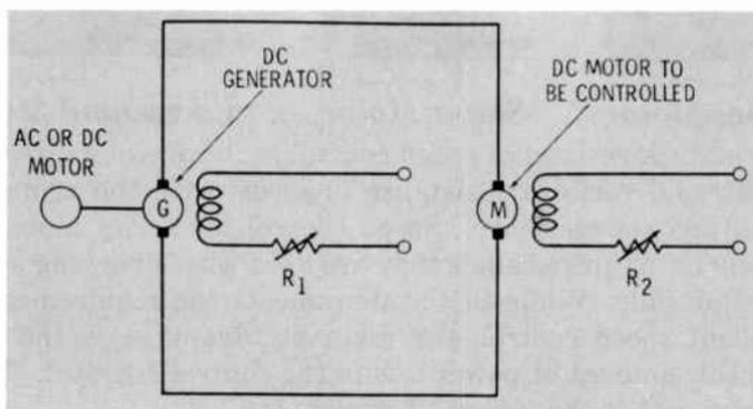
The shunt fields of both the generator and motor are supplied from a constant-voltage source. The DC-generator output voltage is controlled by rheostat  $R_1$ . The voltage variation (out of G and into M) gives a wide range of speed control. In addition, by varying the motor rheostat ( $R_2$ ), a wider speed range can be obtained.
