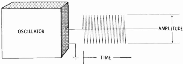
Signal generators are classified in accordance with the frequency range of their oscillators. Audio-frequency (AF) generators usually cover a range from about 20 to 20,000 cps. Radio frequency (RF) generators begin at 20,000 cps and end at several thousand megacycles.
