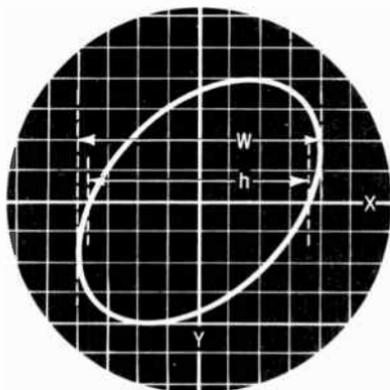
The graticule is placed on the CRT, and the Lissajous figure is centered. The overall height and width of the ellipse should be equal in length. The distances  $h$  and  $W$  are shown in the figure above. The ratio  $h/W$  is the sine of the angular phase difference. For example, if  $h$  were equal to 7 units and  $W$  equal to 8, then:
