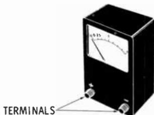
**Terminals** — The voltmeter, like other electrical devices, has two terminals. Both terminals are connected into a circuit when using the instrument. The terminals are sometimes colored red (+) and black (—) to identify the positive (+) and negative (—) connections.
