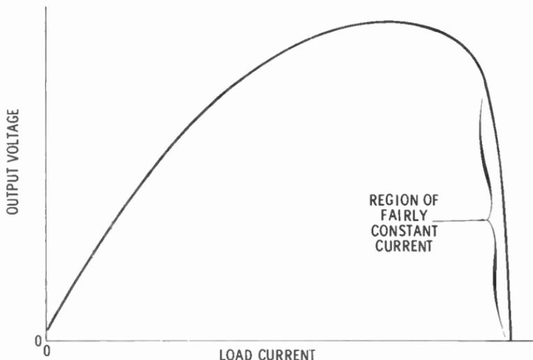
As more current is demanded (within practical limits) from a series-wound DC generator, the output voltage increases. When the practical limit of current is reached, a further demand has a reverse effect. The practical limit is reached when the magnetic field strength reaches its maximum value.
