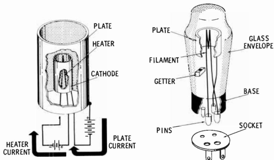
**Indirectly Heated Cathode      Directly Heated Cathode**
