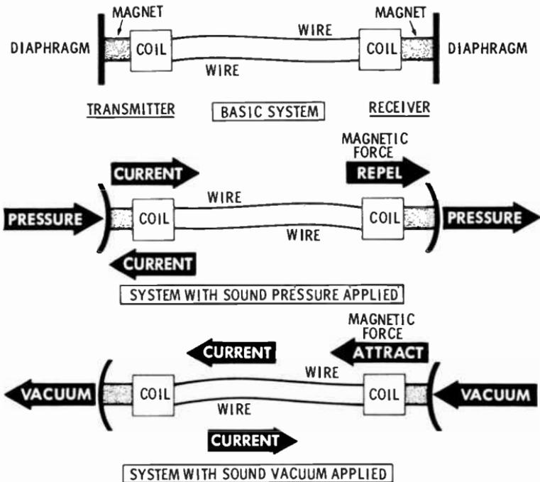
ing magnetic field. The bar magnet responds by moving back and forth at the same frequency as the current, causing the diaphragm to reproduce the original sound.
