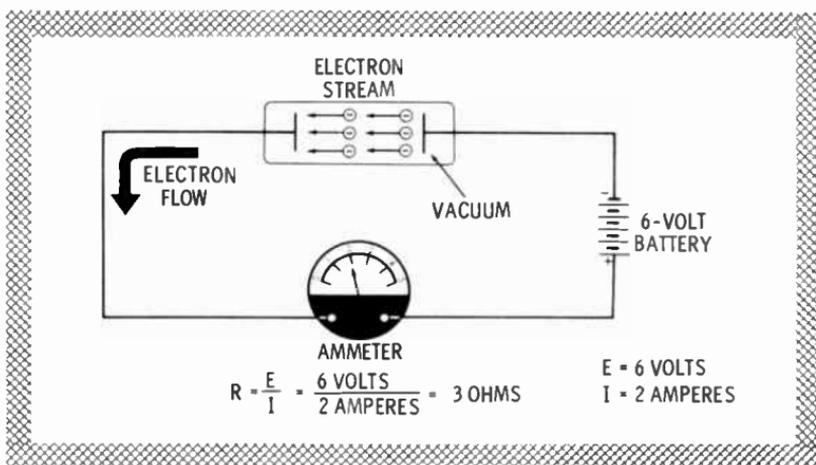
One terminal of a 6-volt battery is connected to one of the plates, and the other terminal is connected to the other plate through an ammeter. An electron stream flows through the
