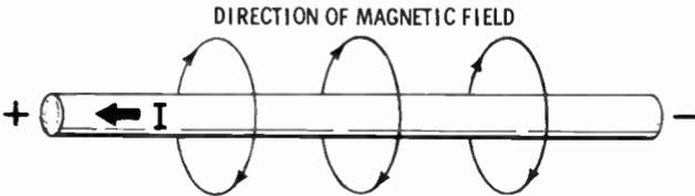
THE DIRECTION OF THE MAGNETIC FIELD IS DETERMINED BY USING THE LEFT HAND RULE
