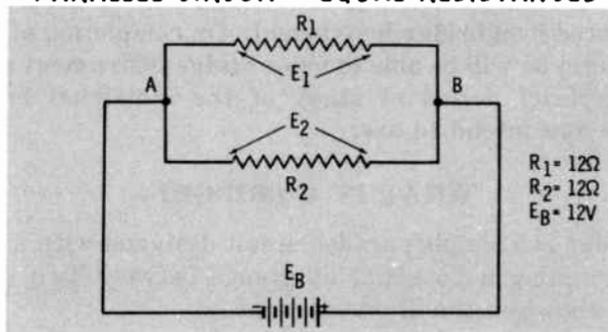
Disregarding the voltage drop in the conductors, the voltage difference between points A and B (above) will be that of the source (12V). The current through  $R_1$  and  $R_2$  will be 1 amp each, or a total circuit current of 2 amps. Since the resistances and currents in both legs are equal,  $E_1$  is equal to  $E_2$ . Now divide one resistance into four equal parts.
