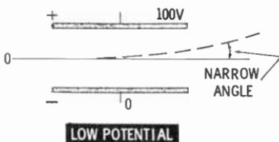
**Beam Acceleration**—The faster the electrons are moving, the smaller their deflection angle will be.
