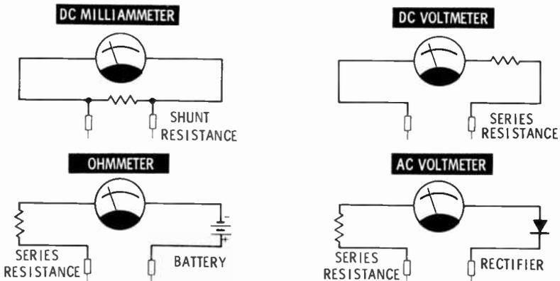
**Meter-Circuit Components**—The figure on the opposite page shows that multimeter circuitry requires series and/or shunt resistances, a battery for measuring ohms, and a diode for limiting current direction when measuring AC voltage. To obtain different ranges for volts, amps, or ohms, resistances of selected values must be used in the circuit. The circuits are connected to front-panel controls that provide means of selecting the desired function and range.
