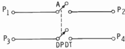
The dashed line indicates that the two poles of the switch are actuated at the same time.
