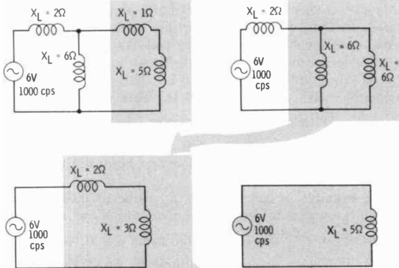
**Q6. What is the equivalent  $X_L$  in the following circuit?**
