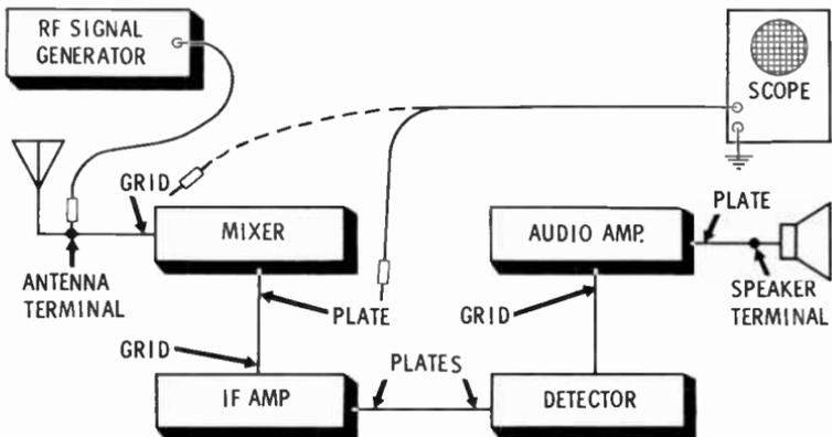
An oscilloscope is best for signal tracing. You can use a VTVM, however, to check for the presence of a signal. You must use an RF probe with the meter when testing at points where either RF or IF signals are present.
