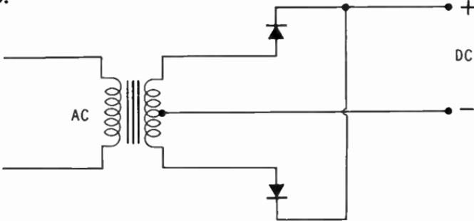
**A14.** Rectifiers have a **high resistance to current flow in one direction** and a **low resistance in the other direction.**
