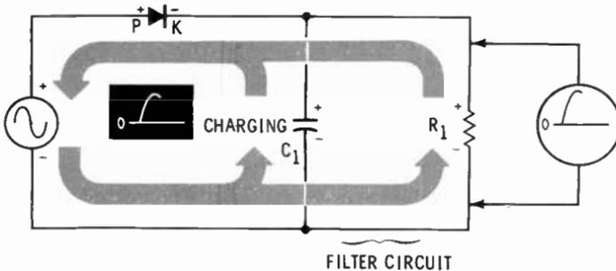
As the source voltage rises to maximum positive, current flows through  $R_1$  and the diode. Some of the current also charges the capacitor to the value of the source voltage.
