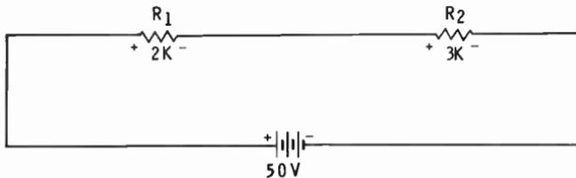
A54. Voltage across  $R_1$  is 20 volts.
