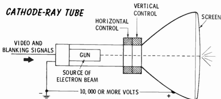
The basic construction and connections of a CRT are illustrated above. At the left end is shown an electron gun which shoots a narrow stream of electrons toward the screen. To speed the electrons on their way, the inner surface of the flared portion of the tube has a conductive coating energized with a voltage that is several thousand volts positive with respect to the electron source.
