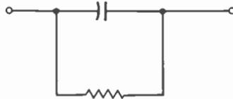
from one plate to the other. Leakage is considered to be a resistance in parallel with the capacitor.
