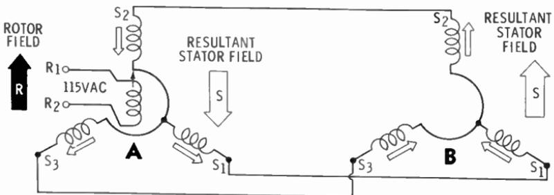
In synchro A, the direction of the developed rotor field is up, as shown. The induced magnetic fields in the individual stators are along their axis but in a downward direction. The combination of all the stator fields produces the resultant field shown by the large white arrow. It is an induced field and is directly opposite to the rotor field.
