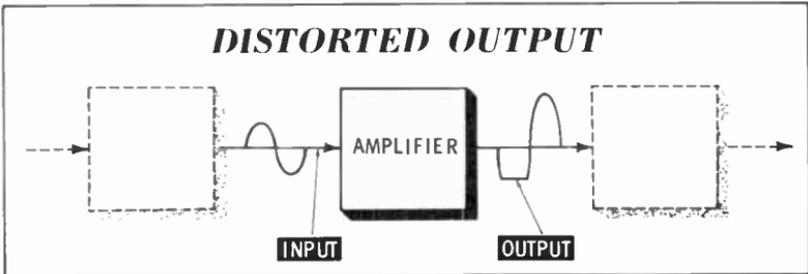
In the figure above, the leading half of the cycle in the output has been distorted. You would, therefore, suspect that the amplifier had gone into saturation and was clipping off that portion of the wave. You could also reasonably conclude that the most probable cause of the trouble was a change in tube bias.
