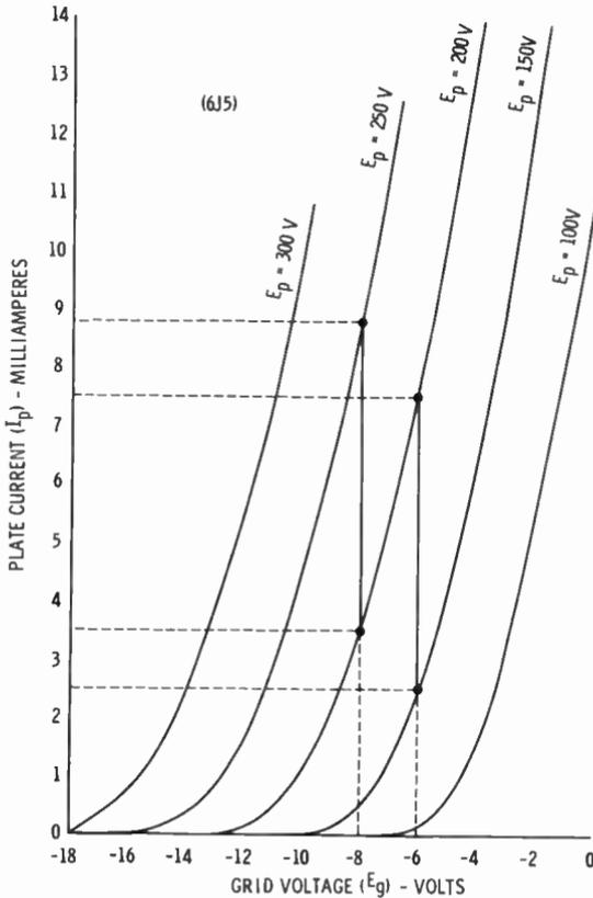
Note that these values (9,280, 10,000, and 9,090 ohms) are all fairly close to each other. When compared to the changes in  $R_p$  (from thousands of ohms to hundreds of thousands of ohms), the AC plate resistance ( $r_p$ ) may be considered almost a constant for a particular triode.
