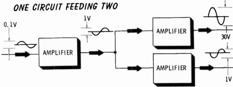
A low-amplitude sine wave is amplified by the first amplifier and fed to two others. Their outputs are quite different.
