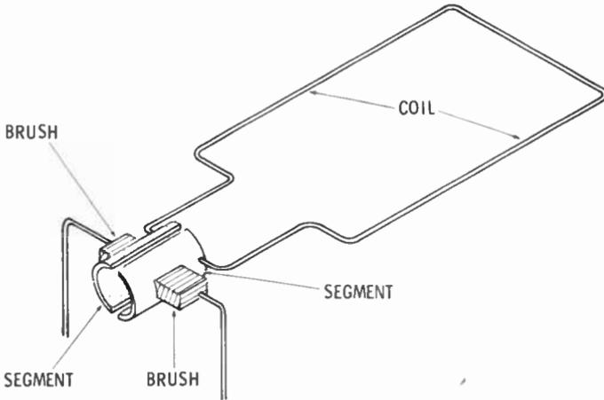
of the coil is connected to the other segment. Two brushes touch opposite sides of the commutator. As the commutator turns, the two sides of the coil are short-circuited for a moment as the brushes touch both segments of the commutator at once. Then the connections are reversed.
