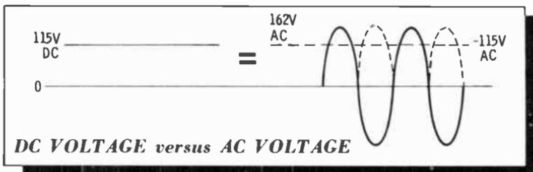
The peaks of 115 volts AC are actually 162 volts. A capacitor with a 150-volt rating will work well on 115 volts DC but not 115 volts AC. Standard practice is to use a capacitor with a working voltage about 50% higher than any voltage expected in the circuit.
