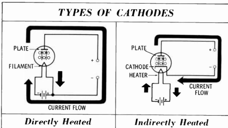
emitted by the thorium are replaced by the tungsten. The figure shows how the filament battery sends current through the filament, heating it and causing it to emit electrons.
