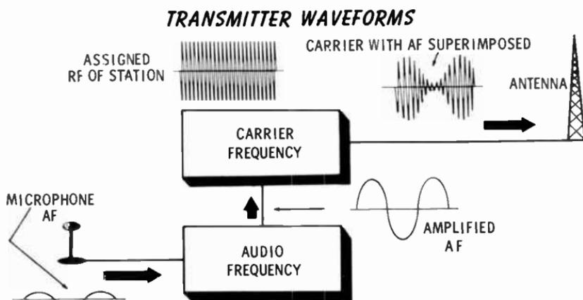
**Superimposing the Sound**—The process of superimposing AF on the carrier, as shown in this particular example, is called **amplitude modulation (AM)**. In amplitude modulation the audio frequency (varying at the changing rate of the original sound) is mixed with the carrier (a constant frequency) in a manner that causes that carrier **amplitude** to vary at the same rate as the audio. The carrier **frequency** remains unchanged.
