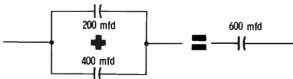
If a 200-mfd and a 400-mfd capacitor are connected in parallel, the equivalent capacitance of the combination is
