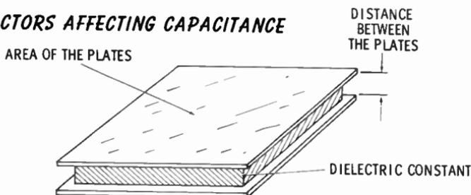
Capacitance (farads) is determined by three factors:
