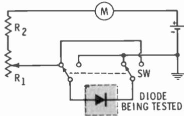
The diode is inserted in the device, and  $R_1$  is used to adjust the meter reading so that the pointer will remain on scale when the switch is thrown. The switch reverses the current direction through the diode.  $R_2$  limits the current to a safe value.
