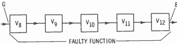
on the diagram show a good input and a bad output. The concept of Step 4 is to isolate the one faulty circuit among the five with the fewest tests.
