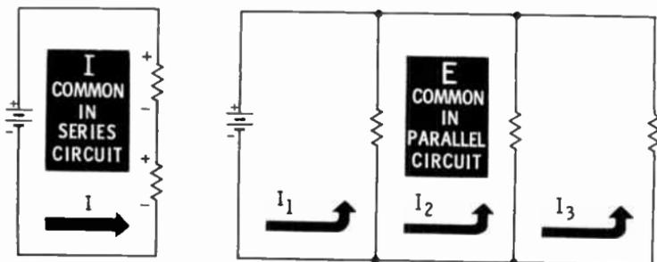
A parallel circuit has a common supply voltage, and thus a possible different current through each resistance (branch), depending on the value of the resistance.
