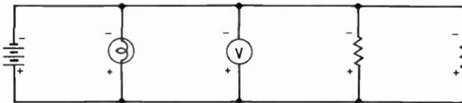
Polarity across each component is determined by circuit tracing. The terminal that current enters is negative.
