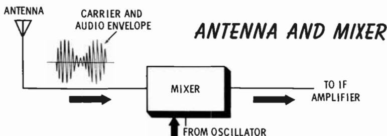
**The Antenna and Mixer**—Carrier frequencies from all stations within range of a receiver appear on the antenna of the receiver. When you turn the dial of your radio to a specific station, you adjust the electronic components of the **mixer** input so that the receiver will accept a particular carrier frequency and reject all others. The received carrier enters the mixer to be amplified. Some radios have, in addition, an **RF amplifier** between the mixer and antenna.
