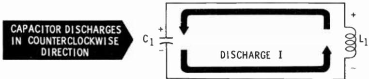
When the source is removed from  $C_1$ , the capacitor will begin to discharge. Current will flow through  $L_1$  in the direction indicated and develop a magnetic field around the turns of  $L_1$ . When the charges on the plates of  $C_1$  have equalized, current would normally stop flowing. However, the magnetic field around  $L_1$  continues to collapse (initial collapse occurred as discharge current decayed), sustaining the current flow.
