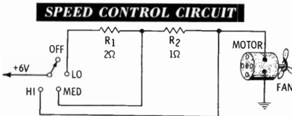
In the LO position the series resistance equals 3 ohms, which permits 1 ampere of current to flow. The 3 ohms is not the only resistance in the circuit. The motor adds its resistance in series with the circuit. In the MED position of the switch, the series resistance is 1 ohm. Again, the motor resistance is in series with it.
