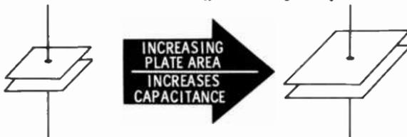
Capacitance can also be increased by placing the plates closer together. When the plates are closer, the attraction
