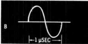
$$\text{FREQUENCY} \left\{ \begin{aligned} &= \frac{1 \text{ SECOND}}{1 \text{ MICROSECOND/CYCLE}} \\ &= \frac{1,000,000 \text{ μSEC}}{1 \text{ μSEC/CYCLE}} \\ &= 1,000,000 \text{ CYCLES PER SEC.} \end{aligned} \right.$$
