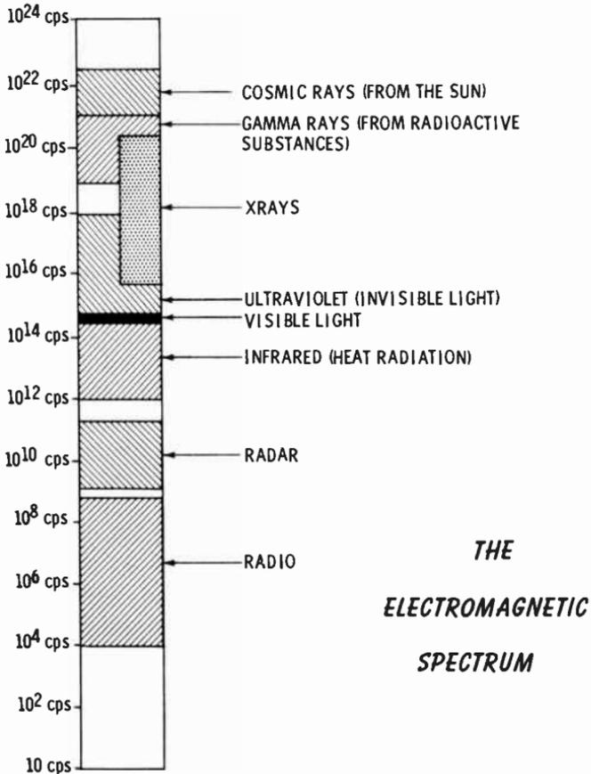
The chart shows that cosmic rays are radiated at a frequency of around  $10^{22}$  cycles per second. (The number  $10^{22}$  is 1 followed by 22 zeroes, or ten-thousand, million, million, million cycles per second.) At the lower end of the radio portion, radiation frequency is under  $10^4$ , or ten thousand cycles per second.
