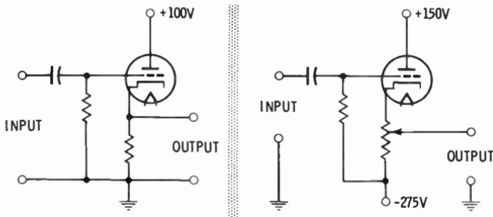
The only true way to determine whether the same triode will operate in either one of these cathode-follower circuits is actual trial in the circuit and observation of its performance. Laboratory models of tube testers approach this capability, but the simpler types do not.
