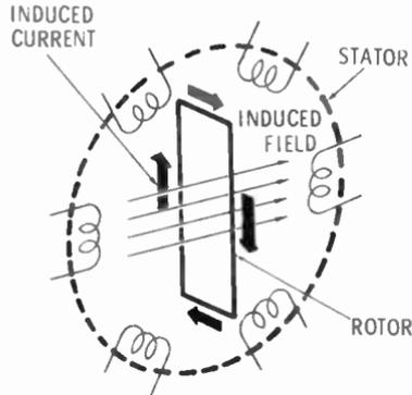
motor). This voltage, in turn, creates a large current in the rotor circuit. The current is large because the only resistance opposing it is the resistance of the wires. This high current in the rotor loop creates a magnetic field of its own. The rotor field and the stator field tend to attract each other. This situation creates a torque which spins the rotor in the same direction as the rotation of the magnetic field produced by the stator.
