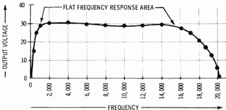
tings for readings in the rising and falling portions of the curve should be made in multiples of 500 cps. Intervals of 2,000 cps are satisfactory along the top part of the curve.
