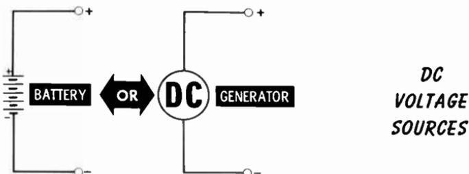
Symbols used for DC voltage sources in schematic diagrams are normally those of a battery or a DC generator.
