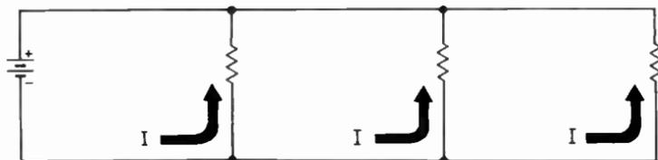
A string of Christmas-tree lamps which will permit one or more lamps in the circuit to be opened and still allow the others to operate properly is one example of a parallel circuit. Each lamp has the same voltage applied.
