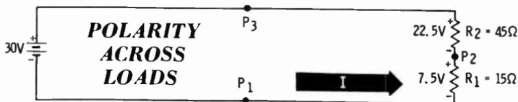
Voltage in a circuit exists only between two points—never at one point only. Therefore, voltage is expressed as being across two points in a circuit, or in terms of one point with respect or in reference to another point. The point at which current enters a resistance is negative with respect to the point at which it leaves.
