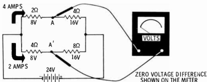
Suppose the 8-ohm resistor in the illustration above is changed to 4 ohms. The resistance ratios are no longer equal. The current in the lower leg is now 3 amps, and the voltage at A' becomes 12V compared to 16V at A. The meter now reads 4V.
