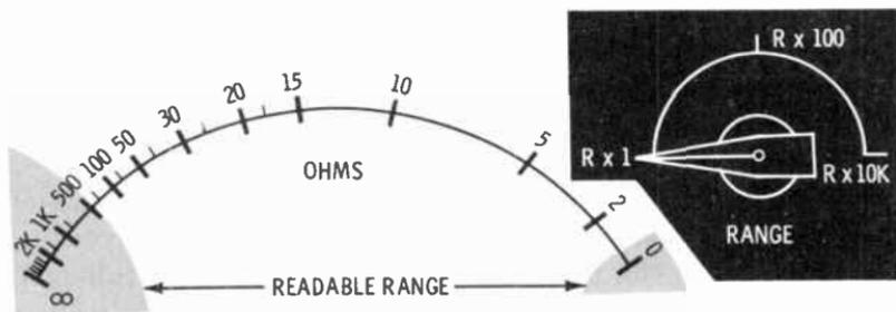
Q25. Using the above diagram, which range setting should be used to measure an estimated  $1,500$  ohms?
