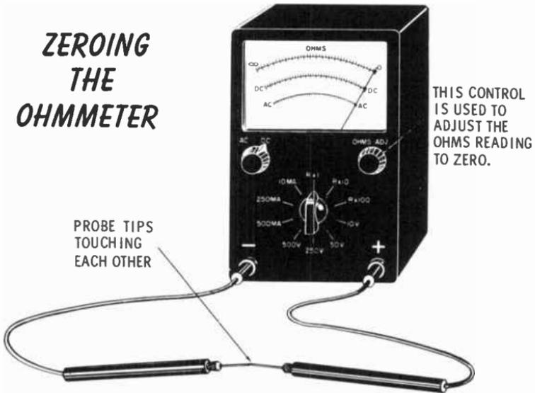
The ohmmeter is now zeroed and a resistance measurement can be made. The pointer should swing back to infinity when the meter is not in use and the probes are not touching each other.
