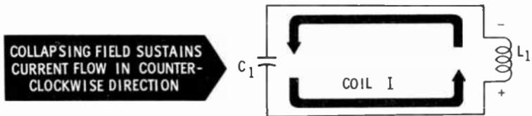
$L_1$  now becomes a voltage source, taking on the polarity shown in the figure above. Collapsing magnetic lines cut the coil turns, producing a current that builds an excess of electrons on the upper plate of  $C_1$ .  $C_1$  is now charged in the opposite direction.
