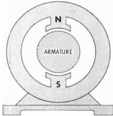
More than one pair of poles are sometimes used in order to produce a stronger magnetic field. When this is done, opposite poles are always next to each other. You can see from the following illustration how this arrangement creates the strongest magnetic field through the armature.
