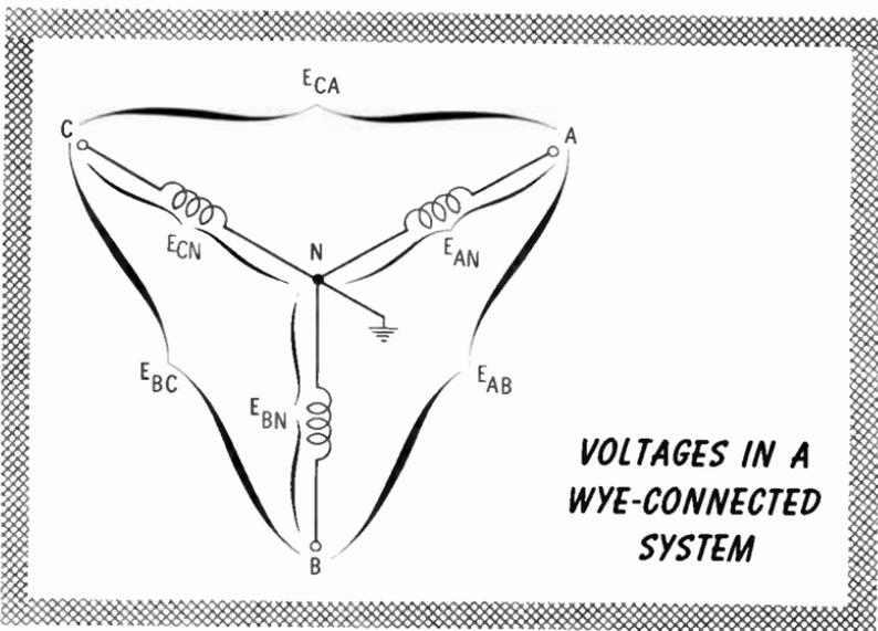
In most cases, the voltages between each phase terminal and the neutral are equal. Thus,  $E_{AN} = E_{BN} = E_{CN}$ . The voltages between any two phases will then also be equal. Thus,  $E_{AB} = E_{BC} = E_{CA}$ .
