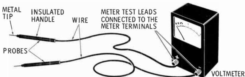
**Connections**—When measuring voltage, the probes are touched to the terminals of the voltage source or device. A voltage measurement is always taken across the terminals, and is never made between a terminal and an open wire.
