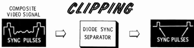
A diode can also eliminate undesired portions of a signal. This is called **limiting**, or **clipping**. In the figure above, another type of TV signal is shown; it is the composite video signal. For certain applications, only the two sync pulses
