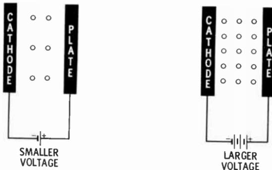
**CURRENT FLOW IS AFFECTED BY PLATE VOLTAGE**
