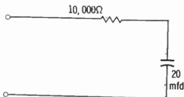
**Q23. How long will it take the circuit above to charge to 63.2 volts if a 100-volt input is continuously applied?**
