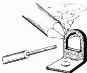
Place an ice pick or soldering aid into the eye of the terminal by following Step 3. This will prevent the opening in the terminal from remaining filled with solder.
