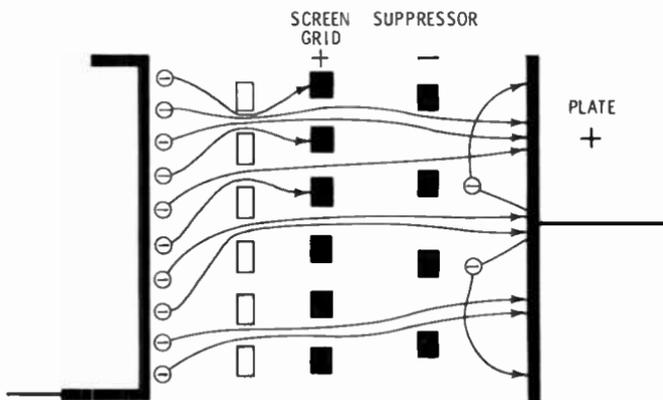
The addition of the suppressor grid between the plate and screen grid also serves to reduce the interelectrode capacitance between the plate and control grid still further. This results in a tube with even better high-frequency performance than the tetrode. Pentode amplification factors are in the order of 1,200 to 1,500 (as opposed to 200 or 300 for a tetrode).
