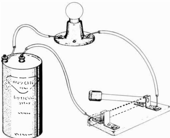
There are many other types of switches, some of which you have used. For example, there are switches on the walls of your home, on the front of your appliances, and on the dashboard of your car. Nearly all operate on the knife-switch principle. In the closed position, a metal blade makes an electrical contact between at least two conductors.
