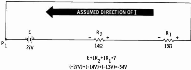
The sum of the voltages in the loop from point 1 back to point 1 equals  $-54V$ . Therefore the current was assumed to be going in the wrong direction.
