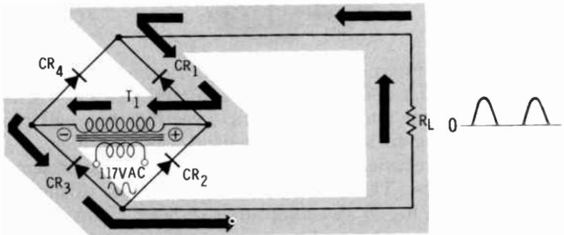
On the positive half cycle, current flows through CR<sub>3</sub>, up through the load resistor, and back through CR<sub>1</sub>. CR<sub>2</sub> and CR<sub>4</sub> are reverse-biased and act like open switches.
