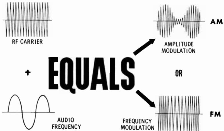
Both AM and FM start out with a carrier frequency and an audio frequency (sound originating in the studio). In amplitude modulation, as you already know, the sound is superimposed on the carrier frequency (which is constant) by varying the carrier **amplitude** in conformance with the voltage and frequency of the audio.
