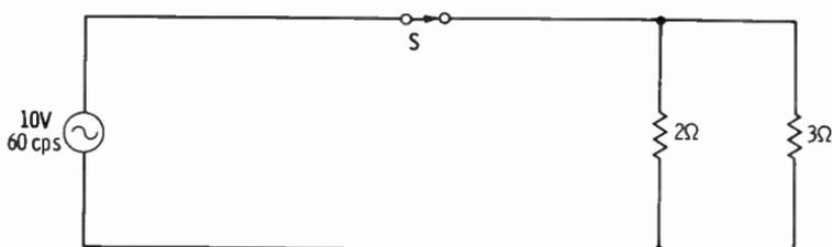
The formula for the equivalent resistance of two resistors in parallel is:
