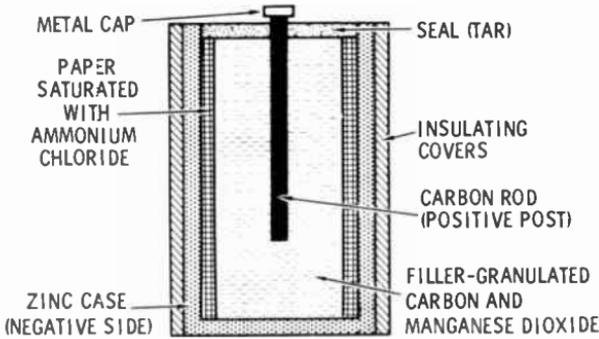
The zinc and the electrolyte are gradually “used up” as the dry cell supplies electricity. A dry cell is called a **primary cell** for this reason. The consumption of material in the cell is a result of chemical action between the zinc and the electrolyte. When the zinc case and the electrolyte have been used for some time, the chemical action which created the ion movement will decrease to a point where the cell is considered run-down (discharged).
