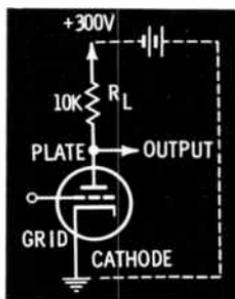
In effect, the grid varies the resistance of the vacuum tube. P<sub>2</sub> is always +300V (to ground). P<sub>1</sub> is a positive
