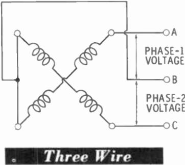
It is also possible, however, to combine two of the output connections to produce what is called the **three-wire system**. In this system the voltages of the two separate phases remain the same. Phase 1 appears between A and B. Phase 2 appears between B and C. But a third voltage is also available, the voltage between A and C. This voltage is the **vector sum** of the other two voltages.
