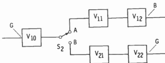
In the diagram above, when  $S_2$  is switched to position B, the conditions indicate that  $V_{10}$ ,  $V_{21}$ , and  $V_{22}$  are good. This leaves  $V_{11}$  and  $V_{12}$  in the circuit group as the only suspects. The quickest way to determine which is bad is by testing between them.
