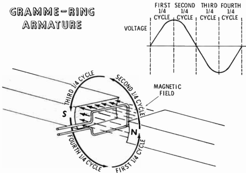
Since the armature windings of the Gramme-ring core are wound on the surface of the core, the distance between the core and the pole pieces must be **great enough** that there is no danger of the armature windings touching the pole
