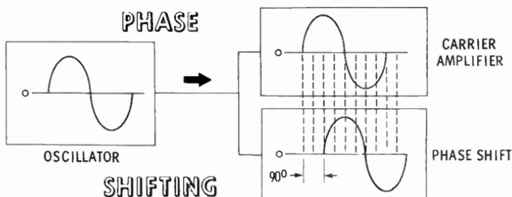
(moved) to the right a quarter of a cycle. This is called **phase shifting**. The starting, maximum positive, return-to-zero, maximum negative, and ending points occur one quarter of a cycle later in the lower block than they do in the upper block. Since there are  $360^\circ$  (one way of designating the period of a sine-wave cycle) in a complete cycle, the lower waveform has been shifted in phase by  $90^\circ$ .
