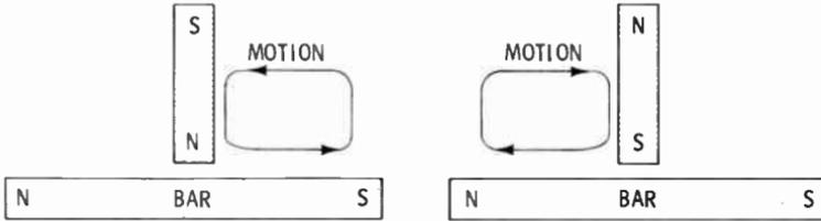
A steel bar can be magnetized in exactly the same way. Steel requires a greater force to align its molecules and therefore takes longer to magnetize. However, steel retains its magnetic properties for a much longer time than iron.
