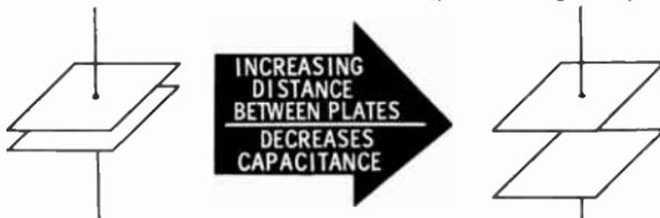
between the negative charges on one side and the positive charges on the other side is greater, and thus more charge can be stored. It is, of course, necessary to keep the plates far enough apart so that the charge does not cross the gap.
