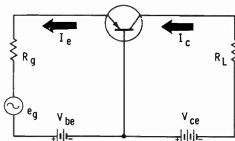
equal to  $\Delta I_e R_i$ . The voltage across the load resistor is  $\Delta I_c R_L$ . The voltage gain in this case is  $\frac{\Delta I_c R_L}{\Delta I_e R_i}$ . Note that  $\frac{\Delta I_c}{\Delta I_b}$  in this case is not  $\alpha$  because the collector voltage does not remain constant.
