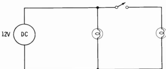
The two lamps are in parallel across the generator. The open switch disconnects the second lamp. With the switch closed, both lamps will light. The dots show the points at which the wires are connected.
