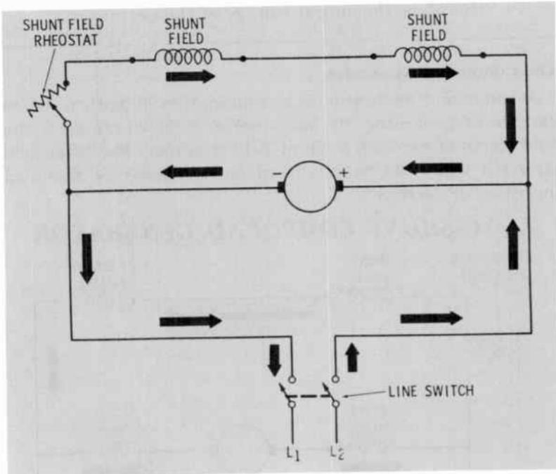
Building up in a self-excited shunt generator does not require that the external load be connected to the generator because the current supplied to the electromagnetic field does not flow through the external load. This means the generator can be started, and the full strength of the magnetic field and the induced emf reached before the external load is connected.
