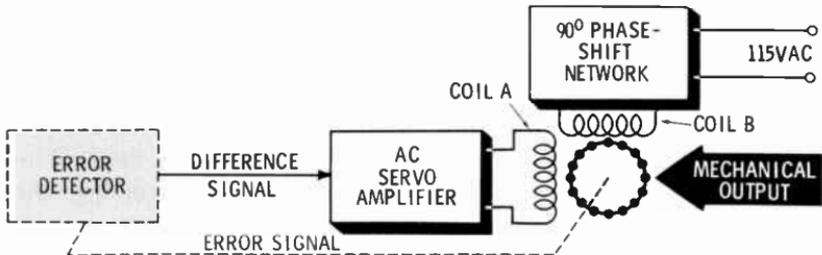
Coil B, the reference winding, is excited from an AC line through a  $90^\circ$  phase-shifting network. Since the same line feeds the rest of the servo system, the difference signal, in phase or  $180^\circ$  out of phase with the line, will either lead or lag the voltage in coil B by  $90^\circ$ . The servo amplifier amplifies the difference signal before it is applied to coil A.
