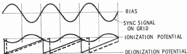
A sync signal on the grid will cause a fall and rise in ionization potential, as shown in the figure above. Without the sync signal, the ionization potential is steady, and the sawtooth waveform is as shown by the dashed line in the figure above. When the sync voltage is added, the sawtooth voltage reaches the ionization potential sooner in each cycle. The rise time of the sawtooth is shortened, and its frequency is increased. This is shown by the solid waveform.
