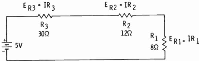
$$I_T = \frac{E}{R_1 + R_2 + R_3} = \frac{5}{50} = 0.1 \text{ amp}$$
