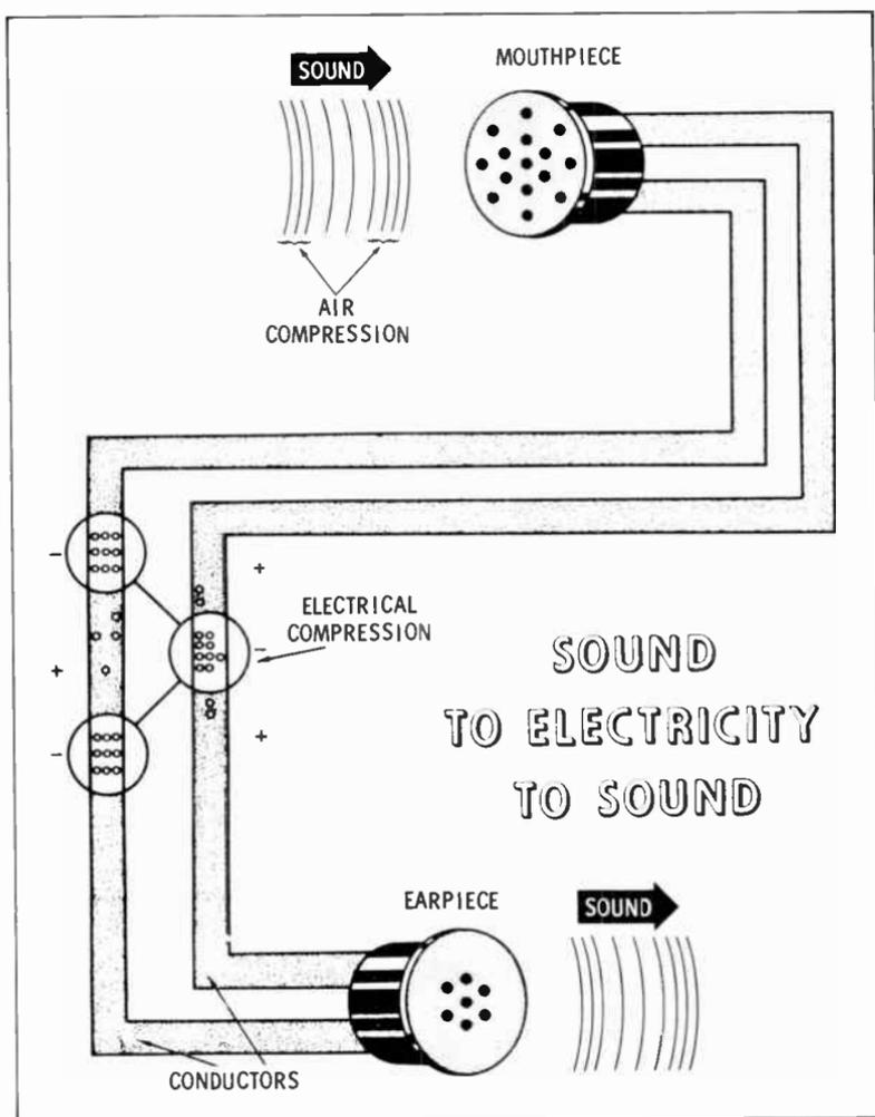
The ability of these crystals to produce a voltage when subjected to mechanical stress is called the **piezoelectric effect**. Conversely, when a voltage is applied to such crystals, a mechanical stress is produced.
