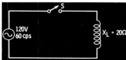
Assume that the resistance in the leads and the coil is negligible. The problem is to find the rms value of the current in this circuit.
