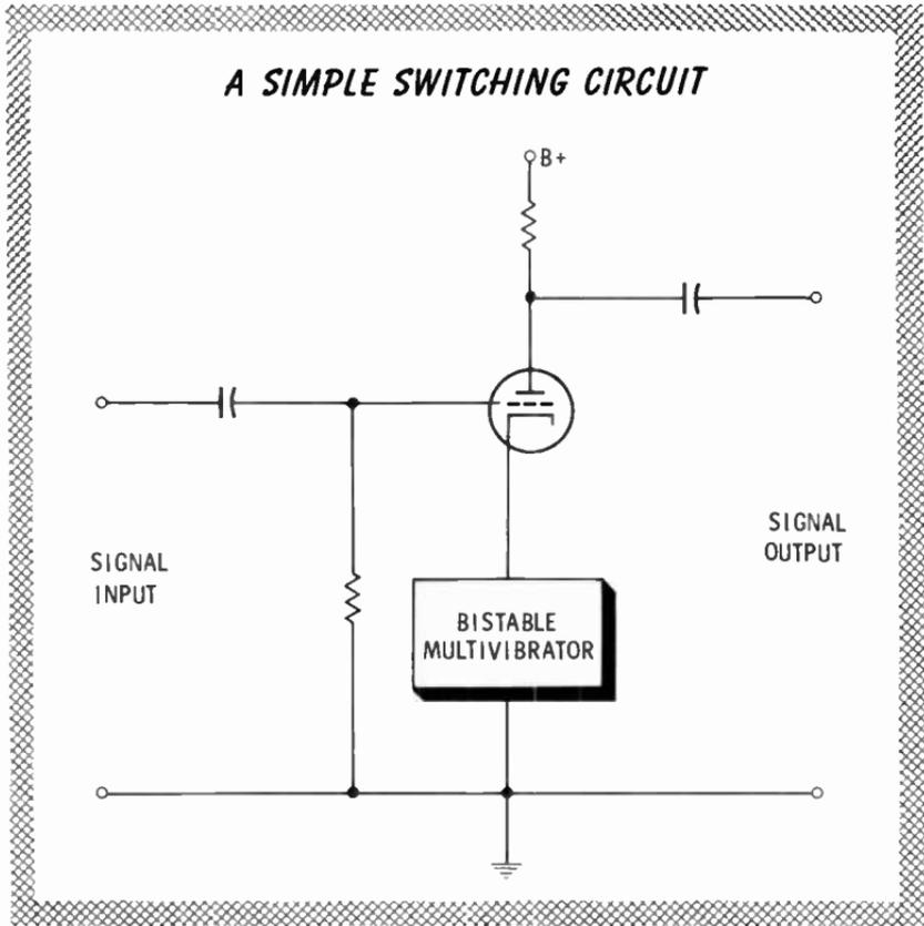
a large positive voltage to the cathode. This has the same effect as making the grid negative, and the tube is cut off. Another pulse to the multivibrator causes it to change states again, the cathode of the tube is returned to its operating voltage and the tube is able to amplify.
