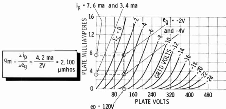
A34. Grid bias is the difference in potential between the **grid** and the **cathode** (not cathode to grid).
