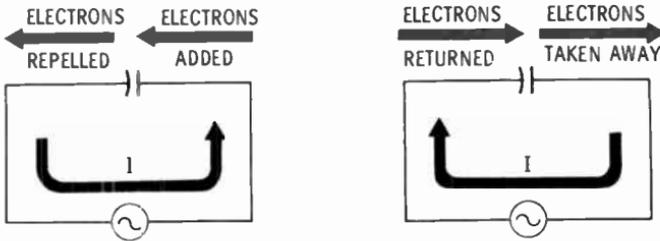
An AC voltage can, in effect, get across the dielectric; since the voltage is alternating, it causes an AC current on the other side. In other words, **voltage changes** are transmitted across the gap.
