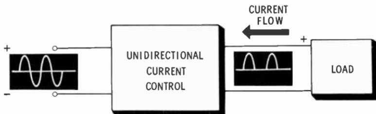
This simple principle is shown above. An AC voltage is applied to a unidirectional current-control device. Current flows only during the positive portions of the input signal.
