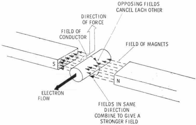
The direction of the magnetic field surrounding the conductor can be determined by applying the **left-hand rule** for straight conductors. Wrap the fingers of your left hand around the conductor so that your thumb points in the direction of electron flow through the conductor. Your fingers then show the direction of the magnetic field surrounding the conductor. External magnetic fields are considered to flow from the north pole to the south pole.
