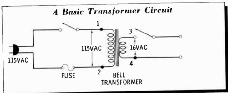
The lines between the primary and secondary windings indicate an iron core which provides an easier path for the magnetic field through the coils.
