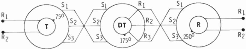
When connected to two synchro transmitters, the DR rotor position is the sum or difference of the rotor positions of the two generators. The synchros below are connected for subtraction.
