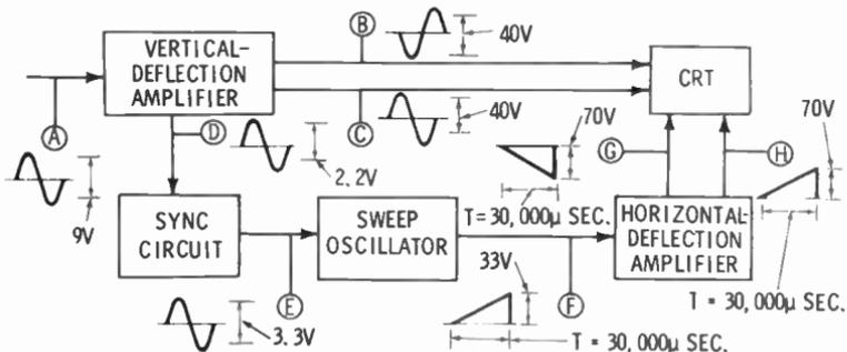
The above illustration is representative of a **servicing block diagram**. The letters in circles identify significant test points. The waveforms beside them show the shape, voltage,
