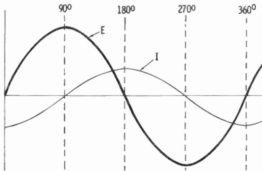
**CURRENT LAGS THE VOLTAGE BY  $90^\circ$  IN AN INDUCTANCE**
