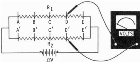
How much voltage would you measure between points D and D'? The answer is zero volts. The potential difference between A and D is 9V; this is equal to the difference between A' and D'. Therefore, no potential difference exists.
