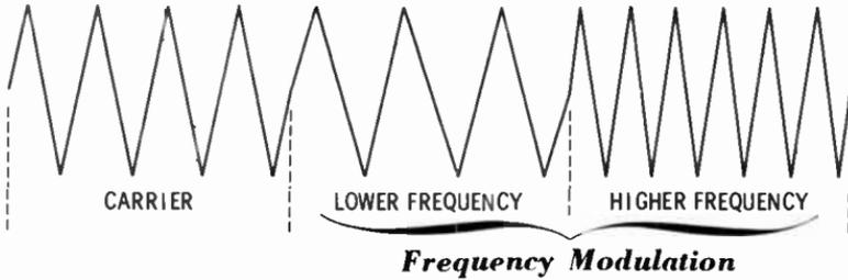
of a carrier is varied in accordance with the amplitude of an audio signal.
