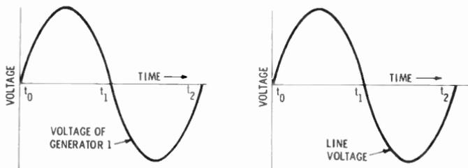
**OUTPUTS OF TWO SYNCHRONIZED GENERATORS**
