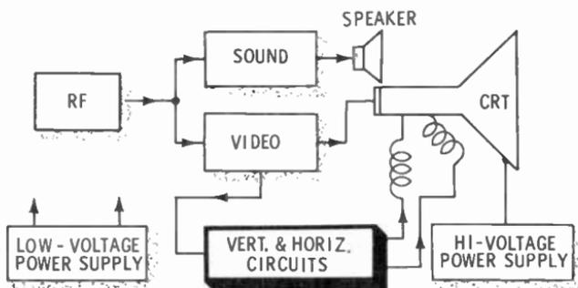
The schematic diagram included in the technical manual or servicing folder for the receiver should be used in locating the output test point of the probable faulty function. You will find that a schematic diagram will be your most valuable single item for troubleshooting.
