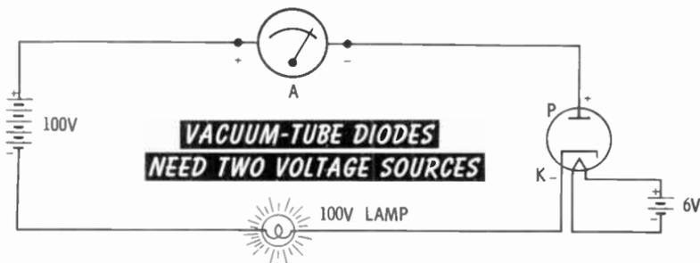
Current flows. Note that this particular diode requires a 6-volt source to heat the filament and 100 volts across the cathode and plate. Other vacuum-tube diodes operate with higher or lower voltages, but all require two sources.
