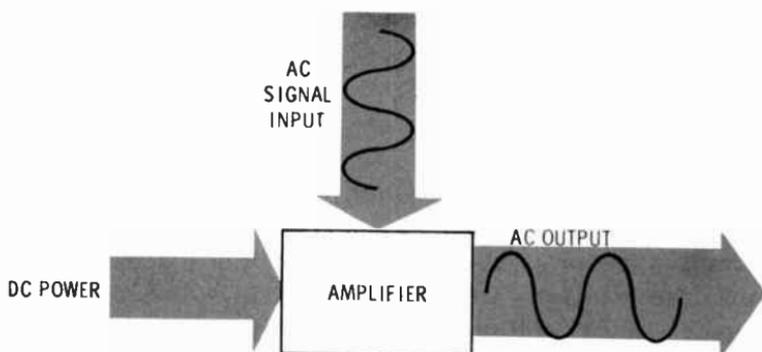
You can see from this diagram that the amplifier does not magically transform a low-power or low-voltage signal into a larger one. You can't get more power out than you put in. Instead, an amplifier controls the DC power from the power supply according to the variations in the AC input signal.
