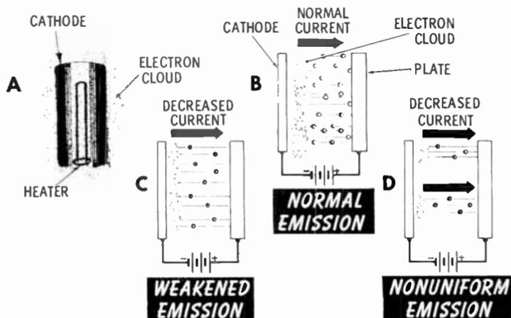
capability of the cathode has decreased after many hours of operation. A smaller quantity of electrons in the cloud causes a reduction in plate current. In figure D the cathode has weakened more in some areas than in others, resulting in a reduced number of electrons available for plate current.
