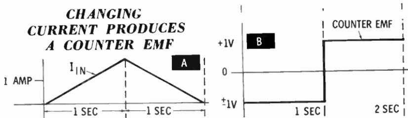
In part A above, with the current **increasing** at 1 ampere per second, a counter voltage of 1 volt appears and opposes the increase in current. In part B, as the current is **decreasing**, the inductive counter voltage of 1 volt is in a direction that tends to keep the current flowing. One henry is a very large value of inductance. Therefore, inductances in millihenrys (mh) and in microhenrys ( $\mu$ h) are more often found.
