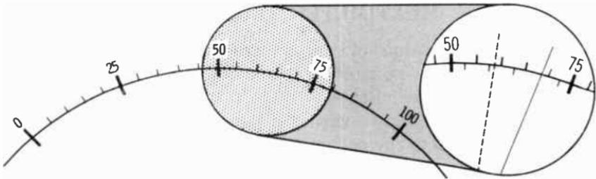
**Q16.** The solid pointer in the diagram above is between 65 and 70 and slightly beyond the midmark. The meter reads 68. What is the reading indicated by the dotted pointer?
