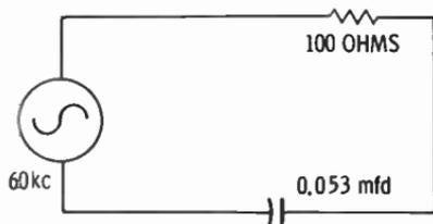
Draw a vector diagram on graph paper to find the impedance in the circuit above. Measure the phase angle with a protractor.
