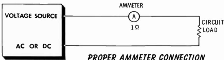
The resistance of most ammeters is less than 1 ohm. Added in series with the load resistance, very little change is made to the total resistance. If the load were 10,000 ohms, for example, the new total resistance would be 10,001 ohms—hardly enough change to make a significant difference in the current. If the load were only 1 or 2 ohms, however, a difference would be noted.
