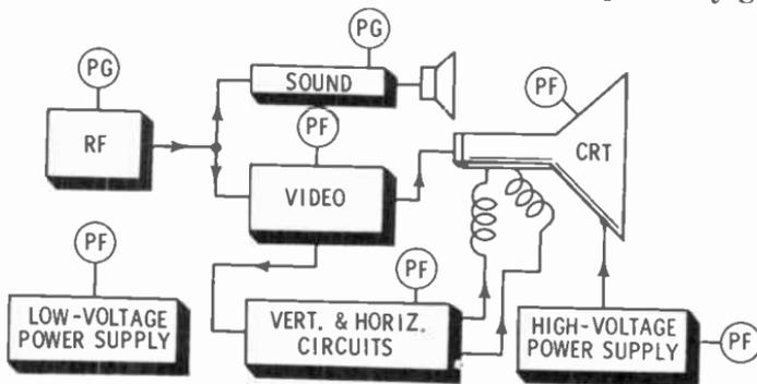
Five functions are suspected as being probably faulty. In which order should they be tested to arrive at a Step-3 conclusion (exposure of the single faulty function)?
