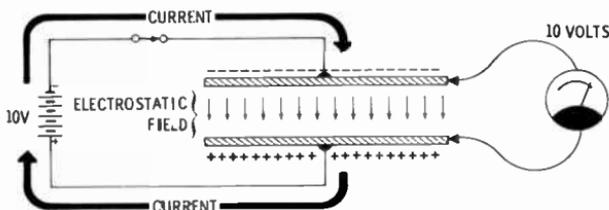
Current will flow until a charge (voltage) of ten volts appears across the plates. The plates are conductors and therefore have electrons free to flow as current. Electrons
