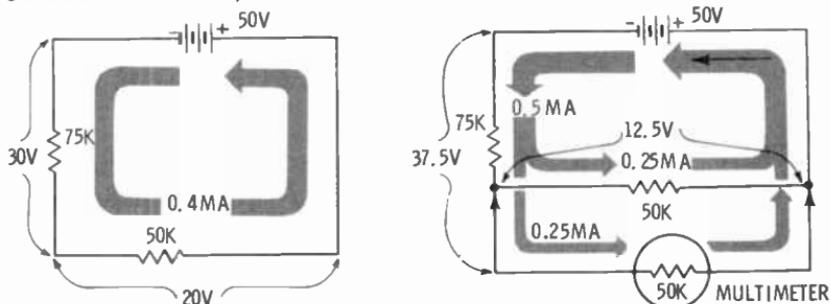
*A Multimeter Loads a Circuit*
