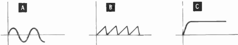
Q7. AC currents and voltages usually change regularly in a smoothly curved form. Which of the following is the usual AC waveform?
