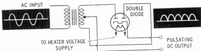
Both halves of the AC sine wave appear in the output of the full-wave rectifier. The output is still a pulsating DC, but it is smoother than the half-wave output. With proper filtering, the output of a full-wave rectifier can be smoothed further into a steady DC current.
