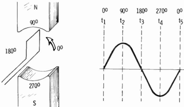
**A ROTATING COIL CAN CREATE A SINE WAVE**
