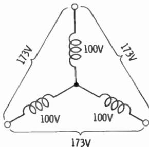
**VOLTAGES IN A WYE-CONNECTED, THREE-PHASE ALTERNATOR**
