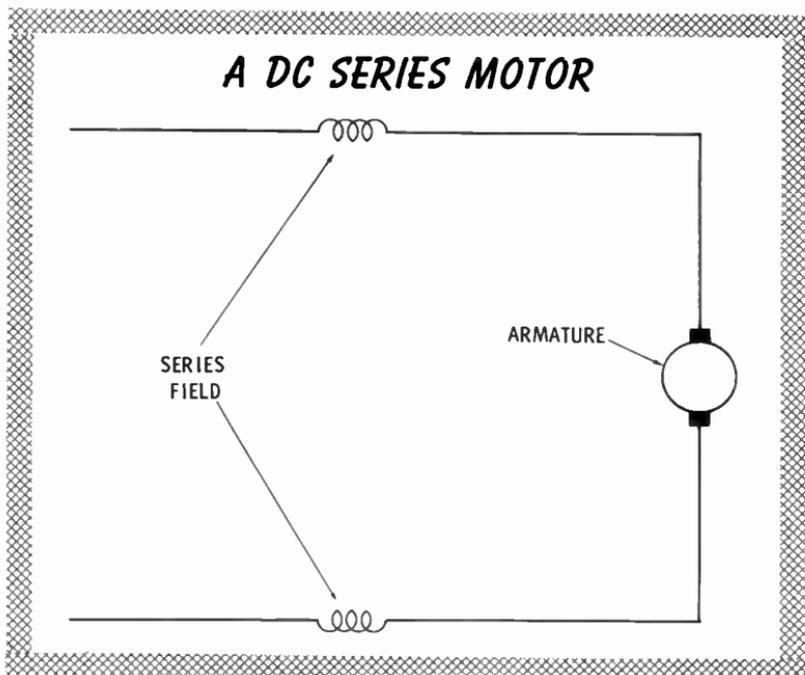
The starting and stalling torque of a series motor is excellent. It will start and carry very heavy overloads. Speed regulation, however, is very poor. The speed decreases as the load increases. Therefore, the motor turns slower with
