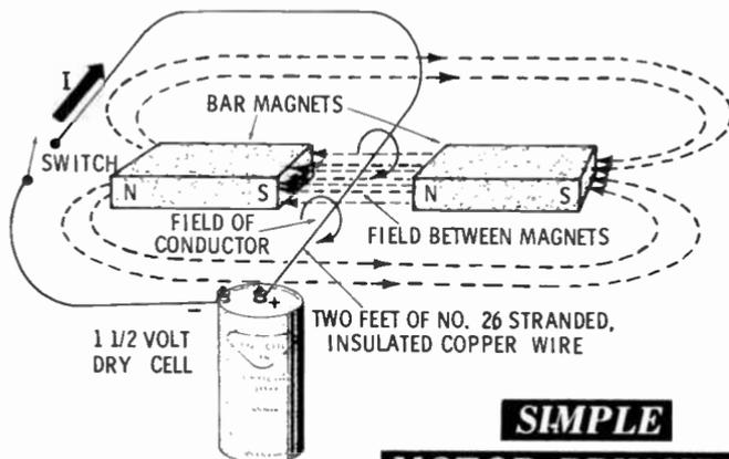
reopened quickly, the battery will be drained of its electrical energy. When the switch is closed, the conductor should jump. When the switch is opened, the conductor should return to its original position.
