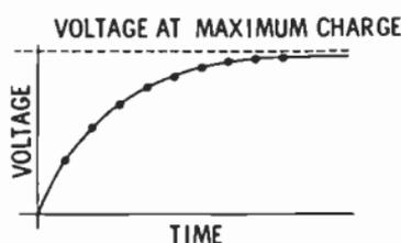
The figure above shows the way a capacitor charges. The dots show the voltage increase for each input pulse. The actual amount of voltage depends on the nature of the pulses and the circuit. It is not desirable to design the counter so that  $C_2$  discharges near its maximum-charge value. This is because each additional pulse causes a smaller increase in voltage, and it is difficult to be sure that the capacitor will discharge after the desired number of pulses.
