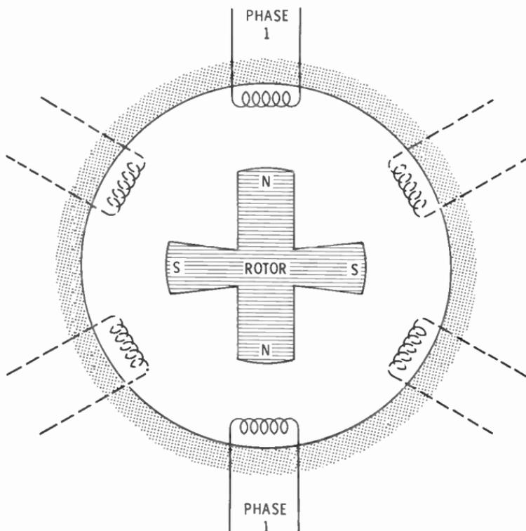
Now look at the figure above. This machine has four poles on the rotor. Four poles pass each winding during each revolution. Therefore there are two complete cycles of current in each winding for each revolution of the rotor. A machine with eight poles will have four complete cycles of current in each winding for each revolution of the rotor, etc.
