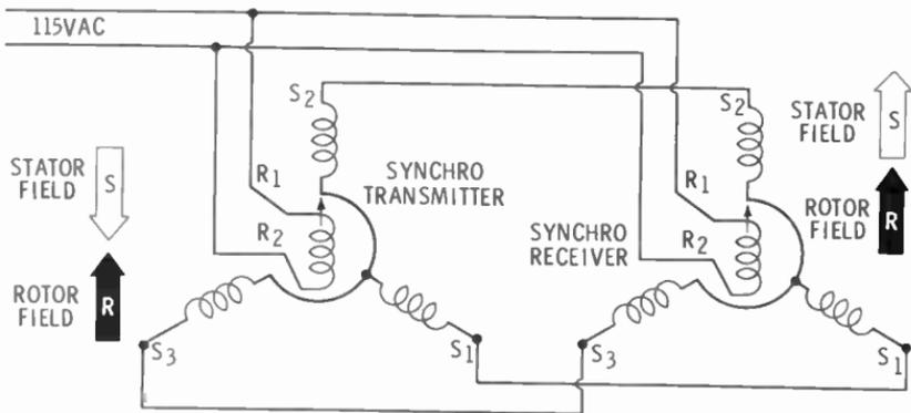
Since the rotor currents are in phase, the directions of their magnetic fields will be identical. The stator field in the transmitter is opposite to the rotor field. However, the stator field of the receiver will be in the same direction as the transmitter rotor field. The rotor field of the receiver will be attracted to align itself in the stator field direction.
