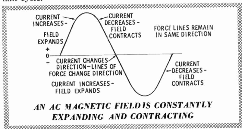
The diagram on the opposite page demonstrates how the magnetic field expands and contracts with the rise and fall of current. The field is in constant motion. An alternating current, therefore, induces current to flow in another conductor or coil. In this case, the induced current will also be alternating.
