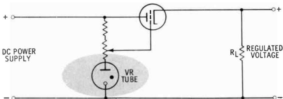
A vacuum-tube circuit can be used as a series voltage regulator. The current passing through the tube from cathode to plate depends on the grid bias. Another way to say this is that the resistance of the tube depends on the grid bias. Therefore, by varying the voltage on the grid, the tube resistance can be changed as necessary.
