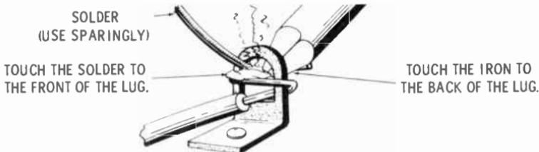
The iron should be applied to the back side of the terminal and held firmly against the wire. After a few seconds, touch the solder to the wire at the front of the terminal. If the solder readily melts, the connection is sufficiently heated. If the connection is not hot enough, remove the solder and continue heating until it is. Do not touch the solder to the iron.
