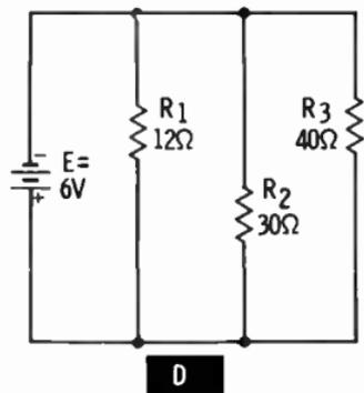
**Q9. What is the power dissipated by each resistor and the total power for each circuit above?**
