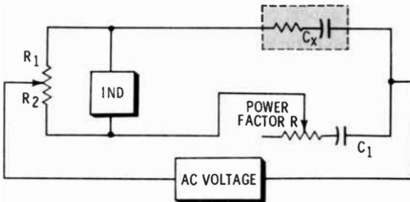
The  $R_1/R_2$  potentiometer is adjusted for a null indication as was done before, or as close as the resistance of  $C_x$  will permit. The variable resistance in series with  $C_1$  is then adjusted for the final null reading. A front-panel extension of the variable resistance, probably labeled **POWER FACTOR**, will give the percentage of power factor.
