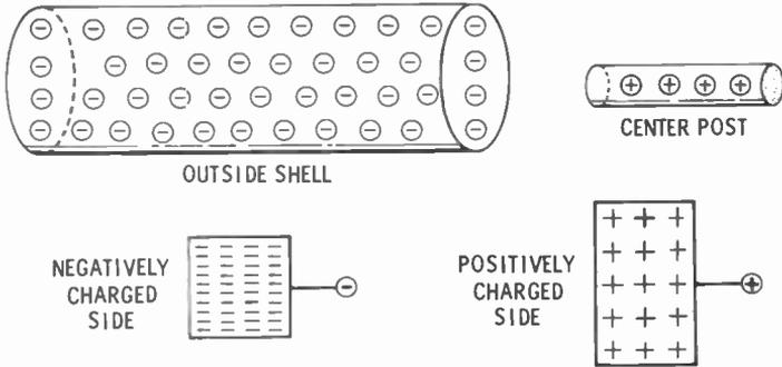
A battery is one such form of voltage source. It has an excess of negative charges on one terminal and a lack of negative charges on the other terminal. When the two battery terminals are applied properly to other elements, a complete path from one terminal to the other is formed. The more negative terminal gives off negative charges that pass through the other elements to the positive terminal.
