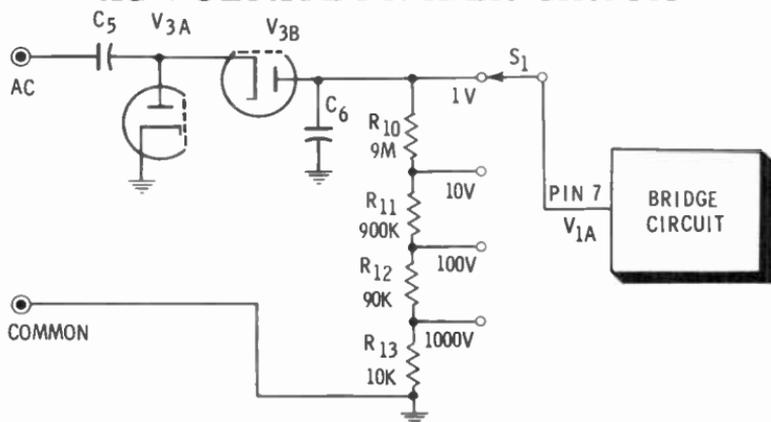
vent the DC that may be present in the input voltage from reaching the bridge circuit. In this arrangement the VTVM actually measures the peak value of the AC voltage. The rms value of a sine wave is 0.707 times the peak value. The scales of most VTVM's are marked to read the rms value.
