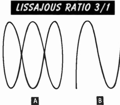
the starting point. The figure is continuous; it has no beginning or end. Figure B, however, is not continuous; it has a beginning and an end. Its pattern is **open**.
