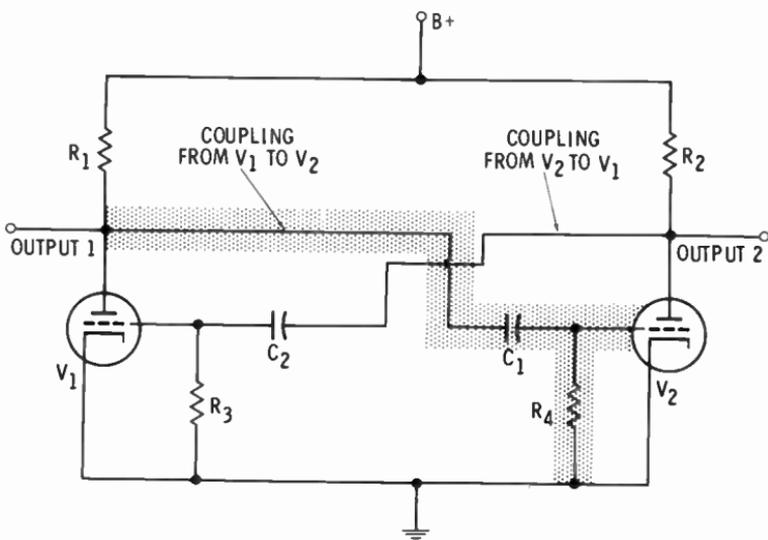
How does this circuit work? When the B voltage is applied, both tubes begin to conduct, as in a normal amplifier. If the current in both tubes were precisely the same, that is all that would happen. However, because of slight differences in the tubes or other components, one tube will conduct a little more than the other.
