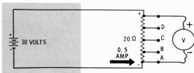
If a 20-ohm resistor is connected across a 10-volt source, as shown in the illustration, a voltmeter reading across the resistor will be 10 volts. This means that the voltage of the source is not only applied across the load, but it also exists within it.
