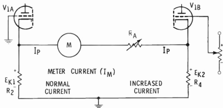
Suppose a positive voltage is applied to the grid of  $V_{1B}$ . Plate current in  $V_{1B}$  will increase, raising the voltage across  $R_4$ .  $E_{K2}$  will now be a larger positive voltage than  $E_{K1}$ . Current will therefore flow from left to right through the meter.
