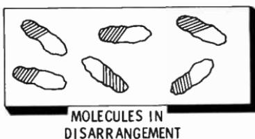
Each molecule within a bar of iron has its own north-seeking and south-seeking poles. Although the magnetic strength of a single molecule is very weak, there are many millions of molecules in a very small piece of metal. When magnetically aligned in the same direction, they can develop a strong magnetic field. This is known as the **molecular theory of magnetism**.
