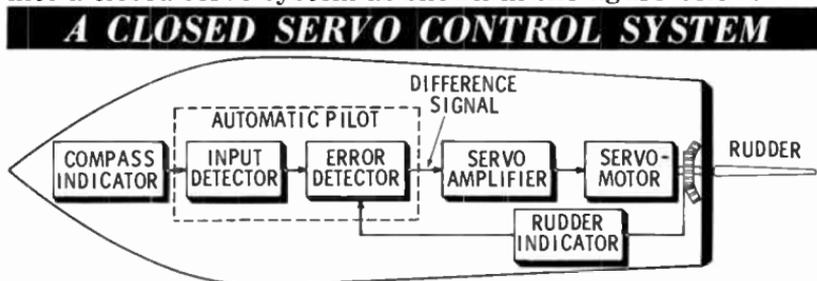
When the ship drifts off course, the change in compass heading generates a voltage signal which is transmitted to the error detector. Since the rudder and heading (compass) positions no longer agree, a difference signal is sent to the servo amplifier and motor to turn the rudder an amount and in the direction required to bring the ship back on course. When the ship is back on course, the rudder will have been returned to its amidships (straight ahead) position.
