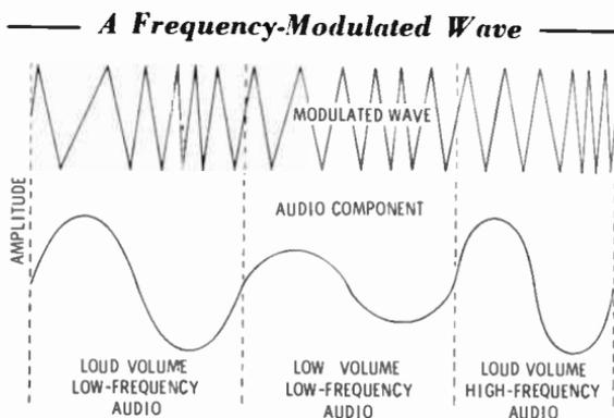
**The Detector**—FM and AM detectors have the same purpose—to remove the audio component from the modulated intermediate frequency. For FM, the variations in frequency are changed into voltage variations by the detector. The output of the detector (quite frequently called a **discriminator** because it discriminates between AF and IF), is
