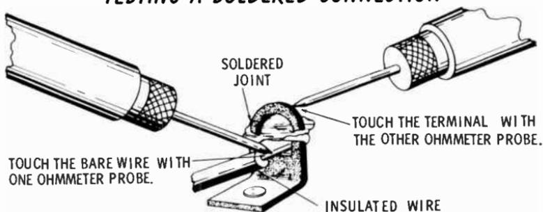
An ohmmeter test does not always reveal a poor soldering job. But if the meter reads zero; the solder looks neat, smooth, semishiny, and well blended into the metal; and you observed all the precautions, the connection should be electrically good. The precautions are restated below.
