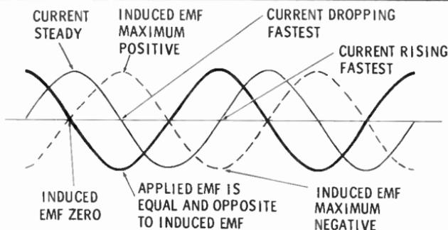
In a DC circuit, inductance has an effect only when the direct current first starts to flow, and then again when you try to stop it. But in AC circuits the voltage is constantly changing and inductance constantly acts to retard the change in current.
