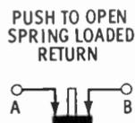
A **push-button switch** uses a button which must be pushed to form a closed (or open) condition. One type remains closed (or open) until the next push. Another kind is the **momentary** push button. It stays closed (or open) as long as the button is depressed.
