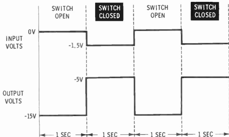
With the switch open, the input registers 0 volts and the output  $-15$  volts. With the switch closed, the input changes to  $-1.5$  volts and the output to  $-5$  volts. The same readings occur each time the switch is opened and closed.
