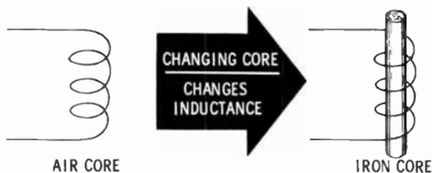
There are formulas for calculating the inductance of various types of coils. There are also tables for simple, one-layer coils. Using these formulas, you can design a coil to have any desired value of inductance, or calculate the value of an unknown inductance.
