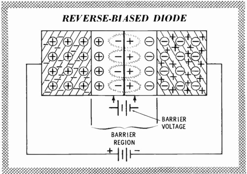
in a larger barrier voltage. The action continues until the barrier voltage equals the reverse bias (battery voltage). No current flows because these voltages are equal and opposite. This condition is called equilibrium.
