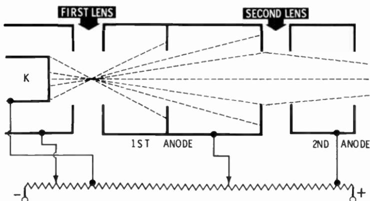
cross at a focal point within the field. The second lens bends the spreading streams and returns them to a new focal point.
