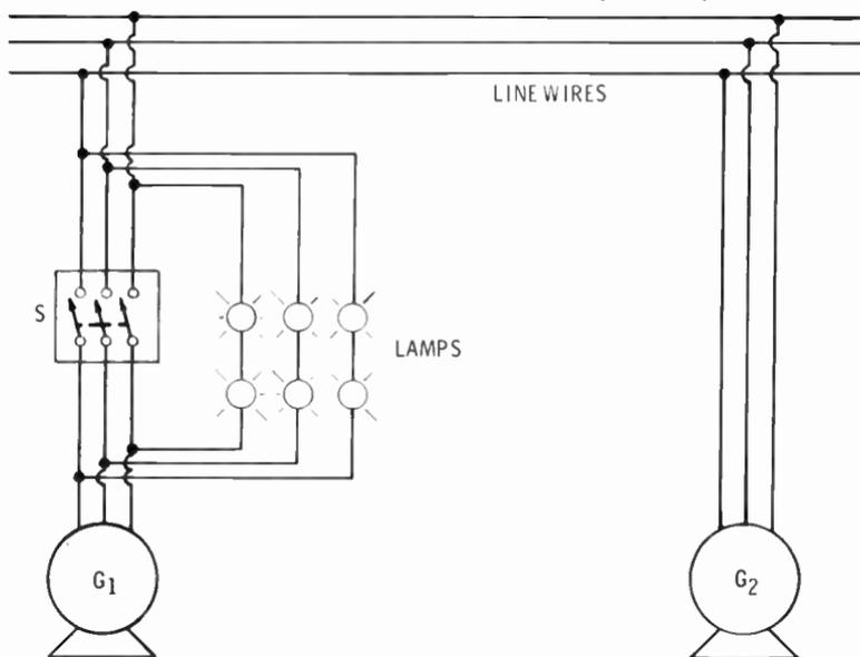
Care must be taken that the three phases are in the right sequence. If the phases are reversed in the generator being placed on the line, it will be damaged. In order to avoid this
