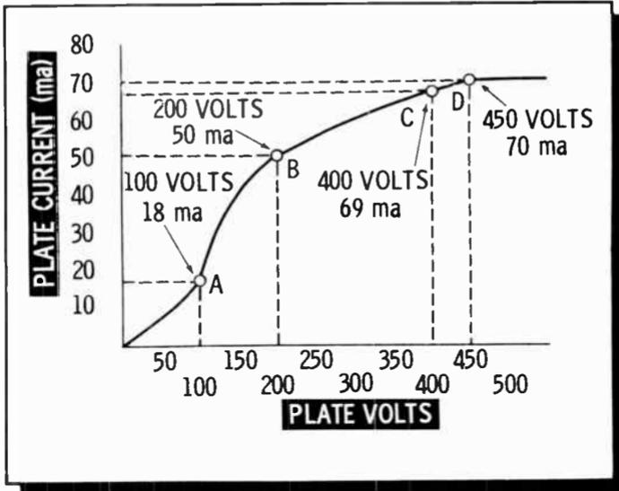
To see how the DC plate resistance varies with plate voltage, calculate  $R_p$  at each of the points marked on the graph. The calculations yield the following results:
