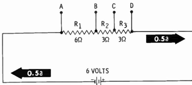
Normally, the relatively small voltage drop of conductors is disregarded since the wire resistance is usually a very small fraction of the total load resistance. The tapped resistance in the diagram above has a total of 12 ohms with a total of 6 volts (from the source) applied across it. A current of 0.5 amp flows through each portion. The voltage (IR) drop between terminals A and B will be 3 volts in accordance with Ohm's law, resistance ratio, or a voltmeter measurement.
