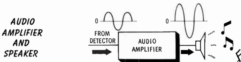
**The Audio Amplifier**—The final circuit in the receiver amplifies the AF fed to it by the detector. The amount of amplification can be varied by the volume-control knob on the front of the receiver. The output of the audio amplifier is applied to the speaker voice coil, causing the speaker cone to reproduce the sound that originated at the studio.
