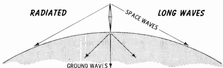
The diagram illustrates the **propagation** (travel of electromagnetic radiation) of long waves as they radiate from the antenna of a commercial radio station. The frequency is between 535 and 1,605 kilocycles. The radiated energy has a **space wave** that travels essentially in a straight line. Low frequencies also have a **ground wave** that hugs the ground until the radiated power decreases so much with distance that reception is no longer possible.
