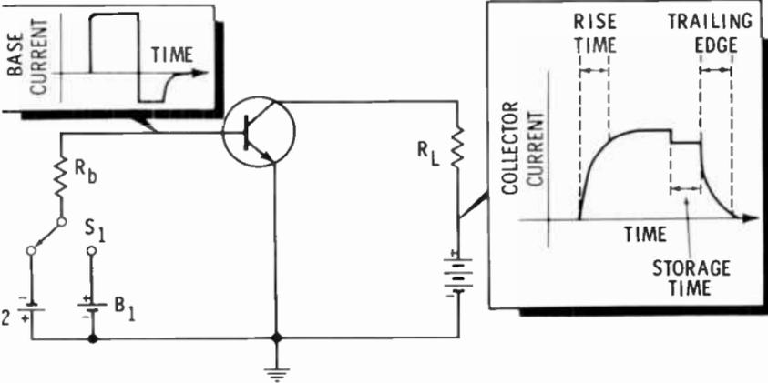
voltage of battery  $B_1$  forward-biases the emitter-base junction. The base current quickly reaches maximum. The collector current also increases. The time required for it to increase from 10% to 90% of maximum is the rise time.
