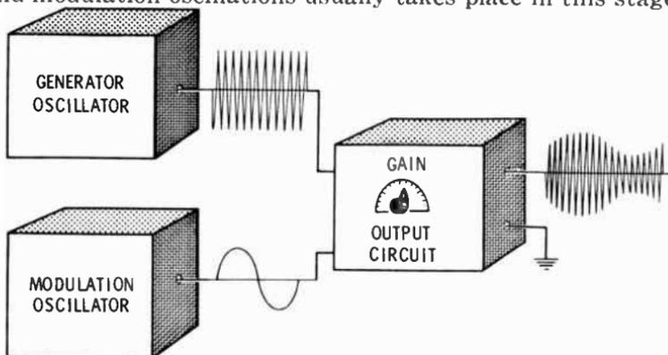
A gain control is normally provided to vary the amplitude of the output signal. To permit impedance matching of the
