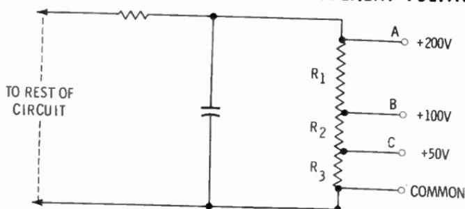
Suppose that the DC requirements of the rest of the equipment were +200, +100, and +50 volts. A power supply can be selected or designed to produce a current large enough to cause a drop of at least 175 volts across  $R_1$ .
