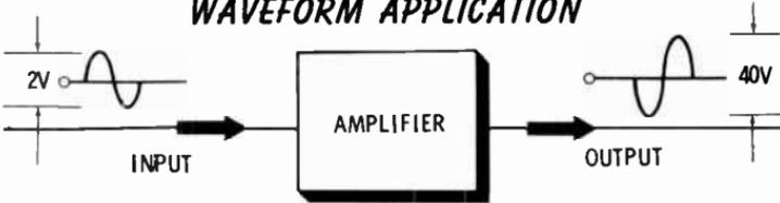
In the circuit above, the amplifier has a sine-wave input and output. Because of the characteristics of this amplifier, the output waveform is a reversal of the input. The output is also greater in amplitude: 40 volts output as compared to 2 volts at the input.
