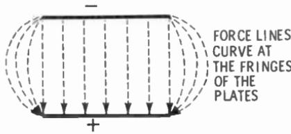
in all directions around a line of force. The lines of force at the edges of the field are bent outward because there are no lines outside the field to repel them inward.
