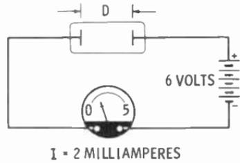
**Distance Between the Plates**—The figure shows two sets of plates with the same voltage applied between the plates of each set. The plates in one are twice as far apart as the plates in the other. The plates that are  $d$  distance apart allow four times as much current to flow as the plates  $D$  distance apart.
