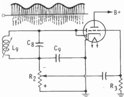
**Audio Amplifier**—This stage further amplifies the audio signal and feeds it to the primary of the speaker transformer. The speaker is energized, and the audio originating at the broadcast studio is reproduced.
