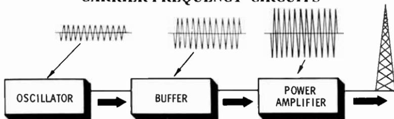
**The Oscillator**—The purpose of the oscillator is to generate a stable RF signal. The resistance, inductance, and capacitance that make up its input circuit are such that they will not allow the vacuum tube in the oscillator to amplify any other signal but that of the desired frequency. The stable-frequency, low-amplitude output of the oscillator is shown above.
