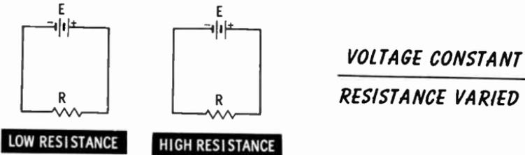
Current cannot flow as easily through a high resistance as it can through a low resistance. Thus, the circuit on the left will have the greater current flow. The circuit with the higher resistance will require a higher voltage source to cause an equal amount of current to flow.
