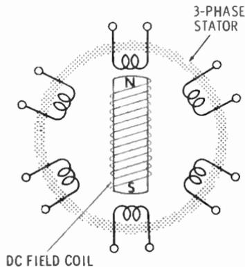
As the magnetic field in the stator rotates, the constant DC field rotates to keep aligned with it. As you can see, the speed of this motor depends on how fast the magnetic field rotates. The speed of the magnetic field depends on the frequency of the three-phase AC source. The synchronous motor cannot operate at any speed except that of the rotating field, which is called **synchronous speed**. Synchronous motors are used where it is important to maintain constant speed.
