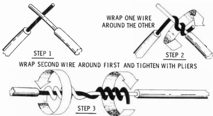
**Stranded-to-Solid Splice**—Twist the stranded wire into a straight, tight spiral and wrap around the solid wire as in Step 2 of the Western Union splice. Make at least a half-dozen turns. Fold and tightly crimp the end of the solid wire over the turns. Solder and wrap the splice with tape.
