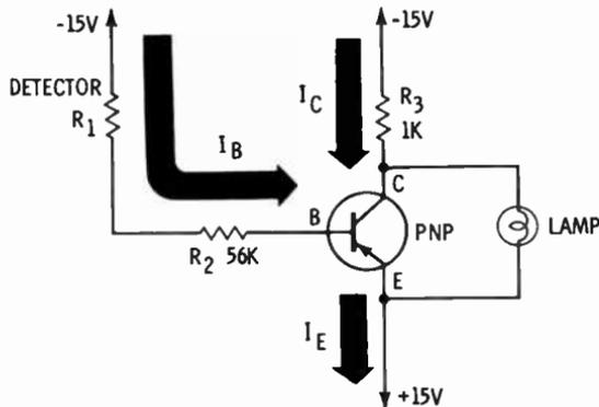
*Current Flow in the Transistor Alarm Circuit*
