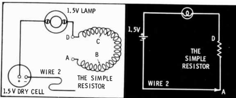
**A Rheostat**—A device that can be adjusted to provide a desired amount of resistance is called a **rheostat**. It has a moving contact that performs the function of moving wire 2 across the resistance from point A to D.
