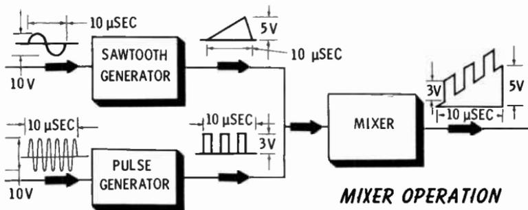
The sawtooth and pulse generators have sine-wave inputs of different frequencies. The input frequency of the pulse
