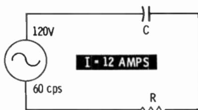
Suppose you know the input voltage, the frequency, and the current flowing in the above circuit. Also, suppose you know that the phase angle of the circuit is  $60^\circ$ .
