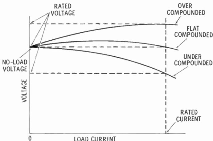
When the effect of the series winding produces a greater terminal voltage at rated load than at no load, the generator is said to be **overcompounded**. Compound generators are usually wound so that they are slightly overcompounded.
