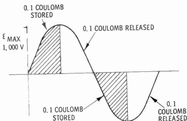
**Q16.** How much energy will be stored in a 100-mfd capacitor in the first quarter cycle of an applied AC voltage of 1,000 volts maximum?
