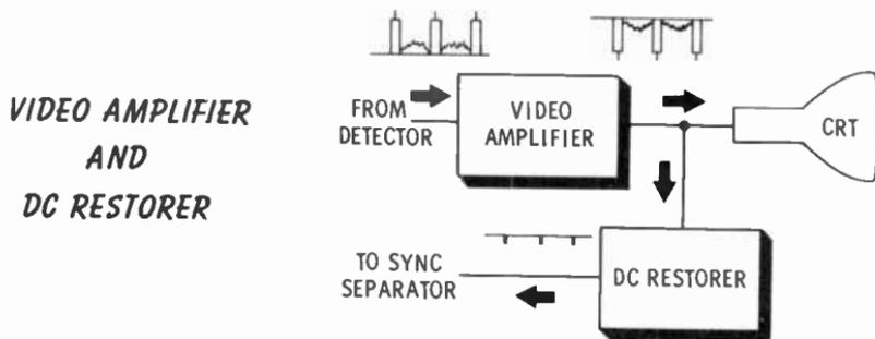
**Video Amplifiers**—The output of the detector is a relatively weak signal, not strong enough to cause a reproduction of the picture. Video amplifiers are therefore required to achieve the necessary signal amplitude. These must be wide-band amplifiers because the frequency content of the picture signal covers a wide frequency range.
