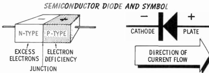
Voltage polarities necessary for current to flow are labeled on the symbol. Current flows through the diode toward the arrowhead.
