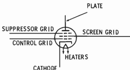
The fifth element of the pentode is called a **suppressor grid**. This element is usually connected internally to, and has the same potential as, the cathode. In other words, the suppressor grid is negative with respect to the plate. Spacing between the turns of wire of the suppressor grid is wide enough for plate current to pass through, but yet sufficiently close enough to repel the negative secondary electrons back to the plate.
