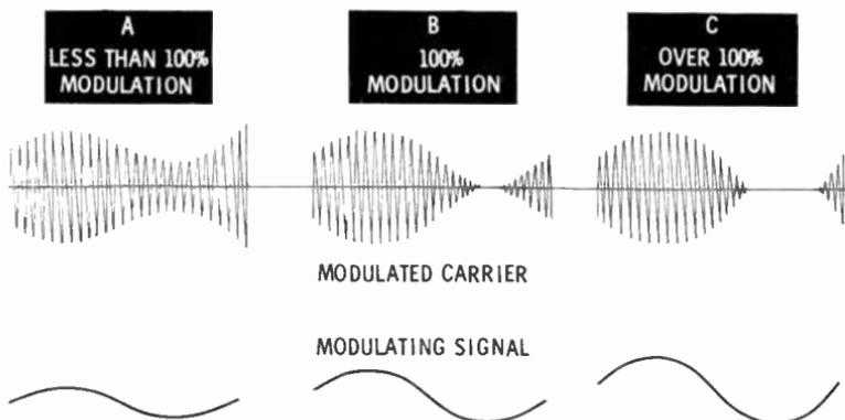
The amplitude of the modulating signal in part B above is such that the **envelope** (outline of modulation on the carrier) is caused to become zero for an instant before rising again. This is 100% modulation. Modulation is less than 100% in part A. The exact percentage is determined by the relationship between the amplitudes of the carrier and modulating waves. Part C shows modulation greater than 100%. This causes distortion in reception.
