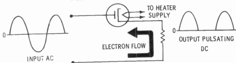
The device just described is called a **half-wave rectifier** because only half of the AC sine wave appears in the output. Although this current never reverses direction, it is a very rough, pulsating DC which is not satisfactory for most purposes. A smoother DC can be obtained from a **full-wave rectifier**.
