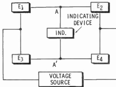
If voltage were applied across the bridge (parallel) circuit, current through the indicating device would be zero only when the voltages appearing at points A and A' were equal.
