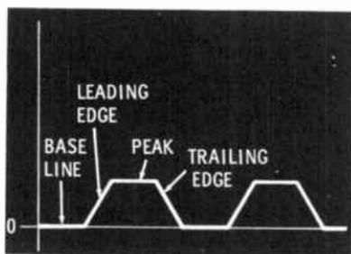
It is often necessary to know how long it takes a pulse to rise from the base line to its peak (**rise time**) or to go from its peak value back to the base line (**decay time**). These times are measured between 10% and 90% of peak value.
