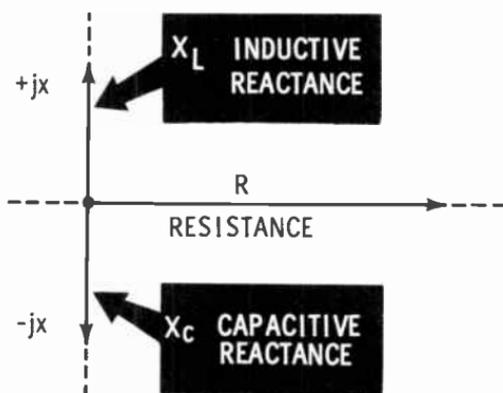
This difference is in the direction of the greater of the two reactances. So, if a circuit contains a capacitor, the reactance of which is  $-j50$  ohms, and an inductor, the reactance of which is  $+j100$  ohms, the net result is equivalent to an inductive reactance of  $+j50$  ohms.
