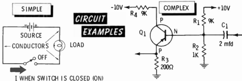
travels from the voltage source through the conductors and the load and returns to the source. This includes the path from terminal to terminal through the source.
