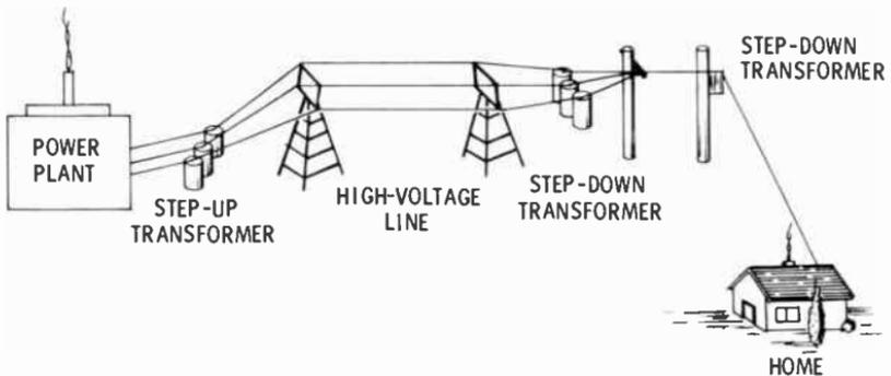
Alternating currents are generated in very large quantities in power plants. The electricity used in your home comes from a power plant. The total current capacity of a power plant can reach several thousand amperes at 4,160 volts.
