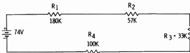
Q18. What is the voltage, with reference to ground, for all the points (P) on the following diagram?
