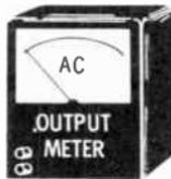
VTVM OR OTHER AC MEASURING INSTRUMENT. ATTACH PROBES TO SPEAKER VOICE-COIL TERMINALS.
