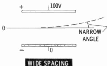
**Difference of Potential**—Intensity of the electric force can also be varied by the difference of potential on the plates.
