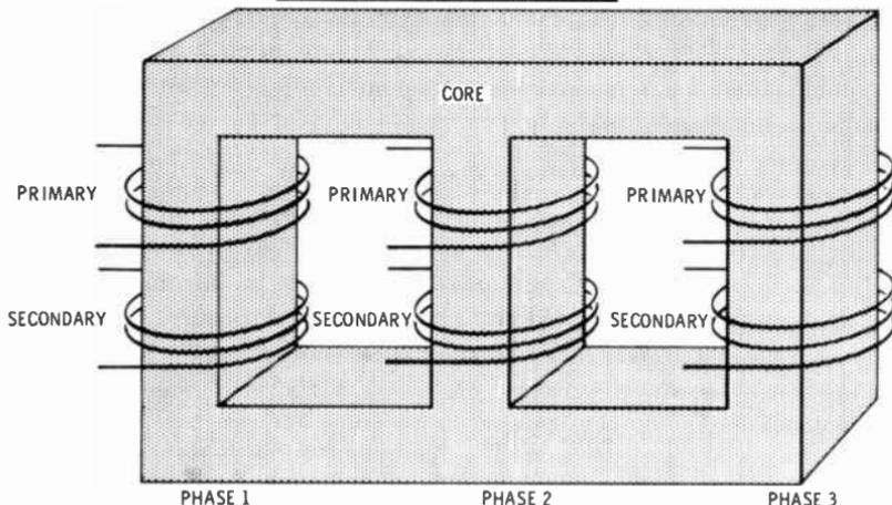
The primaries and the secondaries can be connected in any combination of delta and wye. For example, the primaries can be wye-connected and the secondaries delta-connected, or vice versa. Or both the primaries and the secondaries can be wye- or delta-connected.
