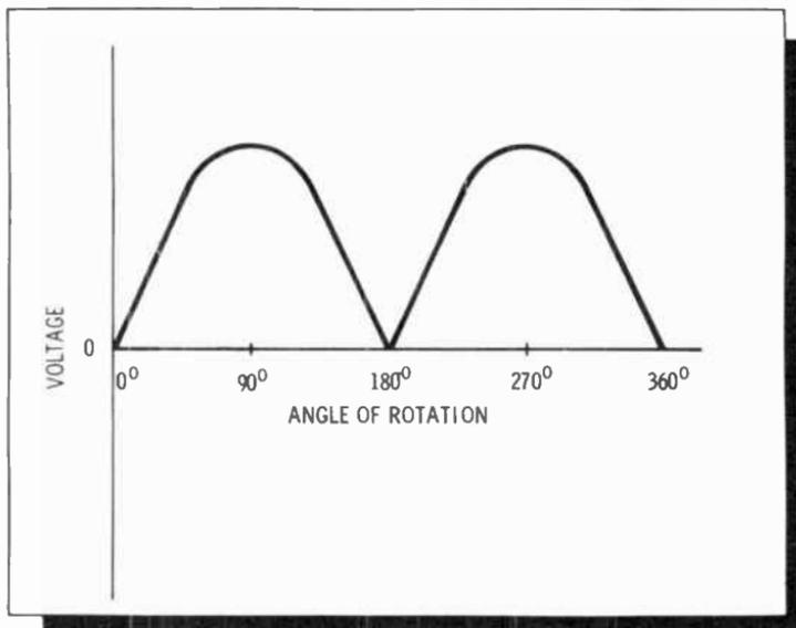
obtained because the connections to the armature coil are reversed every half cycle when the voltage is zero and is about to change polarity.
