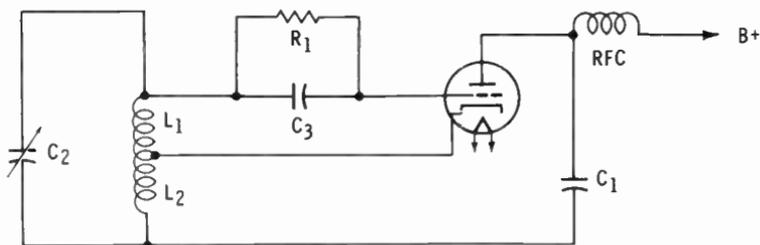
frequency of the tank is adjusted by  $C_2$ . The RFC (radio-frequency choke) in the B+ line prevents AC on the plate from entering the B+ source.  $R_1$  and  $C_3$  establish grid bias.
