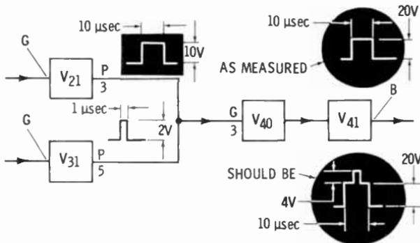
The first test should be made at the converging point ( $G_3$  of  $V_{40}$ ). A comparison of the two output waveforms—the measured waveform and the correct waveform—indicates that the 1-microsecond pulse is missing. A proper deduction shows that the small pulse does not leave  $V_{31}$ , therefore it is correct to make a test at the output of  $V_{31}$ .
