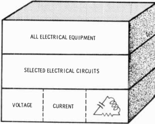
capacitance, and resistance. If you reduce any electronic equipment to the bare essentials, you will find that the equipment operates the way it does because of the circuit arrangement of L, C, and R and their effect on current and voltage.
