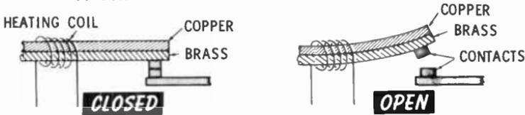
When the bimetal strip is heated, the brass expands more than the copper, and the strip bends away from the fixed contact and opens the circuit. The action of this relay depends on the heating effect of the current. That is, it depends on both the amount and the duration of the current. If a heavy current flows for a short time but not long enough to cause overheating of the motor, the relay will stay closed.
