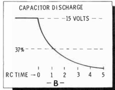
RC is a quantity obtained by multiplying R (ohms) by C (farads). Any capacitor in an RC circuit (such as this one) charges to 63% (actually 63.2%) of its final value (battery voltage) in one RC second. In 5 RC seconds it reaches full value. The arithmetic statements are:
