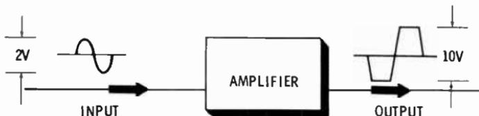
Instead of a sine-wave output, the tops of both peaks have been flattened. A section of circuit components (different from those in the preceding circuit) is responsible for the different outputs. The amount of gain is also different.
