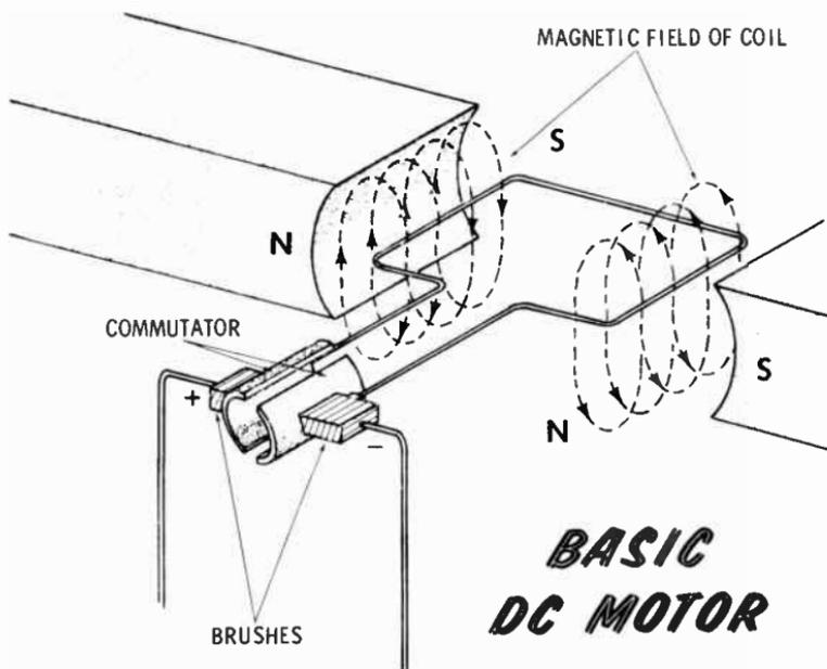
You can analyze the magnetic forces acting on the simple coil by using the left-hand rule for straight conductors. The figure above shows the field around the coil.
