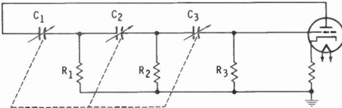
**Q12.** What characteristics of  $R$  and  $C$ , as shown in the above schematic, establish the value of frequency?
