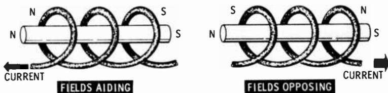
When current flows through the coil in the direction shown, the north pole of the magnet is on the left, and the south pole is on the right (left-hand rule for a coil). The magnetic polarity of the core material is identical to the polarity of the coil. When the circuit is de-energized, the magnetic field collapses. Any residual magnetism remaining in the circuit retains its original polarity.
