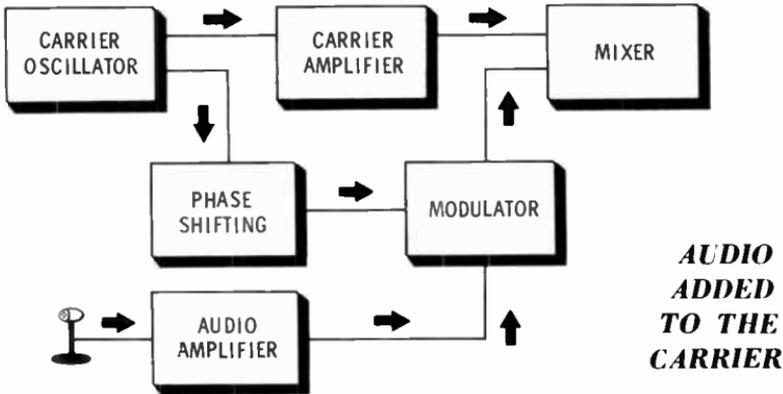
The **oscillator** generates a stable frequency which is simultaneously fed to an **amplifier** and a **phase-shifting** network. The phase-shifting stage shifts the frequency by a quarter of a cycle. The carrier and the shifted signal are no longer in step. The amplified audio from the microphone is mixed with the out-of-phase signal in the **modulator**. The output of the modulator is a series of sine waves that vary in amplitude in accordance with the amplitude of the original sound.
