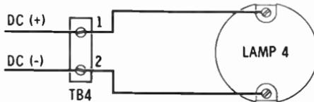
**The Airline Wiring Diagram**—The airline wiring diagram shows wire destinations without a connection between terminals. This type of diagram is used in the same manner as the highway diagram.
