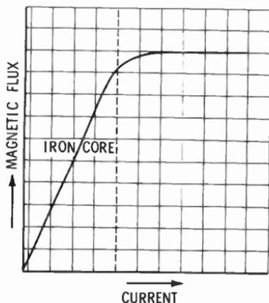
**AN IRON CORE BECOMES SATURATED AS CURRENT IS INCREASED**
