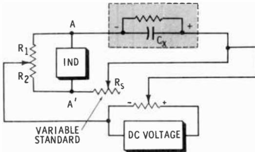
Essentially this is the same basic circuit as before. A switch on the front panel connects a variable resistance in place of  $C_1$  and changes the voltage source to a variable DC. Voltage is set at the rated working voltage of the capacitor. An electrolytic capacitor will be damaged if polarities are not observed when connecting it to the measuring posts.  $R_s$  is adjusted to balance the bridge and obtain a null reading. If the measured resistance is low, leakage is high.
