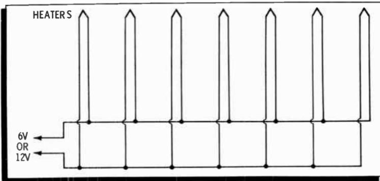
In each case, you can see that all sources or all loads are connected across the same two points. This produces a circuit which has one common voltage applied to all loads.
