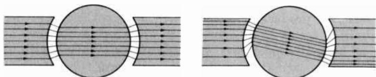
*No Armature Reaction*      *With Armature Reaction*
