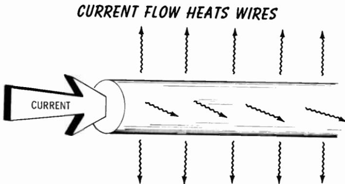
given off by a wire is determined by the type of metal in the wire and the quantity of current that is forced through it. A large current produces more heat in the same size and type of wire than a smaller current. If the current is the same, a smaller wire gives off more heat than one that
