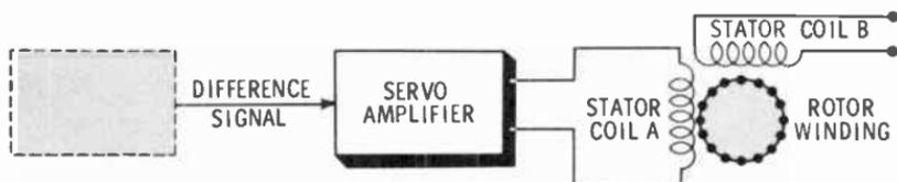
The diagram illustrates a two-phase induction motor, the type most frequently used in AC servomotor applications. Either a squirrel-cage or short-circuited rotor may be used.
