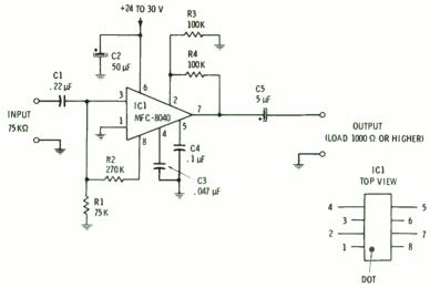
High-gain microphone preamplifier.
