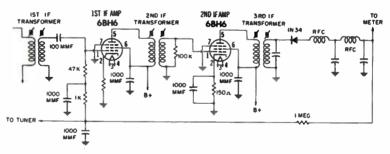
Typical IF and detector circuits for a field-strength meter.
