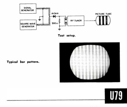
To Align a Split-Sound System in a TV Receiver
