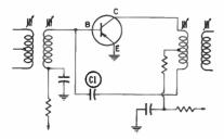
IF amplifier stage of a transistor radio.
