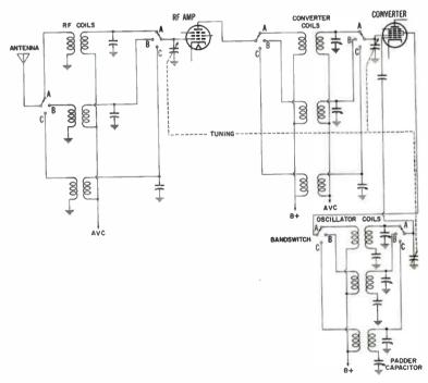
Head-end circuits of a typical multiband receiver.
