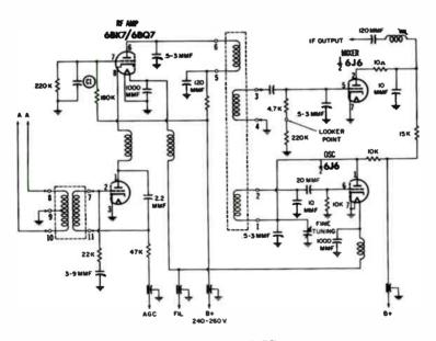
Schematic of a typical RF tuner.
