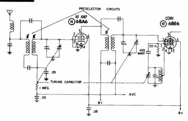
Preselector circuits in a typical receiver.
