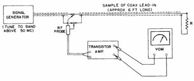
Measuring characteristic impedance of coaxial cable.
