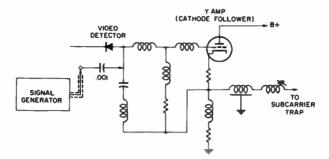
Typical picture detector and video-amplifier circuit.
