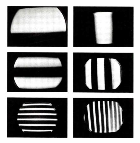
Typical bar patterns displayed on picture-tube screen when signal generator is modulated by audio oscillator.
