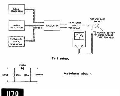
To Make an Over-all Signal-Channel Test For Transient Ringing
