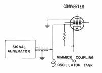
Substituting signal generator for local oscillator signal.
