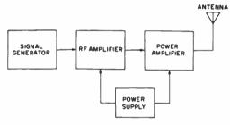
Using signal generator as VFO.
