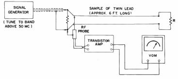
Measuring characteristic impedance of twin lead.
