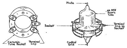
Figs. 15-23 (left), 15-24 (right). The ceramic socket for an acorn tube, showing the terminal clips. Connections to the control-grid and plate of the pentode are made directly to the leads from the tube instead of to clips on the socket.
