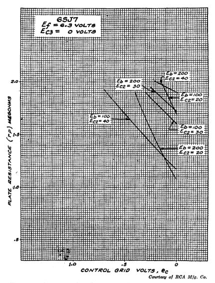
Fig. 12-10. These curves show the variation of the very high plate resistance of the 6SJ7 pentode as the control-grid voltage is varied. These curves are discussed on the next page.
