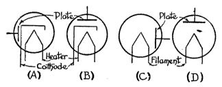
Fig. 6-4. The line indicating the plate may be drawn in any one of the four positions shown in the above schematic symbols of a diode.
