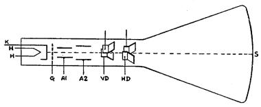
Fig. 15-25. The fundamental elements of a cathode-ray tube.
