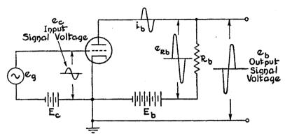
Fig. 11-9. The waveforms shown indicate the relative values of the voltages or currents, their phase relationships, and their locations in the triode circuit.
