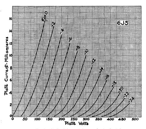
Fig. 8-6. The plate family of characteristic curves for the 6J5 triode.
