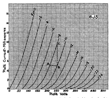
Fig. 8-8. The amplification constant can also be determined by using the plate family of characteristic curves as outlined in the accompanying text.
