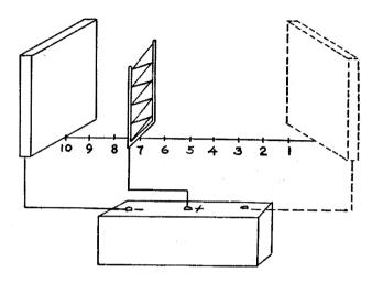
Locating a charged body closer to the test charge requires a much lower voltage to exert a certain constant force upon an electron than another charged body further removed.
