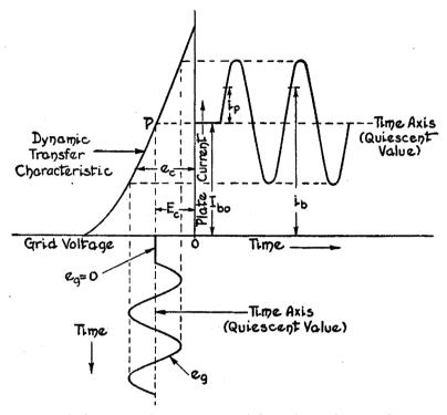
Fig. 11-4. The a-c and d-c components of the various voltages and current are identified in conjunction with a general dynamic transfer characteristic. Compare with Fig. 11-3.
