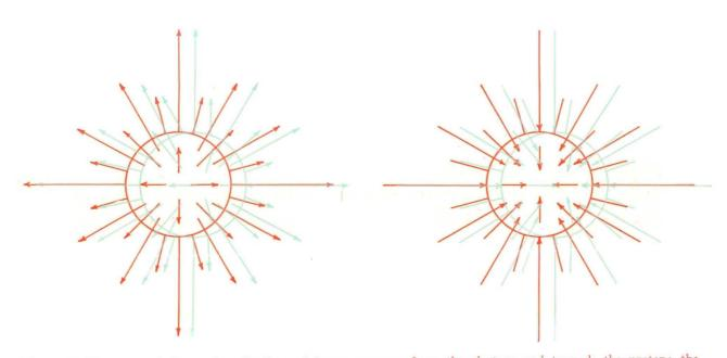
PLATE 2. The arrows indicate that the lines of force are away from the electron and towards the proton; the direction of the force exerted upon a negative test charge is indicated by the arrows. The lines of force radiate in all directions.
