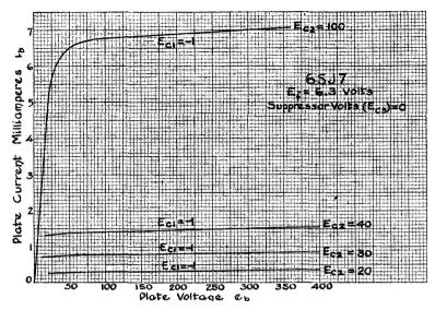
Fig. 12-12. These characteristics were made with the same control-grid voltage (—1 volt) and different values of screen-grid voltage. Note that the plate current increases with an increase in E<sub>cc.</sub>
