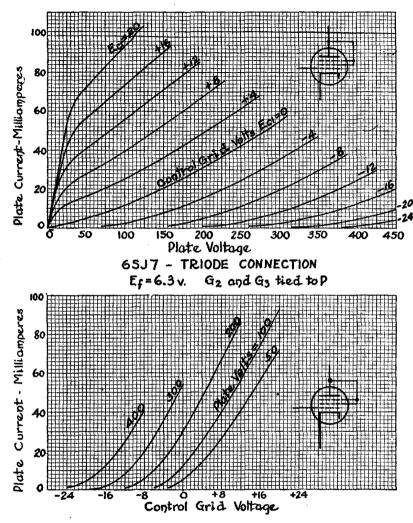
Figs. 12-23 (above), 12-24 (below). The plate and grid families of a 6SJ7 connected as a triode with the screen and suppressor grids connected.
