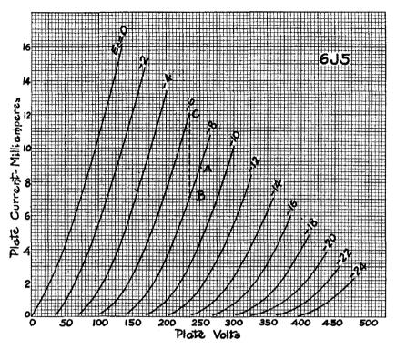
Fig. 8-12. The plate family of a 6J5 triode can also be used for finding the transconductance.
