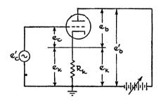
signal voltage applied between grid and ground is designated  $e'_c$  in order to indicate that it is equivalent in nature to the actual instantaneous grid voltage  $e_c$ , but that  $e'_c$  is the instantaneous grid-to-ground voltage, whereas  $e_c$  represents the instantaneous grid-to-cathode voltage. Similarly,  $e'_b$  signifies the instantaneous plate-to-ground voltage, as compared with  $e_b$  which is the instantaneous plate-to-cathode voltage.
