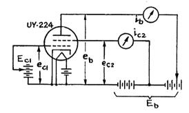
the graph of Fig. 12-6. The tetrode used in this test was the now obsolete filament-type UY-224, because it exhibits certain properties of fundamental interest which later types of tetrodes do not show. Curves for just one control-grid and screen-grid voltage setting are shown in Fig. 12-6 for illustrative purposes: the control-grid voltage  $e_{ct}$  is equal to -1.5 volts and the screen-grid voltage  $e_{ct}$  is equal to +75 volts.
