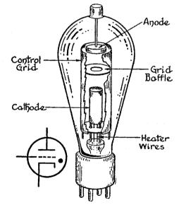
Figs. 15-44 (right), 15-45 (left). The arrangement of the elements of a thyratron tube are shown on the right. The dot in the schematic symbol at the left indicates that the tube is gas-filled.
