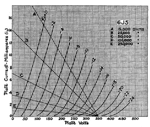
Fig. 9-9. The lines representing different values of load resistance are drawn on the plate family of the 6J5 triode. Note that as the resistance of the load increases, the plate current flowing in the circuit decreases.
