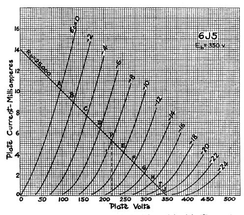
Fig. 9-7. The line superimposed on the plate family of characteristics of the 6J5 represents a 25,000-ohm load in the plate circuit, as shown in Fig. 9-1.
