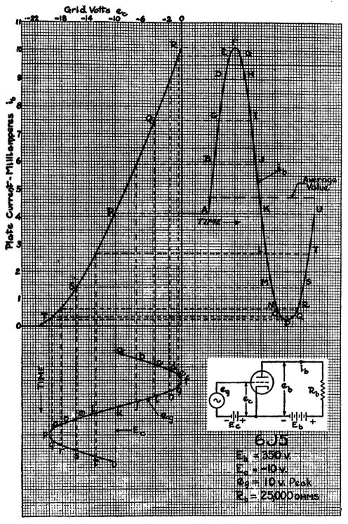
Fro. 10-6. How the plate-current wave is developed using a dynamic transfer characteristic with a sine wave input signal on the grid of a triode.
