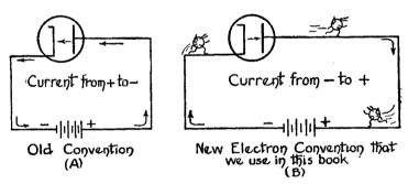
Fig. 6-7. The old convention of current flowing from + to - is illustrated in (A) and the modern convention of current flowing from - to + is shown in (B).
