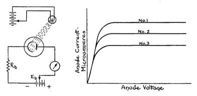
Fig. 15-49. If the anode voltage of a photocell is held constant and the amount of light falling on the cathode is varied, the anode current will change correspondingly. Curve No. 1 in the family of characteristic curves is for the greatest light intensity which is held constant while the anode voltage is increased; curve No. 2 is for less light intensity, and curve No. 3 is for the smallest amount of light intensity.
