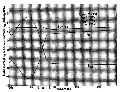
Fig. 12-6. The plate voltage—plate current characteristic curves showing the variations of current flow in the plate and screen-grid circuits, (curves marked  $i_b$  and  $i_{cz}$  respectively) and the total current flow, which is the sum of these two currents.
