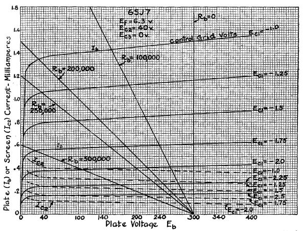
Fig. 12-21. The plate family for a constant screen-grid voltage of 40 volts. Load lines for various values of load resistance are shown, the plate-supply voltage in each case being 300 volts.
