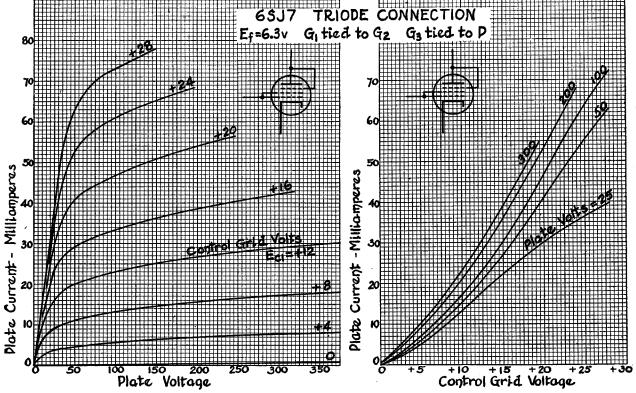
Figs. 12-25 (left), 12-26 (right). The plate and grid families of a 6SJ7 connected as a triode when the control-grid is connected to the screen-grid and the suppressor-grid is connected to the plate.
