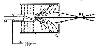
Fig. 15-26. The elements of the electron gun of the cathode-ray tube. The arrows on the dashed lines indicate the direction in which electrons are urged to move by the field, the resulting path of the electrons being indicated by the series of dots.
