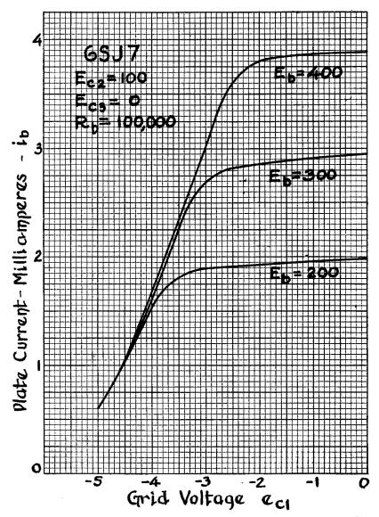
$F_{1G}$ . 12-20. These three dynamic transfer characteristics are derived from the load lines of Fig. 12-19 on the opposite page.
