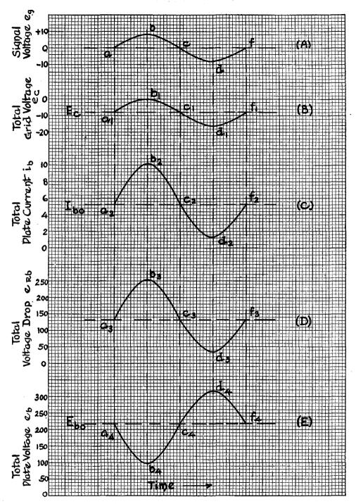
Fig. 11-8. This series of waves shows that the input voltage  $e_{\rm g}$  is in phase with the plate current  $i_{\rm b}$  and that  $e_{\rm g}$  is 180° out of phase with the plate voltage  $e_{\rm b}$ .
