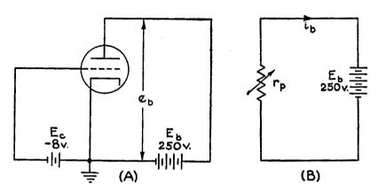
Fig. 9-2. The triode circuit in (A) has no load resistance in the plate circuit  $(R_b = 0)$  and no input signal; compare Fig. 9-1. The equivalent circuit of (A) is shown in (B) where the plate resistance  $r_p$  is shown as a variable resistor.
