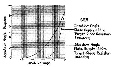
Fig. 15-43. These curves show that the shadow angle of a 6E5 visual indicator tube decreases in width the more negative the grid of the tube is made.
