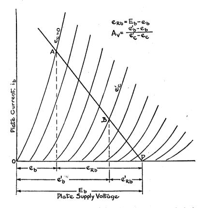
Fig. 11-2. The plate voltage  $e_b$  and the voltage drop  $e_{Rb}$  across the load resistance are indicated on this general plate family upon which any load line has been drawn.
