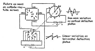
Fig. 15-34. A linear voltage is applied to the horizontal plates and this moves the spot from left to right across the screen; a sine-wave voltage is simultaneously applied to the vertical-deflection plates, thereby resulting in a cycle of the sine wave on the screen.
