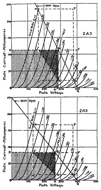
Figs. 14-4 (above), 14-5 (below). In these two and the two graphs on the next page, different load lines are drawn on the plate family of a 2A3 for different values of loads as indicated, in order to indicate the power output and plate dissipation.
