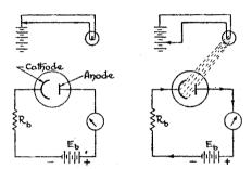
Figs. 15-47 (left), 15-48 (right). When no light energy falls on the cathode of a photocell, no electrons flow through the anode circuit in which is connected the load R<sub>b</sub>. In Fig. 15-48 light is indicated hitting the cathode of the photocell with a resulting current flow through the anode circuit.
