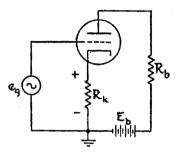
Fig. 13-1. The plate current returning to the cathode passes through the cathode resistor  $R_{\rm k}$  and causes a voltage drop equal to the product of the current and the value of the resistance.
