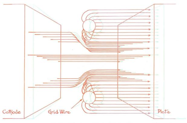
PLATE 3. The arrangement of the lines of force in a triode, in which the grid is negative with respect to the cathode.
