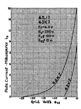
Fig. 15-19. The grid voltage—plate current curve marked 6SJ7 is for a sharp-cutoff pentode and that marked 6SK7 is for a remote-cutoff (variable mu) tube. These show that the 6SK7 can be operated at a grid voltage that is about five times more negative than the other.
