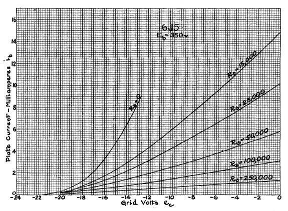
$F_{1G}$ . 9-11. These dynamic transfer characteristic curves correspond to the load lines of Fig. 9-9 for the same operating conditions.
