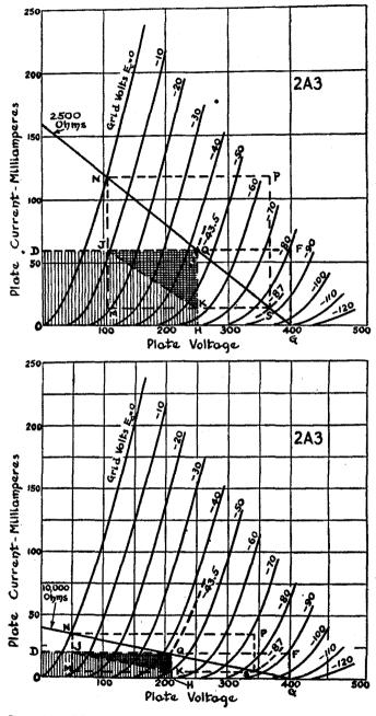
Figs. 14-6 (above), 14-7 (below). In these four sets of curves, observe how the proportion of power output area (QJK) and the plate dissipation area (ODJKH) changes as the load resistance is changed.
