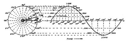
Fig. 10-7. The instantaneous values of a sine wave for every 15° are shown at each division of the positive half-cycle; although not shown in entirety, these values are the same for the negative half-cycle.
