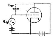
Fig. 12-3. The capacity  $C_{\rm gp}$  existing between the grid and the plate in a triode can be disregarded at low frequencies, but at high frequencies (above 15,000 cycles) this capacity effect interferes with proper operation of the tube. The screengrid of the tetrode greatly reduces this condition.
