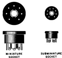
Fig. 12-2. Top and bottom views of miniature and subminiature sockets.
