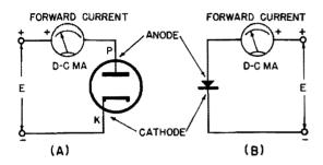
Fig. 12-36. Connection for forward-resistance check of: (A) tube diode, and (B) crystal diode.
