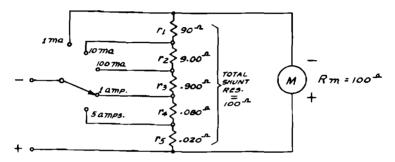
Fig. 8-3. A universal shunt operated by means of a single-gang switch.
