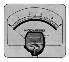
Fig. 1-9. Cutaway view of "taut-band" suspension-type meter. Hickok
