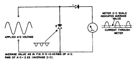
Fig. 6-3. Double-rectifier arrangement, which minimizes "back-current."
