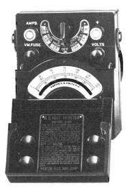
Fig. 8-1. Photos of multi-range instruments with terminals and with switch selector.
