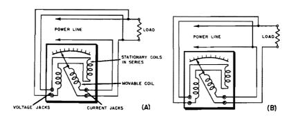
Fig. 5-4. Organization of dynamometer type wattmeter.
