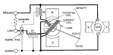
Fig. 4-8. Circuit of c typical megger. The metal guard ring and associated components prevent leakage cur. Its along the surface of the instrument case when readings over 100 megohms are being made.
