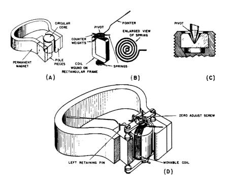
Fig. 1-2. Construction details of a D'Arsonval moving-coil mechanism.
