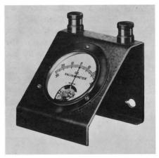
Fig. 1-5. A Weston center zero galvanometer.
