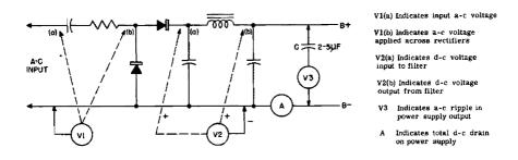
Fig. 12-24. Selenium rectifier power supply (full-wave voltage doubler).
