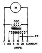
Fig. 8-5. Circuit of multi-range a-c ammeter with tapped current transformer.
