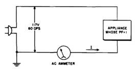
Fig. 5-3. Diagram of arrangement which measures power with an ammeter providing the voltage is constant and the power factor of the load is 1.
