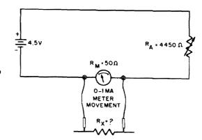
Fig. 4-4. Circuit of shunt type ohmmeter.
