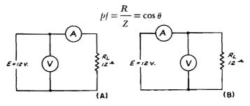
Fig. 5-2 If the ammeter A is connected as shown in A at the left, only the current drawn by the load  $R_{\rm L}$  will be indicated on it; if it is connected as in B, right, then the ammeter reading will be the current drawn by both the load and the voltmeter, V.
