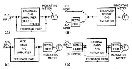
Fig. 9-25. Main VTVM circuit types: (A) multistage d-c amplifier; (B) rectifier plus d-c amplifier; (C) multistage a-c amplifier plus rectifier; (D) d-c modulated type.
