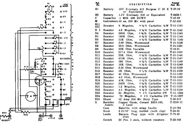
Fig. 8-11. Schematic of Triplett Model 630A VOM.
