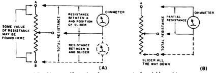
Fig. 12-7. Diagrams illustrating the measurement of variable resistors.
