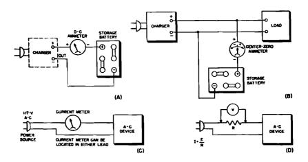
Fig. 11-3. (A) An ammeter connected to indicate rate of battery charge. (B) A centerzero meter used as a charge-discharge instrument. (C) and (D) Ammeter and voltmeter connected to measure current drain and power of device operated from the power line.
