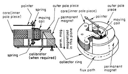
Fig. 1-8. Construction detail sketch of 250°-arc meter. Westinghouse
