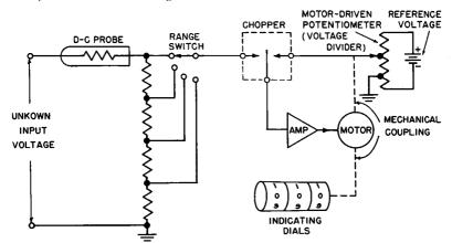
Fig. 14-11. Simplified diagram of servo-motor action in d-c circuit of digital VTVM.
