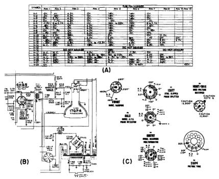
Fig. 12-11. Forms of service information: (A) voltage chart; Emerson (B) Partial schematic showing operating voltages next to tube electrode symbols; RCA (C) Voltage labels adjacent to socket terminals or underside of chassis.
