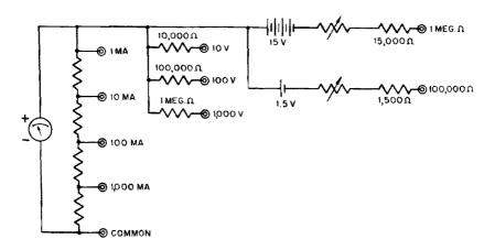
Fig. 8-9. Circuit of combination multi-range d-c voltmeter and current meter used by Armed Forces.
