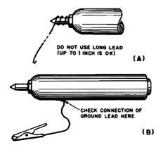
Fig. 10-6. (A) Addition of a piece of wire to the tip of the r-f probe may introduce error.
