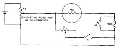
Fig. 3-10. Method for determining meter resistance.
