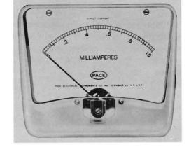
Fig. 1-4 The linear scale used with a typical moving-coil meter (0 1 ma). Pace Elec. Inst., model 45P, (clear acrylic case)
