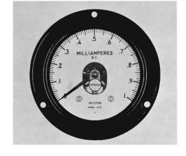
Fig. 1-6. Long-arc (250°) meter scale. Weston
