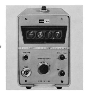
Fig. 14-12. All-electronic digital VTVM. Kintel model 801
