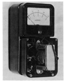
Fig. 8-4. Internal view of Simpson a-c current meter with current transformer.
