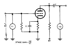
Fig. 12-31. Arrangement for measuring stage gain of an a-f amplifier using a-c meter of suitable type.
