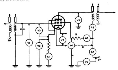
Fig. 12-14. A pentode transformer-coupled amplifier stage, showing locations for current and voltage readings. In a triode stage, readings are the same except that those connected with the screen grid and suppressor grid circuits are eliminated.
