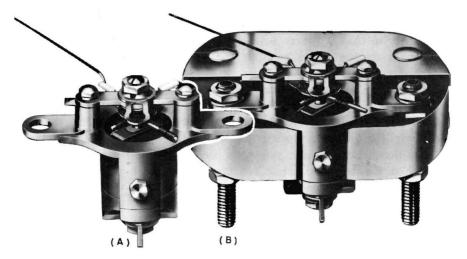
Fig. 1-3. Assembly of commercial moving-coil meter: (A) full double-bridge suspension of D'Arsonval movement; (B) movement assembled on permanent magnet without scale.
