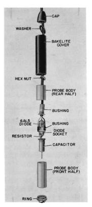
Fig. 9-19. Disassembled RCA duo-diode probe used for measurements from audio frequencies up to about 250 mc.
