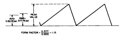
Fig. 6-9. Sawtooth waveform and relative value of the rms and average compared to peak. The form factor here is 1.15, compared with 1.11 for the sine wave.
