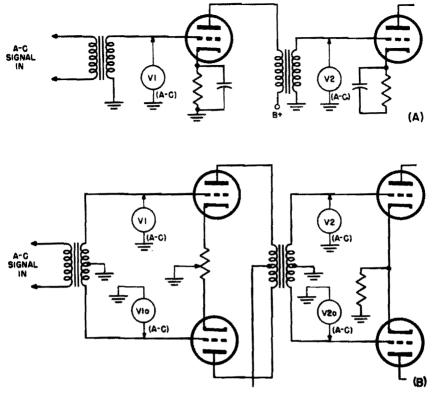
Fig. 12-32. Measuring gain in transformer-coupled amplifier.
