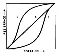
Fig. 12-8. Resistance variation and application of various tapers in volume controls.
