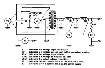
Fig. 12-25. Full-wave synchronous vibrator power supply.
