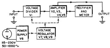
Fig. 14-1. Block diagram of a-c amplifier type VTVM. Hewlett-Packard model 400D
