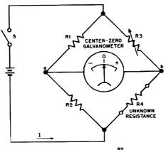
Fig. 11-4. Wheatstone-bridge circuit for measuring resistances.
