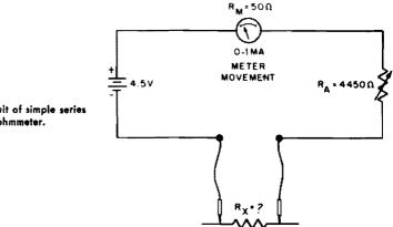
Fig. 4-2. Circuit of simple series type chameter.
