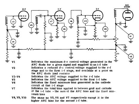
Fig. 12-18. Examples of d-c control valtage measurements in radio receiver.
