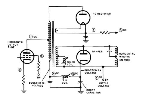
Fig. 12-27. Typical horizontal autput system and high-voltage supply.
