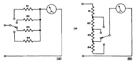
Fig. 3-6. Switch control of multi-range voltmeter amplifier (A) in individual multipliers,
