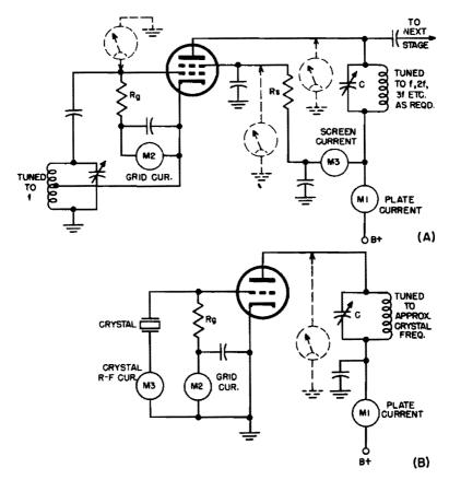
Fig. 13-1. Oscillator circuits: (A) electron coupled circuit such as is used for the frequency-controlling circuit of transmitters, and locations of typical meter measurements;
