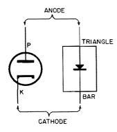
Fig. 12-35. Crystal-diode symbol corresponding to tube-diode symbol.
