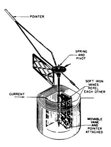
Fig. 2-4. Details of construction of the radial-vane type of moving iron meter.
