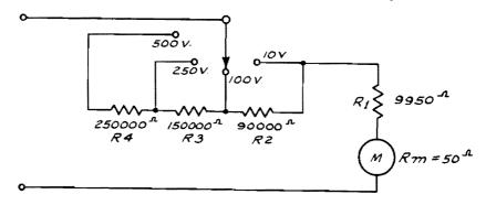
Fig. 8-7. Switching system for series connected voltmeter multipliers, using 50  $\mu$ a meter for 500-volt maximum scale.
