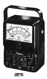
Fig. 8-10. Multi-range and multi-function VOMs: Triplett model 630A and Simpson model 260.
