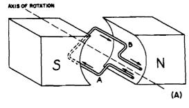
Fig. 1-1. Illustration of the basic motor principle employed in moving-coil permanent-magnet
