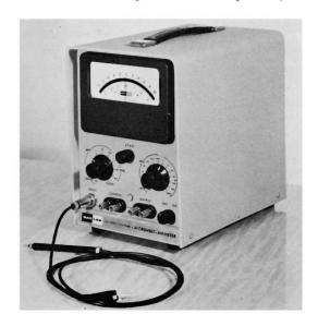
Fig. 14-8. D-c chopper-modulated microvoltmeter. Key Lab (Kintel) model 203
