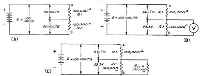
Fig. 3-12. Effect of voltmeter resistance on circuit resistance: (A) with voltmeter not present; (B) with voltmeter connected across R2; (C) equivalent circuit of B with voltage connected across R2 shows how the voltage drops across R1 and R2 are changed from those shown without the voltmeter.
