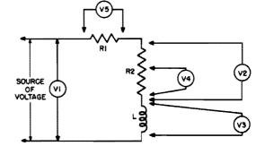
Fig. 3-11. Application of voltmeters for voltage measurement.
