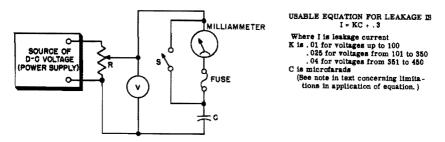
Fig. 11-8. Arrangement for measuring leakage current of capacitors.
