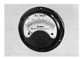
Fig. 6-12. Logarithmic scale, Ballantine a-c electronic voltmeter model 300
