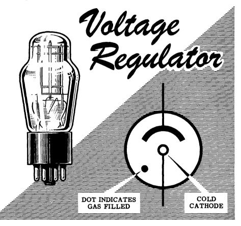
When a large enough potential is applied between the cathode and the plate, the gas in the tube conducts and electrons flow from cathode to plate. Conduction is characterized by a bluish glow inside the tube—the heavier the conduction the brighter the glow.
