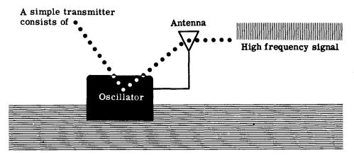
If your home radio set picked up the constant-amplitude signal from such a transmitter, you would hear nothing at all. If a special type of radio received this signal, a constant audio tone would be heard. In either of these cases, no message could be "read" from the incoming signal—such a signal is said to contain "no intelligence." To add intelligence to the signal, the oscillator would be turned on and off with a key to produce dots and dashes.
