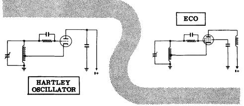
The oscillator section of the electron-coupled oscillator may be a Colpitts circuit instead of a Hartley circuit with equally satisfactory results. The "electron-coupling" effect refers to how energy is delivered from oscillator to plate circuit, not to how the oscillations are generated.
