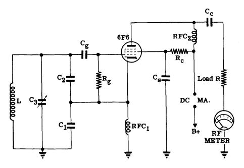
A pentode connected as a tetrode is used in place of the triode of the Colpitts oscillator. The cathode, control grid and screen, along with the tank circuit, act as a conventional Colpitts oscillator. The screen RF by-pass capacitor,  $C_g$ , shields this triode from the plate and supplies feedback across  $C_1$ , the AC screen grid load.
