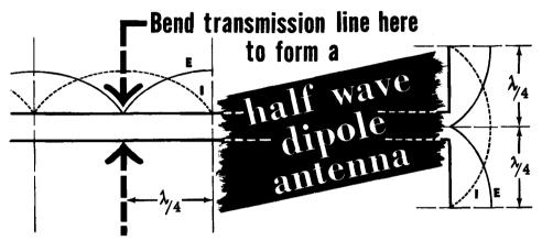
Although the voltages at any two points on the antenna wires (also on the transmission line), equidistant from the ends, are equal in amplitude, they are opposite in polarity just as the ends of a transformer winding are equal in amplitude but opposite in polarity. The same holds true for current. Therefore, to indicate polarity as well as amplitude on the wires that comprise the transmission line and antenna, the wave forms are redrawn as shown.
