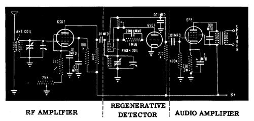
TRF RECEIVER WITH A REGENERATIVE DETECTOR
