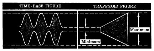
The two 'scope presentations shown above are for the same condition of modulation. You could determine the maximum height (peak) and the minimum height (trough or valley) of the RF from either figure. You could also determine the linearity of the modulation from either presentation, but it is easier to do so from the trapezoid.
