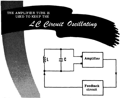
All the oscillators you will learn about in this section operate on the principle illustrated above. The major difference between various oscillators is the method in which a voltage is fed back to the LC circuit in proper phase. You will learn about six basic oscillators: the Armstrong, the Colpitts, the Hartley, the tuned-plate—tuned-grid, the crystal controlled and the electron-coupled oscillators. You will see how these oscillators work, and the advantages and disadvantages of each type.
