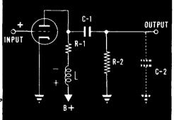
When the grid voltage swings negative, as at (b), the plate current decreases and the back emf across L is in the opposite direction. This then adds to the plate voltage—normally high anyway—causing another peak to appear at (b). Because of the effect of this inductance, it is always referred to as a peaking coil."
