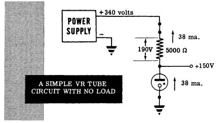
Suppose you attach an 8 ma. load to the 150 volt terminal. Of the 38 ma. flowing through the dropping resistor, 8 ma. flows through the load and 30 ma. flows through the VR tube. Since the VR tube current is yet within the rated range of 5 to 40 ma., the VR tube adjusts its internal resistance so that the plate voltage remains at 150 volts.
