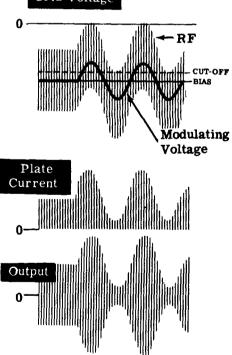
Grid modulation is used in compact or mobile transmitters because this type of modulation does not require a modulator with a large power output. When the modulator's weight is only a minor consideration, plate modulation with the larger modulator it requires is used because it produces much better results than grid modulation.
