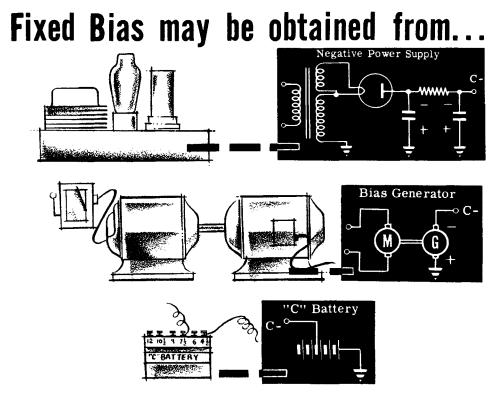
One of the advantages of fixed bias is that the tube remains cut off under no signal conditions.
