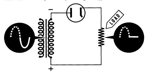
The diode rectifier tube, by allowing electrons to flow through it in only one direction (from cathode to plate), causes pulses of current to flow through the load and, therefore, causes a pulsating DC voltage to appear across the load. The AC voltage input from the transformer appears as a pulsating DC voltage across the load. Notice that the half-wave rectifier has used only the positive half of the AC input. The negative half is not used at all.
