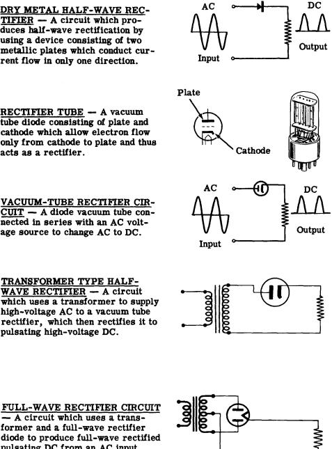
**RECTIFIER TUBE** — A vacuum tube diode consisting of plate and cathode which allow electron flow only from cathode to plate and thus acts as a rectifier.
