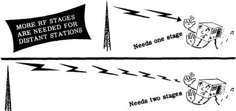
There is a second, and less obvious, reason for using more than one RF stage. More than one RF amplifier stage gives greater selectivity. More selectivity permits a receiver to separate stations whose frequencies are very close together. There are radio frequency bands in which many stations are crowded into a few megacycles. Receivers designed to cover these bands need more selectivity than one tuned RF amplifier can give them.
