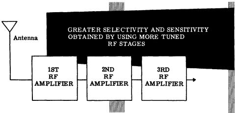
Since the RF amplifier stage is designed primarily for voltage amplification, any tube suitable for voltage amplification may be used. However, triodes are not considered satisfactory because they have a strong tendency to produce undesirable oscillations when employed in RF amplifier stages. Unless the triodes are carefully neutralized to prevent feedback, the oscillations produced are likely to cause considerable trouble.
