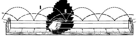
Both voltage and current peaks can be shown by using a long fluorescent light. The light areas are voltage peaks or current nulls.
