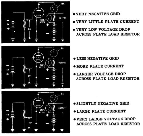
Using this circuit with certain types of vacuum tubes, the change in plate voltage can be made more than 200 times the change in grid voltage—a voltage gain or amplification of over 200.
