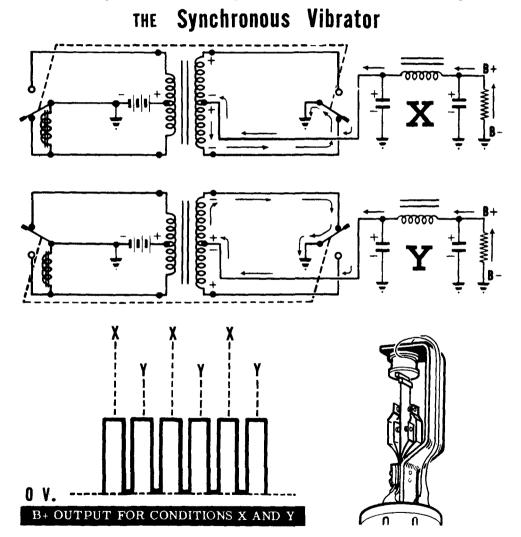
The two vibrating reeds shown connected together by the dotted line in the diagram are actually one reed placed between two pairs of contacts. The action of the reed between the transformer secondary contacts produces the same results as a full-wave rectifier. RF chokes and buffer condensers are used in this vibrator circuit in the same manner as in the non-synchronous vibrator to eliminate contact sparking and radio interference.
