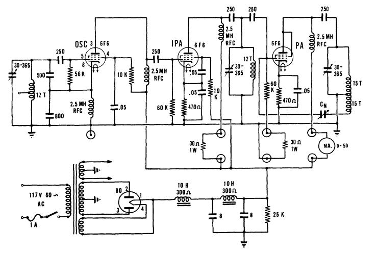
**Complete Diagram of a Three Stage Transmitter**
