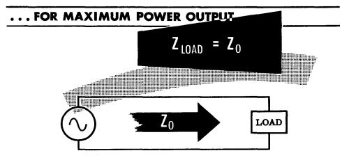
An example of getting maximum power transfer from a transmission line to a load is the case of a line feeding an antenna. If a certain type of antenna, called a half-wave dipole," is used, the impedance at its center feed point is 73 ohms. Therefore in order to get maximum power transfer from the transmission line to the antenna, the characteristic impedance of the line should be 73 ohms or close to it. When this is the case, the line is said to be "matched" to the antenna.
