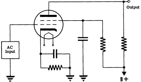
With AC on the control grid of the tube, the plate voltage will vary because of the drop in the load resistor just as in the triode. When the tetrode is used for getting large amplifications, the plate voltage varies over a wide range and, if it drops below the screen grid voltage, secondary emission effects cause distortion in the output.
