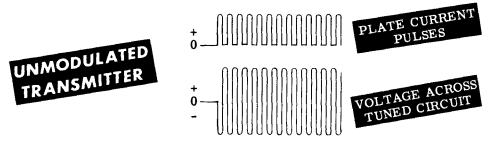
When the transmitter is modulated, the amplitude of the plate current pulses is made to vary according to the amplitude of the modulating signal. Thus the amplitude of the RF current varies from one cycle to the next and the power delivered to the tuned circuit also varies. This varying power causes the RF voltage across the tuned circuit to vary. These variations will follow the modulating signal in amplitude and frequency. This is how modulation is accomplished.
