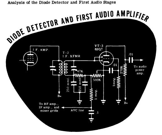
The two 250-mmf capacitors function as the detector filter capacitors. Their purpose is to bypass the IF component of the signal to ground around the 47K and 500K diode load resistors. The 47K resistor is part of the filter network, while the 500K potentiometer also acts as a bleeder resistor across the filter. It controls the amount of detector output delivered through the .01-mfd coupling capacitor to the grid of the first audio amplifier and thus serves as a volume control.
