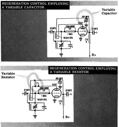
In the detector shown above, regeneration is controlled by a variable resistor placed across the tickler coil.
