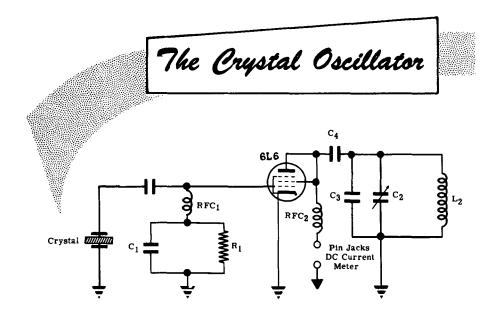
C<sub>3</sub> in parallel with C<sub>2</sub> adds to its capacity and reduces the resonant frequency. This is required if the range of  $C_2L_2$  alone does not extend down to the crystal frequency.
