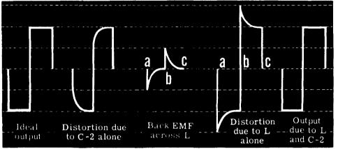
To improve the steepness of the steep portion of the square wave, an inductance (L) is placed in series with the plate load resistor (R-1). The back emf set up in this inductance every time the plate current changes will be in such a direction as to cause a peak to appear in the plate voltage.
