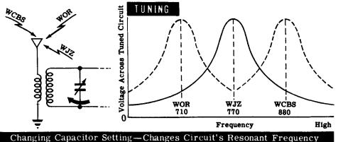
One particular coil and one particular capacitor will resonate to one frequency only. Varying either the inductance or the capacitance of the tuned circuit will change the resonant frequency. In the process of tuning, you can change the capacitance of the tuned circuit by using a variable capacitor. When the resonant frequency of the LC circuit coincides with the frequency of some signal, you have tuned the RF amplifier to that signal.
