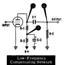
At (b), the current suddenly decreases and the voltage at point 1 rises as the condenser C-3 charges up. Thus between time (b) and time (c), the plate voltage is increasing.
