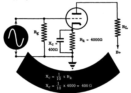
Since  $X_c = \frac{1}{2\pi fC}$ , the capacity of the bypass condenser can be found by using the formula  $C = \frac{1}{2\pi fX_c}$ , where f is the lowest frequency signal to be amplified. Suppose f is 60 cps and  $X_c$  is 400 $\Omega$  as shown above, then C will be  $\frac{1}{6.28 \times 60 \times 400} \approx 6.6$  mfd.
