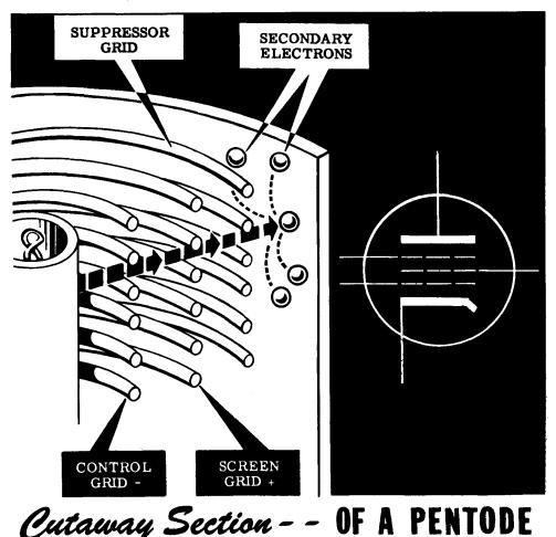
The suppressor grid is usually kept at cathode potential so that it is always very negative with respect to the plate. Therefore, any electron that is in the region between the suppressor and the plate (such as a secondary electron) is attracted back to the plate and prevented from getting through the suppressor to the screen. As a result of this arrangement, secondary emission does not affect the operation of the pentode.
