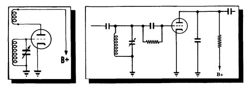
An Oscillator + A Grid-Leak Detector
