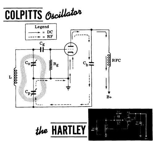
The DC current path is: electron flow from cathode to plate, through the RF choke to B+, through the power supply to ground, back to cathode.
