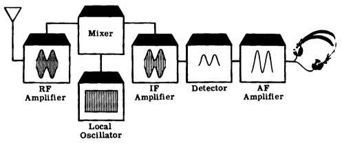
The process of mixing or beating two frequencies together to get a difference frequency is called "heterodyning." That is why the receiver was named superheterodyne.
