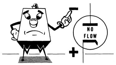
You know from your previous experiment with a diode that when the tube is connected across the 60 cycle power line the diode plate becomes positive 60 times per second and negative 60 times per second. Connecting the diode to the high voltage winding of a transformer keeps the situation exactly the same except that the voltage put on the plate is much higher, and the resulting pulsating DC is at a correspondingly higher voltage. The Diode in a Transformer Type Circuit (continued)
