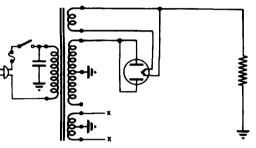
CURRENT FLOW IN A HALF-WAVE RECTIFIER CIRCUIT -AC is applied to the rectifier plate and current flows only during those half-cycles which are positive on the plate side of the circuit input.
