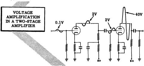
Suppose each amplifier stage can deliver an amplification of 20. If a 0.1 volt AC signal is applied to the grid of the first stage, the output of this stage will be  $20 \ge 0.1 = 2V$ . Since the output of the first stage is connected to the input of the next stage there will be 2 volts AC on the grid of the second stage. The second stage amplifies the signal 20 times and produces an output voltage of  $20 \ge 2 = 40V$ .
