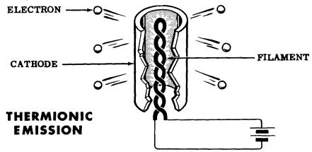
Some tubes such as the Fleming's Valve or the type 80 rectifier tube have what is known as directly heated cathodes, which means that there is no sleeve around the filament and the filament is itself the electron emitter.
