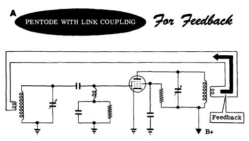
With sufficient coupling, feedback energy will compensate for resistance loss in the grid tank and oscillation will continue.
