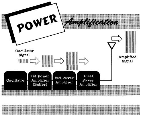
The RF signal is generated in the oscillator circuit and is amplified by the first and second power amplifiers which drive the final power amplifier. The powerful signal from the final power amplifier is fed to the antenna which radiates the signal into space.
