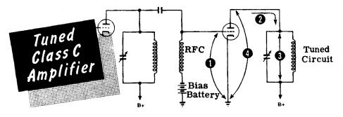
The operation of a Class C amplifier will become clear when you analyze what happens in a tuned amplifier such as the one shown in the schematic diagram. An AC signal is developed across the tuned circuit in the plate of the previous stage. This voltage also appears across the RF choke (RFC) in the grid circuit of the tuned Class C amplifier stage. The DC bias provided by the bias battery causes the tube to operate Class C.
