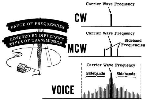
There are many different circuits which are used to obtain CW transmission. They look different and operate differently, but each has the same purpose—to turn the RF of the transmitter on and off. You will learn about some of these circuits on the next few sheets. In the next topic, you will find out more about MCW and voice transmission.
