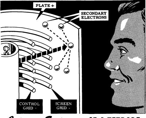
Cutaway Section - - OF A TETRODE
