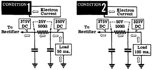
Similarly a change of 100 ma. in the load current will cause the B+ voltage to drop 50 volts. Such a rise and fall in output voltage is very undesirable in electronic equipment. Voltage regulator circuits might be added to compensate for this voltage change due to the filter resistor, but it would require a large and expensive circuit to compensate for changes such as are indicated here. Using a Choke Instead of a Resistor
