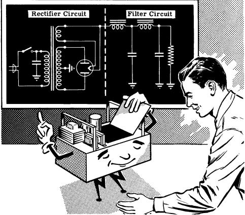
You already know that there are only two types of rectifier circuits in general use—the full-wave and the half-wave rectifiers—and they both perform the same job of changing AC into pulsating DC. There are only three types of filter circuits that are in general use. These filter circuits all have one thing in common—they remove the ripple from the pulsating DC output of the rectifier.
