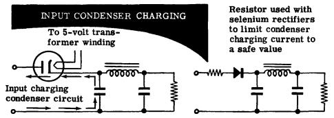
Because of the time lapse between pulses of direct current, the output of a half-wave rectifier requires more filtering than that of a full-wave rectifier and the filtered output voltage will be lower. Filter condensers used in half-wave power supplies are usually from 2 to 4 times as large as those used in full-wave power supplies. Increasing the size of the filter condensers provides additional filtering.
