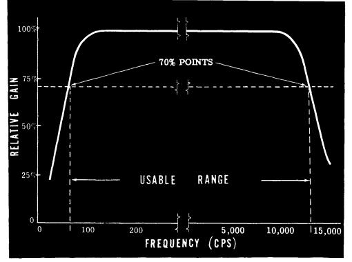
The general shape of the curve shows a flat region (plateau) between the ends of the curve. This means that the gain does not vary by very much as the frequency changes from the low end to the high end of this portion. This represents the usable frequency range of the amplifier.
