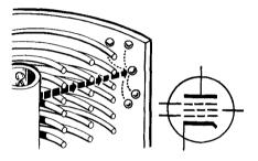
THE BEAM POWER TUBE — Tube using beam-forming plates instead of the suppressor to reduce the effects of secondary emission. Its power output is greater, for a given amount of cathode emission, than that of a pentode.
