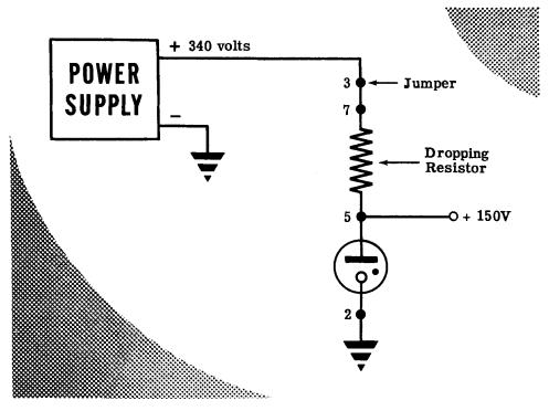
Note that the 150 volt point is disconnected from the power supply if the VR tube is pulled out.
