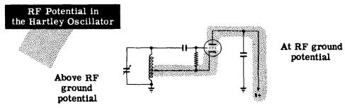
There is a capacitor between the plate of the Hartley oscillator and ground. This capacitor offers a very low impedance path for RF. Since it goes to ground, the plate is considered at RF ground potential, even though it is at a high DC potential.
