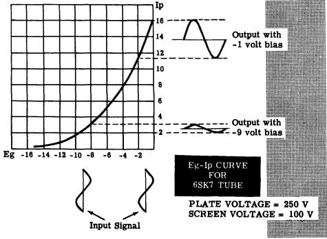
In a remote cut-off pentode the turns of the control grid are spaced closely at the edges and farther apart at the center. The electron flow through the edges of the grid is cut off by very little negative bias. However the electron flow through the center of the grid can only be cut off by a high negative bias. The grid of a sharp cut-off pentode is uniformly spaced. The entire plate current is cut off by one value of bias.
