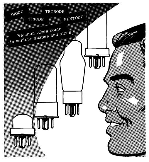
Their names describe them by telling how many parts (cathode, grid, plate) there are in the tube. A diode (di = two) has two parts—a cathode and a plate. A triode (tri = three) has three parts—a cathode, a plate and one grid. A tetrode (tetra = four) has four parts—a cathode, a plate and two grids. A pentode (penta = five) has five parts—a cathode, a plate and three grids.
