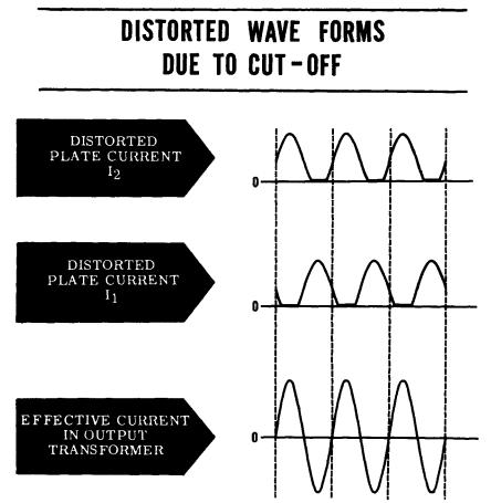
The reason that it is such a big advantage that the push-pull circuit reduces distortion is this—the tubes can be intentionally overdriven to produce a larger output and the output still will be practically undistorted.
