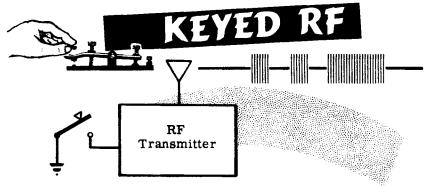
The simplest and most commonly used method of obtaining CW transmission is by "cathode keying." In this type of circuit, the key is connected in the cathode's DC return to ground. Thus, when the key is opened, no current can flow and no RF can be radiated from the antenna. When the key is closed, the circuit operates normally. The stage that is usually keyed in this manner is the master oscillator itself or the master oscillator plus one or more of the following amplifier stages.
