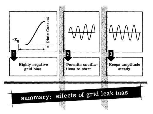
Grid leak bias has one disadvantage. If oscillations should cease, even momentarily, the high negative grid bias would be lost. A large flow of electrons from cathode to plate would occur. This average plate current flow would be so large as to damage or ruin the vacuum tube. Frequency Instability
