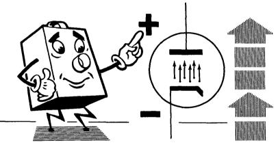
2. The diode does not allow electrons to flow through it when the plate is negative with respect to the cathode.
