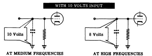
The solution to the problem of loss of gain at high frequencies is to use special amplifier tubes with very low values of input and output capacitances, to use special wiring techniques to reduce the stray capacitance between the wire and ground, and to use lower values of resistors in the RC coupling. These methods increase the frequency at which the shunting effect becomes noticeable.
