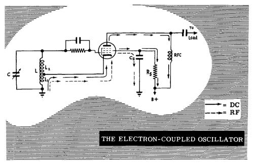
You can see that this is a modified Hartley oscillator. The modification consists in the replacement of the triode by a tetrode, which has an additional element, the screen grid.
