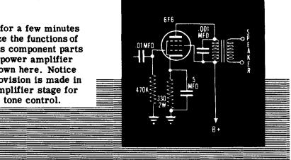
The 0.01-mfd coupling capacitor and 470K grid resistor found in the control grid circuit couple the control grid of the amplifier to the preceding detector stage. The capacitor also reduces the possibility that any DC voltages from the detector stage might be impressed upon the control grid of the amplifier.
