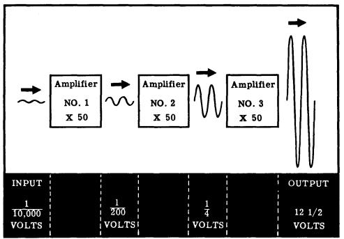
Since nearly all amplifiers require more amplification (gain) than can be achieved with only one tube, multi-stage amplifiers of this type are very common in all types of electronic equipment.
