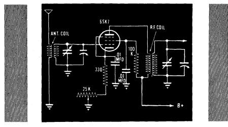
Since signals arriving from different transmitters will vary in intensity, it is necessary to provide a volume control so that the gain of the RF amplifier and the loudness of the signal can be varied. One of the most common methods of controlling the gain of a TRF is to change the bias voltage of the RF amplifier stage by placing a variable resistor in the cathode circuit.
