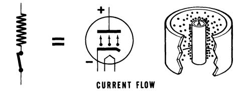
When the plate becomes the least bit negative with respect to the cathode, no electrons will flow from the cathode to the plate. The tube acts as if it were a resistor in series with a switch and the switch were opened up.
