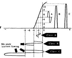
TUNED CLASS C AMPLIFIERS— Used in transmitters because they are very efficient when tuned to the frequency of the input signal.
