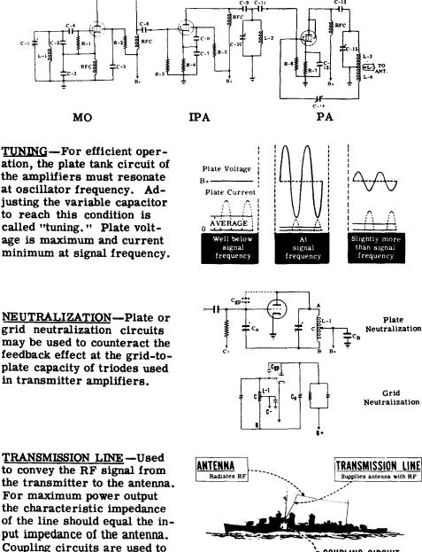
COUPLING CIRCUIT Couples RF from tank circuit to transmission line
