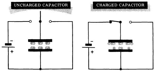
When a short circuit is put across the charged capacitor, the excess electrons are attracted through the shorting wire onto the positive plate. Each plate once more has an equal number of positive and negative charges and the capacitor is uncharged.
