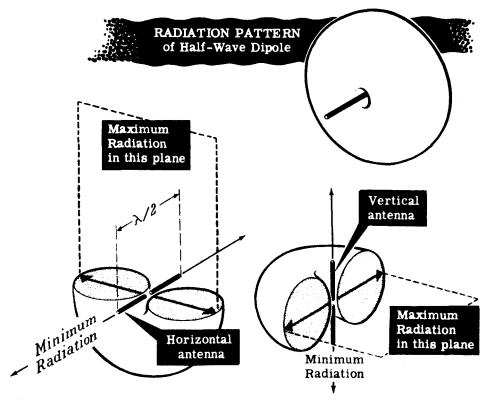
The above radiation patterns assume that the antenna is isolated in space away from all grounds. In actual practice, the antenna is located near ground surfaces so that the radiation pattern is altered appreciably from that shown above.
