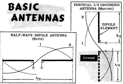
When a Marconi antenna is used, the earth directly beneath the antenna must be a good electrical conductor. Sometimes copper tubing is driven into the ground at the base of the antenna to improve the ground conductivity. On shipboard a vertical quarter-wave antenna may be some distance above the deck. A simulated ground is provided by using grounded metal rods at least a quarter wavelength long and placing them at the base of the antenna. This simulated ground is called a "counterpoise."
