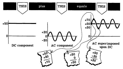
When the +20 volt AC peak is added to the +50 volts DC, the result is +70 volts. When the 0 volt point on the AC wave is added to the +50 volts DC, the result is +50 volts. When the -20 volts AC peak is added to the +50 volts, the result is +30 volts. The total result is a DC voltage which varies from +50 volts—up to +70 volts and down to +30 volts. The voltage of the resulting wave never becomes negative and yet it consists of an AC component and a DC component.
