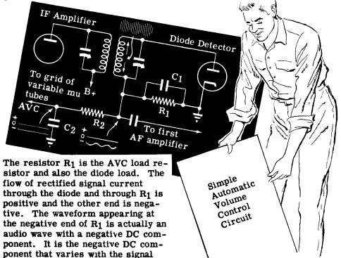
strength. The AVC filter circuit, consisting of  $R_2-C_2$ , filters out the audio and  $C_2$  charges up to the negative DC component. It is this negative voltage that is applied through the AVC line to the grids of the variable-mu tubes in the preceding stages.
