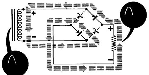
Then, when the AC voltage input swings negative, current flows through the other pair of dry metal rectifiers and the load. Notice that the current flow through the load is in the same direction during both half-cycles of the input wave. Therefore, the voltage developed across the load is pulsating DC which can, of course, be filtered just as any other pulsating DC output from a rectifier circuit.
