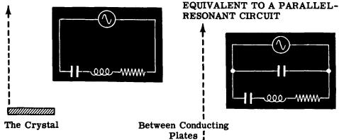
Taken by itself, the crystal acts like a series-resonant circuit. Together with its two plates, it acts like a parallel-resonant circuit. The frequency at which it vibrates depends on its thickness. Thick crystals vibrate slowly, thin crystals vibrate rapidly.
