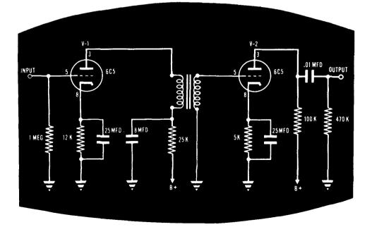
On the next sheet, a signal will be traced through the transformer-coupled amplifier and you will see how amplification occurs in this circuit.
