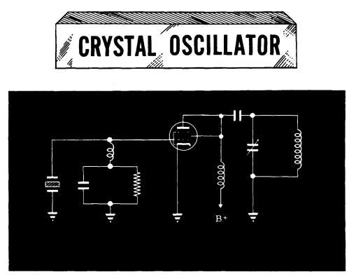
This circuit behaves like the TPTG oscillator in every respect. Feedback is obtained through the plate-grid capacity of the vacuum tube or by using a small feedback capacitor. This voltage feedback causes the crystal to vibrate mechanically at its natural frequency. When the crystal vibrates, an emf appears across the electrodes on the two faces of the crystal. This emf is applied to the grid. The changing emf on the grid controls the flow of plate current and hence the amount of feedback.
