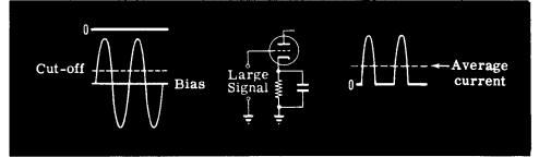
This effect of bias varying with signal strength tends to stabilize the amplitude of that portion of the grid signal above the cut-off level. As a result the amplitude of the current pulses in the plate will not vary as much as their corresponding grid signals vary. Because of the above mentioned effect, self-bias tends to produce amplitude stability of the plate signal and, therefore, is sometimes called "automatic bias." Cathode bias is not common in high-powered transmitter circuits.
