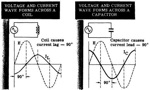
If you connect a coil in parallel with a capacitor, the current in the coil is 90 degrees behind the applied voltage plus 90 degrees behind the current in the capacitor, or, a total of 180 degrees out of phase with the capacitor current. You remember from Basic Electricity that currents which are 180 degrees out of phase cancel one another. If the capacitor alone draws 3 amps and the coil alone draws 2 amps, then the combination of the two will draw 3-2 or 1 amp.
