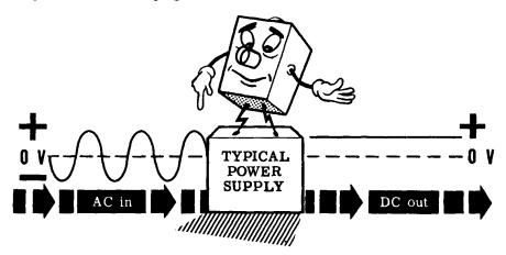
The reason why different types of power supplies are required is simple. One power supply you may build would go up in smoke if you drew much more than 150 ma. of current from the high DC voltage supply. Certain types of transmitters require as much as 5,000 or 10,000 ma. from their power supplies. Certain special oscilloscope circuits may require a DC output of 10,000 volts or more.
