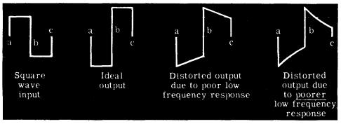
This is what happens in the amplifier. During the flat portion of the square wave between time (a) and time (b) the grid voltage, the plate current and the plate voltage remain constant. At time (b), the grid voltage drops suddenly to a new value and the plate voltage rises just as suddenly to its new value.
