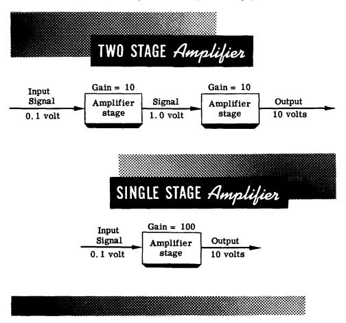
When an amplifier builds up the voltage 10 times, it has a voltage gain of 10. The voltage gain is the number of times a stage or group of stages amplifies the signal.
