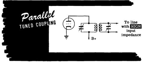
If the input impedance of the line is other than pure resistive, either of the above two tuned coupler circuits can be adjusted so that the reactance of the line is cancelled by the reactance of the tank circuit. This results in a pure resistive load, which is the requirement for maximum power transfer. **Transmission Lines**
