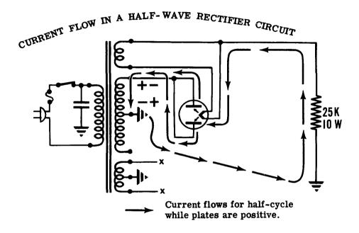
The .001 mfd. capacitor used does not effect the circuits basic operation as a half-wave rectifier. This condenser is connected between one side of the AC power line and ground to reduce electrical interference and prevent such interference from passing through the rectifier circuit. Capacitors used for this purpose may be connected in any of the ways illustrated below.
