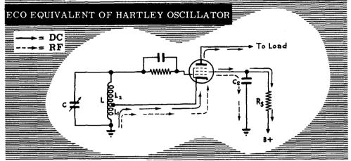
From the diagram it can be seen that both DC and RF paths are identical with DC and RF paths in the Hartley oscillator.
