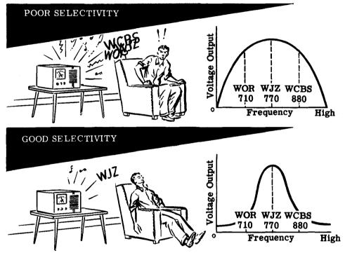
The selectivity of an RF amplifier is determined by its tuned circuits. The lower we can make a coil's resistance in proportion to its reactance, the more selective it will be. The measure of a coil's selectivity is "Q," which is equal to its reactance divided by its resistance. Since the resistance of a capacitor is lower than that of a coil, the coil is the weakest link in a tuned circuit. The Q of the tuned circuit is the Q of the coil.
