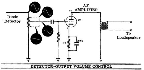
Notice that the detector is coupled to the AF amplifier by means of resistance-capacity coupling circuit. The volume control is basically a voltage divider, the moving arm tapping off the desired amount of signal voltage which is then applied, through the coupling capacitor, to the grid of the AF amplifier. This type of volume control is frequently employed in superhet receivers.
