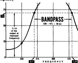
ALIGNMENT — The process of adjusting trimmers in a group of tuned amplifier stages so that all the stages tune to the same frequency. When a multiple-stage RF amplifier is correctly aligned, it will give more selectivity than a singlestage amplifier. When it is not correctly aligned, it may give far less selectivity or even tune to two frequencies at once.
