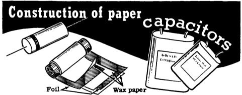
Paper condensers are not polarized and when operated within their voltage rating they last much longer than electrolytic condensers. However, large sizes of paper condensers are bulky and relatively expensive. They are normally not made larger than 16 mfd.
