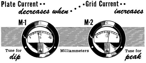
If the grid circuit has fixed bias or combination bias, no grid current will be drawn until the signal is fairly large. This will happen some time after the plate current meter has started to dip. For this reason, the rising grid current indication is sharper than the decreasing plate current indication.
