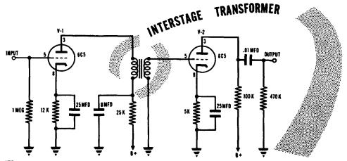
The reasons why transformer coupling is not widely used are, first, that a transformer usually has a poorer frequency response than an RC network. Modern high gain tubes cancel any advantages that the transformer has in voltage amplification. In spite of improvements in the design of interstage transformers, the trend is toward using high gain vacuum tubes with RC rather than transformer coupling between the stages of the amplifier.
