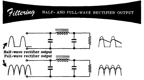
The higher the frequency of the AC input voltage to a power supply the lower the value of the filter condensers required. The time between pulses is shorter at higher frequencies and the inductive action of the choke is greater at higher frequencies.
