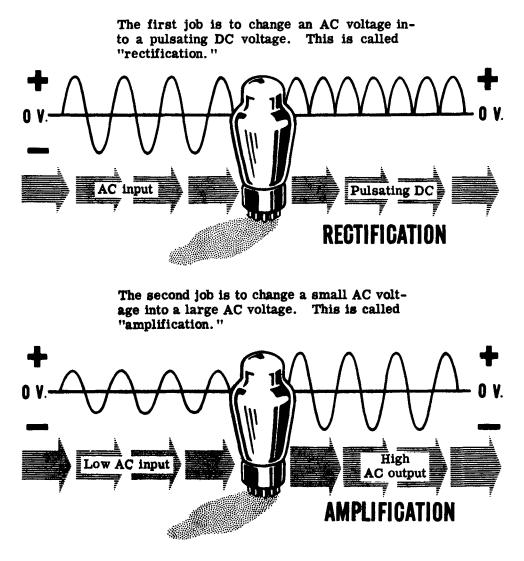
Because of your work with rectifier and power supply circuits, you now know all you need to know about rectification and the diode tubes that are used to do this job. Now you are ready to learn about the second main job a vacuum tube can do—amplification. In this section you will learn about the vacuum tubes that do the job of amplifying small AC voltages into large AC voltages. Types of Vacuum Tubes
