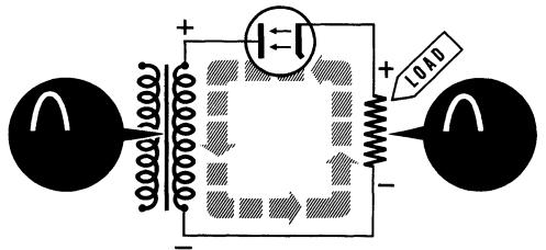
When the transformer voltage makes the rectifier tube plate negative, electrons cannot flow and, of course, no voltage can appear across the load.
