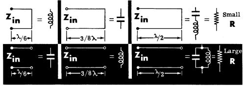
It is obvious from the above diagrams that the terminal conditions at the end of the line are the only factors which determine the type and magnitude of the input impedance at any point along the line.
