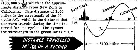
Similarly the wavelength of any frequency radiation can be determined by multiplying the constant velocity by the time for one cycle. Since the time for one cycle is equal to 1 divided by the frequency  $(\frac{1}{4})$ , the wavelength equals constant velocity over frequency  $(\lambda = \frac{V}{\epsilon})$  or the velocity equals the frequency times the wavelength ( $V = f\lambda$ ). Since V is constant, the higher the frequency, the lower the wavelength and vice versa.
