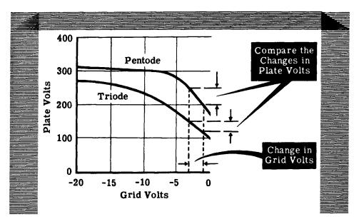
With a larger load resistor in the pentode circuit, larger amplification is obtained. This happens because the grid voltage, and only the grid voltage, can produce a change of current. This current will flow through the load resistor—the larger the resistor, the larger the voltage change.
