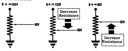
You can see that the hand-operated voltage regulator works very well. You increase or decrease the resistance between ground and the output voltage tap to increase or decrease the output voltage back to the desired value whenever the B+ supply voltage falls or rises for any reason.
