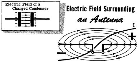
Besides this electric field, there is also a magnetic field which is generated by the antenna current. The plane of this magnetic field is at right angles to the direction of the current flow and therefore is at right angles to the antenna, as shown. The electric and magnetic fields must therefore be at right angles to each other.
