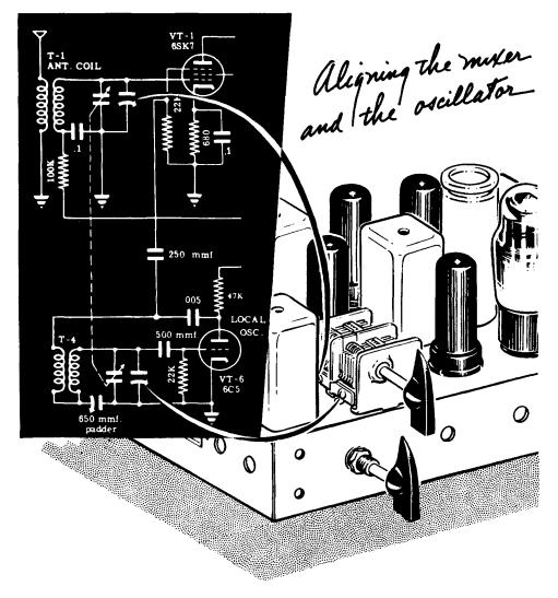
Demonstration—Aligning the Mixer and Oscillator (continued)
