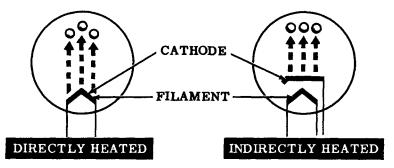
Because they can emit many more electrons than the indirectly heated type, directly heated cathodes are used in vacuum tubes designed for power supplies which supply high currents. Indirectly heated cathodes are more frequently used in low-current power supplies. Having the heater (filament) and the electron emitter (cathode) separate in an indirectly heated tube allows for the separation of the filament's and the cathode's electrical circuits.
