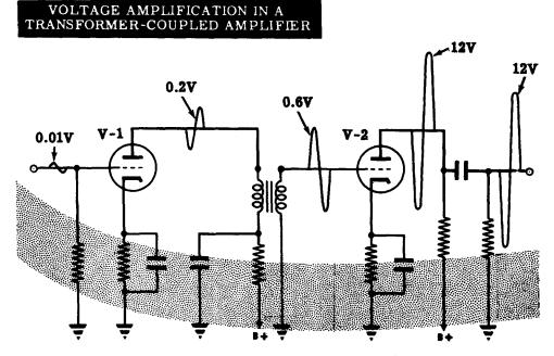
The voltage across the secondary of the transformer (0.6V) is now applied to the grid of V-2. If we assume that the gain of V-2 is equal to  $\mu$ , then V-2 will amplify this signal 20 times. Therefore, the output voltage at the plate of V-2 will be-20 x 0.6 = 12V.
