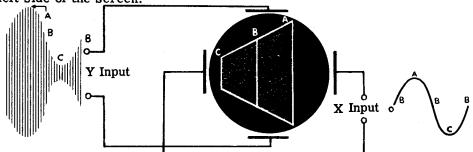
Because of the way in which trapezoid figures are obtained, they represent a graph of the output voltage as compared to the modulating voltage. If the output voltage is always proportional to the modulating voltage—as it will be when the modulation is linear—there will be a straight line along the top and on the bottom of the trapezoid.
