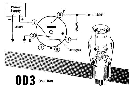
Notice that there is a "jumper connection" between pins 3 and 7 inside the tube. If pins 3 and 7 are wired in series with the circuit, this jumper will act as a switch. When the VR tube is pulled out, the circuit requiring the 150 volts will be disconnected from the power supply. If this jumper were not connected as a switch and the VR tube were pulled out, the 150 volt circuit would receive more than 150 volts—resulting in damage to its components or in improper operation.
