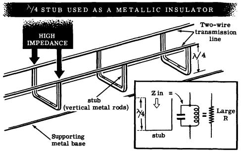
The shorted quarter-wave stub also makes a very effective filter for harmonic frequencies of the fundamental which one does not desire to transmit. For the fundamental frequency the stub is a high impedance as was shown above. For the second harmonic, the stub is now a half wavelength long and will act as a short circuit across the transmission line, shorting out the undesirable harmonic and preventing it from getting to the antenna.
