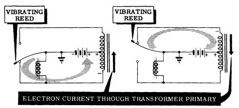
When the vibrator reed hits the lower contact, it puts a direct short across the electromagnet coil. This causes the magnetic field to collapse. Since the electromagnet can no longer hold the reed against the lower contact, the reed springs back past the center position and strikes the upper contact. When the reed strikes the upper contact, the following things happen.
