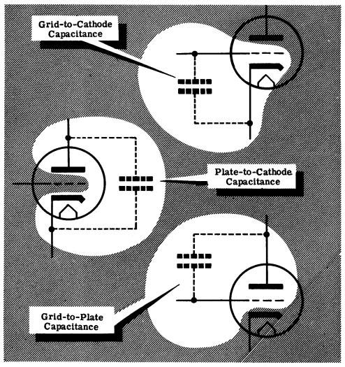
The grid-to-plate capacitance is the one which causes most of the trouble. At high frequencies it produces undesirable effects which may prevent the tube from amplifying properly. This will be explained later.
