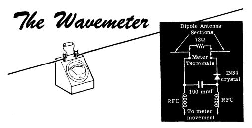
The instructor places the wavemeter far enough away from the transmitting antenna so that the meter needle does not deflect off scale. Then, the transmitter frequency is varied until the meter goes through a peak reading. At this point the transmitting antenna is exactly a half-wavelength long and is therefore radiating at maximum.
