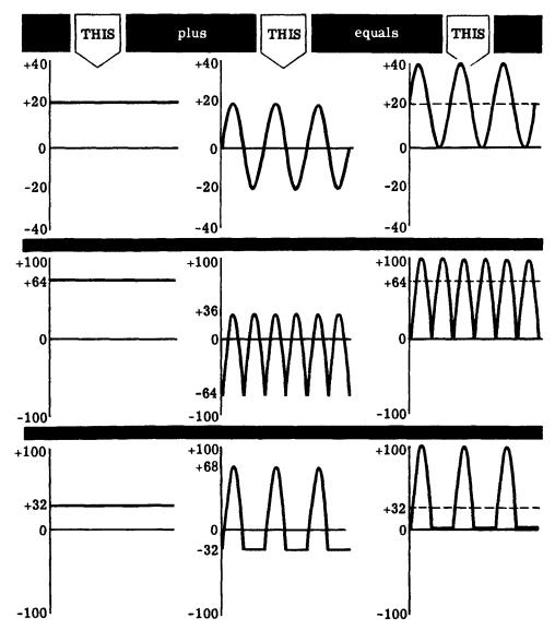
You can see that as long as a voltage varies in any regular manner, it can be broken up into a DC component and an AC component. The output of a rectifier contains both a DC component and an AC component. It is the job of the filter to remove as much of the AC voltage as is possible (and economical!) before the resulting high voltage DC is fed to the electronic circuits which require it.
