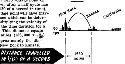
When another half cycle or a total of a full cycle has elapsed (1/60 of a)second), the zero voltage point will have traveled a distance of 3100 miles
