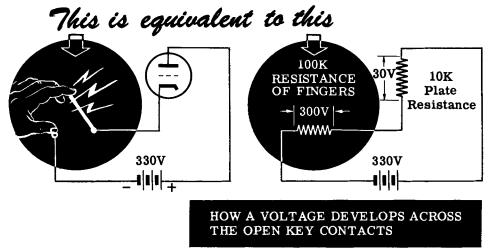
To safeguard the operator, a slight variation is made on this basic circuit. The variation involves the use of a relay. The key is connected to a low voltage circuit containing the coil of the relay. When the coil of the relay is energized, the contacts of the relay, which are in series with the cathode circuit close, permitting the stage to operate normally.
