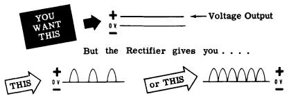
The job of the filter circuit is to smooth out the pulsations in the rectifier output and give you a steady voltage with little or no ripple. Filter circuits come in various forms, but all filter circuits are made up of various combinations of inductances and capacitors or resistances and capacitors. You will learn how these filter circuits work to smooth out the pulsations in the rectifier output as soon as you have done some work with various rectifier circuits.
