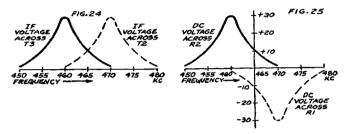
Fig. 24. The frequency response curves of T2 and T3, Fig. 23, show that maximum voltage is induced at 470 kc and 460 kc respectively. These i-f voltages are induced in the secondaries because of the coupling between the several windings
