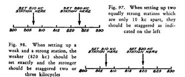
It should be observed that there is no distortion introduced as a result of the mistuning since the AFC action is capable of correcting for the mistuning of 3 kc in each station. This mistuning of course takes place only when the station is tuned automatically and does not occur when the AFC switch is off and the station is tuned in in the conventional way.
