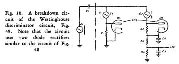
As to the signal voltages active in the circuit, the voltage which is effective in causing rectified current to flow through R1 is E1 + E2 and the voltage which is effective in causing rectified current to flow through R2 is E1 + E3.
