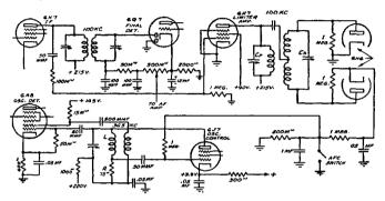
Fig. 70. The double-superheterodyne AFC circuit employed in the Westinghouse Model WR-315 receiver. The limiter amplifier, discriminator, and oscillator control circuits are shown in detail
