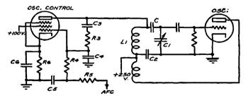
Fig. 65. A basic oscillator control tube circuit, showing how it is connected to the oscillator circuit. R3 and C4 supply the lagging grid voltage, while C3 keeps the d-c voltage from the grid of the control tube
