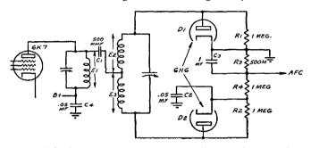
Fig. 49. The discriminator circuit that is employed in the Westinghouse WR-315 receiver
