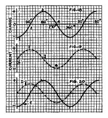
The charge on C in Fig. 17 follows the sine-wave variation of the voltage, see Fig. 18: the positive and negative peaks of charge occur at the same instant as the voltage peaks. The current in Fig. 17 follows a sine-wave variation, but its zero values occur when the charge goes through its peak values as shown Fig. 19. In Fig. 20 both voltage and current waves are plotted on the same axis, showing that the current I leads the voltage E by one-quarter cycle, or 90°
