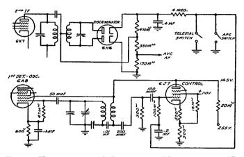
Fig. 73. The AFC circuit of the Grunow Model 12-B receiver. The discriminator circuit is conventional, but the control tube circuit differs from those previously discussed
