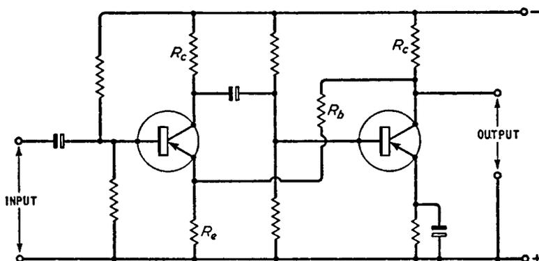
Fig. 7.6. A two-stage transistor voltage amplifier having high input resistance and low output resistance
