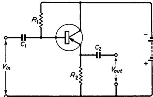
Fig. 5.4. Practical circuit of a common-collector amplifier
