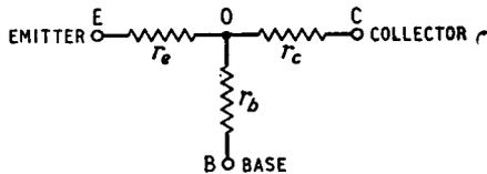
Fig. 3.2. A three-terminal passive network which can be used to build an equivalent circuit for a transistor
