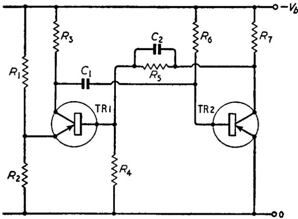
*Fig. 12.5. Transistor monostable multivibrator*
