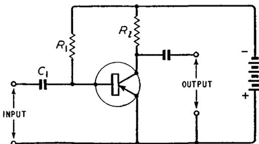
Fig. 4.5. Practical circuit for a common-emitter amplifier
