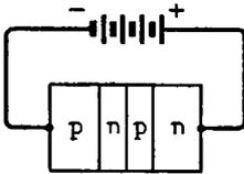
*Fig. 14.5. Reverse-biased controlled rectifier*
