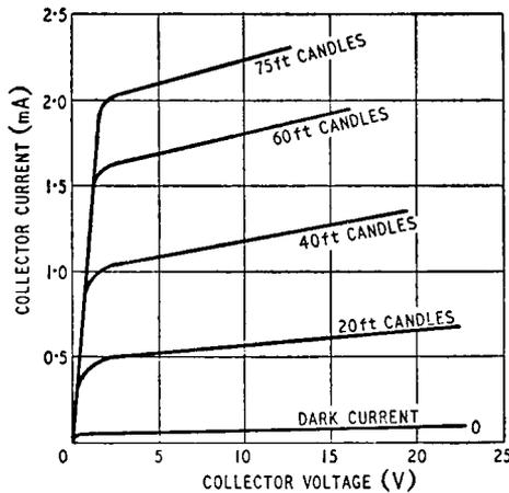
Fig. 13.12. Characteristics of a photo-transistor
