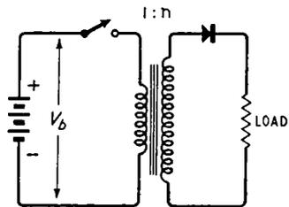
field would in time reach its maximum value and become static: there would then be no secondary voltage. However, before this instant is reached, the switch is opened and the magnetic field collapses suddenly, setting up a secondary e.m.f. with a polarity opposite to that set up on closing the switch. This e.m.f. does
