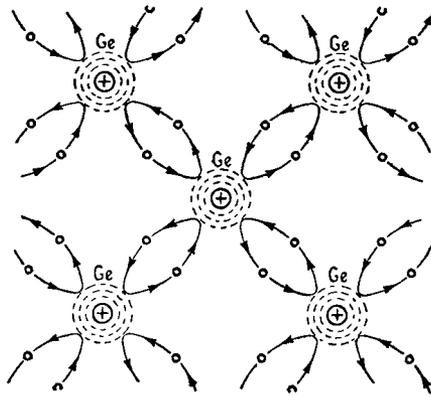
*Fig. 1.5. Illustrating covalent bonds in a crystal of pure germanium :
