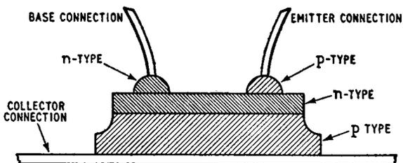
Fig. 2.9. Construction of a Mesa transistor
