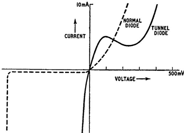
Fig. 14.3. Characteristic of a tunnel diode (solid) compared with that of a normal junction diode (dashed)
