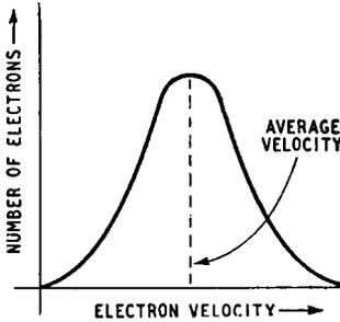
*Fig. 2.10. Distribution of electron velocities about the average value*
