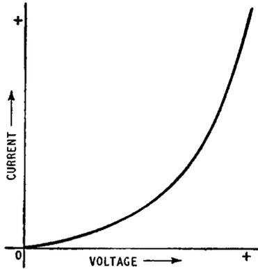
voltages because the internal potential barrier discourages movements of majority carriers across the junction. Increase in applied voltage tends to offset the internal barrier and current increases at a greater rate. Further increase in voltage almost completely offsets the barrier and gives a steeply-rising current. The curve is, in fact, closely exponential in form.
