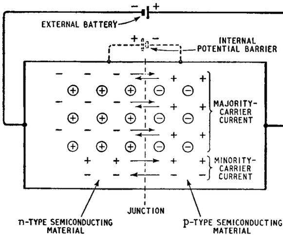
Fig. 1.11. Forward-bias conditions in a pn junction
