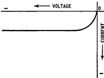
*Left: Fig. 1.10. Current-voltage relationship for a reverse-biased pn junction*
