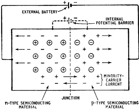
*Fig. 1.9. Reverse-bias conditions in a pn junction*
