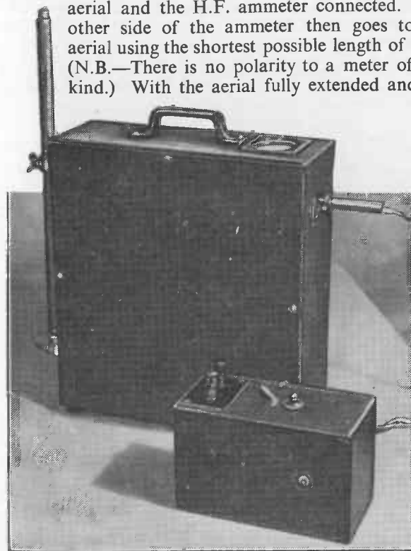
FIG. 25.—A transmitter in its case together with its associated control box. Note the plug and jack connection on the transmitter.
