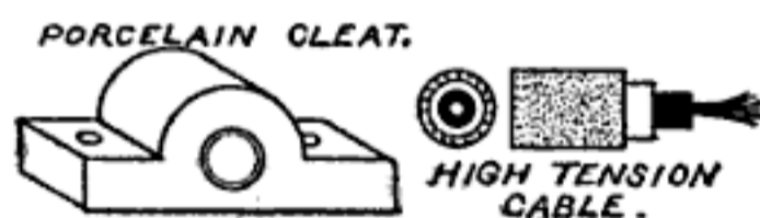
Fig. 21. High-tension Cable and Insulator.
