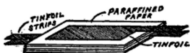
Fig. 39. Construction of a Paper Condenser.
