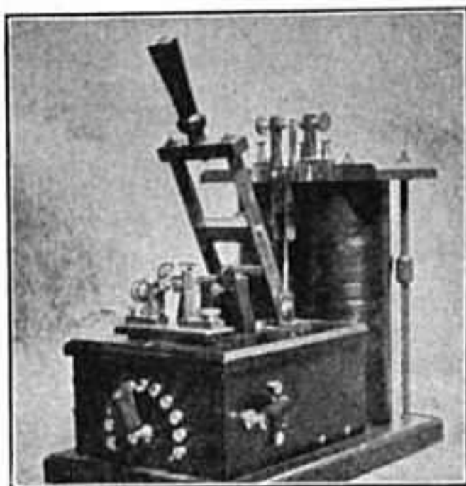
Fig. 126. United Wireless Portable Receiving Set.
