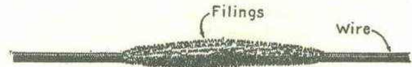
FIG. 81. — Iron Filings Clustered on a Wire Carrying a Current of Electricity.
