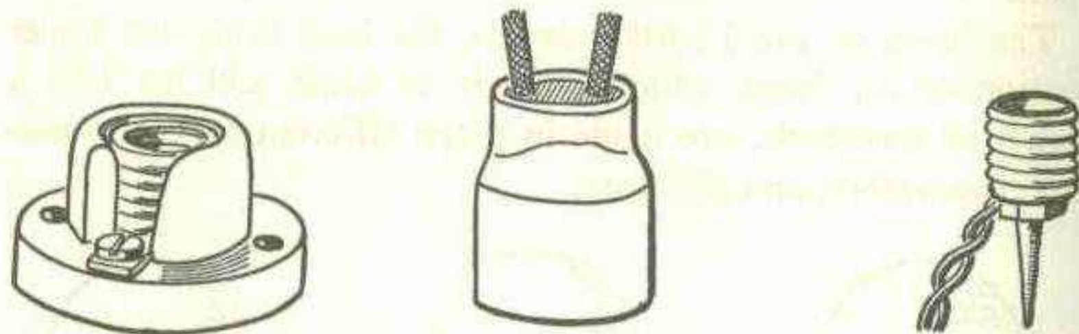
FIG. 267.—A Flat-Base Porcelain Receptacle, An X'mas Tree Socket and a Pin-Socket for Miniature Base Lamps.
