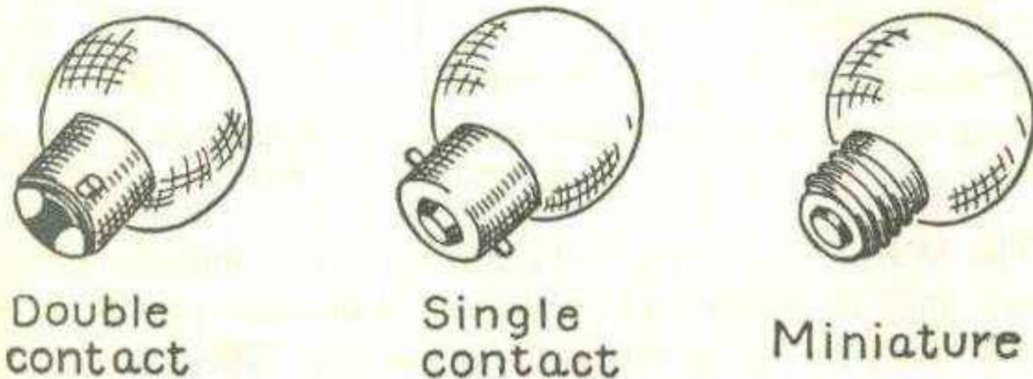
FIG. 266. — Three Types of Bases used on Miniature Lamps.
