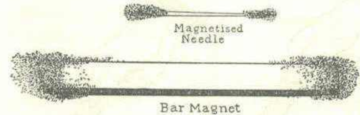
FIG. 9.—A Magnetized Sewing Needle and a Bar Magnet Which Have Been Dipped in Iron Filings. Notice how the Filings Cling in Tufts at the Ends.
