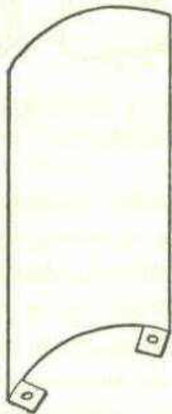
FIG. 289. — The Reflector is bent out of bright tin.
