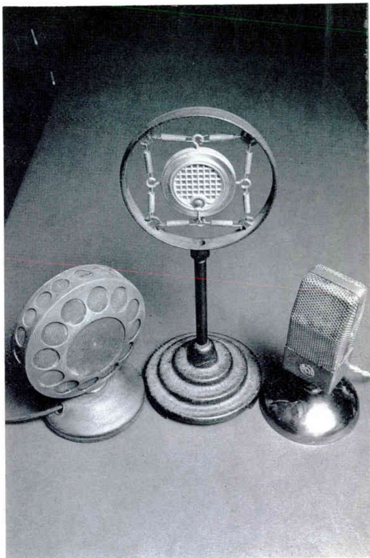
Three generations of microphones (left to right): a carbon mike from 1922, an improved double-button carbon mike from 1926, and an RCA model 44 mike from the late 1930s. (Courtesy of Pequod Restaurant, Morton Grove, Ill.)
