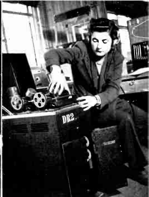
Monitor takes off the wax record from her recording machine after a bulletin.
