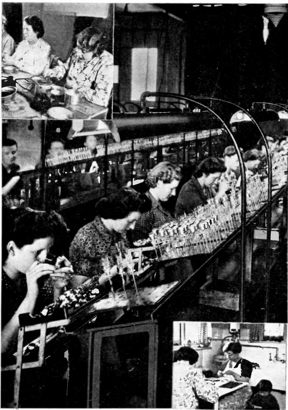
Two methods of manufacture which contributed to radio's war triumph. The main picture shows a production line in a valve factory. The insets show "outworkers" making up components in their homes.
