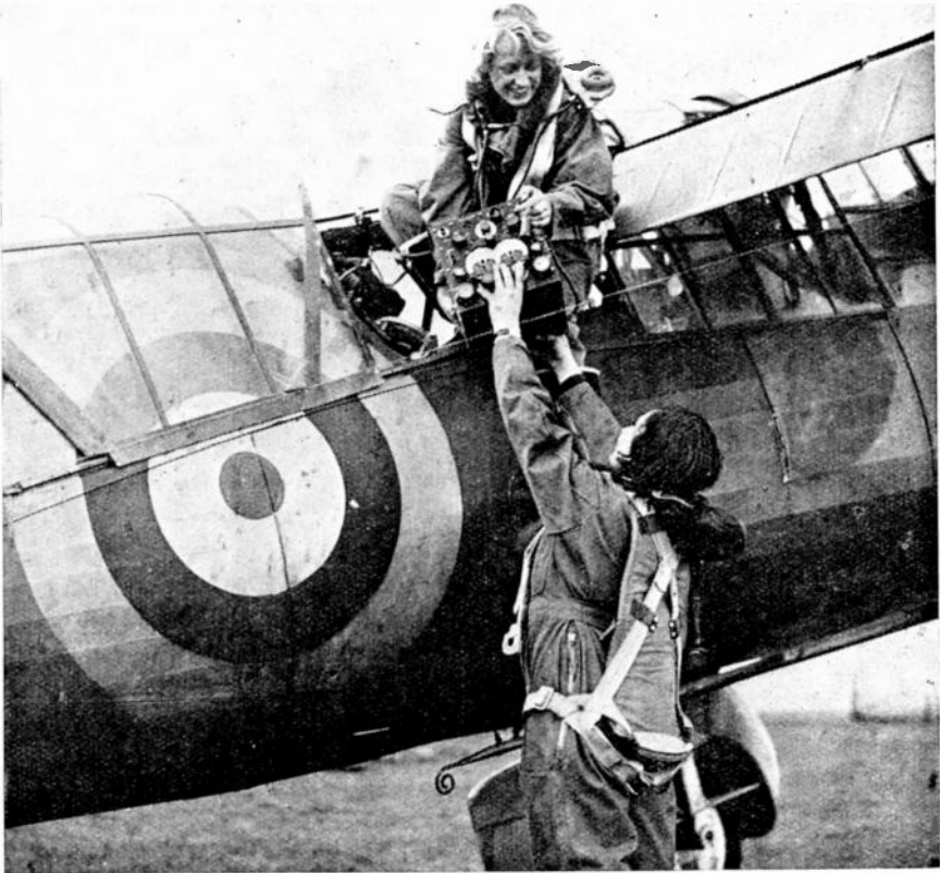
Wrens undertook much highly skilled work, including the servicing of radio equipment. These two Leading Wrens are installing a set in a Fleet Air Arm plane. When the sets are fitted, the Wrens test them, on the ground and in the air.
