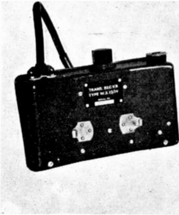
Beautifully designed transmitter-receiver sets, mass-produced for "agents". Little bigger than a miniature camera, they were worn on a belt round the waist, and worked from small batteries.
