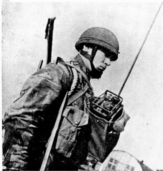
A lightweight portable radio telephone used by Airborne troops. The "38 Set", made in its tens of thousands.
