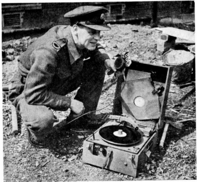
Portable recording unit. This device, more than any other, made it possible for the folk at home to hear the story of the war in faithful, dramatic detail. B.B.C. War Reporters took their clockwork driven portables and their microphones into places where no recording truck could go. The job they did was magnificent.
