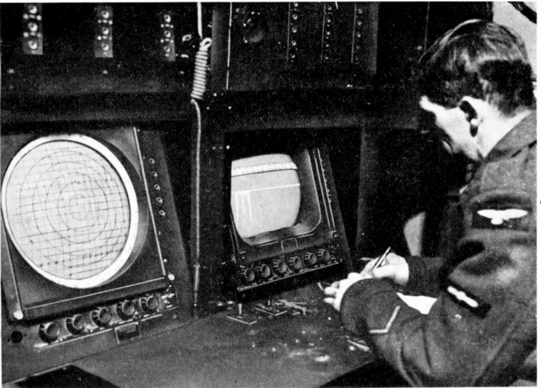
An R.A.F. radar operator on duty at a G.C.I. (Ground Controlled Interception) station. The cathode-ray tube on the left is the P.P.I. (Plan Position Indicator) and has a map of the appropriate section of England drawn upon it. Aircraft appear on this map as starry blobs. The tube on the right gives the range, which is measured off in miles against the scale.
