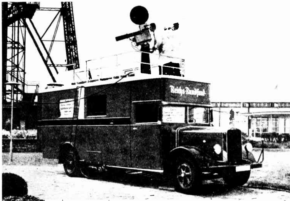
A Reichs-Rundfunk television remote truck equipped with an Intermediate Film Transmitter used between 1931 and 1940 in Germany.
